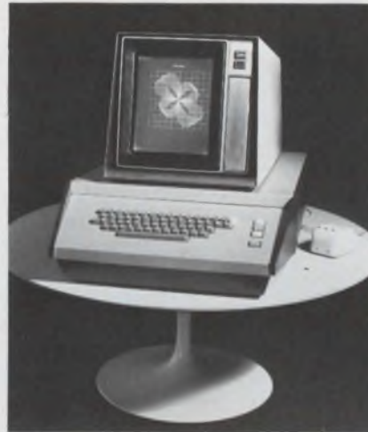
Storage tube display , using a Tektronix 611 CRT, is the poor man's route to graphical interaction. Computer Displays sells this one for $12,500 with "mouse" (right) or joystick control.
