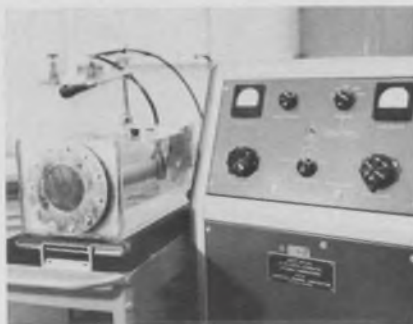
New image converter (left) turns ultra-sound to color pictures.
