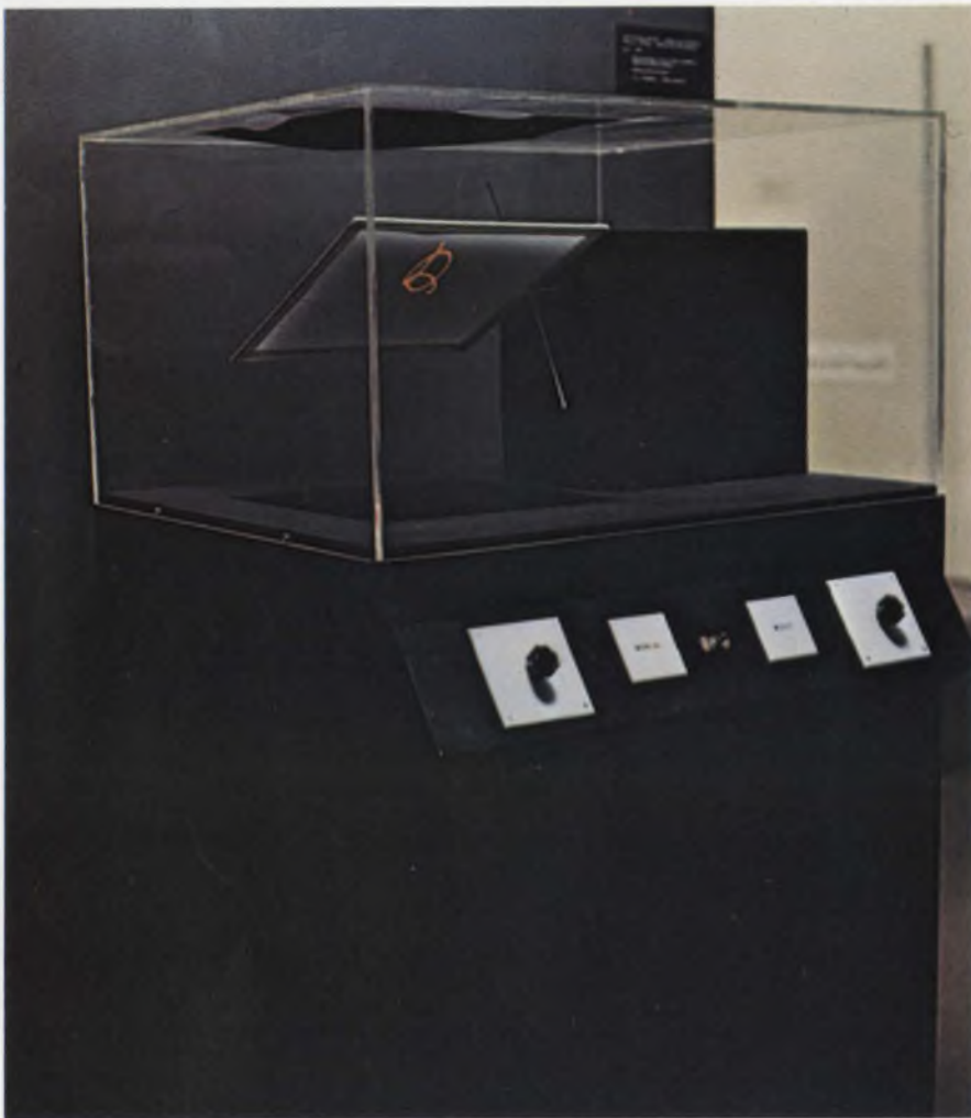
Music moves the laser beam that shines on a rotating card, producing three-dimensional patterns. "ELLI (Electronic Laser Light Image)" by artist John William Anthes and engineer Tracy S. Kinsel, allows an observer to control the beam with knobs on the panel.
