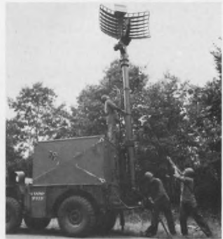
Mobile radar detects and identifies enemy planes at tree-top level.
