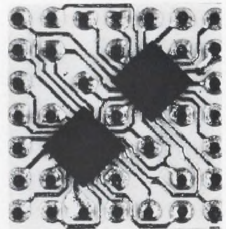
Two identical 64-bit, 3D-organized monolithic memory chips, made by IBM, are mounted, pads down, in a standard module.
