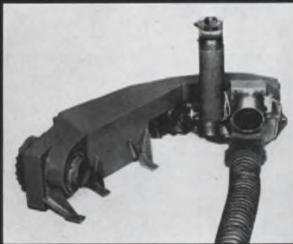
The laser range finding system of the Cheyenne AH56A is kept on the target by this compact cooling system.
