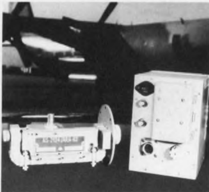
Airborne transponder responds to X-band signals from ground-controlled-approach radar with L-band signals, in order to penetrate precipitation.
