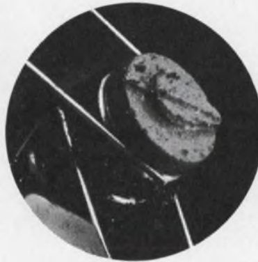
Brush assembly of conventional synchro after 1000 hours
