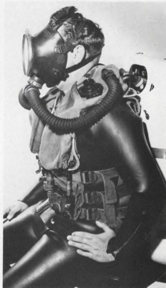
Navy diver wears semi-closed circuit breathing apparatus. Umbilical cable attaches to fitting on his right side. No communication or telemetry equipment is shown.
