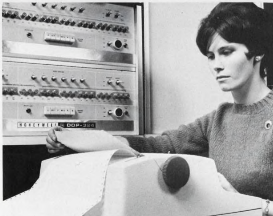
Dual processor computer performs 500,000 operations/s.
