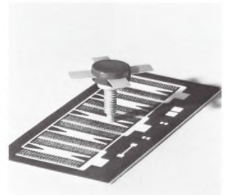
The Balanced Emitter Technology (BET) protects against the development of "hot spots" by providing nichrome resistors in series with each emitter, to facilitate an even current distribution throughout the entire transistor structure.
