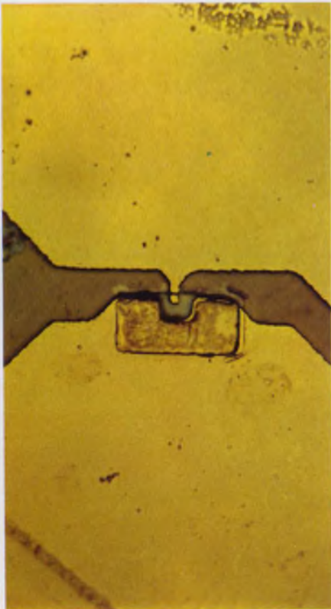
Detail of the Texas Instruments monolithic IC shows a Schottky barrier diode between a strip-line directional coupler and a matching section of the receiver front end.
