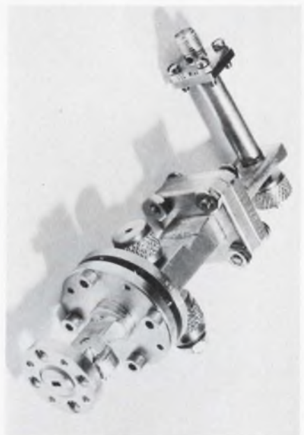
A three-stage multiplier made by Sylvania develops 5 mW at 94 GHz. The driver is an 11.75-GHz, 500-mW source. Cutaway (left) shows the middle doubler that raises the 23.5-GHz output of the first stage to 47 GHz. All waveguide components are electroformed so precisely that tuners have been eliminated.
