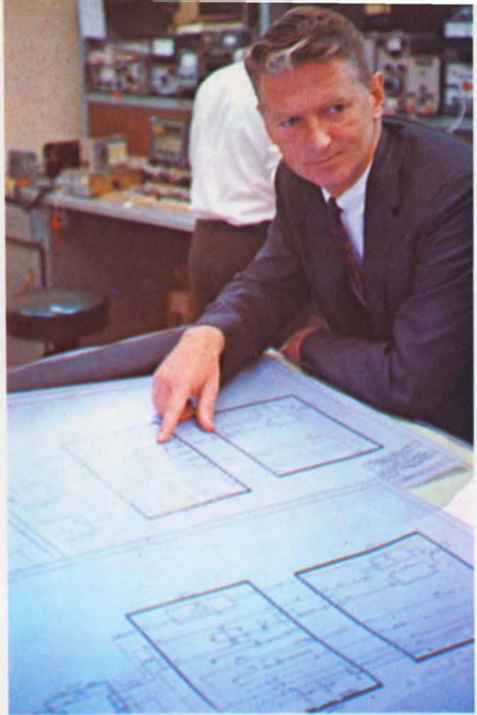
Rapid-transit systems require electronic routing and communications equipment that can withstand steel dust, explains Charles Kalkhof. They should be accompanied by two sets of blueprints: one "black-box" set (above) for use in the field, shows connections and test points for coded leads; a detailed schematic, for shop use, shows every component and every connection.
