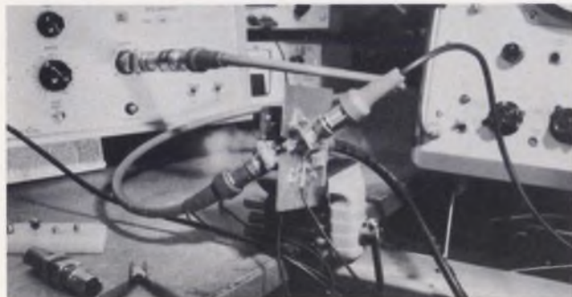
12. The finished jig. Input and output circuitry are mounted on opposite sides of a 2-sided PC board.
