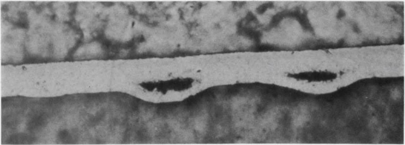
Occlusions in a gold deposit result when some electrolyte is trapped or embedded in the plate as shown in this cross-
