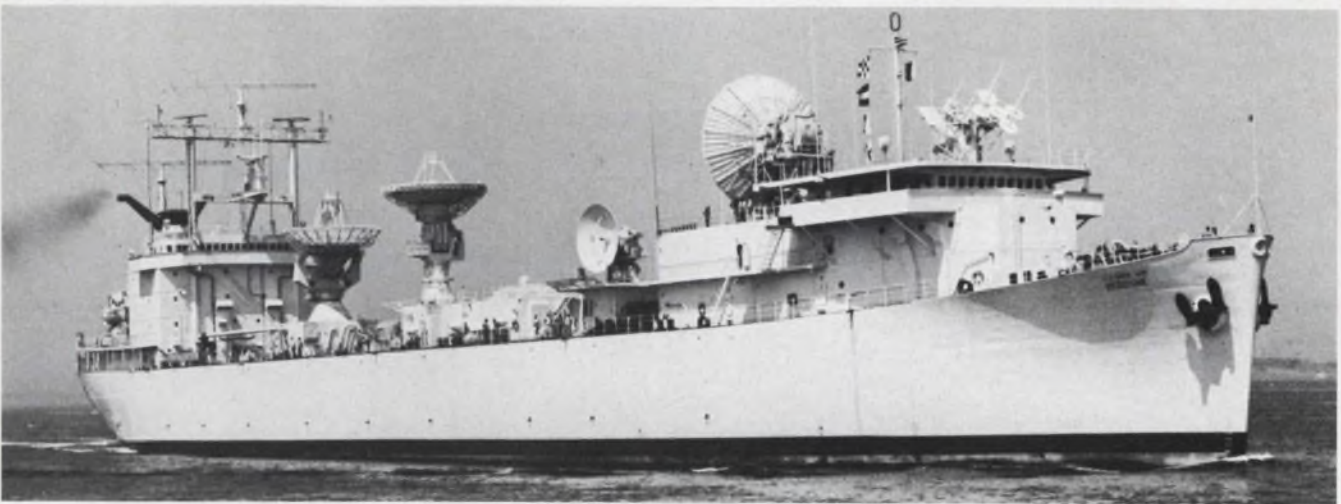
Former oil tanker has been rebuilt to become the best equipped of five Apollo vessels that
