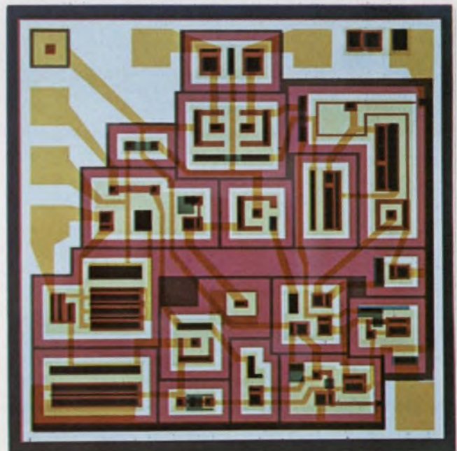
It's hard to find a resistor on the mask set of Widlar's LM101. Most of the high-value resistors are really dc-biased transistors, three are pinch resistors, and the largest ( R1 = 300\text{ k}\Omega ) is a buried FET. It is tricky to control its value, but the LM101 will work with a wide range, allowing Widlar to watch the buried FET in production.
