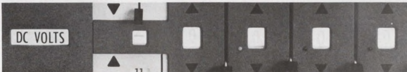
Follow the lighted arrows to an accurate 5-digit reading. This dc voltmeter has a "logic-
