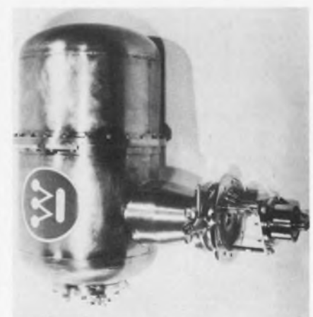
Prototype electron-beam welder developed by Westinghouse is slated for space applications.
