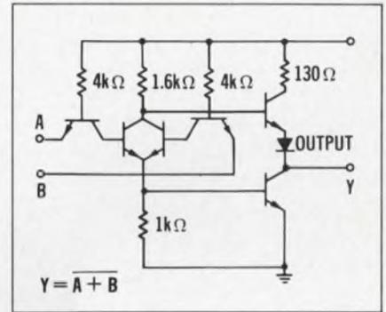
Designers may use the SN5402 with other Series 54/74 circuits... including complex-function types... to reduce overall system costs significantly below that possible with any other logic types.
