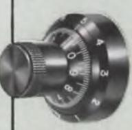
Calibrated dials designed for multi-turn potentiometers up to ten turns or other rotary devices. Requires only one inch of panel space. The knob attaches directly to the shaft, and the body of the dial is mounted rigidly to the panel. Therefore, accurate readings with a ratio of 1,000 to one for ten turns are provided with zero backlash and reading error.
