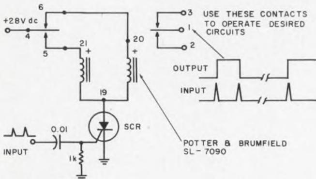
**Electromechanical flip-flop** has high gain and can be operated by very narrow input pulses.
