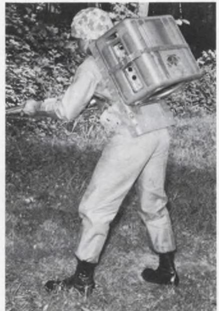
Portable thermoelectric generator weighs 35 pounds, with fuel.
