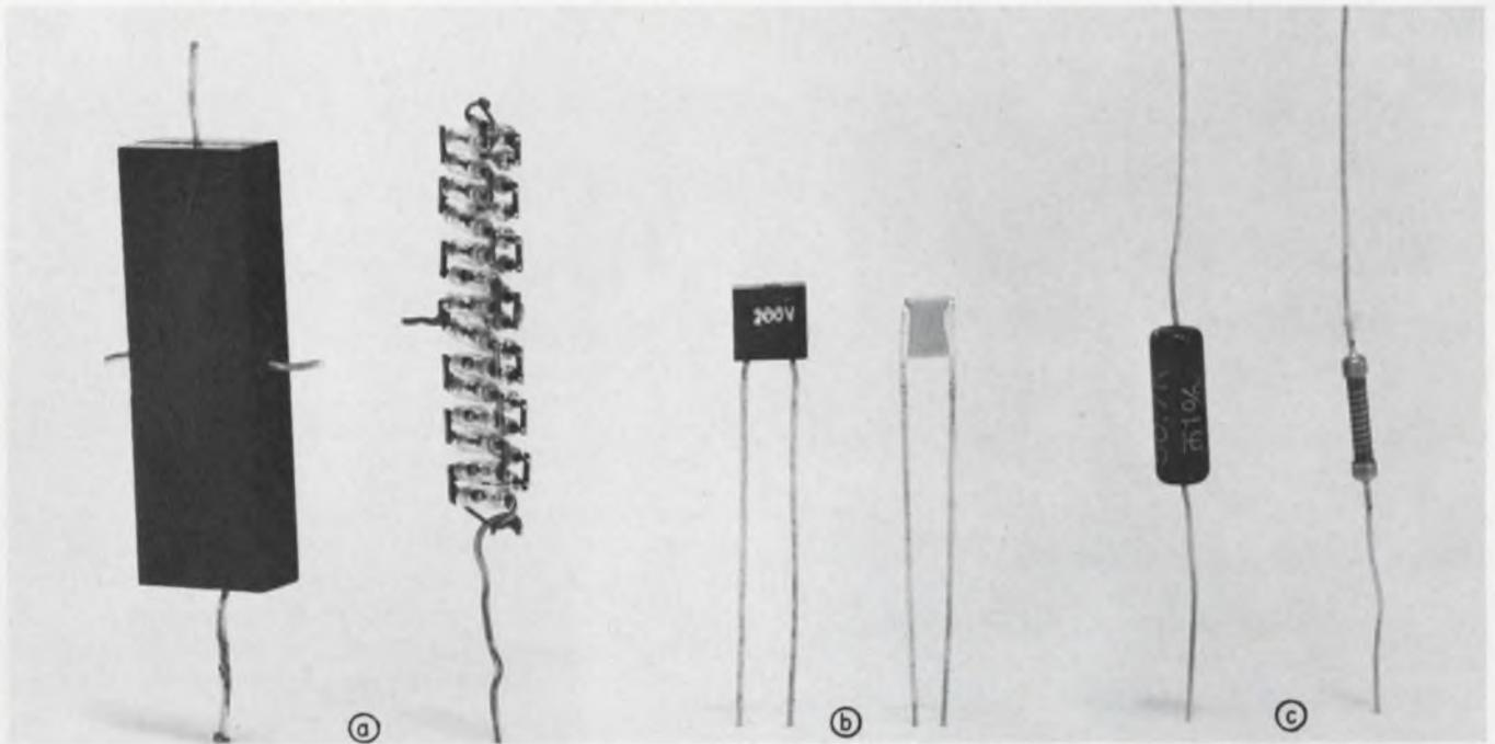
1. **Performance analysis of encapsulated components.** All were immersed in DeCap at 110°C. Glass diode rectifier assembly (a) showed glass breakage due to expansion and contraction of encapsulant and cold solder joints. Materials of construction are glass, plated copper leads, solder, methyl nadic anhydride-cured epoxy. Fra-
