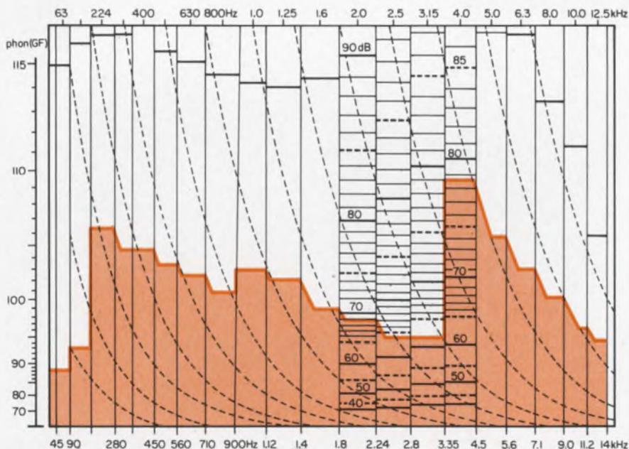
**Simplified Zwicker diagram** is similar to the display presented to the user of the loudness analyzer. Shaded region, representing a complex sound pattern, is integrated to provide an absolute sound intensity reading in sones on an adjacent meter. Note the curved vertical lines which define the threshold which sounds in higher frequency bands must exceed to be perceived as separate.
