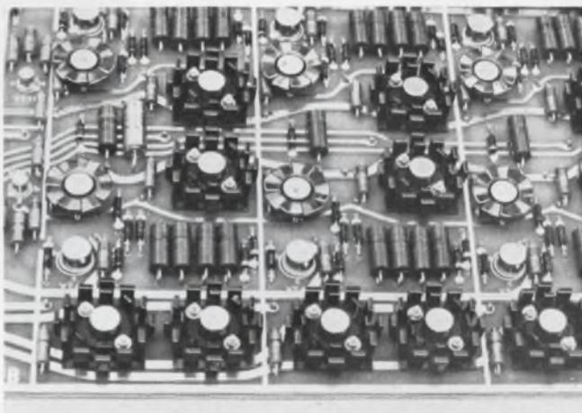
A 2N1837 transistor mounted only to a p-c board with IERC's unique LP dissipator can be operated at 5 watts with a junction temperature of only 153°C. The LP's clamping method makes good thermal contact on both surfaces of the transistor flange, minimizing thermal resistance from transistor to dissipator.
