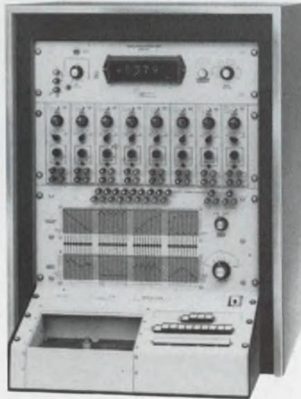
Now even a non-technical operator can speed through comprehensive DC tests on all types of IC packages with from 2 to 40 pins. Test conditions are easily set up on the programming switches of MICA-150 and pushbutton sequencing of the test from pin-to-pin of a device is simple and fast with test results indicated by direct digital readout. On a typical 10-pin, 5-input gate circuit, as many as 24 parameters of the device can be checked within two minutes without changing a single crossbar switch.
