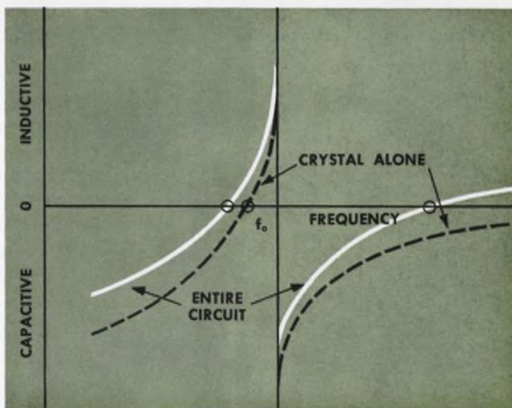
Figure 2 — Reactance-Frequency Plot for Typical Damon VCXO
