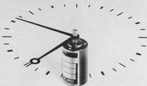
... try Globe's Type CC sub-miniature motor, one of the smallest a.c. hysteresis synchronous motors made. This tiny 2-ounce unit is only 21/32" dia. by 1.34" long. It's used extensively for MIL-spec timers, actuators, and drives requiring compact, exact-speed motors. Voltage is 26 v.a.c., 400 cps, single phase. Both 2- and 4-pole models produce .08 oz. in. sync. torque. Write for Bulletin CC, and ask us about production quantities.
