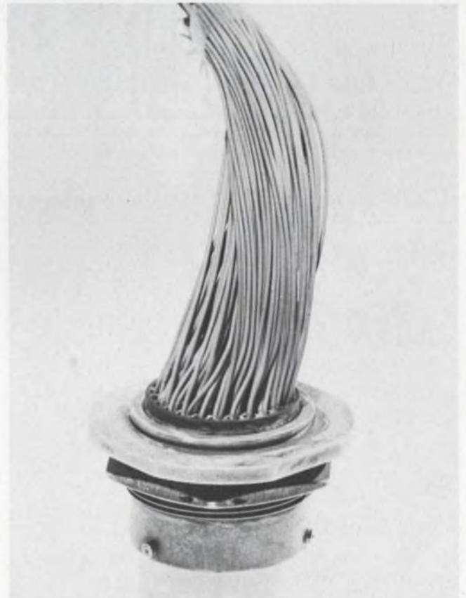
2. **To replace a faulty wire in this cable assembly,** Coast Pro-Seal 794 cured urethane encapsulant was removed with Uresolve. Materials of construction include anodized aluminum shell, neoprene insert, gold-plated connector, copper wire, irradiated polyethylene cable insulation and fluorinated silicone O-ring. The only material affected other than the urethane was the O-ring.
