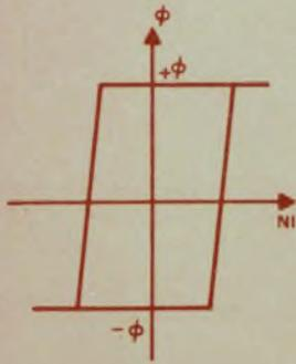
1. Square-loop hysteresis characteristic such as that exhibited by Orthonal or Deltamax constitutes the basic core requirement for the pulse transformer.
