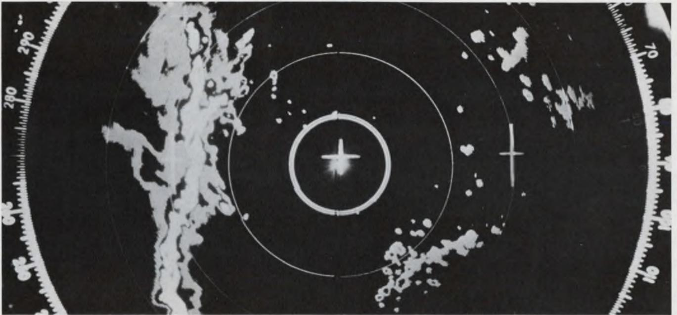
**New weather radar system** enables intensity of storms to be read directly off a scope face.
