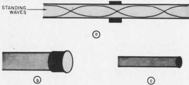
**Standing waves** occurring within hollow vhf antenna elements (a) can be avoided by sealing ends either with a plastic cap (b) or with a small amount of epoxy.
