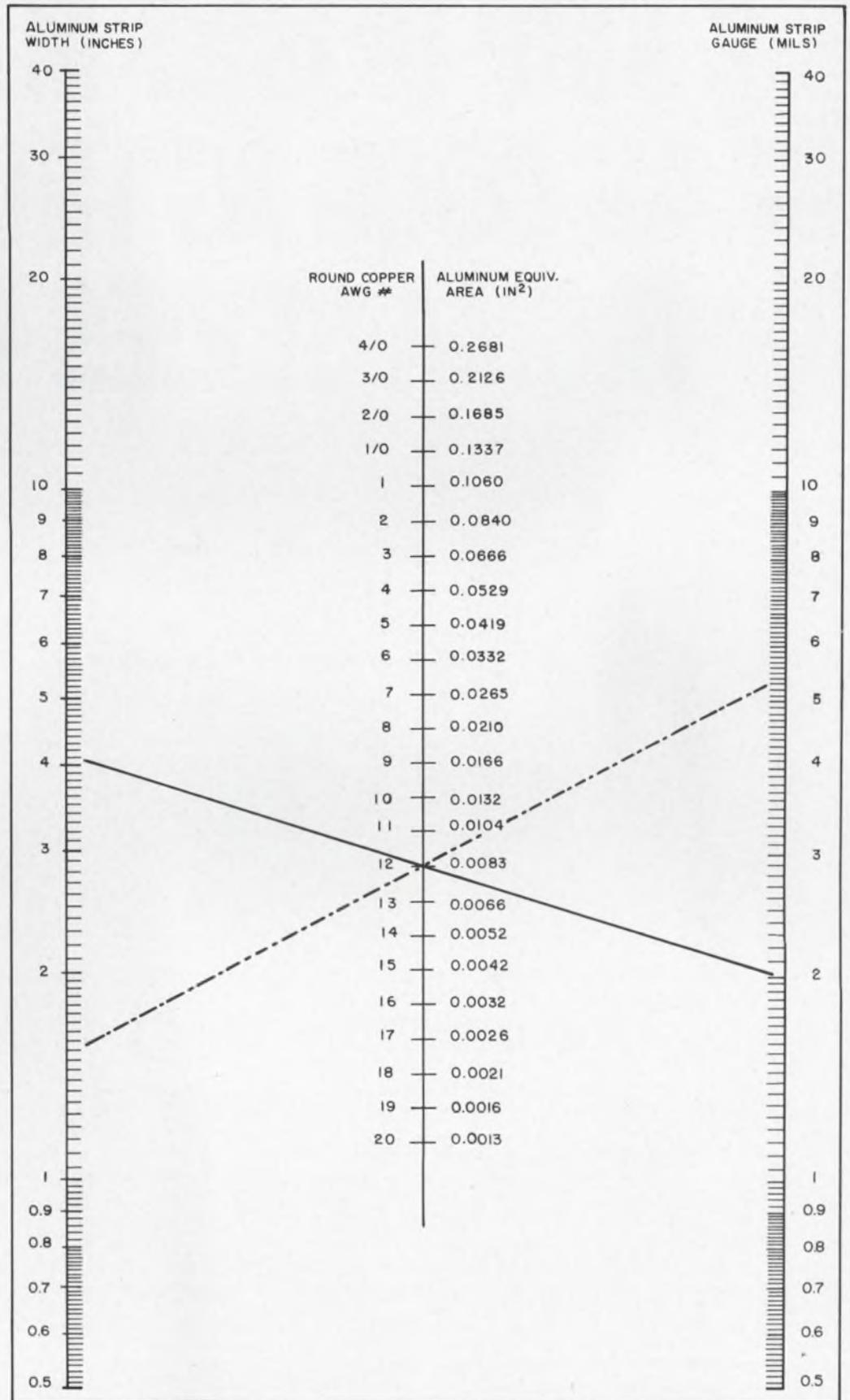
Aluminum strip equivalents for round copper conductors are found by pivoting a straight line through the AWG number of interest. Two equivalents for AWG #12 copper wire are shown above.
