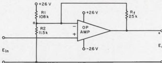
An operational amplifier has  $-6\text{-V}$  zero input voltage offset. Component values are calculated from Eqs. 4 and 6.
