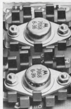
New dissipator for TO-66 transistor uses only 1.7 sq. in. of board space. IERC's unique, staggered-finger design dissipates 9 watts with case temperature of less than 150°C.
