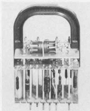
Mounting matched transistors for thermal stability so electrical characteristics stay identical is simple with back-to-back Therma-Link dissipators/retainers. Also used as heat sinks.
