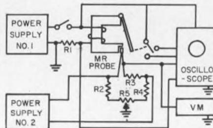
A magnetoresistor is placed in a recess in the contact end of the relay core. This probe is operated by its own power supply and, through a bridge circuit, its reaction to change in relay magnetic flux is indicated on a voltmeter and displayed on an oscilloscope.
