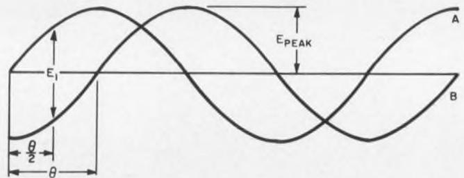
2. Maximum phase shift voltage occurs at  $\theta/2$  where  $\theta$  is the phase shift between the two sine waves.
