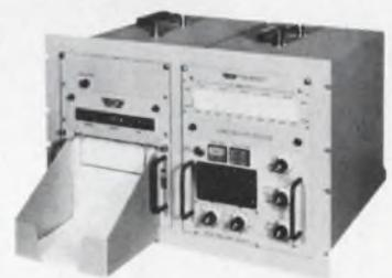
The BH103 incorporates a 100-point Scanner with direct digital readout and prints the data on folded paper. i.e., EVENTS, TEMP °F, TIME.
