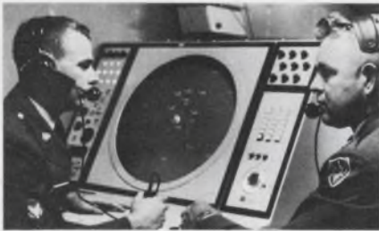
Display console of Missile Mentor uses symbols and alphanumeric characters to identify targets.
