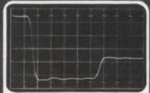
Time Domain Reflectometry (TDR) Display (with 281 Pulser) of 50 \Omega system, with transition to a 25 \Omega system. Any portion of the display can be expanded vertically and horizontally for more detailed analysis. 100 mV/cm—5 ns/cm
