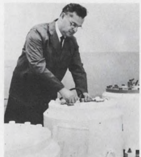
Submersible nuclear generator, fueled with strontium 90, produces 3 watts.
