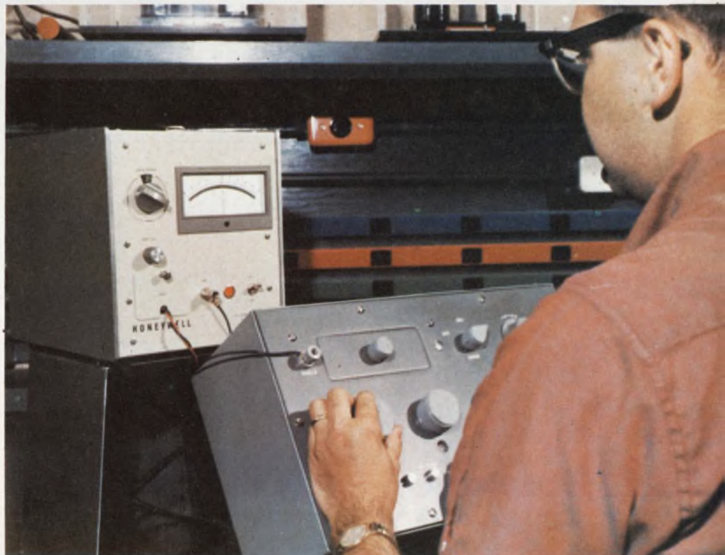
Microvolt null detector operated by Honeywell metrologist measures the potential difference between two standard cells (not shown) (Paper 59/2).
