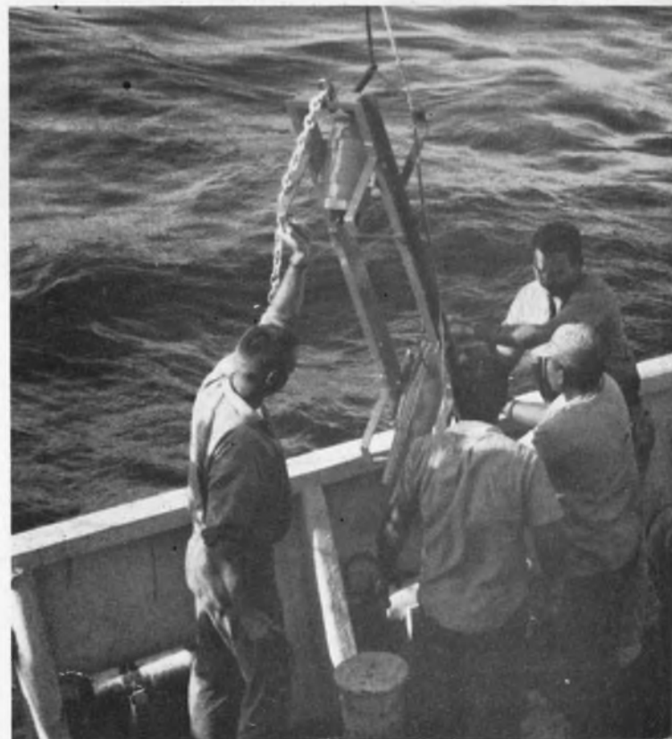
An acoustic transponder signals the location of an under-sea camera and helps to position it above the sea floor.
