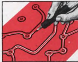
With sharp blade, outline the areas to be masked. Do not cut through the backing sheet. The Ulano Swivel Knife does the job quickly, easily.
