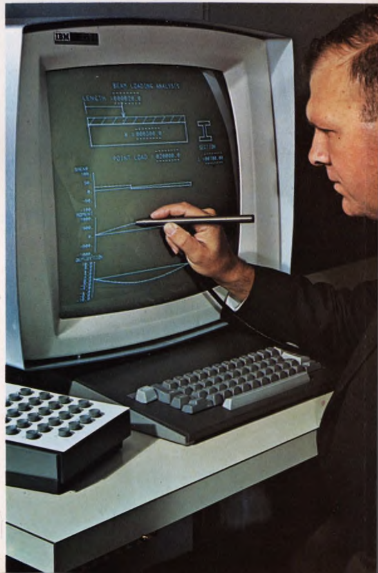
Design engineer uses a light pen to feed data into a digital computer which performs the computations necessary to solve a mechanical engineering problem (Paper 24/4).
