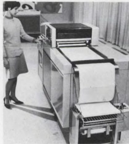
Continuous computer output is reproduced by high-speed Xerox copier that can be housed alongside the computer.
