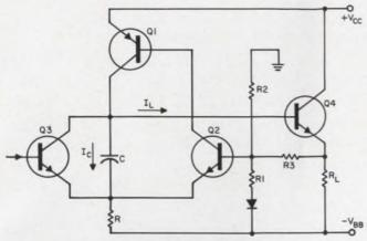
2. Ultralinear current source uses only four transistors. All transistors should be high-speed, high-beta, low-leakage. In particular, Q2 should have high beta at low collector currents. Timing capacitor C should have flat characteristics over the operating temperature range.
