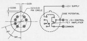
Spdt relay and FET driver are mounted in standard TO-5 can. Supply voltage is 12 Vdc nominal and relay coil is rated at 500  $\Omega$ .
