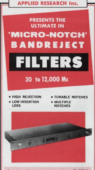
A series of *Micro-Notch Bandreject* FILTERS have been developed by APPLIED RESEARCH Inc. to provide high rejection for specific frequencies over the frequency range of 30 to 12,000 Mc. Undesired signals within one percent or less of the operating frequency are eliminated. Various models are available including octave bandwidth units with tunable reject notches and low VSWR throughout the operating range.
