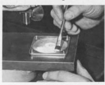
G-E two-part RTV, available in a range of viscosities, seals filament condenser plate in dielectric heater. Also protects against vibration.
