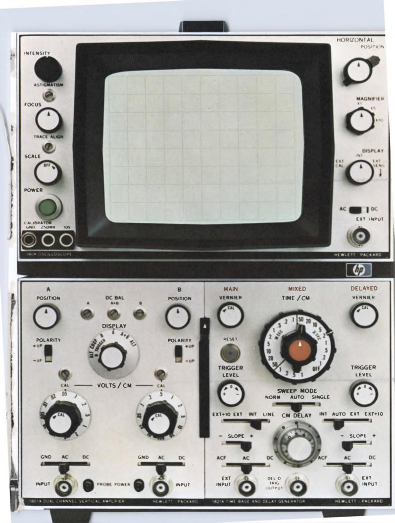
hp 180A Oscilloscope is shown here ACTUAL SIZE:
