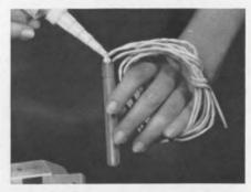
G-E RTV is ideal for high temperature moisture sealing of heating elements. It withstands temperatures as high as 600°F, as low as —75°F.
