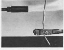
Silicone rubber wire and cable insulation passes UL vertical flame tests and is frequently used in high-voltage circuits.
