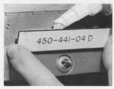
Screws and drilling are eliminated by adhering identification plates with RTV sealant. It won't harden, soften, crack or shrink.
