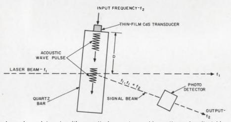
Laser beam interacts with acoustical wave to provide continuously adjustable delay for RF and microwave signals. The delay depends on the distance D.
