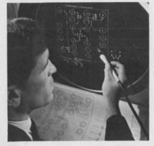
**Computer-aided computer design** with a computer-controlled graphic display and light-pen. Final hard-copy drawing is used to make mask for actual fabrication.
