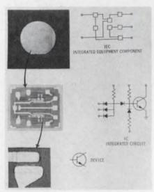
1. Integrated equipment components perform complex logic functions (top) as opposed to conventional integrated circuits (middle) which perform simple logic functions. These, in turn, are compared with the single transistor (bottom) which cannot perform any function independently.
