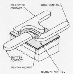
New junction seal shown on epitaxial silicon transistor.
