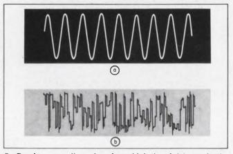
5. Random sampling of a sinusoidal signal (a) results in the collection of samples shown in (b). All time information about the original waveshape is lost but the probability distribution of both waveforms is identical.
