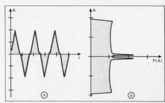
3. Crossover distortion of the equiprobable triangular waveform (a) is easier to detect if the signal's density function (b) is examined.
