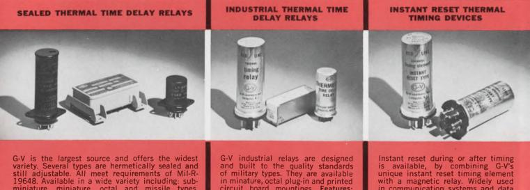
still adjustable. All meet requirements of whether 19648. Available in a wide variety including: sub-miniature, miniature, octal and missile types. **Features:** delay time, 0.1 sec. to 3 min.; heater voltages to 230 V; ambient operating temp.,  $-55^{\circ}$ C to  $+125^{\circ}$ C; vibration to 2000 Hz; shock to 50g.
