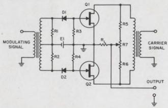
1. FET balanced modulator gives 180° zero-crossing phase shifts as the resistances of Q2 and Q1 are modulated during the first and second half cycles, respectively.
