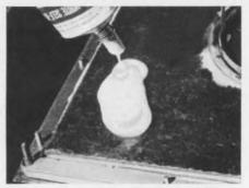
Laminated layers of mica sheeting are securely bonded with G-E RTV silicone sealant. Ready to use, it bonds to most materials.
