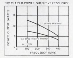
When you apply ITT 2N3375s, you get 5 watts minimum saturated power output at 400 MHz and Vcc=28 V, tested 100%.
