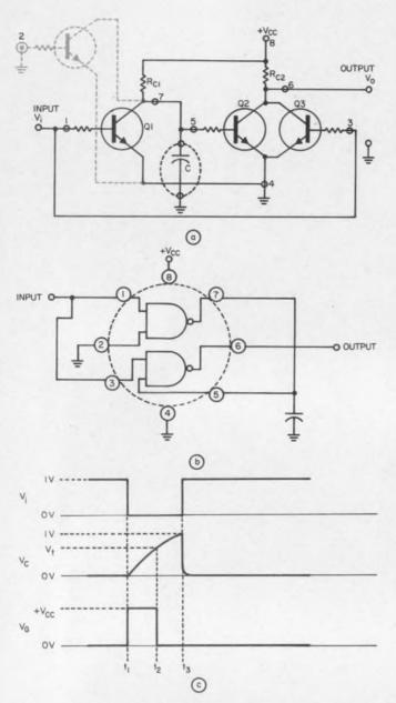
**RTL microcircuit**, with the addition of a capacitor (dotted loop), produces a pulse of period  $t_2-t_1$  when the input voltage shifts from a high to a low state. An RTL block (top) is connected as shown below with the pin 2 input grounded.
