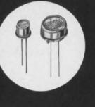
Clairex Type 7H Photocells now offer decay times of .006 sec @ 100 ft-c. Couple this with 240 ohms @ 100 ft-c, CdS stability, and your problems are solved. Available in TO-18 and TO-5 cases. And 6 resistance ranges.
