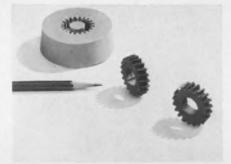
For prototypes or short-run parts production, G-E RTV is an excellent flexible moldmaking material. And it needs no release agent.
