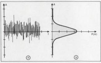
2. Gaussian noise (a) is described statistically by the familiar normal, or Gaussian, distribution curve (b). It is from this description that Gaussian noise gets its name.
