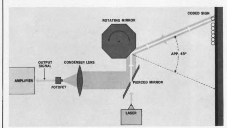
Laser beam reads signs on the side of box cars by focusing the binary-coded reflected light onto a photo field-effect transistor. The transistor output is amplified and fed into a computer or printer.
