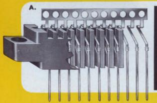
A. Tail stability is provided by the comb contact construction which permits force fit through the insulator.
