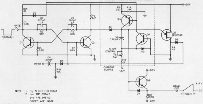
4. Type-II ramp generator uses a unijunction transistor to improve linearity. This circuit is particularly useful for
