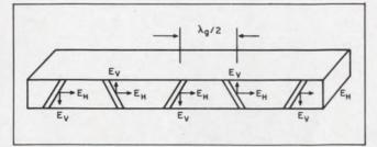
1. In an edge-shunt slotted waveguide array antenna the horizontal field components,  $E_{\rm H}$ , are in phase and the cross-polarized components,  $E_{\rm v}$ , are out of phase for adjacent slots. The spacing between slots depends on the half-wavelength in the guide,  $\lambda_{\rm g}/2$ .
