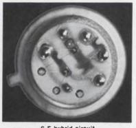
G-E hybrid circuit for multi-vibrator applications.
