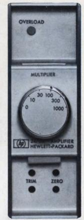
Built-in reliability: The predicted MTBF of the 2470A is in excess of 20,000 hours. Silicon transistors are used throughout, and passive and active components are selected for dependability, as well as performance. Amplifier meets spec at 95% humidity at 40°C. Critical para-meters (zero drift, full-scale accuracy, common mode rejection) are verified after 100 hours of "run-in" at elevated temperature.
