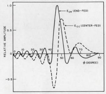
2. Calculated cross-polarized radiation pattern shows difference between end-fed and center-fed arrays. The array has 20 slots, the wavelength is 32 mm and the distance between slots is 22.35 mm.
