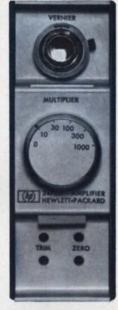
Use if for: Amplifying signals from low-level resistive transducers, such as thermocouples, strain gages. High input and low output impedance make it ideal for amplification over long transmission lines; use it. with resistive or reactive loads, such as x-y, strip-chart or oscillographic recorders, digital voltmeters, null detectors and servo systems, telemetry systems ... or use it as a highperformance bench amplifier.
