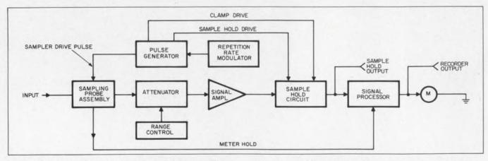
6. Waveform sampling can be accomplished by using a sampling voltmeter. A block diagram of an instrument of
