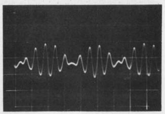
3. Typical output waveform shows the modulation of 3 -kHz signal by a 300-Hz one. The vertical scale is -50 mV/cm, and the horizontal,  $500 \mu \text{sec/cm}$ .
