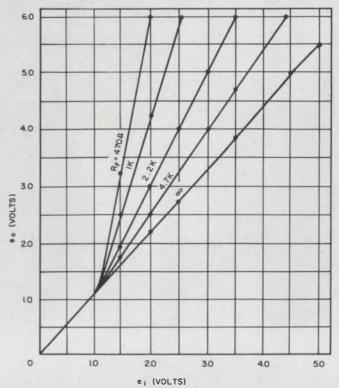
2. The transfer characteristics of the amplifier may be adjusted by varying  $R_{\rm F}$ . The diodes are biased into conduction at the break point of 1 volt.
