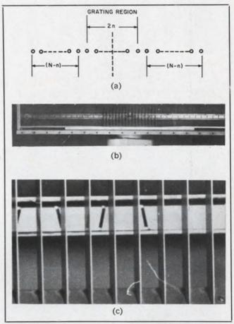
3. Partial grating across the center section (a) and (b) suppresses cross-polarization. For example, a grating, consisting of 16-mm wide and 0.5-mm thick metal plates, placed 12.5 mm apart, yields -20 dB attenuation (c).
