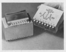
Impregnation of transformer coils with G-E RTV provides electrical insulation and environmental protection at high temperatures.
