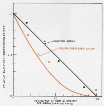
4. Measured suppression effects show good correlation with calculated values. Dots indicate measured results, solid lines represent calculated ones. The effect is more pronounced for Dolph-Chebyshev arrays (in color). The results are valid for an array having 38 slots and operating at 9375 MHz.
