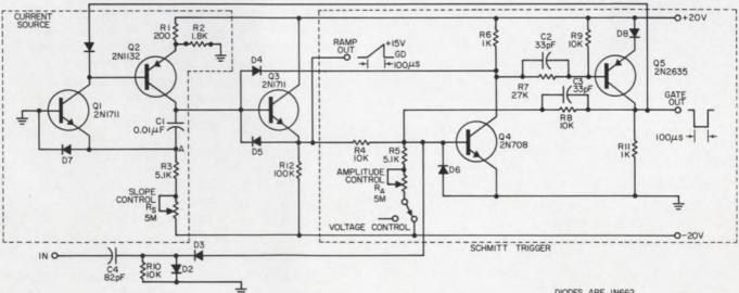
3. Type-I ramp generator has ramp and gate outputs. Pulse width modulation can be obtained by applying a
