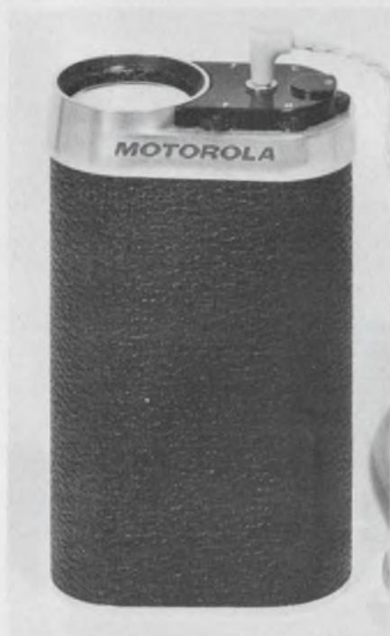
1. Motorola's experimental TV set is powered by four penlight cells.
