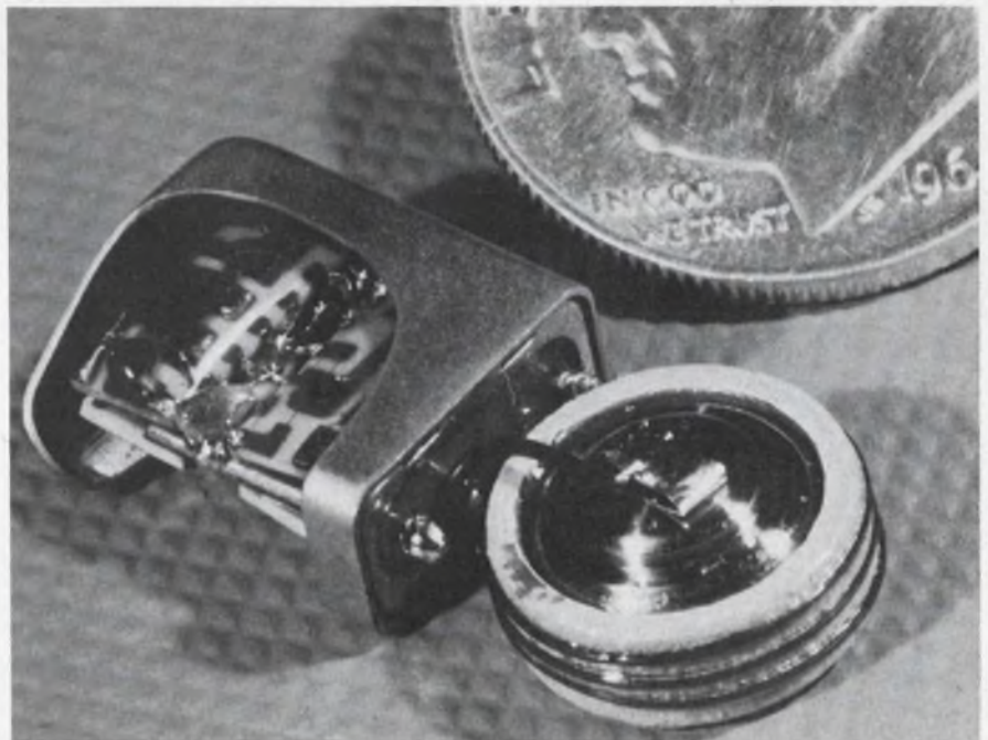
Microminiature temperature transmitter , designed to be implanted in a human body, is said to be capable of detecting temperature changes of 1/100 to 1/1000°C. Developed by NASA's Ames Research Center, the transmitter contains four hybrid integrated-circuit chips mounted inside a hermetically sealed can for protection from body fluids. The circular portion contains the battery and antenna and is usually left outside the body.
