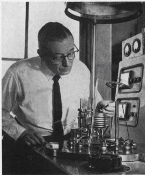
H. C. Theuerer of Bell Laboratories prepares to place a thin-film substrate in getter sputtering equipment.
