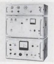
Diodes, rectifiers, transistors, and FETs are checked by model 259 in- or out-of-circuit. It measures both transistors and diodes, in-circuit, for reverse leakage down to 500 ohms of loading. It also measures FETs for leakage and transconductance, and both low and high power transistors for Beta  $(h_{je})$  within a 1 to 100 range.
