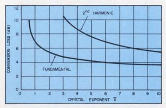
4. The actual conversion loss at the diode's junction may be expressed in terms of  $\bar{x}$ , which is d log i/d log v (a logarithmic relation of the diode's V-I characteristics). The loss decreases rapidly as  $\bar{x}$  increases. These curves were plotted while the image frequency in the mixer was matched. As a result, the diode has wide dynamic range.
