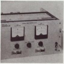
The Model 219A phase-lock tracking filter and phase comparator provides two identical  $100 \pm 3$  Hz channels and selectable noise bandwidth from 0.03 to 3 Hz. Phase slope is only 0.7 degrees/Hz. The system is entirely solid-state. Pulse outputs are furnished for use with an external digital phase meter. Applications are in the area of radio interferometry and other angle measuring systems.
