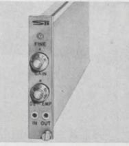
Features of the Model S-29 telemetry amplifier include a switchable de-emphasis circuit and a frequency response of 300 Hz to 2 MHz at a gain of 5 or less. In addition, dual inputs provide a low impedance for summing the outputs of the manufacturer's line of VCOs containing built-in mixing resistors. Output voltage is 20 V and current is 100 mA.
