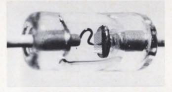
9. Schottky-barrier diode has a multiple pad surface which allows whisker contact to any one of the metal pads.
