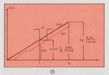
3. Longer time lags are the result of a ramp (instead of a step) function being applied to the input of Fig. 2a. A plot of the resulting output waveform (a) is used to determine the transient and error portions. Here  $C_1(t)$  represents
