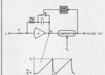
2. The simple addition of a feedback resistor and a one-shot to the circuit of Fig. 1a produces an A-to-F converter that operates up to 250 Kpps with a 0.01% linearity figure.
