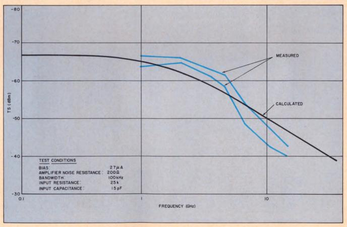
12. A comparison of measured and calculated sensitivity values for hot-carrier diodes indicates a close correlation.
