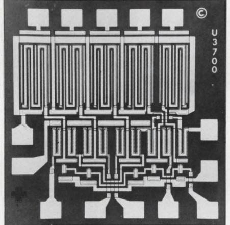
Multi-channel IC commutator has low on-resistance.
