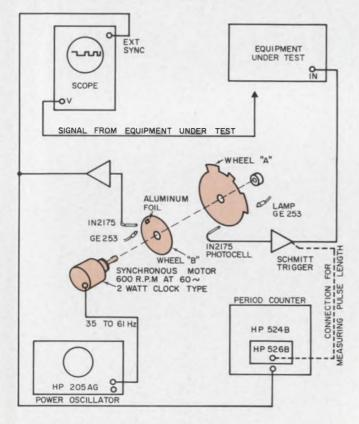
**Teletype signals are generated** by this variable-speed photochopping system. Wheels A and B produce the various facsimile and timing pulses. The system is also capable of viewing teletype signals. be cut for any type or degree of distortion. Accurate measurements of the pulse lengths may be made with an electronic time-interval meter by installing one disc at a time.
