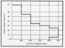
TYPICAL SPECIFICATIONS Input Voltage: 105 to 125 VAC Line Regulation:  $\pm 0.5$  to  $\pm 0.05\%$ (depending on model) Load Regulation:  $\pm 1.0$  to  $\pm 0.05\%$ (depending on model) Ripple: 5 to 1 mv (depending on model) No additional external heat sinking required. Write for Acopian's 16-page catalog and price list to: Acopian Corp., Easton, Penna., or call collect (215) 258-5441.
