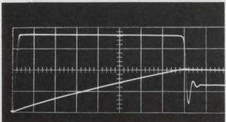
7. Step-up display performance: Coil voltage and coil current data taken from a single-ended deflection amplifier show good agreement with calculated values. For  $E_s$ =18 volts, L=25  $\mu$ h,  $R_L$ =0.5 ohms and  $T_c$ =50 ns, the system exhibited a settling time of 17.0  $\mu$ s. One vertical centimeter represents 5 units (volts and amps) and each horizontal centimeter 2  $\mu$ s. Voltage is displayed as a step function and current as a ramp.
