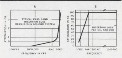
Graphs A and B show typical characteristics of Potter signal line filters. These filters are used on systems which must meet Defense Communications Agency criteria and provide maximum attenuation above the pass band with less than  $\frac{1}{2}$  db attenuation in the pass band.  $\blacksquare$  Write for further information on these and other Potter filters.
