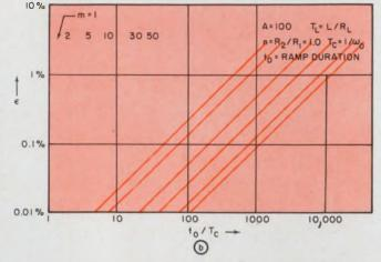
the ideal case and C(t) the actual signal. The amount of ramp delay is a function of both amplifier gain and bandwidth, and (of course) the system time constants ( $T_L$  and  $T_o$ ) (b).
