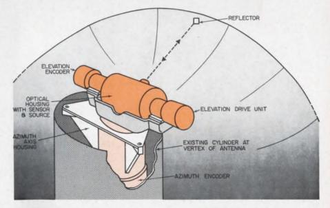
**Photoelectric sensor and source,** mounted on a platform at the vertex of the antenna, directs a laser beam at one of 1100 reflectors. The system is designed to detect surface deflections by measuring the angular coordinates of the targets with an accuracy of  $\pm 5$  seconds of arc.
