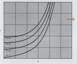
8. Either horizontal or vertical stepping can be used for carpet plotting. The choice depends on the particular set of curves.
