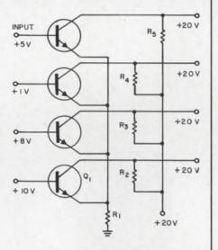
circuit. With the maximum input voltage on the base of  $Q_1$ , the base-emitter junction of  $Q_1$ will be the only one forward biased. Voltages on the emitters of all transistors, except  $Q_1$ , will be more positive than the voltages on their respective bases and they will be cut off. The output voltages of these transistors will be very high compared to that of  $Q_1$ .
