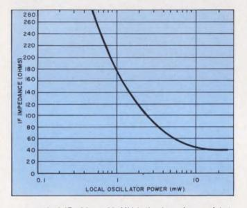
6. At typical IF (30 to 60 MHz) the impedance of hotcarrier diodes is a pure impedance and depends only on the level of the local oscillator drive signal. For hpa-2350 diodes the impedance is around 180 ohms at the optimum local-oscillator level of 1 mW. In the case of balanced mixers the combined impedance is about 90 ohms, el<sup>i</sup>minating the need for extra matching circuits for IF amplifiers.
