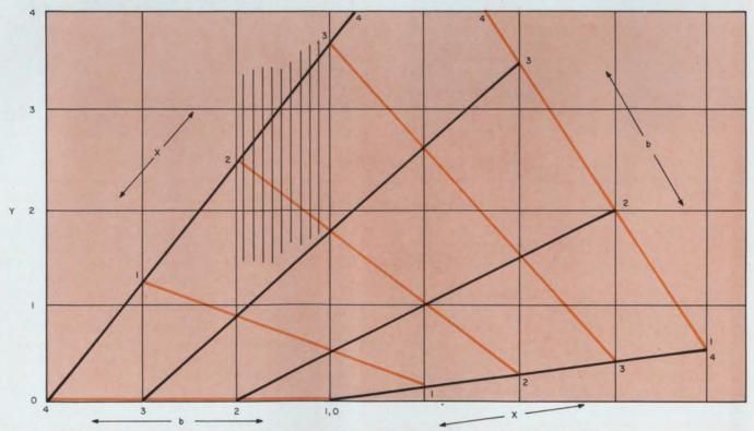
6. Joining of X = 0, X = 2, X = 3, and X = 4 points on overlay. Interpolation is the next step.
