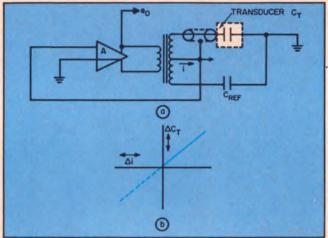
7. **Basic RF oscillator circuit** has a disadvantage in that it responds to the capacitance of the lead connecting the transducer to the measuring circuit.
