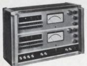
makes the balancing automatic; the meters can read the first, second, third or fourth digits. The Bridge produces analog voltage proportional to the meter readings and BCD (in a 1248
