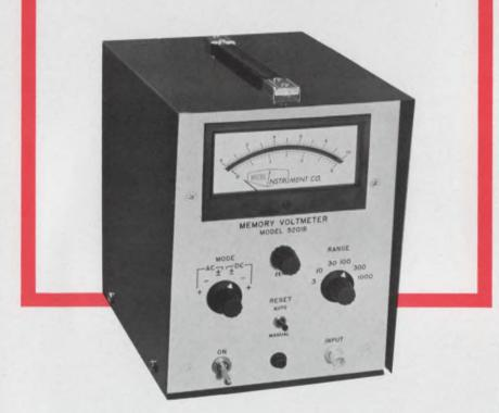
The Model 5201 memory voltmeter is a dc to 20 mc instrument which measures and stores indefinitely the maximum peak voltage applied, including continuous or one shot pulses as short as 50 nanoseconds. A memory reset-switch on the front panel allows the 5201 to monitor peak values of a varying waveform, either positive or negative going.
