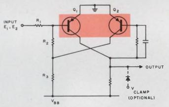
**Dc-coupled flip-flop acts** like a Schmitt trigger, but provides a ground-level output capability.  $Q_1$  and  $Q_2$  are saturating transistors with small  $V_{CE}$  and large  $V_{BE}$  ratings.
