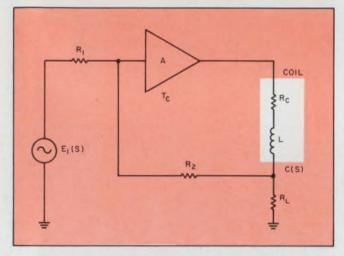
4. Greater coil inductances exhibit large resistances. For larger yokes, the resistor's influence on the transfer function must now be considered. Here  $R_e$  denotes the coil resistance, which modifies the gain and feedback values, according to its comparison with the load.
