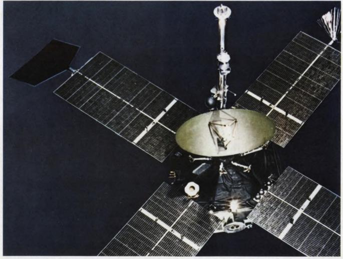
Mariner IV completed its flight to the vicinity of Mars on July 14, 1965 and sent back photographs and other measurements of the "red" planet. Its 10-watt telemetry transmitter spanned the unprecedented distance of 300 million kilometers in telemetering the data back to earth. (paper 67.2)
