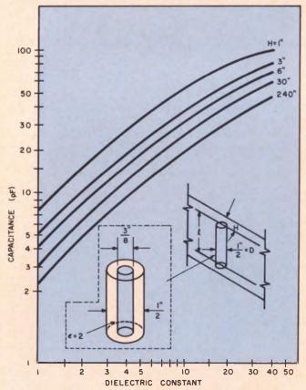
5. For a cylinder next to an infinite wall, the capacitance variations are similar to those for the coaxial-cylinder case, although the absolute values are lower.
