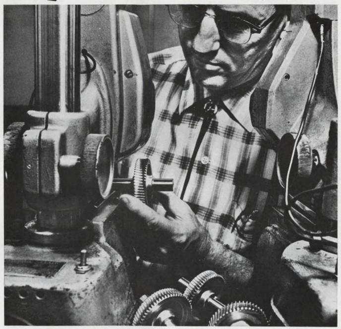
We use forged, heat treated bronze for gears in Bodine motors designed to withstand shock loads. We hob them ourselves, taking full advantage of bronze physical properties.
