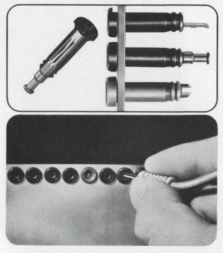
Now Ucinite offers you press-in test jacks for high-density, low-weight applications. Using nylon insulators available in 11 colors, these new test jacks have stamped or screw-machined closed-entry, beryllium-copper contacts that meet the performance requirements of MS-16108. They are available in a variety of terminal styles, and finishes. For complete details write for Bulletin 7072.
