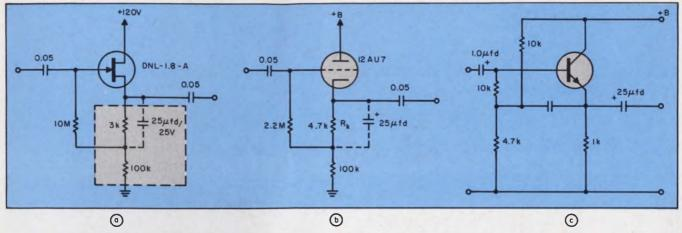
1. The FET source-follower stage is a basic audio circuit (a). It exhibits high input impedance and low output impedance because of the negative feedback employed in the source. Use of the FET yields higher gain and lower,
