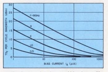
10. The frequency-dependent sensitivity factor, TS increases with increasing bias current. It also depends on the cut-off frequency, f.
