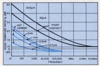
3. The intristic noise temperature,  $t_d$ , of hot carrier diodes is less than that of point-contact types. The asymptotic value of  $t_w$  is shot and thermal noises.
