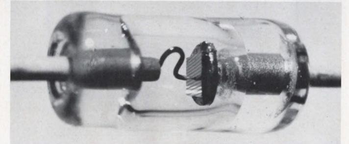
Schottky-barrier diode bridges the gap. 178
