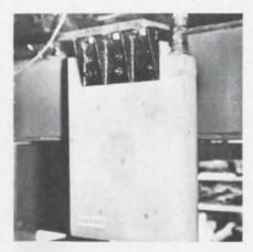
6. Slab antenna transmits signal via tracklength wire back to computers. Fields held light and 1 shot photo.
