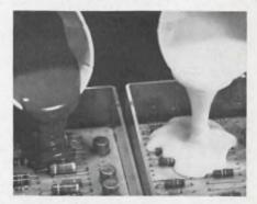
**Dow Corning 3110 RTV encapsulant** can be readily color coded by mixing in master batch pigments. It is a low viscosity, deep section curing compound that cures at room temperature and is designed for potting, encapsulating and embedding of electronic circuit and components. It flows readily into place and cures to form a tough, resilient solid. (Circle No. 851)
