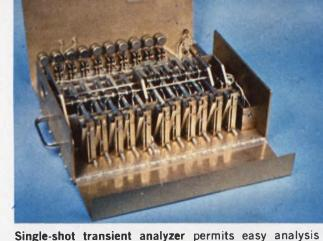
Single-shot transient analyzer permits easy analysis of complex transient waveforms. The analyzer was developed by General Dynamics/Convair for use in electromagnetic compatability measurements. (paper 65.2)
