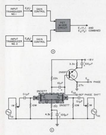
Two closely spaced transducer audio input signals are combined in a FET mixer (a). Complete circuit (b) shows high isolation ( $Z_{\rm in} = 10 \ M\Omega$ ), good linearity (400 mV dynamic input range) and dual outputs (0° and 180° phase shifts).
