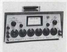
Designed for use in industrial, academic, and medical laboratories, the 10-14 dc oscilloscope is available in either kit or wired form. The vertical channel of the scope has a dc to 8 mc bandwidth and a sensitivity of 0.05 V/cm ac or dc. The horizontal channel of the 10-14 has 18 triggered sweep rates in 1, 2, 4 sequence from 0.5 sec/cm to 1 usec/cm with an accuracy of  $\pm 3\%$ .
