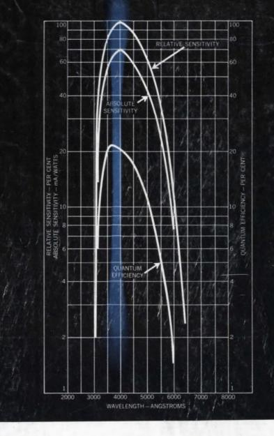
The Bialkali Photocathode is now available in many new RCA tube designs as well as in variants of most of RCA's commercially known photomultipliers. This new photocathode provides advantages in higher quantum efficiency and lower dark current. Designed for scintillation counting and other low-light-level detection and measurement systems, units with the RCA Bialkali cathode offer
