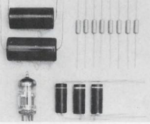
**Reap another beneFET!** In addition to the superior performance FETs offer in audio equipment, they require (top) less in the way of associated components and size than bipolar (middle) and tube (bottom) counterparts.
