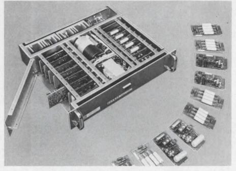
Current and voltage are fully programable with easily interchanged modular circuits.
