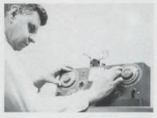
1. **T. A. Benham** operates a Heath Impedance Bridge that he fitted with Braille-readout dials.
