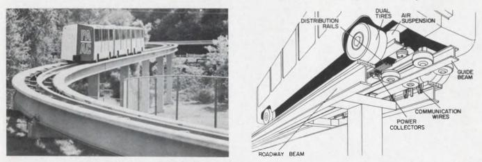
1. The Westinghouse Sky Bus rolls quietly through South Park controlled completely by computers. Its dual rubber tires run on two concrete tracks that are supported by steel "I" beams. Two dc motors propel each car.
