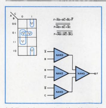
1. DeMorgan's theorem can be used for quick conversion of a function to a NAND form. But the results contain complemented and uncomplemented variables.
