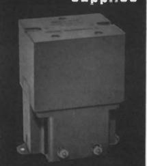
Building-block construction provides a basic transformer, rectifier, and where necessary a regulating device. The three molded elements bolt together quickly and maintenance is simplified. Output is completely isolated. DC voltage is filtered and provides 5% or less ripple. Most units rated for 5 ma, current. Input 115V, 60 cycle. Units available from 15 volts to 100-KV-DC.
