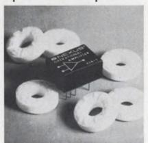
Designed for services requiring low power consumption, Model 2LV-1 operational amplifier features a 4 mW standby power drain at  $\pm 2.5$  V. The all-silicon unit can be operated from batteries, and offers a dc open loop gain of 10,000 with an output capability of  $\pm 1.5$  V at  $\pm 1.5$ mA. The 2,02 x 1.14 x 0.62-in. device operates from  $-25^{\circ}$  to  $+85^{\circ}$ C.
