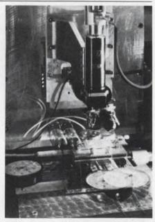
Light source and movable table that reproduce acceptable wiring on wafer.
