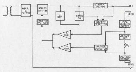
**Current and voltage limiting** are accomplished through independent regulator channels which provide automatic crossover to either mode for limiting or control. Remote sensing and load are related by these systems.
