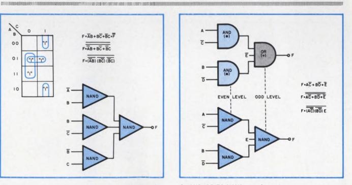
2. AND/OR TO NAND transformation results in the complementing of all variables that are present at odd levels. Variables at even levels are not.
