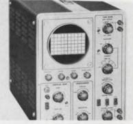
Model DAN 60 differential volt/ ratio meter combines 3 instruments: differential voltmeter, differential ratiometer, and null detector—into one package. The unit has two primary components —a complete differential voltmeter and a differential ratiometer. In addition, independent use of the transistorized voltmeter as a sensitive null detector is provided.
