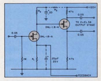
5. To obtain higher output levels in audio stages, a FET source-coupled phase inverter may be put to work. However, the balance here is not sharp, unless the generator source impedance is 100 kohms or more.
