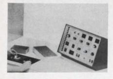
Model 8708A signal-generator synchronizer uses phase-lock techniques to give test signals stable within 2 parts in  $10^7$  over 10 minutes. Automatic synchronization is achieved within the range of the 606B (50 kHz to 65 MHz) or 608F (10 MHz to 455 MHz sig gens.
