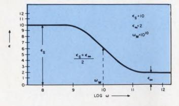
1. Dielectric constant decreases with increasing electricfield frequencies of about 10<sup>9</sup> Hz and higher. This is shown for a low-density material.
