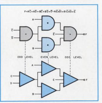
4. By rearranging the function equation, complemented variables can often be located at odd logic levels.
