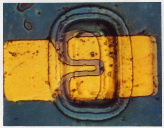
resistivity silicon substrates. It will be used to convert an incoming 9 GHz signal down to a 500 MHz IF frequency. (paper 45.1)
