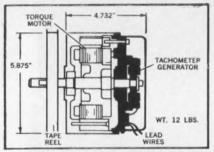
turned from conventional tape transport designs and developed a unique militarized system capable of optimum tape handling without damage or distortion. This modern, miniaturized design provides rapid reversal (less than 6 milliseconds) so programming is not restricted, high controlled acceleration and deceleration. (empty reel: 570 rad/sec2, full reel: 270 rad/ sec<sup>2</sup>), wide dynamic speed ranges (1000/1).
