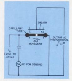
**C**<sub>1</sub> and **C**<sub>2</sub> are differentially proportional to the position of the electrolytic gap, thus proportional to the time integral of the input amplitude.
