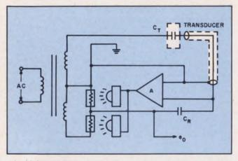
10. Light-sensitive resistors and light sources can be used as the balancing elements in an electronic self-balancing bridge network.
