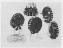
Trimmer needs in printed-circuit test, measurement and communications equipment are met by a new miniature closed-construction potentiometer. It features a rotational life in excess of 25,000 cycles and is 0.696" in diameter and 0.250" deep (including knob). Designated the Model 9, its range is 100 $\Omega$  to 10 M $\Omega$  (1/5 W) in the linear version and 200 $\Omega$  to 1 M $\Omega$  (1/10 W) with a non-linear taper. 20% tolerance is standard; 10% optional.
