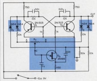
UJT, steering diodes and potentiometer add to versatility of bistable multivibrator.  $Q_3,\,D_1-D_4$  and  $R_{\rm T}$  enable symmetry, pulse width and repetition rate to be independently controlled.
