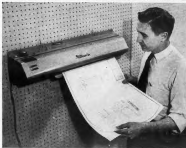
New, improved Rotolite Expediter conveniently makes sepia reproducible and diazo films in addition to low cost whiteprints.
