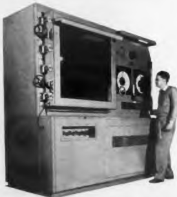
This altitude chamber is used for environmental testing of airborne equipment. It simulates altitudes up to 80,000 ft with temperature control to -67^{\circ} F.
