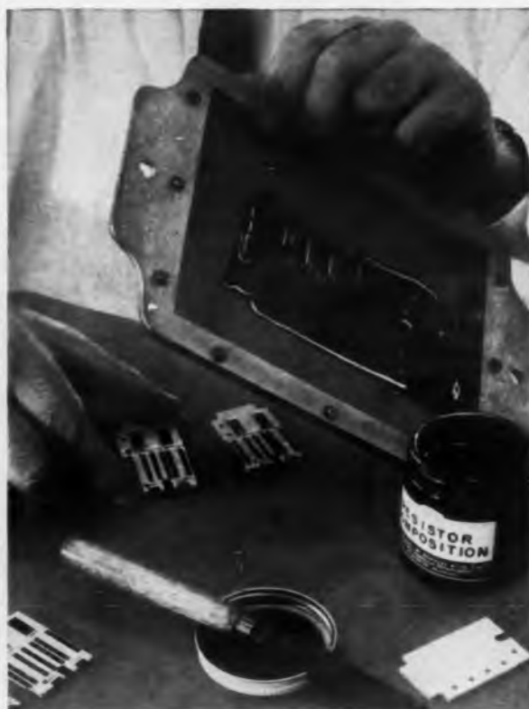
Laboratory demonstration shows Du Pont Resistor Composition being applied to a ceramic base by stencil screen and squeegee (left). When stencil is removed from ceramic base, resistor is ready for firing (right).
