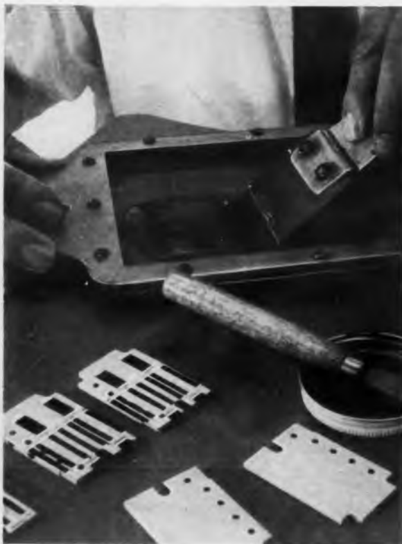
Laboratory demonstration shows Du Pont Resistor Composition being applied to a ceramic base by stencil screen and squeegee (left). When stencil is removed from ceramic base, resistor is ready for firing (right).
