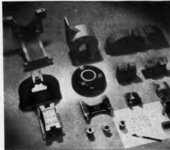
Typical group of permanent magnet assemblies.
