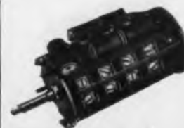
5-gang assembly with precision resistor network between sections.
