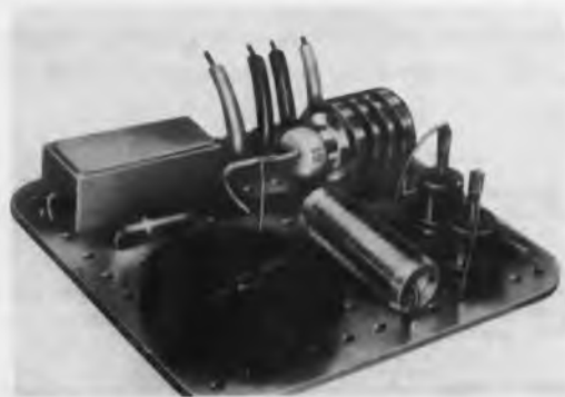
Constant-speed control for small appliance motor is one of typical consumer-electronic applications of controlled rectifiers. This unit, designed for low-current use, is less than 2.5 in square. It permits constant-speed operation at any selected point.
