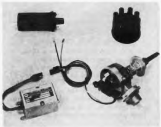
Electronic ignition system consists of ignition coil (top left), distributor cap (top right), transistorized pulse amplifier (lower left) and magnetic pulse generator.
