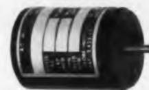
TYPE SC Sub-miniature motor rated .15 oz. in. max. sync. torque. Size: 1.07" dia. x 1.32" long. 2.4 oz. To 200 v. a. c. 2, 4, or 6 poles. 49 std. gear ratios.
