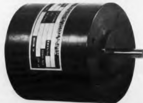
TYPE LC Small motor rated 10 oz. in. max. sync. torque. Size: 3 1/4" dia. x 3 1/4" long. 53 oz. To 200 v. a. c. 2, 4, or 6 poles. Gearing to order.
