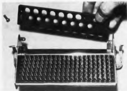
Fig. 3. Removable high-impact plastic fanning strip on each side of the boards permits wiring harnesses to be fabricated independently of one another, either in place or on the bench. The holes in the fanning strips align the wire bundles to facilitate final connections.
