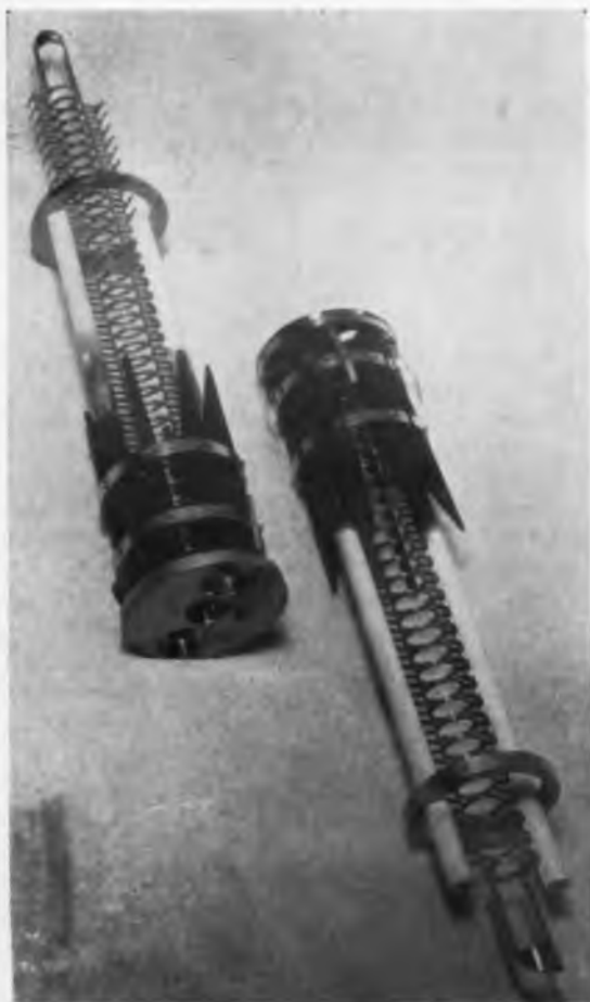
Internal structure of meanderline twt. Tube is shown in two halves, normally joined at the midpoint where the carbon-impregnated lossy vanes and ceramic rods are situated. Note unusual slow-wave structure consisting of two serpentine lines separated by row of rings. Ceramic rods stop short near output end where the serpentine is loaded with pins. Over-all tube length is about 27 in.
