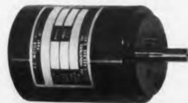
TYPE FC Small motor rated 1.6 oz. in. max. sync. torque. Size: 1 1/4" dia. x 2 1/4" long. 13.4 oz. To 200 v. a. c. 2, 4, or 6 poles. 101 std. gear ratios.
