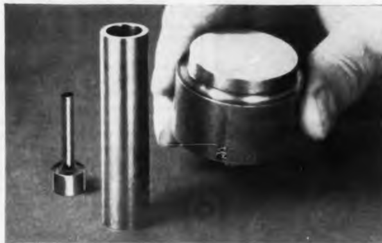
Typical electronic shapes fabricated from crystal tungsten (l. to r.): target emitter; zero-porosity tungsten anode for high-powered electron tubes with fluid cooling; high-power vacuum switch contact of zero-porosity tungsten mounted to copper.
