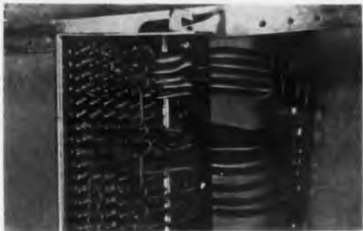
Fig. 5. Strapping for power supply distribution or relay ganging is easily superimposed by pushing special tabs on the strapping into the free ends of the female tabs.
