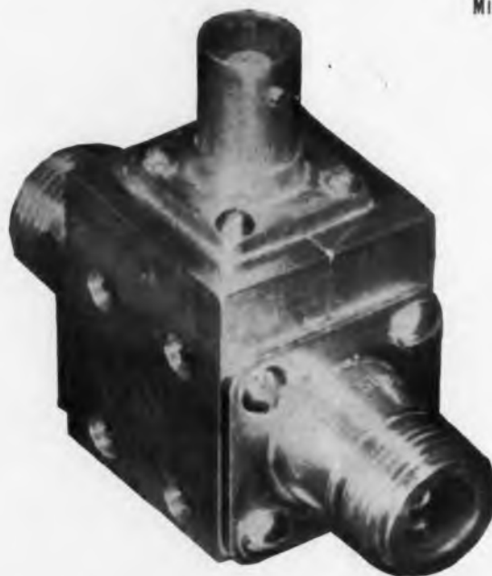
Fig. 5. Packaged diode switch. Entire assembly is housed in 1-in x 1-1/4-in aluminum block, exclusive of connectors.
