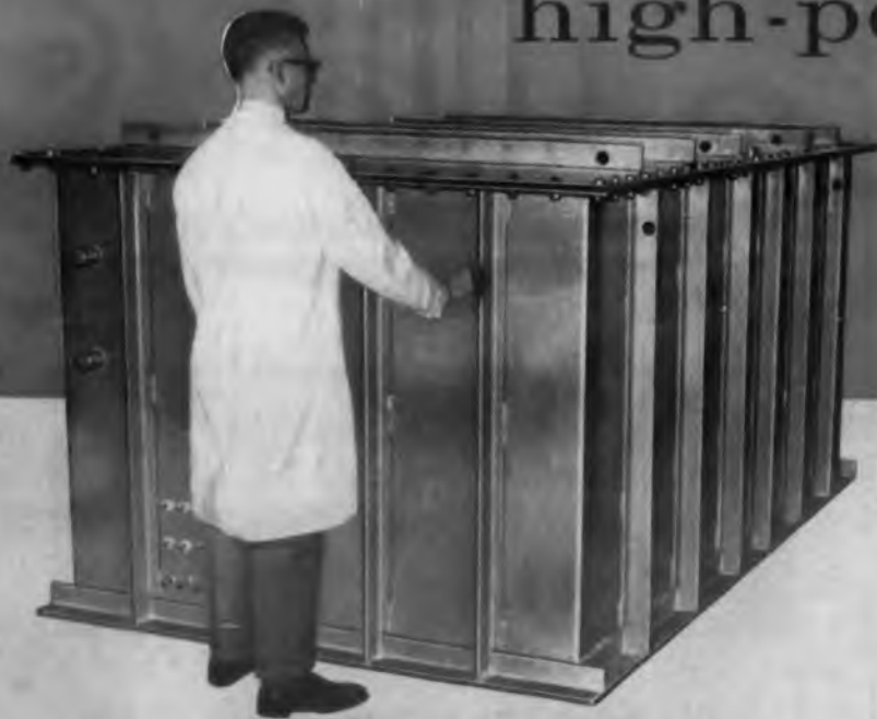
2½ TON POWER SUPPLY delivers 52.5 kVA, is insulated for 70kV and is capable of withstanding heavy short circuit fault currents.
