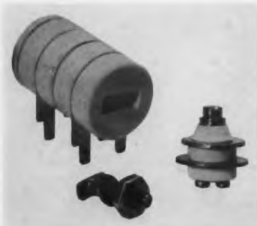
Fig. 1. Typical socketless planar triodes. The type 7296 tube at left comes with T-bolt for mounting to circuit board or metal chassis. The type 22866 tube at right is designed for direct soldering into coaxial cavities.
