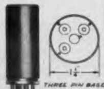
S-5019 Pin Connection Pin #8 (Cathode) Pin #5 and #4 (Anode) Replacement for 5R4
