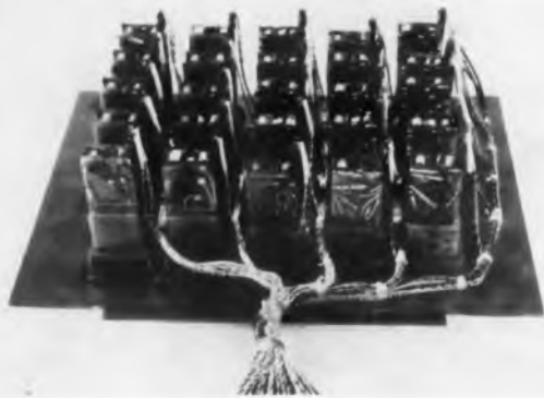
Fig. 2. Close-up of first approach to packaging being used on the Mark I. Though these soldered cordwood modules were quite compact in themselves, by the time they were mounted on the motherboard and mounted in a system, the amount of interconnection space they used up more than offset their individual packaging densities. Besides, these modules had high center-of-gravities off the motherboard and needed additional support. The cable was used to connect test leads out of the tops of the modules during development.
