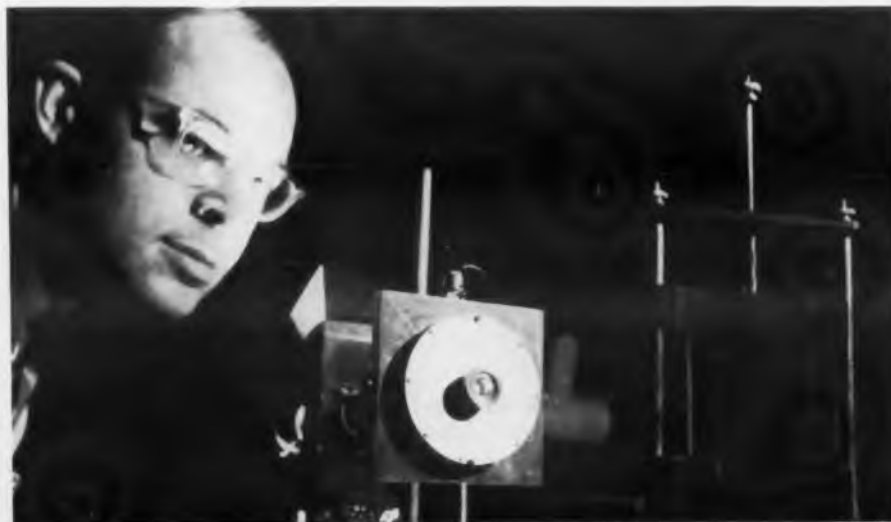
Light modulator mounted in front of arc light modulates beam aimed at mirror target at right. Square frame holds cylindrical resonant cavity containing an electro-optical crystal subjected to an electric field. Lens-like polarizer is one of two that pass light beam turned by crystal. Intensity of passed light varies with that of impressed field. This unit operates at 870 mc with a 2-mc bandwidth and a modulation factor of 30 per cent. Device was developed by Sperry for use in a cw optical radar for space use.
