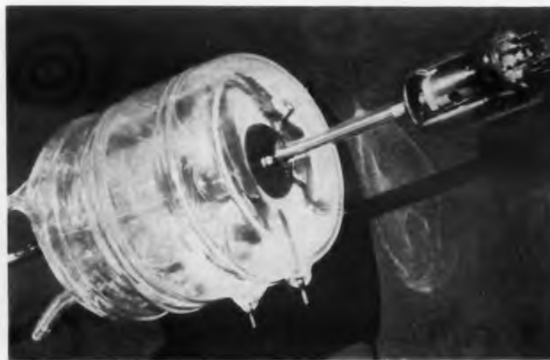
Cesium-beam amplifier developed at Stanford University. Plasma region is in large tube at left, with electron gun at right. The amplifier is operated in a solenoid to confine the plasma. Tuning could be achieved by varying the density of the plasma.
