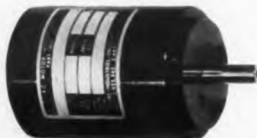
TYPE FC Small motor rated 1.6 oz. in. max. sync. torque. Size: 1 1/2" dia. x 2 1/2" long. 13.4 oz. To 200 v. a. c. 2, 4, or 6 poles. 101 std. gear ratios.
