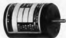
TYPE SC Sub-miniature motor rated .15 oz. in. max. sync. torque. Size: 1.07" dia. x 1.32" long. 2.4 oz. To 200 v. a. c. 2, 4, or 6 poles. 49 std. gear ratios.
