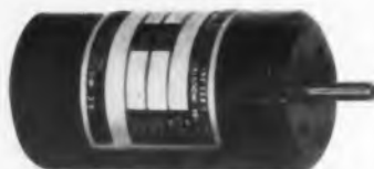
TYPE MC Miniature motor rated 0.8 oz. in. max. sync. torque. Size: 1 1/4" dia. x 2 1/4" long. 6.5 oz. To 200 v. a. c. 2, 4, or 6 poles. 101 std. gear ratios.
