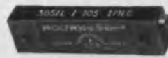
High-Temperature Humidity-Proof Resiston Carbon Trimpot—Model 3051. Only .19" wide. Operates to 150°C / L, S, P terminals / ¼ watt / 20K to 1 Meg. Sealed. Meets Mil Specs for cycling humidity.
