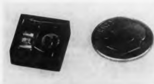
Fig. 3. Third and fourth progressions of the module are built around single-NOR units cleverly potted in their own welding fixtures, using the leads of their components as pins.
