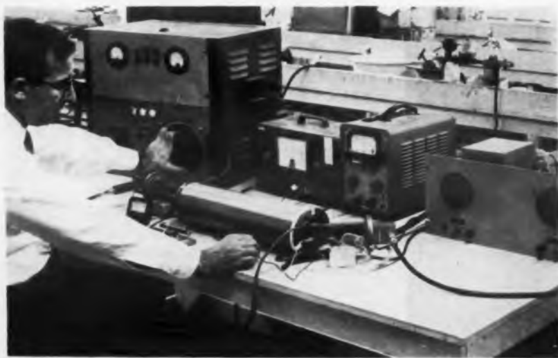
Plasma amplifier developed by Metcom is housed in rectangular waveguide. External solenoid provides magnetic field for tuning the device. Bandwidths to seven octaves at microwave frequencies are believed feasible with magnetic tuning.
