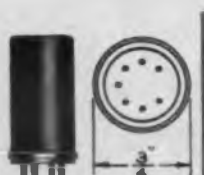
S-5207 Pin Connection Pins #1 and #6 are A.C. (Anode) Pin #7 is Pos. (Cathode) Replacement for 6X4, 6063, 6202.
