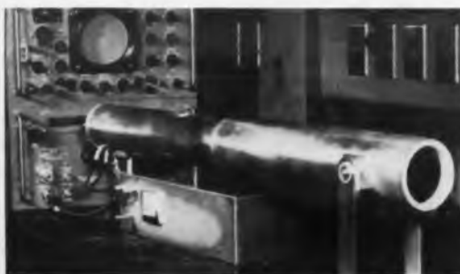
Optical-frequency transmitter (left) contains a ruby-laser light source and a light modulator consisting of a KDP crystal in a cavity oscillator. Modulating carriers of up to 160 mc have been applied to information carriers of 5-mc bandwidth at the frequency of red light. With a mercury-arc lamp source and a photo-multiplier-tube detector, communications over 1,000 ft have been achieved. Receiver is shown at right.
