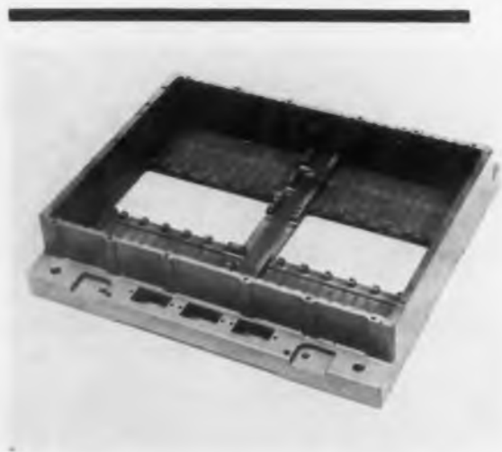
Fig. 6. The casting was quite intricate but made up for this by simplifying other parts of the package.
