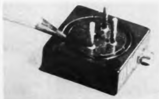
Subminiature trimming pot uses liquid sealant to lock aluminum collar in place without requiring a force fit.
