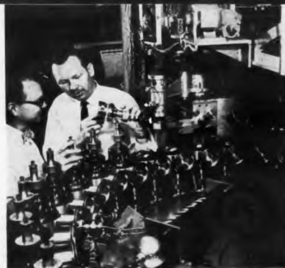
Bell jar held by Western Electric engineer has a gold cathode, used to deposit a layer of gold on the ends of carbon-coated resistor cores passing through the line. The gold termination forms a contact on each end of the resistors, to which the next machine attaches wire leads and caps.
