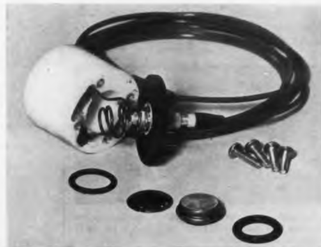
Photodetectors for space using semiconductors and liquid electrolytes are under development at International Business Machines Corp.'s Thomas J. Watson Research Center in Yorktown Heights, N. Y. The photodetector above is sensitive enough to detect weak signals from the moon, but rugged enough to withstand intense direct sunlight. It is expected to operate for several years with a 1.36-v battery. In normal solar cells light must pass through a thin silicon layer to reach the junction where energy conversion takes place. In the IBM device the surface layer is a sulphuric acid electrolyte which absorbs very little light. Sensitivity is 740 \mu\text{a}/\text{cm}^2 measured at 0.9 micron at a light level of 24 \mu\text{a}/\text{cm}^2 , according to IBM. High sensitivity to ultraviolet is used in ultraviolet detector using similar principle, below.
