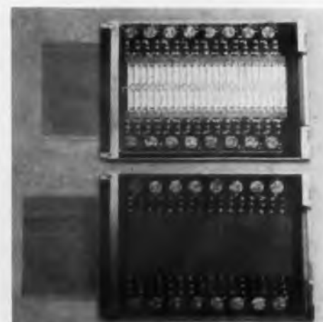
Logic board for thin-film DDA contains 32 NOR circuits consisting of thin-film capacitors and resistors, and micro-semiconductors.
