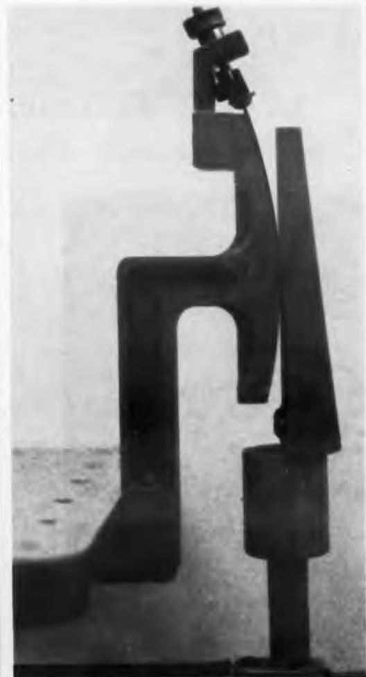
Steel ribbon , secured to flat tangent plate and curved rocker, converts linear-to-angular motion with virtually no backlash. Ribbon has been emphasized in photograph for clarity.
