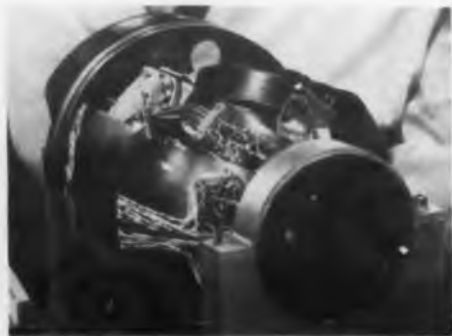
Developments such as this miniature all-attitude inertial platform (above), weighing less than 20 lb, are being handled by United Aircraft Corp.'s new Norden Div. research laboratory in Norwalk, Conn. This platform will be used in a new navigational system.
