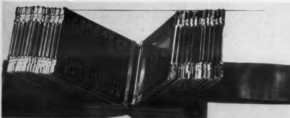
Thin-film digital differential analyzer built by Hughes to demonstrate feasibility of techniques weighs 1 lb, occupies 20 cu in, contains more than 8,000 parts, yet draws only 30 w. Hinged wafers are of Fotoceram. Components along edges are micro-transistors and diodes in ultrasonically drilled holes. Thin-film components are in center of wafers.
