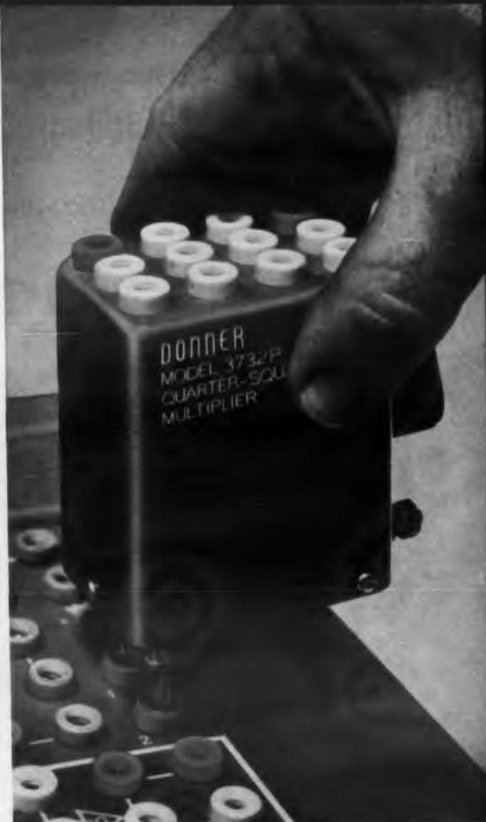
Model 3732 electronic multiplier is available without enclosure for panel mounting or as a single printed card for inclusion in your system. The unit is also available with up to three solid state multipliers on a 3\frac{1}{2} " x 19" panel for rack mounting.
