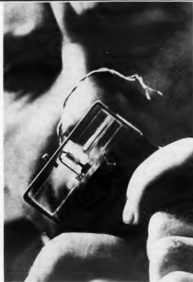
Photodetectors for space using semiconductors and liquid electrolytes are under development at International Business Machines Corp.'s Thomas J. Watson Research Center in Yorktown Heights, N. Y. The photodetector above is sensitive enough to detect weak signals from the moon, but rugged enough to withstand intense direct sunlight. It is expected to operate for several years with a 1.36-v battery. In normal solar cells light must pass through a thin silicon layer to reach the junction where energy conversion takes place. In the IBM device the surface layer is a sulphuric acid electrolyte which absorbs very little light. Sensitivity is 740 \mu\text{a}/\text{cm}^2 measured at 0.9 micron at a light level of 24 \mu\text{a}/\text{cm}^2 , according to IBM. High sensitivity to ultraviolet is used in ultraviolet detector using similar principle, below.
