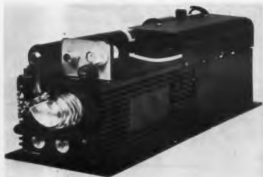
Twt radar augmenter , which provides a gain of 70 db at 9,000 Gc, is intended for installation in drone or target aircraft to reinforce radar tracking by missile-carrying aircraft.
