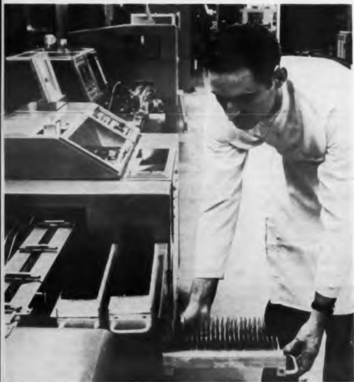
End of the line for the deposited carbon resistor is the packing machine, above. Here resistors are imbedded in styrofoam blocks, and loaded into a magazine. The magazines are then removed by an operator, who will prepare the blocks for shipment.
