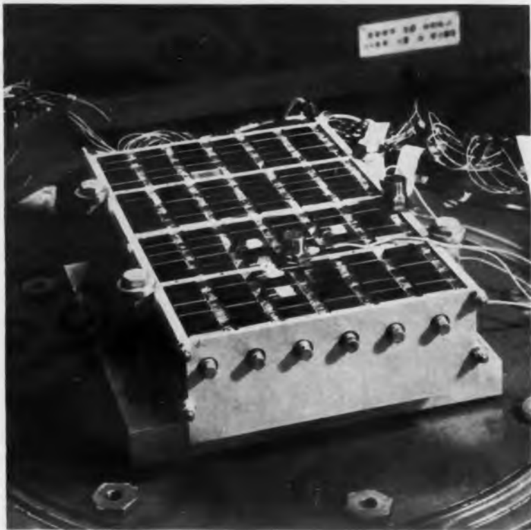
Fig. 5. Typical vibration test setup, showing circuit module assembly, compression webs, structural frame parts, tensioning bolts, and cold plates (corrugated metal parts).
