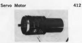
Designed for missile use, this 6-pole, 400-cps, size 15 servo motor offers the following characteristics: theoretical acceleration at stall, 22,-700 radians per sec2; minimum power output, 1.151 w; input power at stall, 6.1 w; motor dampening, 130 dyne-cm per sec.
