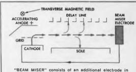
the crossed field device which collects a portion of the spent beam at cathode potential and returns it to the cathode by means of an internal conductor.
