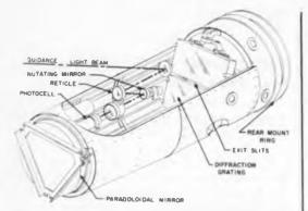
**Spectrometer** portion of system will fit in 30-in. long by 14-in. diam volume. Before fine-guidance system takes over, coarse positioning will be provided by inertial gyroscopes.
