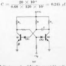
(a) Maximum value of R in this monostable multivibrator is limited by the value of  $\beta$  for transistor  $Q_1$ . Thus, for long pulse widths, capacitor C must be large.
