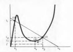
Fig. 2. After being switched to state 2 by trigger pulse, capacitor C causes current to decrease to  $l_1$  and the diode switches back to its original state.
