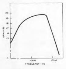
Fig. 7. Gain-frequency characteristic of the half-wave parant. Pump frequency was 600 mc.
