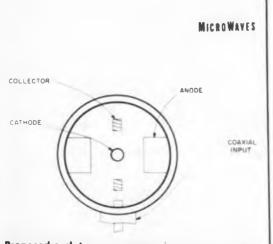
Proposed cyclotron resonance microwave power converter. Rf input, in conjunction with magnetic field (perpendicular to plane of drawing), accelerates electrons to the collector plates. Studies indicate that the device could approach 60 per cent efficiency. Back bombardment of cathode would eliminate need for heater.
