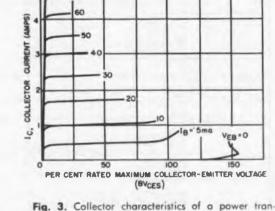
rig. 3. Collector characteristics of a power from sistor in a common emitter connection.
