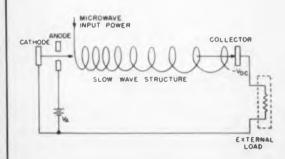
Inverse traveling-wave-tube microwave power converter. Electron beam is accelerated by absorbing energy from rf wave in the helix. The gradually increasing pitch of the helix keeps the traveling wave in phase with the accelerating electrons. A separate heater is required for the cathode.
