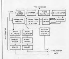
Fine-guidance system to aim ultraviolet spectrometer from rocket depends on rotating image formed by optical system to actuate servos that adjust aimbal ring mounts. Spectrometer is to be rocketed above the atmosphere early next year to analyze radiation from bright stars.
