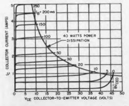
Fig. 1. Typical output characteristics of a Motorola 2N1530 power transistor.
