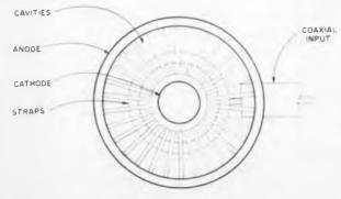
Inverse magnetron converter developed by Raytheon. Left to right: cathode, anode-cavity structure, coaxial rf input and cover. Final version of this device may approach 60 per cent efficiency and generate up to 1 kw cw in the 1- to 2-Gc range. Wright Air Development Div. is presently emphasizing development of this type of microwave power converter over other possible inversely operated tubes. The weight of the final version, including magnet, will be approximately 35 lb.
