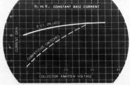
Extremely flat Beta vs. Collector Voltage is one of the many advantages made possible by the PSI Triple Diffusion Process.
