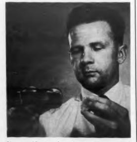
Direct amplification of sound waves using microwave radio energy has been achieved with this apparatus being assembled by Dr. E. B. Tucker of General Electric Research Laboratory. Amplification of the sound waves, or phonons, is accomplished by "stimulated emission" of energy by atoms as they change from higher to lower energy levels in a ruby crystal. The same mechanism is used in the maser (microwave amplification by stimulated emission of radiation) to amplify electromagnetic radiation.
