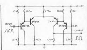
**High frequency** sine-to-square converter is made up of transistorized emitter-coupled lihiteds.
