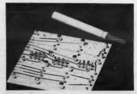
Beryllium oxide board 3-in. square by 0.06-in. thick was used for the thermal link between the modules and the heat sink which would be clamped on one edge. Kovar studs were weld points for the module leads of nickel-plated copper.
