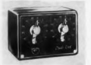
This compact recycling timer, designated series Dual-Trol, produces a series of on-off electrical pulses. It consists of two timing modules. one for the on and the other for the off signal, which can be adjusted to vary the timing interval. Ten replaceable modules are available with timing ranges from 6 sec to 3 hr. Units are rated at 10 amp and measure  $7-1/2 \ge 5-1/8 \ge 5-9/16$  in.
