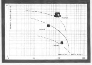
FREQUENCY-POWER OUTPUT RANGE OF PSI COMMUNICATIONS TRANSISTORS
