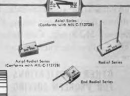
When tested at 125 C with more than twice previous test voltages applied (750 VDC vs 350 VDC and 450 VDC vs 200 VDC) and with the time extended to 2000 hours (more than 10 times as stringent a test) post-test dissipation factor is .002 max, and insulation resistance is greater than 100,000 megohms (10 times better)!
