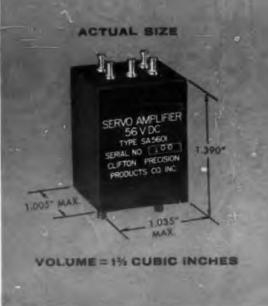
CPPC's new 5 watt servo amplifier provides a unique combination of exceptional stability and miniature size. Built around a DC amplifier with high frequency cutoff above 30 kcps, the SA 5601 provides uniform response over its full operating range. With a 10 k $_{\Omega}$  input resistor the SA 5601 yields a voltage gain of 54  $\pm$  1 db from  $-55^{\circ}$  to  $+125^{\circ}$ C with all signal levels below saturation, and supply voltage of 56  $\pm$  3 volts. Idling power is under 1 watt.
