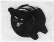
Semiconductor voltage regulation, holding the output to  $\pm 2\%$  from 1,000 to 12,000 rpm, is provided by these alternators. Two types are offered: 15 v dc, 1,000 w; 100 v dc, 1,500 w. Construction features radially oriented ceramic magnets in the rotor.
