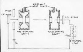
**Inverse klystron** microwave power converter. Electron beam between cathode and collector is accelerated by microwave input. Efficiency is reduced by need to divert some of the input to the pre-bunching cavity. A separately heated cathode is required.
