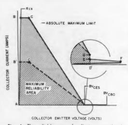
Fig. 6. The reliable area of collector operation is contained within the shaded region shown.
