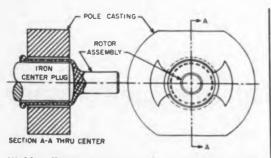
Highly efficient dc motor design is expected to produce 7-1/2 hp inside a 5-in. diam and with a weight of only 11 lb. Commutation would be by silicon-controlled rectifiers mounted in rotor and switched optically by phototransistors.
