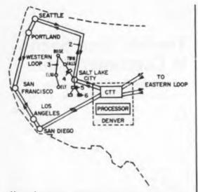
Map of western portion of Instamatic flight-reservation network shows (1) Concentrator, (2) High-speed trunk line, (3) Low-speed line, (4) Distant Central Office Transceiver, (5) Keyset Multiple Selector, and (6) Agent set.
