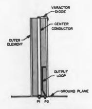
Fig. 4. Construction details of the quarter-wave parant. The antenna is single-ended and uses only one diode. However, additional diodes can be wired in parallel with the first, if desired. Construction of the quarter-wave antenna is simpler than that of the half-wave parant.
