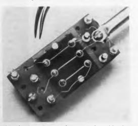
Three laminar superconductors are formed by deposition of thin-film lead strips on wider and thicker thin-film strips of silver. Intimate superposition of strips makes normal silver become superconductive at proper cryogenic temperature. In these three separate samples on glass substrate, the lead film is about 500 A thick, and the silver films vary from about 1,000 to 5,000 A. Electrodes facilitate measurements.
