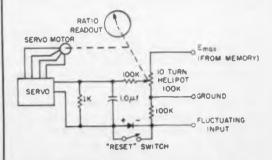
Automatic readout supplies lobe peak to null depth ratios of antenna pattern.
