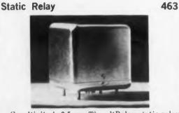
Sensitivity is 0.5  $\mu$ w. The ultRelay static relay with meter-movement sensitivity handles up to 750-w, 650-cps loads, and is virtually unaffected by shock and vibration. Power amplification ratios are 90 to 100 db. Operating temperature range is -40 to +160 F
