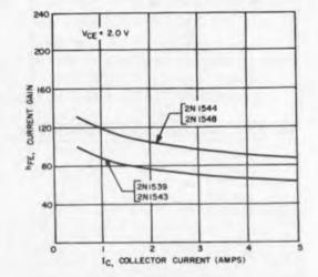
Fig. 4. The current gain,  $h_{FE}$  of alloy transistors decreases with increased collector current.
