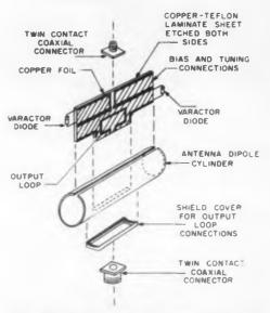
Fig. 10. Etched circuit, half-wave parant. This design approach should prove useful for antennos operating up to 500 mc. The etched circuit board replaces inner conductor of the lower-frequency parants. Resonant region is achieved by the stripline construction. Distributed elements would be used for tuning.
