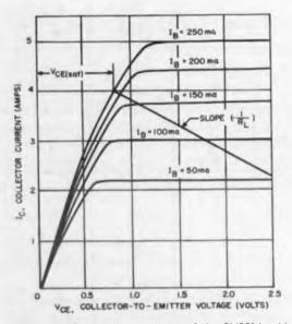
Fig. 5. Output characteristics of the 2N351A with the saturation region indicated.
