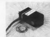
Sorts by color. Photoelectric reader model 150 provides a resistance range of about 25 K to 250 K from white to black surfaces at a distance of 1/8 in. from the lens. Volume is 2/3 cu in. Range is flush to 1-1/2 in.; weight is 1 oz.
