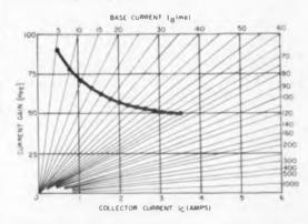
**Current gain**  $H_{FE}$  is plotted directly from  $I_b$  and I, measurements by laying out base current "guidelines" beforehand.
