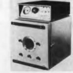
**Range** is -100 F to +600 F. Temperature can be lowered from 70 F to -100 F in 5 min, and raised to 600 F in 45 min. Heating unit is electric resistance type, operating on 15 amp, 115 v ac. Refrigerant is liquid CO<sub>2</sub>. Sealed construction is said to permit continuous operation at -100 F without condensation. Unit measures  $21-1/2 \times 14 \times 18$  in. Test space measures  $9 \times 11 \times 10$  in.
