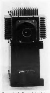
Thermoelectrically cooled television camera (with front cover removed). At top are the heat-radiating fins of the cooling elements, which enclose the vidicon. Motors and pulleys at the bottom control the focus and aperture of the lens.
