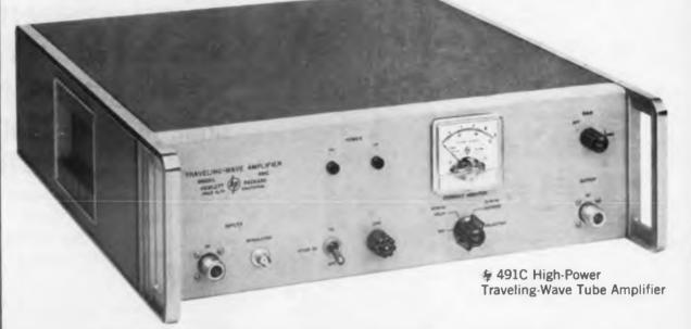
The new (a) 489A (1 to 2 GC) and 491C (2 to 4 GC) are broad band, low noise **Traveling-Wave Tube Amplifiers provid**ing at least 1 watt output for 1 milliwatt input over their full frequency range.
