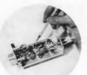
Fig. 9. Tuning network for the halfwave, 108-mc parant. Unit is conveniently mounted at center section of the antenna.
