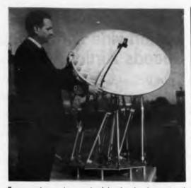
Foam antenna is examined by its developer, Mack Suliteanu, engineer at Sylvania's Electronic Defense Laboratories. Semi-transparent fiber-glass mesh covering the face of the antenna forms a base for a subsequently applied outer plastic coating. Note feed horn buried in the foam. The antenna is supported by a series of hydraulic jacks that can be programed to impart any desired tracking motion to the antenna.
