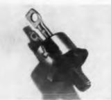
Rated at 25 amp at 100 C, diffused silicon controlled rectifiers of the TI-150 series are housed in stud package. Rated breakover voltages, both forward and reverse, are 50, 100, 200, 300, and 400 v respectively for the TI-150, 151, 152, 153, and 154.
