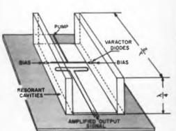
Fig. 11. Dual slot parant for use up to 2 Gc. Cavities behind slots in ground plane provide resonant storage for parametric amplification. Initial model of this design is undergoing operational tests.
