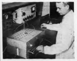
**Phase-angle master standard** designed by National Bureau of Standards operates continuously from 0 to 180 deg at 400 cps with 0.01-deg accuracy. One of the designers, H. N. Cones, adjusts a mercury contact for a portion of  $\pi$ -section used as delay line.
