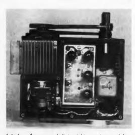
Interior of camera. Left to right: aperture and focus controls, 10-mc video preamp strip, and vidicon tube enclosed within the thermoelectric coolers.
