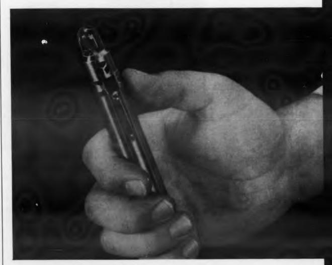
**PERSONAL RADIATION MONITOR**, developed at Oak Ridge National Laboratory, warns of radiation levels by flashing a neon lamp and sounding a tone in a hearing aid earphone. The transistorized circuit operates 24 hours a day for 30 days at a time, from power by a single Mallory TR-133R mercury battery.
