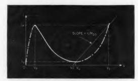
Fig. 5. Graphical representation of  $R_{D3}$  and  $V_2$ .
