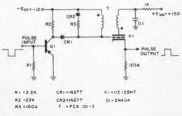
Pulses applied to the transistor stage trigger the vacuum-tube blocking oscillator.
