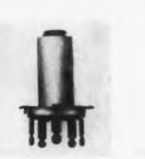
Vertically mounted ceramic coil form No. 2501 is for printed circuit work. The grade L-5 ceramic form is silicone-impregnated and is internally threaded for tuning cores. It is available with four different powdered-iron tuning cores having overlapping frequency ranges from 0.2 to 150 mc. Dimensions are 0.255 in. for the form OD and 0.625 in, for mounted height.
