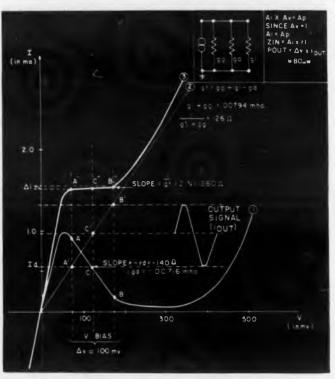
swing is limited to about 100 mv (peak-to-peak) by the nonlinearities occurring around points A and B. If point C is allowed to deviate from the center of the linear slope, the dynamic range would be greatly reduced and/or the distortion increased.
