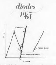
Fig. 5. Straight line representation of the input characteristic when base current flows before tunnel diode valley region is reached.
