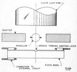
Scribe line splits silicon solar cell into two equal parts in the light-operated accelerometer. Quartz rod pendulum splits light beam into a pair of matched beams at null position. If acceleration is applied the pendulum moves and the change in light flux on the twin cells is compared to get an output proportional to the amount of acceleration.
