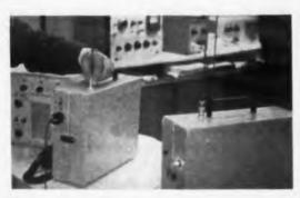
Test model of Racep random-access, discrete-address communications system consists of encoder-decoder for addressing, left; transmitter, center, and receiver, right. System is said to be capable of supporting up to 700 users on 4 mc.
