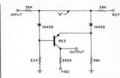
When input voltage is at the reference level, voltage at A is at zero, transistor is cut off and output rises to the supply voltage level.
