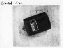
With A 2.0-cps bandwidth at 100 kc f., model BP-104D crystal bandpass filter is designed for vibration-analyzing equipment. The crystal is housed in a thermostatically controlled oven to maintain 135 C. Specifications are: insertion loss, 22 db; impedance, output and input, 1.2 K; size, 4 in. in diameter x 5 in.; maximum drift, 0.0005% of f. over operating temperature range.
