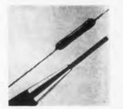
Vitreous-enameled, wirebound 1-w resistors are made in axial-lead configuration. Length is 9/16 in. max, diameter 1/8 in. max. The resistor shows stability under constant full load, low noise, long life and good overload capability. Resistance range is 1 to 6,000 ohms, tolerance  $\pm 5\%$ .
