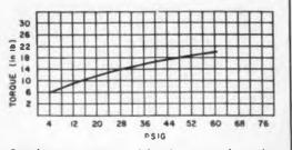
**Breakaway torque** vs inlet-air pressure for a size 10 air clutch.
