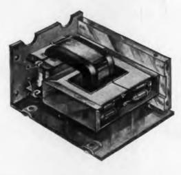
The drawing shows the unique construction of the Isoformer (isolation transformer). This is the key element in new Elcor isolated power supplies ... called ISOPLYS.
