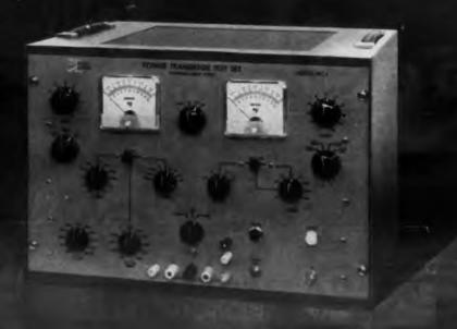
Minimizes heat sink requirements. Under optimum conditions, requires only 6 10ths of 1% of the input power used in conventional DC current tests.
