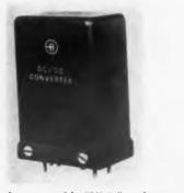
Designed for use with "Nixie" indicator tubes, models VC 12-170 and VC 28-170 have an output of 170 v dc from 12 and 28 v dc respectively. Full load current is 30 ma for each, enough to power 10 "Nixies."
