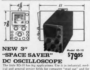
ical and general service fields for computer "read out" and for voltage, frequency and phase shift measurement. It features identical vertical and horizontal AC or DC coupled amplifiers, external sync terminal, external capacity binding posts for sweep rates lower than 5 cps, transformer-operated power supply, voltage-regulated B + and bias and excellent specifications. 3RP-1 CR tube included. Send for free Heathkit catalog or see your nearest Heathkit dealer.
