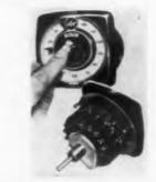
Offered in 11 standard ranges, series 312 shaftdriven counter has a repeat-count accuracy of 0.25per cent of the dial range. The shaft requires an operating drive torque of 1-1/4 oz-in. Applications include process, batch system and automatic flow control.
