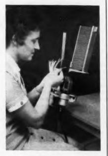
As a result of wide customer acceptance of BURNDY Omaton Division's YD-2, a new version of this semi-automatic, portable, pneumatic crimping tool has been developed. The new edition, the YD-2-3 is a bench-mounted, foot-operated tool with a magazine holding almost eight times (533 contacts) as many contacts as the original version (70 contacts).
