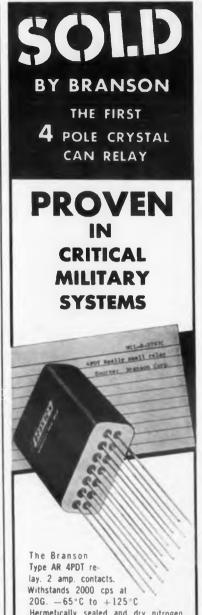
20G.  $-65^{\circ}$ C to  $+125^{\circ}$ C. Hermetically sealed and dry nitrogen filled for high altitudes. Wt 15-20 gms. Dim. 384 x 784 x 882. Hook, plug-in or wire leads available. Std. 0.1 in grid spacing. Suitable for dry circuit conditions. Meets specs: MIL-R-25018, MIL-R-5757C, MIL-E-5272C.
