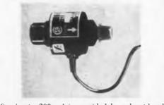
Service to 200 psi is provided by solenoid valve for use in fluid control. Available in standard ac and dc voltages, the valve operates in any position with a maximum rate of 1,000 cycles per min at 100 psi. Temperature range is -65 to +350 F. The 5-oz valve measures 2-5/8 in, long with a diameter of 1-3/8 in. Inlet connection is 1/2 in, outlet 1/8 in. General Magnetics, Inc., Dept. ED, 2641 S. Louisiana Ave., Minneapolis 26, Minn.
