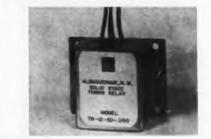
Solid-state timing relay, for pulse or squib applications, can turn on a 50-amp load within 10  $\mu$ sec of the application of a short, low-energy, voltage trigger having an amplitude of  $+17 \pm 11$  v. The relay, model TR-12-50-.030, operating from a 12 v dc source, shuts off the load after 50 msec.
