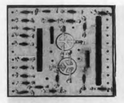
2-D circuit, above, has Texas Instruments microtransistors, Pacific Semiconductor microdiodes, and deposited carban resistors mounted on a 1-in. sq alumina wafer. Holes at the edges of the wafer are for wires used to connect it to a printed-circuit board. All joints are made with solder. Intraconnections on the wafer are made with silkscreened silver conductors. Below, deposited carbon resistors are put on a wafer using an injection printing process, giving good thickness control.
