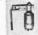
High-temperature, hermetically sealed switch uses a rotary linkage actuator for positive operation regardless of dust or ice conditions. Lever can be adjusted through 360 deg. Rating is 2 amp inductive, 28 v dc and 1 amp inductive, 115 v, 60 or 400 cps. Temperature range is -65 to 600 F.
