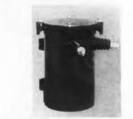
**Broad-band balun** transformers match 50 to 75ohm coaxial lines to 600-ohm balanced transmission lines over the hf range. Devices operate from 2 to 30 mc and display essentially flat input impedance vs frequency curves. Model 517 is designed to pass 10 kw cw, and may be pole-mounted. Model 532, a receiving type, passes 500 w.
