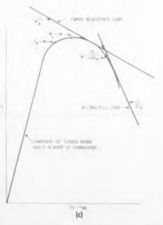
**Fig. 6.** Exaggerated input characteristics for a practical case. Full (a) or degenerate (b) loops will be formed depending on the load conditions (c).
