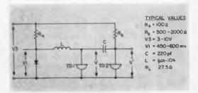
Fig. 11. Complete circuit of the square-wave generator using a single power supply.
