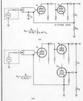
Fig. 2. Similar cable connections can be made for amplifiers of two or more stages.
