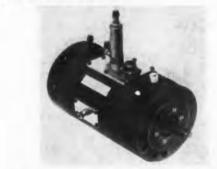
Variable inductance transducers, series C-B4, measure angular twist proportional to torque. Electrical measurement of a torsional strain and a mechanical assembly for producing the strain are provided. Speeds are to 20,000 rpm and torque ranges from 0 to 50 in.-lb through 0 to 12,000 in.-lb full scale.
