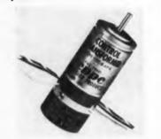
A sector switch provides a closed circuit when the position of the synchro exceeds  $\pm 70$  deg from EZ. Adding 0.5 in. to the over-all synchro length, the unit can be used wherever switching is required in conjunction with synchro angular positions.
