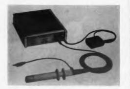
CONVERTING CURRENT TO VOLTAGE, the new Hewlett-Packard AC current probe simplifies measurements of alternating current. Two Mallory Mercury Batteries provide the instrument's low impedance power supply, with fade-free service of approximately 400 hours.
