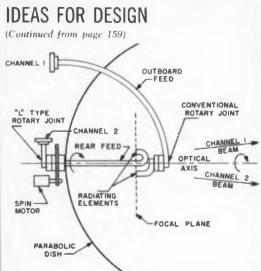
Standard rotary and L-type rotary joints are used in dual-channel conical scanning antenna
