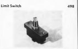
Snap action limit switch is designed to bridge the gap between the very small and larger, enclosed limit switches. Ratings are as follows: ac, 40-amp make, 15-amp break; dc, 2-amp make and break on single throw forms with 0.040-in. gap.
