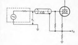
Fig. 1. Effective cable-input capacitance can be reduced by connecting shield to the cathode follower input.
