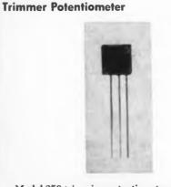
Model 356 trimming potentiometer provides resistance values from 10 ohms to 50 K in a  $1/2 \times 1/2 \times$ 0.195 in. package. The unit can operate from -55 to +200 C. Circular mandrel design provides 0.086% resolution at 50 K. The trimmer can dissipate 1 w up to 50 C.
