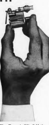
The Type A Silic-O-Netic Relay is a light, small timedelay relay. It weighs a mere three ounces, gives you any delay you spec from 0.25 to 120 seconds. Keeps at it, too, for several million operations; the time-delay element cannot stick, bind, or wear. The Type A Silic-O-Netic Relay is a light, small load relay. The continuous-duty coil does the trick. The Silic-O-Netic can be energized continuously, eliminating lock-in auxiliary circuits. Saves wire. Saves work. Saves space. Saves money.
