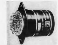
The spdt relay features operation which produces a self-cleaning or brushing action. The relay has a minimum life of 100,000 cycles at rated load. The solenoid for nominal 26.5 v dc operation; other voltages can be supplied. Type 1000 relay meets specifications MIL-R-5757 and MIL-R-25018, Class C, Type II, Grade 3. The unit weighs 4.7 oz.
