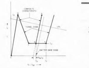
Fig. 1. V-I characteristic curves of negative resistance devices.
