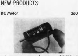
A permanent-magnet de motor, model PM-1 is suitable for military and commercial uses. With efficiencies to 54% through high-flux utilization, the motor requires very low current at full load. Weight is less than 2 oz; length is 2 in., OD 7/8 in. Motor operates from -55 to +100 C, under vibration, shock and acceleration satisfying military specifications. Voltage range is 3 to 30 v dc.
