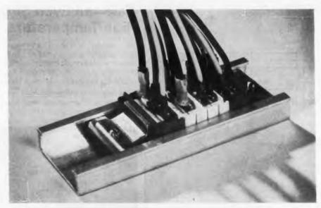
Assembled terminal block stack is locked into aluminum track.
