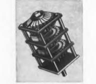
**Progressive shorting-type** switches have separate collector-ring connection for complete or continuous programing. Switches, which can be ganged, come in a 1-3/4 in. sq for 20 and 24 positions, and in a 2-1/4 in. sq for 24 and 32 positions. Daven Co., Dept. ED, Livingston, N. J.
