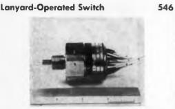
A 4pdt lanyard-operated switch, type M-479-1 withstands high-level sinusoidal and random noise vibration tests in both axes, in normally open and closed positions, without contact movement. Switch has passed vibration test of 92 g at 2 kc. Contacts are rated at 10 amp dc. Weight is 0.5 lb, length 2.7 in. Life exceeds 5,000 cycles per min.
