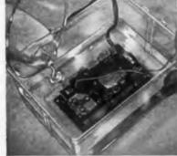
**LTV-602** is easily applied, flows freely in-and-around complicated parts. Having a low vis-cosity in the uncured state, 800-1500 centi-poise, LTV is ideal for potting and embedding of electronic assemblies. Unlike "gel-like" potting materials, I.TV-602 cures to a flex-ible solid. Oven cure is overnight, or from 6 to 8 hours at 75 to 80°C.
