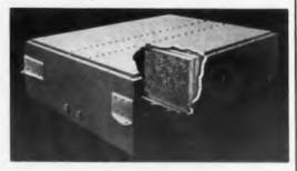
bly frame will hold 8 to 10 boards. A central duct in the computer will allow free air flow through the assembly frame slots and over the flat circuit surfaces, carrying away heat.
