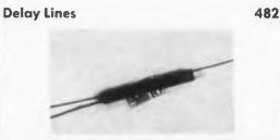
Encased in a 13 32-in. diam tube, these distributed constant delay lines have an impedance of 500 ohms. Delay times are 0.05 to 1.0 µsec, with rise times from 50 to 120 nsee. Operating temperature is from -55 to +125 C.
