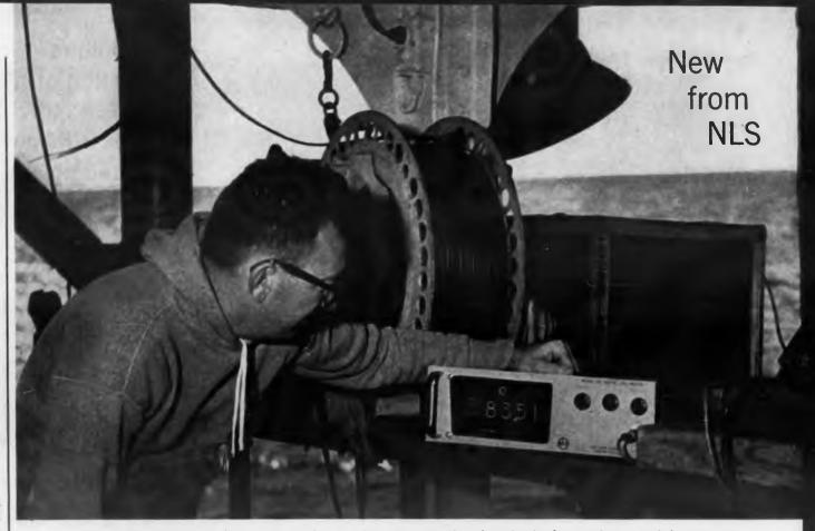
The NLS V60 Digital Millivoltmeter is designed for a wide range of scientific, industrial and military applications including strain gage and thermocouple measurements, calibrating millivolt devices, process monitoring, and semiconductor research and testing.
