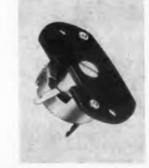
Preset and variable, type INS-110 has a mounting plate to insulate the control. It is for hot-chassis or other potentiometer uses and can be furnished with a molded shaft. Diameter is 3/4 in. Rating is 1-1/4 w at 40 C, derated to no load at 105 C. CTS Corp., Dept. ED, Elkhart, Ind.
