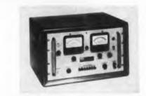
**Fm-monitor** deviation calibrator, "Monocal 500", provides better than 0.5% deviation accuracy. It combines the functions of five instruments previously needed to determine the peak deviation of an fm signal by the carrier drop-out method. It can be used directly with any fm monitor tuning to 12 mc. Deviation ranges are: 10-, 30-, 100-, and 300-kc peak.
