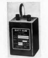
Constant voltage supply, model BS(TC)-2 can substitute for dry and wet cells for use with precision laboratory potentiometers such as the L&N types K2 and K3 and the Rubicon types B and S. Voltage stability is better than 0.01 per cent for 10 per cent variations in 117 v line. Over 15 C to 35 C temperature range, stability is 0.001 per cent per deg C.
