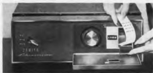
Decoding unit of Phonevision pay-TV system being installed in Hartford, Conn., enables subscribers to receive programs sent in scrambled form. It contains tape that records programs viewed, charges and quality of reception. Current models of the Zenith decoder have a two-way switch.
