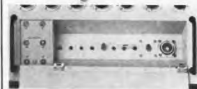
Shielded measuring compartment, easily accessible in front panel, permits critical measurements without stray pickup.
