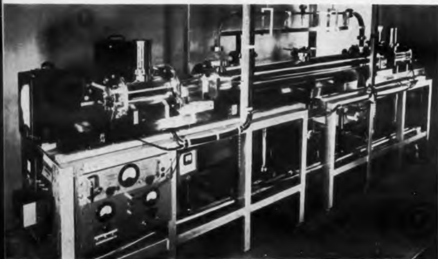
Cesium-beam frequency standard at the National Bureau of Standards. Accuracy is said to be 2 parts in 10^{-11} .
