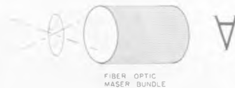
Fiber-optic maser bundle would also enable spatial modulation; here, multiple beams transmit entire image simultaneously.
