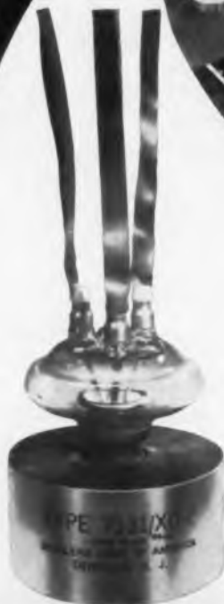
7131 XD-2's in a 20 Mw Modulator made by Manson Laboratories Incorporated, Stamford, Conn.
