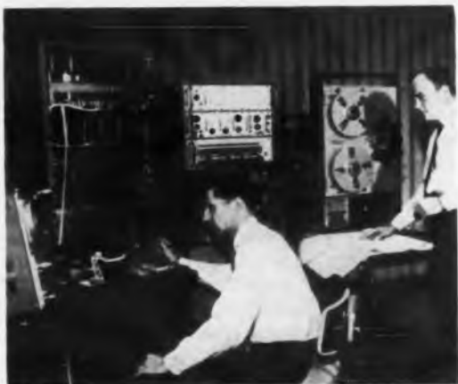
High-density recording system undergoes test. Digital tape handler is at far right next to a computer simulator. A high-speed central control unit appears next to the oscilloscope.
