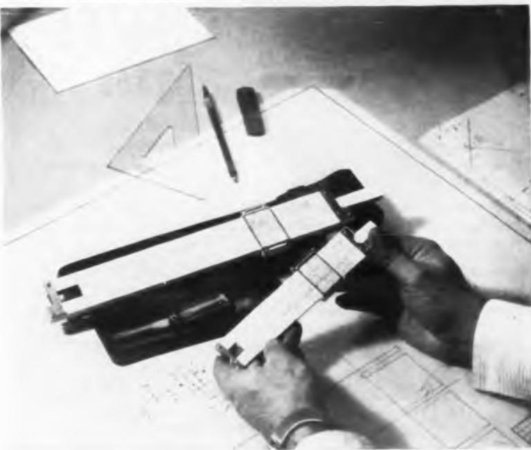
This is a size comparison between the 10" POST Versalog and its 5" replica, the POST Pocket Versalog.
