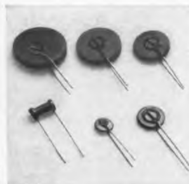
Disc and rod type GLOBAR varistors are shown above. Wide variation in voltage coefficients may be obtained through changes in length-diameter ratios.
