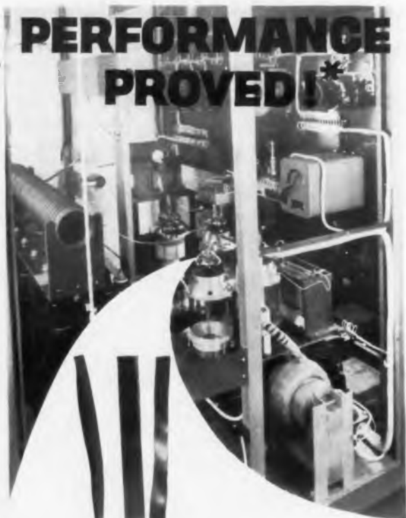
7131 XD-2's in a 20 Mw Modulator made by Manson Laboratories Incorporated, Stamford, Conn.
