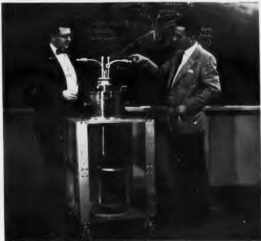
Project Echo traveling-wave maser is discussed by Bell Telephone Laboratory scientists R. W. DeGrasse and H. E. D. Scovil. The two-channel device operates at a signal frequency of 2.4 mc.
