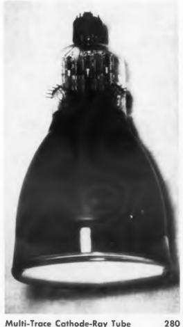
Multi-Trace Cathode-Ray Tube Provides Triple Display
