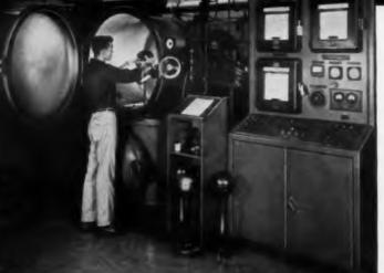
maximum use of automatic precision control of temperature, vacuum and deposition rates. The result is a predictable life of 80,000 hours or more, and unexcelled functional reliability. The sphere (see larger photo) holds each cell at an equal distance from the "boiler," creating even, uniform deposition cell to cell.
