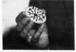
**Tunnel-diode module** for developmental computer memory handles 64 bits in 3-in. diam. Complete readwrite cycle was performed in 40  $\mu$ sec with same circuit in different configuration—an 8 x 8 array on 9-in. circuit board. Module is for a word-organized memory designed at Plessey Co., Ltd., Hants, England, that uses voltage-mode selection. Circular arrangement was chosen to reduce delays caused by leads, which slowed read time in array format to 10  $\mu$ sec.
