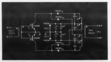
Fig. 1. Phase detector matches phase relationship between reference voltage and monitored function.
