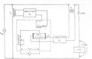
Fig. 2. Experimental audio wattmeter uses a Hall device as a current-voltage multiplier.
