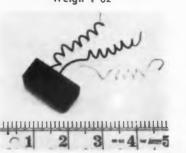
Designed for airborne systems, these telemetering filters measure 23/32 x 23/32 x 1-3/8 in. and weigh 1 oz. Center frequencies range from 1.7 ke to 70 kc, with an impedance of 51 K. Attenuation is less than 3 db at  $\pm 7-1/2\%$  and more than 20 db at  $\pm 27\%$  of the center frequency. The filters are encapsulated and environmentally tested to military specifications.
