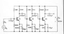
Fig. 4. Low-noise three-stage amplifier.
