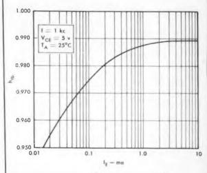
Fig. 3. Hybrid parameter his vs emitter current In.
