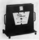
Used to calibrate any torque measuring equipment, model 6500-T2 also checks breakaway and static torque. Three scales provide a measuring range of 0.5 to 40.0 oz-in. and 20 to 2,800 g-cm at an accuracy of  $\pm 0.2\%$  of indicated reading. Operating on weight-vector principle, the device uses no springs. It weighs 24 lb, and measures 14-1/4 x 16 x 8 in. over-all.
