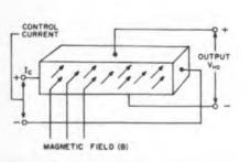
**Fig. 1.** Typical Hall generator develops a voltage which is a product of a magnetic field and a perpendicular current flow in a semiconductor.
