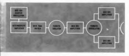
**QKW** 750.4 TWT has 20 db nominal gain and 100 kw nominal peak power to drive Amplitrons in MOPA chains. Duty cycle is 015 for pulsed operation over the 2,900 to 3,100 Mc range. A similar tube, the QKW 782, covers the 2,700 to 2,900 Mc range. Circle 201 on Reader Service Card.
