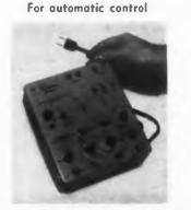
This tape transport programer automatically controls digital tape machines to run in forward and reverse. Run times and stop times are adjustable from 2.5 msec to 1 sec. Outputs are capable of driving the actuator control circuits of the tape machine. The unit is contained in a case measuring 4 x 7 x 8 in.
