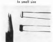
These miniature ceramic capacitors combine small size, a wide range of capacitances, and high electrical quality. Style 374, enamel-coated, is 0.320 in. long and 0.125 in. in diameter; style 375 is a phenolic-coated capacitor 0.320 in. long by 0.140 in. in diameter. A wide range of dielectrics is available. Capacitance is 2 pf to 56 pf. The unit operates at 100 wyde to 125 C, and 200 wyde to \$5 C.
