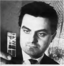
Thin-tilm titanium tunnel diodes deposited on glass substrate, held here by Dr. Franz Huber of Republic Aviation Corp., operate at room temperature.
