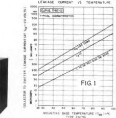
Clevite type 2N1761 (see chart). These are relatively new, fully specified at high temperatures to allow stable, predictable operation in DC coupled circuits. Figure 1 shows leakage current versus temperature for various common emitter operating conditions. The Clevite Spacesaver transistor exhibits low phase shift at high audio frequencies, allowing its use in systems having large amounts of negative feedback. Frequency response of the 2N1761 versus collector current is shown in figure 2.
