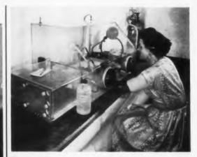
Fig. 4. Vacuum oven inside the air lock contains components which have been baked dry. The components are taken from the air lock into the dry box where they are hermetically sealed. Bubbles in the glass bottle indicate the air lock is being constantly purged with clean dry air.
