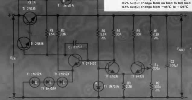
NOTE: All composition fixed resistors are TI MIL-LINE precision carbon film types, RN65B or RN70B.
