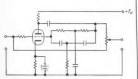
**Fig. 4.** Subtraction network in Fig. 1. can be eliminated if an addition circuit, such as shown here, is used for the feedback amplifier.
