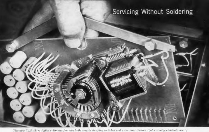
The new NLS 481A digital coltmeter features both plug-in stepping switches and a snap-out readout that virtually climinate use of a solder gun or other tools in servicing. Note the "finger-control" leverage bars for easy switch removal.
