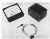
This direct-readout temperature meter, for the range of 50 to 150 F, uses thermistor probes for rapid response. It is easily used in systems for measuring gas temperatures or the surface temperature of solids. Probes are corrosion-resistant; wire leads are covered with Teflon. Special models to 1,000 F are available.
