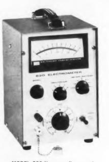
MODEL 620 Battery-Operated Electrometer offers 31 ranges.
