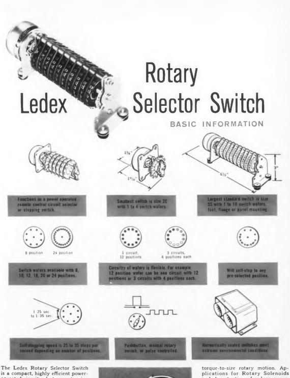
is a compact, highly efficient poweroperated circuit selector or stepping switch, designed for remote control. Nearly unlimited design combinations permit great variety of applications for stepping, counting, adding, subtracting, programming and sequencing. Many stock models on hand for immediate shipment. Hermetically sealed models also available. Power source is the Ledex Rotary Solenoid. This unit gives highest-
