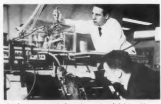
Antiferromagnetic isolator is tested at 140 kmc with carcinotron signal source. Isolator, in liquid nitrogen Dewar between poles of the large electromagnet at bottom of photo, is adjusted by Dr. Gerald S. Heller, leader of the Resonance Physics Group at Lincoln Laboratory. At top, John J. Stickler monitors carcinotron output. The tube is said to average 20 mw of power within a 7 per cent tuning band.
