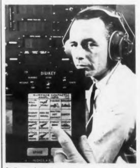
Digikey, a device that sends messages in digital form, is being used in the Hughes-built long-range communication system, Hacon, now operational with the B-58 Hustler supersonic bomber. Developed by Hughes Aircraft Co., Culver City, Calif., Digikey operates through heavy electrical interference by breaking up a message into a series of coded electrical pulses. These are transmitted over several frequencies. The unit operates at 150 words per minute.
