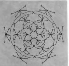
Input of system would be network of 72 photoreceptors differentiated four at a time and also in clusters of 16. Solid black circles represent 36 optic fibers to carry differentiated signal pulses. Entire system was designed to operate as closely as possible to a biological image processing organ. It would be used as input to computer in which stored patterns would be available for comparison.
