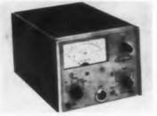
Model 431A power meter has a drift stability of less than 2  $\mu$ w per deg C over a range of 1  $\mu$ w to 10 mw. One zero adjustment is needed for all seven ranges. The meter face is also calibrated in dbm with 5 db between ranges.
