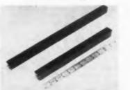
These precision linear-motion potentiometers have infinite resolution in stroke lengths up to 30 in. Designed for operation on ac or de inputs they provide outputs without amplification as great at 350 v per in. of shaft movement, with sensitivity of 5 millionths of an inch. They have a guaranteed life in excess of 10 million strokes, depending on circuitry.
