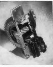
Typical CLARE stepping switch. Type 20, is shown above. This switch offers up to 480 contact points in twelve 40-point levels, or 320 in sixteen 20-point levels.
