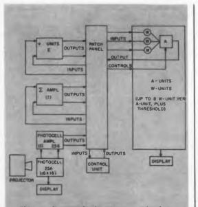
This medium-scale learning network of the perceptron type is under construction at Aeronutronic Div., Ford Motor Co., to test design of the company's biax-type magnetic integrators, which are intended for Cornell Aero Labs' perceptron program.
