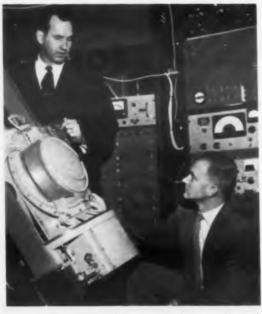
A Mark II inertial guidance system for an advanced, 2,500-mile version of the Polaris missile is under development by a team of 300 engineers and technicians at Massachusetts Institute of Technology's Instrumentation Laboratory. Shown inspecting the Mark I system, used in the present 1,200-mile version and a 1,500-mile Polaris now in development, are Ralph Ragan, left, deputy associate director of the Laboratory, and David Hoag, right, assistant director. These two head the Mark II system team.
