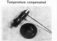
Model VCJ463 is available in fixed capacitance values from 2.0 to 12.0 pf. Operating temperature range is from -55 to 200 C. Capacitance tolerance is 3% at 25 C. Adjustment provides any temperature coefficient between -500 ppm and  $\pm 500$  ppm per C.
