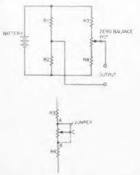
**Fig. 2.** If pot does not have sufficient range for zerobalancing, Wheatstone Bridge can be modified as in (a) or as in (b). Jumper is connected from either A to C, or from B to C, whichever permits the Bridge to be balanced.
