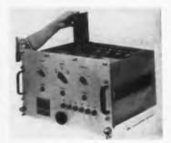
Developed for use in automatic checkout applications, the model M7 multimeter is a solid-state, analog-to-digital converter. Frequency measurements from 1 cps to 100 kc, to an accuracy of 0.01% 1 count, can be made in 0.1 sec. Periods from 0.001 to 0.1 sec can be measured to an accuracy of 0.01%. Voltage and resistance ranges extend to 1 kv ac or dc and 1 meg. The requirements of MIL-E-16400 are met.
