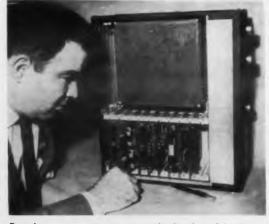
Random-access memory unit developed by Westinghouse Electric Corp. operates at 0.6-usec cycle time with an access time of 0.20 usec.
