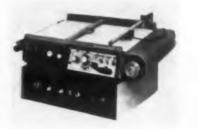
Any time delay encountered in a process control or experimental situation may be reproduced by the model 2D-5 transport delay simulator. It consists of a controller, a standard X-Y recorder, and an optical line follower. Delay time may be varied in steps from 2 to 32 min, or continuously from 4 sec to 7 min. Slopes up to 80 deg can be tracked to within 0.05 in. at speeds through 15 in. per min. An alarm circuit detects errors up to 0.1 in.
