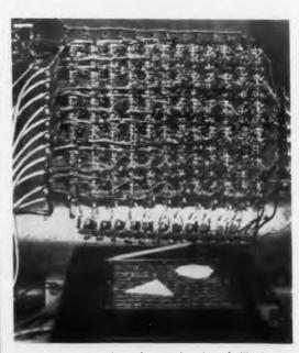
**Recognizer developed** at University of Illinois was designed to exhibit property filtering. System is able to sense the "n-ness" of whatever is laid on photocell matrix.
