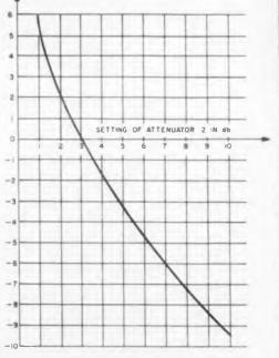
Fig. 2. Correction factor C can be found from curve when attenuator 2 is set at value other than 3 db.
