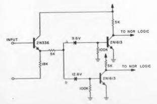
Fig. 3. Sample level detector provides no-go command if voltage level is below 11 v or above 14 v.
