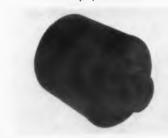
Designed to provide continuous quiet operation and long life, these multistage blowers deliver up to 100 cfm and meet pressure requirements to 1 psi. Low noise level makes them ideally suited for computer applications. Ambient temperature range is -55 to 85 C. Power requirement is 60 to 400 cps, 1 or 3 phase, to 440 v. Air Marine Motors, Inc., Dept. ED, Bayview
