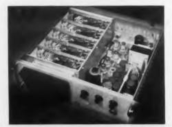
The 481A features the basic circuitry of the NLS 481, today's most widely used digital voltmeter.
