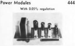
The series 5VT power supply packages deliver 150 to 425 v dc, at 100 to 400 ma. Output regulation is 0.05%, line and load. Ripple is less than 1 mv with either output terminal grounded or both terminals floating. Designed to mount in customer equipment, the supplies may be joined for higher outputs.
