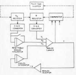
**Block diagram** shows how proposed analog-digital system could be used to solve the differential equation  $dx/dt \Delta x$ .
