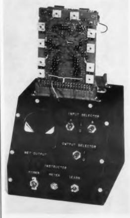
Device built by Philco to demonstrate and explore a concept of adaptive logic and to aid in patternrecognition research consists of "student" circuit board and black-box "teacher," which instructs student to learn 14 Boolean-logic propositions. Battery-operated circuit is wired as a net of three digital adaptive gates. Each adaptive gate may assume three states; shortcircuit, open-circuit, and inversion. Net organizes itself to recognize propositions, by relating two inputs and one output.
