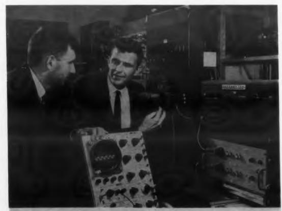
Adaptive waveform recognition system is able to pick limited-bandwidth signals out of high-level additive noise. System consists of four racks in background and paper tape recorder for monitoring performance.
