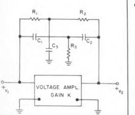
Fig. 1. High-Q active filter can be used in low frequency spectrum analyzer.
