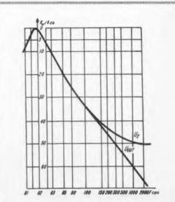
Fig. 3. Amplitude-frequency characteristics of compensated, U<sub>out</sub>, and uncompensated, U<sub>2</sub>, amplifiers. CIRCLE 861-869 ON READER-SERVICE CARD ➤
