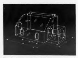
Fig. 3. Dimensions of a dust hood or dry box are based on a compromise length for a human arm. An average person can just barely reach all parts of the box. Room must be left for test equipment.
