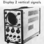
Types 1120 Portable and 1120-R Rack-Mountable permit the simultaneous display of two vertical signals against time, against each other, or versus a third variable fed externally to the X-axis. These main-frame indicators have 64 contacts to mate with plug-in circuits. Both are designed for safe off-ground operation up to 500 v dc.
