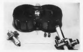
Millimeter wave sources in use at Lincoln Laboratory. From left to right: Raytheon QK396 klystron (4 mm), Compagnie Sans Fil COE-20R carcinotron (2 mm), and Amperex DX151 klystron (4 mm). Note the small, rectangular output waveguide for all three tubes.
