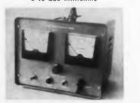
Designed for testing printed circuit boards and cable assemblies, this circuit resistance meter has a range of 0 to 200 milliohms. A safety circuit protects meters from overload damage. The solid-state device is permanently calibrated, and may be operated from 115/230 v, 50/125 cps, or from 30 v dc power supply. It measures 8 x 10 x 8 in. and weighs 11 lb.
