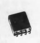
Series 2LB microminiature dc magnetic latch relay has rotary balanced construction and measures 0.4 x 0.8 x 0.875 in. Sensitivity at pull-in at 25 C is 150 mw spdt or 300 mw dpdt. Contact rating is dry circuit to 2 amp resistive at 32 v dc. Dielectric strength is 1,000 v rms, insulation resistance is 1,000 meg min.
