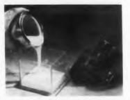
A fluid silicone rubber for deep-section potting, RTV 601 vulcanizes at room temperature to form solid sections of unlimited thickness. The low-viscosity material cures without heat, pressure, or moisture, even when totally confined. After 24 hr at 77 F, it can be put into full service at temperatures from -100 to 500 F. Set-up time can be lengthened or reduced without affecting the properties of cured parts.
