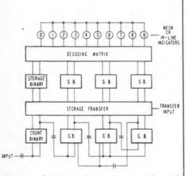
**Diagram shows** count-binary, storage-transfer, and storage-binary arrangement.
