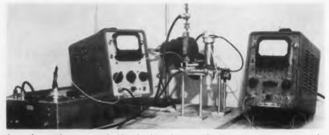
**1-mm harmonic generator** is driven by 4-mm Amperex tube. Harmonic generator types under study include varactor diodes, paramagnetics and point-contact silicon whisker diodes. This method is inefficient at the low powers available from klystrons.
