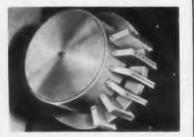
This magnetic drum delay and memory system, designed for process or equipment-control systems, has 20 channels with storage densities up to 9,000 bits per channel. Recording heads adjust to provide continuously variable delays from 2 to 60 sec. The system receives input from standard transducers; output is digital in the form of on-off pneumatic, hydraulic or electrical process control signals. Drum drive is by synchronous motor, servocontrolled synchro, or direct coupling.
