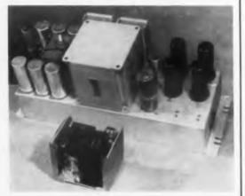
Space-saving preamplifier (foreground), which replaces the cumbersome vacuum-tube unit behind it, is part of a new all-transistor sound system developed by the Grass Valley Group, Inc., of California. The system, said to be capable of 450-w total audio power with fidelity to 20 kc, will be used by Cinerama, Inc., in theaters around the world.
