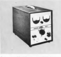
New portable fully transistorized d-c power supply. QR36-4AP regulates 0 to 36 vdc output voltage to  $\pm$  (0.02% + 1mv) against combined line or load variations. Fully metered. Front panel terminals for remote sensing. Circle 224 on Reader Service Card.
