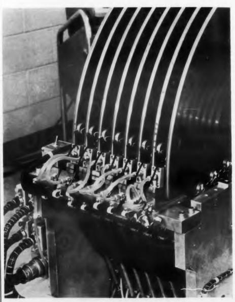
Hydraulically driven read/write heads track disk-filed data quickly and accurately.
