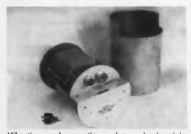
Vibration and acoustic analyzer, developed by Army in cooperation with Gulton Industries, operates at a frequency of 2,000 cps. Power requirement is approximately 75 ma.
