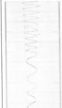
The unique carbon transfer writing method of AO's TRACEMASTER 8-channel recorder provides a trace that is a minimum of 2-3 times finer than that of any other direct writing recorder. The trace shown above, taken from a TRACEMASTER record, is an excellent example of the fine trace state and distinct, and reveals significant detail with great clarity.
