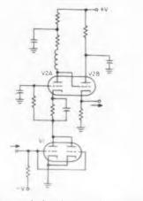
Fig. 1. Voltage gain bandwidths of over 650 mc can be obtained with cathode-follower coupled to cascode stage.
