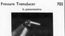
This miniature piezoresistive pressure transducer has a sensitivity of 40 mv per v. There are 3 ranges, from 0 to 25, 100, and 500 psig. Temperature range is from -65 to 350 F. Natural frequency is greater than 4 kc; dynamic frequency response ranges from 0 to 1 kc. Vibration sensitivity is rated at less than 0.008 mv per v per g.
