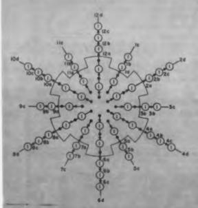
Network of logic elements is designed to transform 36 optic fibers into delay space. Each unit of length for an image transforms into a specified unit of time. Dark disks represent optic fibers, and cogshaped borderline represents outer boundary of delay transformer. Delay space lies outside this line. Image of a circle would be recognized by a coincidence of all even or all odd radials.
