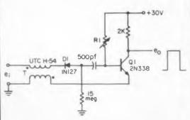
With input crossing zero and going negative, diode D is forward biased and transistor  $Q_1$  begins to cut off. Cut-off is hastened because emitter pulse is fed back to base through pulse transformer. Fast rise time pulse results at output.
