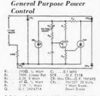
G:E Vac-u-Sel selenium bridge rectifier regulator 685X762 combination is available to replace CR, through CR: and CR: It rells for obstraintiely 54 00. The circuit shown is a full wave phase controlled rectifier. The unit is not only a fine lamp dimmer, but it demonstrates the versatility afforded by General Electric SCRs. For example, it can be used as a general purpose control simply by substituting other types of loads for the lamp.
