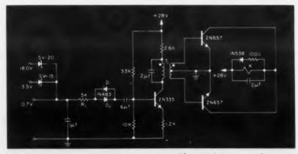
Fig. 2. Null detector is basically a transistor amplifier with full-wave rectification for relay operation.
