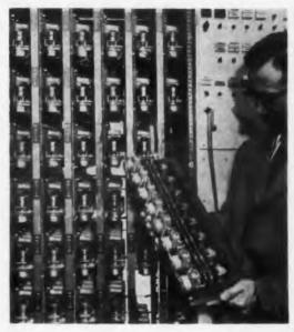
Mark I perceptron, now moved to Cornell University, first full-scale learning machine used for pattern recognition, is prototype for smaller versions in many organizations. Mark II now in design at Cornell Aeronautical Laboratory will be special-purpose digital computer programed for threshold logic. Elements shown are transistor-driven relay circuit that operates as association units
