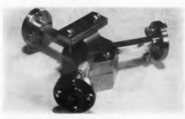
**Three-port, Y-type circulator** developed for use at 4 mm. Small permanent magnet clamped to top supplies field for ferrite rod inside cavity.
