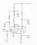
Fig. 2. With a single pentode-triode tube, gainbandwidth is still high, but somewhat decreased.
