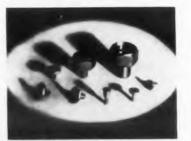
The cold-formed bases of these semiconductor mounts are oxygen-free copper or a zirconiumcopper alloy. The former material has higher thermal conductivity than the conventional tellurium-copper alloy. The zirconium copper retains its strength at brazing and welding temperatures. The base doubles as heat sink and electrically conducting mount.
