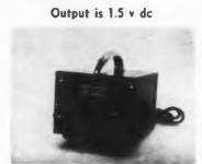
This solid-state power supply, designed for use with thermo-electric cooling units, changes 115 v, 60 or 400 cps, to 1-1/2 v dc. Ripple content is less than 10%. The 4-1/2-lb unit measures  $3 \times 4 \times 5$  in. It is available with adjustment and meter.
