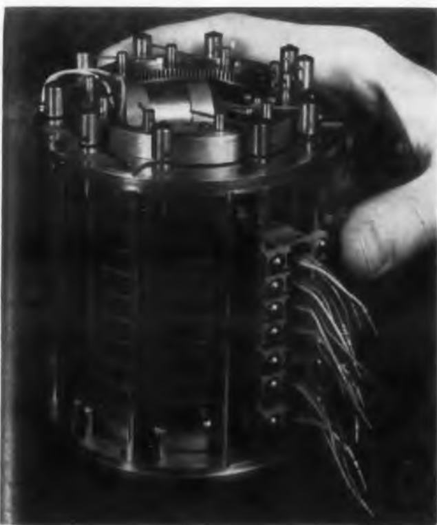
Miniaturized drum assembly shows seven read-write heads in place. Up to 60 heads can be used depending on application.
