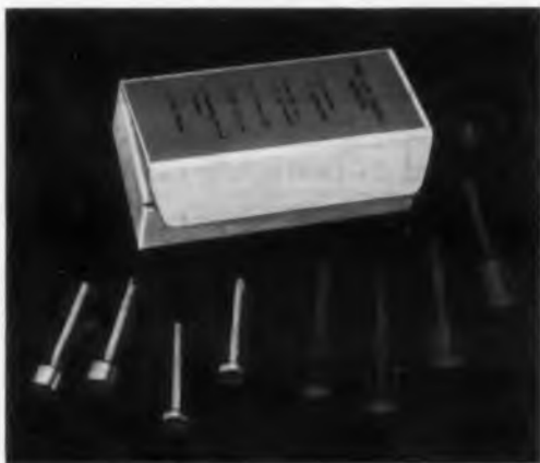
Two each of these four different types of cores: 1) red dot, 5.0 permeability; 2) blue dot, 9.2 permeability; 3) 1/4" brass; 4) 3/16" brass.
