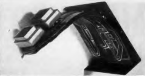
AFTER — Wiring Errors Eliminated; Weight, Cost and Time Saved Using Flexprint Wiring
