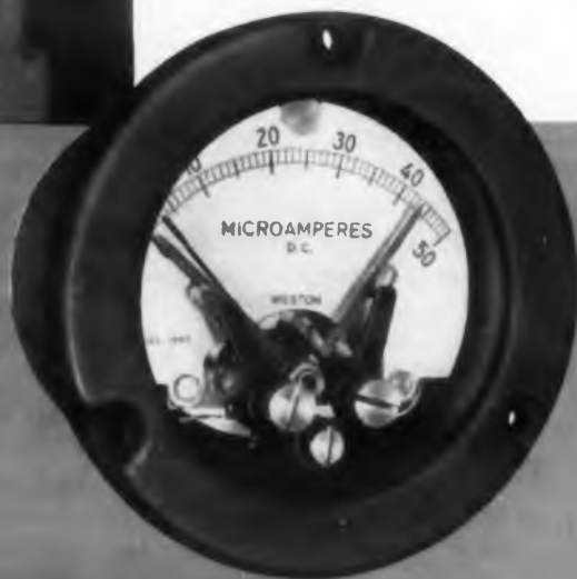
Model 1097 Load Current-Contact Aiding Relay is 3½" in diameter, with a 100° scale. Accuracy: within 2% of full scale. Contact rating 5-25 ma DC at 75-125 volts DC. Available in 24 types.
