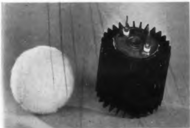
Only slightly larger than a tennis ball Transitron Electronics Corp.'s thermoelectric generator delivers 10-12 w output with 6-8 per cent efficiency. The device, available for engineering evaluation, uses lead telluride elements and operates at a hot temperature of 300 C and a cold temperature of 150 C.
