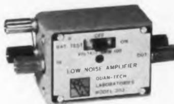
**LOW NOISE AMPLIFIER.** Model 203: A very low noise, self-contained, miniature transistor amplifier. Features a voltage gain of 100 and a frequency range of 30 cycles to 100 kc. Increases sensitivity of Model 303 to 1 microvolt full scale.
