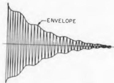
Fig. 3. This oscilloscope (slow sweep) pattern results when tuning fork is unbalanced (traces are at two different frequencies).
