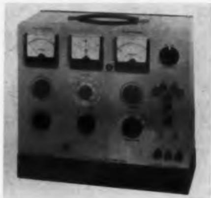
Power transistor measurements to 30 amp collector current and 300-v breakdown test potentials are possible with the Type 300 precision power transistor test set. Direct meter readings of large signal current gain,  $H_{FE}$  and collector characteristics,  $I_{CBO}$ ,  $I_{CER}$ ,  $BV_{CEC}$ , and  $BV_{CBO}$ , can be made under conditions typical of their actual applications.
