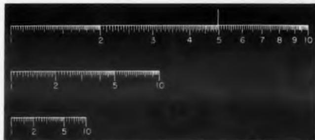
Fig. 4. The scales of Fig. 3 subdivided twice as often. Excessive subdivision of scales reduces readability.
