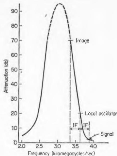
Fig. 8. Ferrite resonance absorption curve showing application to receiver image rejection.
