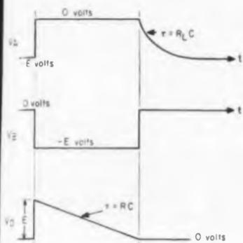
**Fig. 2.** Voltage waveforms at several points of conventional multivibrator circuit for a fixed  $R$ , and low-duty cycle.
