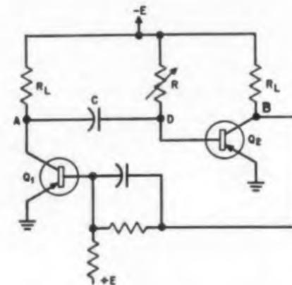
Fig. 1. Conventional, collector-coupled, monostable multivibrator.
