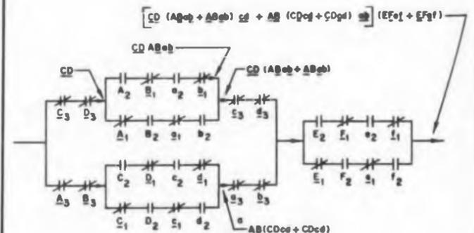
**Fig. 1.** The hardware equivalent of the mathematical solution. Each symbol represents a relay contact. The letter denoting the contact denotes what relay it is on. Letters with bars represent normally closed contacts; letters without bars, normally open contacts.
