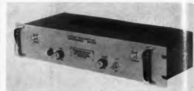
Model HFW-5(C)-326 vhf amplifier, having a coverage of better than three octaves, provides a 20-db gain and an 8-db noise figure. The range is 30 to 265 mc; source and output impedances are low. The unit features synchronous tuning. Using five tubes, it requires 22.5 w of anode power and 1.5 w of heater power. Dimensions, not including those of the optional power supply, are 19 x 3.5 x 6.5 in. Weight is 7.25 lb.
