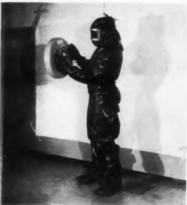
Suit to protect against high-density rf radiation is made of neoprene-coated nylon with nylon linings. Visor is wire mesh.
