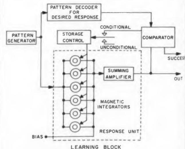
How modified Biax elements are connected in learning block of Aeronutronic perceptron.
