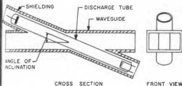
Fig. 2. Microwave noise source is placed in waveguide at angle of 5-10 deg.
