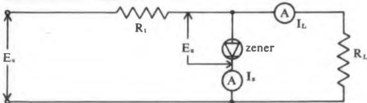
As the input voltage increases the inverse bias across the zener diode will increase and cause a large current to flow. This increase will cause more current to flow through  $R_1$  and increase the drop thereby adjusting the load voltage. Load variations have a similar effect. The result is a substantially constant output voltage.
