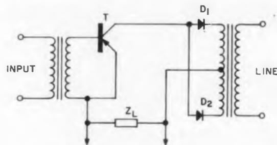
Fig. 5. Amplifier fed with pulsating current.
