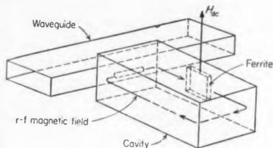
Fig. 7. Ferrite-loaded band elimination filter,  $TE_{101}$  cavity mode.
