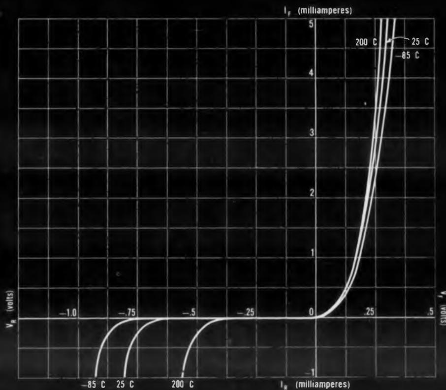
TYPICAL UNI-TUNNEL DIODE CHARACTERISTICS
