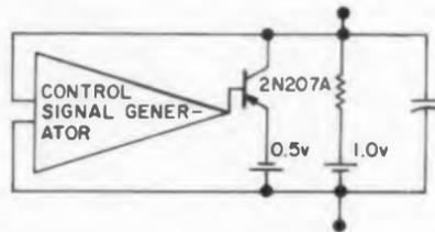
value. The integrating capacitor is discharged through the transistor, which is biased so that it is highly conducting when the membrane potential is near its resting value.
