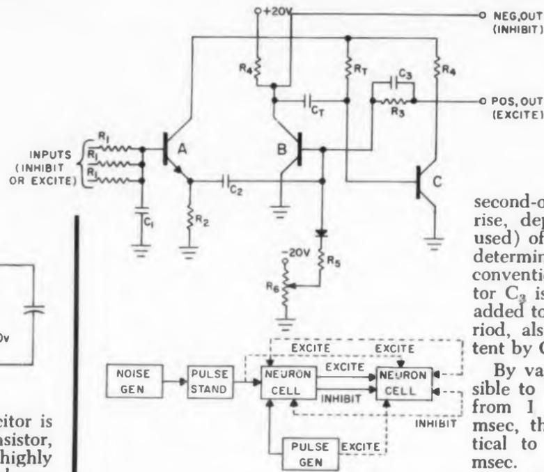
Clever circuit design enabled researchers at the Applied Physics Laboratory of Johns Hopkins University to build a more ambitious neuron analog by modifying a single-shot multivibrator. Transistor A is an emitter follower included to sum several inputs without interfering with the time constants on the base of transistor B of the multivibrator. Capacitor  $C_1$  simulates the
