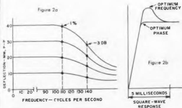
Frequency and amplitude response are shown in Fig. 2a, while Fig 2b depicts the square-wave response for optimum frequency and optimum phase monitoring.
