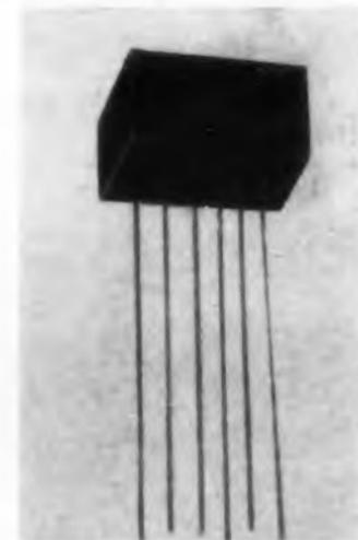
This rectangular transistor audio amplifier, measuring 1/2 x 1/4 x 1/4 in., has four stages and a density of 416 components per cu in. The device has a gain of 65 db at 1 kc, an input impedance of 2,500 ohms, and an output of 5 mw without clipping. Response is to 20 kc. A 1.34 v mercury battery serves as power supply. The amplifier drains 1.8 to 2.4 ma.
