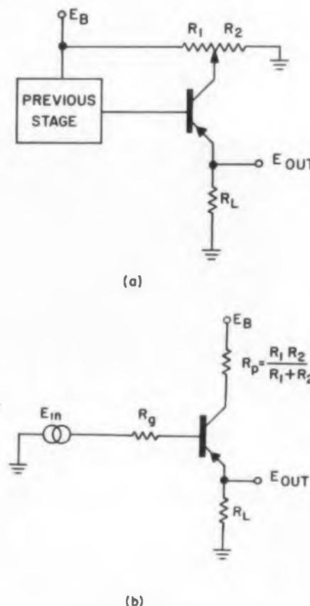
Fig. 1. Output voltage of this pulse amplitude limiting circuit (reprinted from Ideas for Design, *ED*, April 27, 1960, p 120) is still a function of the input voltage (see Eq. 1).
