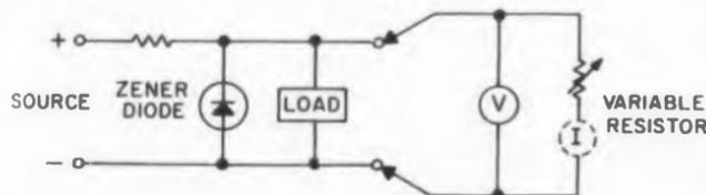
Current in variable resistor equals Zener diode current when voltmeter reading begins to drop as resistance value is reduced.
