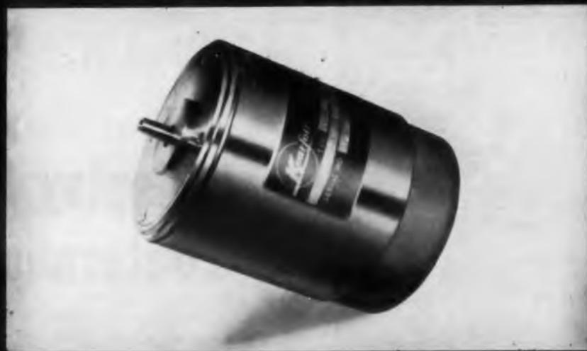
Available in both conventional and gimbal mounted configurations, these synchros provide component accuracies of 20 seconds of arc or better. They permit RMS accuracy for 3 unit strings of better than 0.75 minutes. Specifically designed for precise data transmission in missile-borne applications, these components eliminate the need for 2 speed servos and complex electronics, provide increased reliability and marked improvement in over-all system performance.
