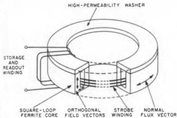
In this modified Biax element, orthogonal field is not uniform throughout cross-section.
