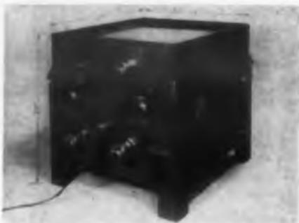
Heat transfer test fixture, model T-400, measures the heat transfer rate from an electronic module to the cooling air stream in a well-defined temperature environment surrounding the module. It can accommodate a module up to 9-in. wide by 4.5-in. high. The outer structure measures 20 x 20 x 20 in. The fixture will condition 0.4 lb of dry inlet air per min over a temperature range of  $-20$  to  $+70$  C. Maximum input power is 900 w.
