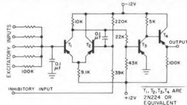
This electronic neuron, developed at Bell Telephone Laboratories is a four-transistor device with variable threshold capable of an integrating time constant of 2 msec and a refractory time constant of about 10 msec. These values approximate those of biological neurons.
