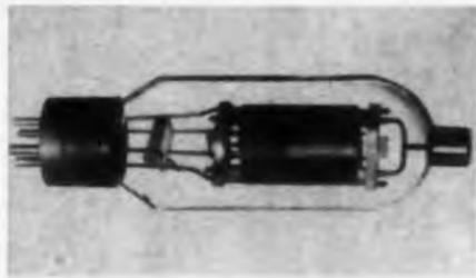
Type 572 triode is a ruggedized, one way replacement for the prototype 811A in most applications. Ruggedized construction includes hard glass envelope, heavy-duty tungsten lead wires, a non-frangible filament and enclosed getter traps. The manufacturer claims the 572 has a 50% increase in plate dissipation over the 811A.
