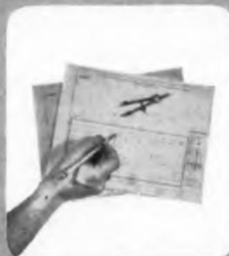
Schematic is laid out, full scale, on Alden Terminal Card Planning Sheets.
