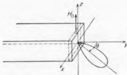
Fig. 9. Ferrite radiator.  $\theta$  is measured in y-x plane.
