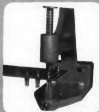
Using planning sheets as masters, terminals and sockets are swaged and eyeleted securely into place on pre-punched terminal cards.
