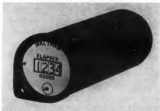
Type WT-3 elapsed-time indicator with digital readout weighs 3.75 oz, measures 1-1/16 in. OD x 2-3/4 in., and operates at 360 to 440 cps with a 2.5-w maximum power input. The digital presentation runs to 9,999 hr and the numerals are 5/32 in. high. Jewel bearings are used.
