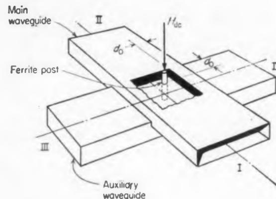
Fig. 5. Crossguide ferrite directional coupler.
