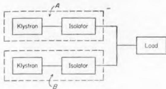
Fig. 2. Use of isolators in isolating sub-systems.
