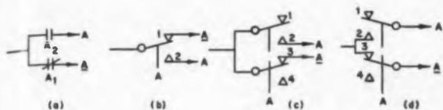
Fig. 2. How to convert the symbol for two parallel, opposite-acting contacts on the same relay into the actual relay configuration.
