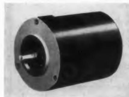
This self-orienting, synchronous motor insures synchronization of the rotor within  $\pm 5$  deg with respect to the rotating stator field. No dc excitation of the rotor is required. Motor is two phase, 60 cps, 115 v ac; synchronizing pull-in torque is 0.50 oz-in.; fall-out torque is 0.65 oz-in. Unit measures 2 in. long with a 1-3/4 in. diam and weighs 10 oz. Units designed for 400 cps are also available.
