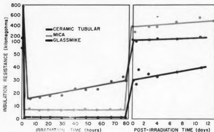
Fig. 3. Post-irradiation recovery of insulation resistance is illustrated for three capacitor materials.
