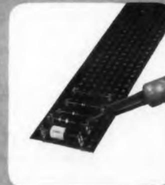
Components are snapped into terminal jaws, ready for soldering.
