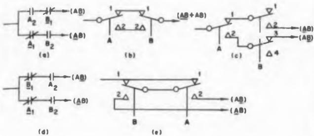
Fig. 3. How to deal with parallel paths through two relays. Part (b) indicates how a careless arrangement of connections can give an undesirable output.
