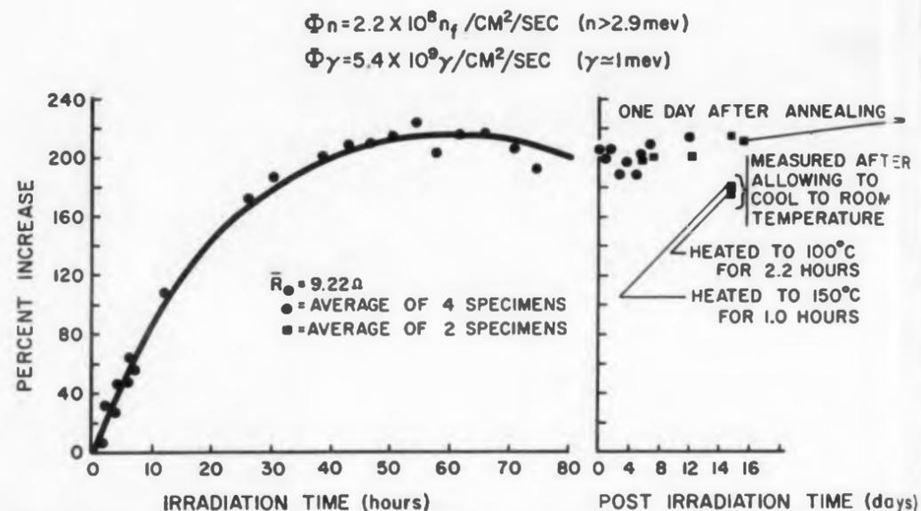
Fig. 4. Permanent increase of forward resistance of germanium diodes would not be reduced by annealing.
