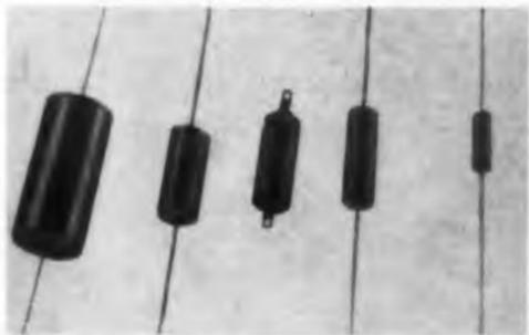
The HI-Lar mylar film capacitors are for high-altitude space probe applications. Other uses are in instrument-quality recorders, pulse networks, and computers. The line is available in increments of 100, 200, 400, and 600 v and in ranges of 0.0047 to 1  $\mu$ f. Temperature range is  $-55$  to  $+125$  C, dielectric absorption is 0.1%, and retrace stability is less than 0.2%. Dissipation factor is less than 0.5 at 25 C and 100 cps.
