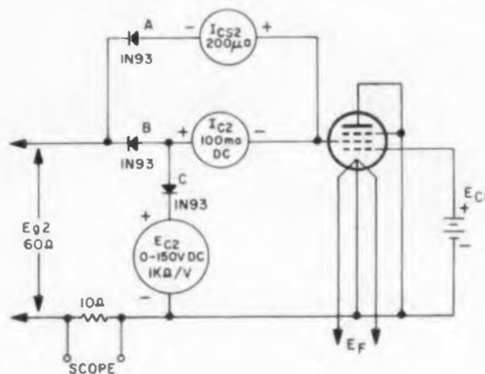
Reverse screen grid current is measured after tube has been operated at rated screen dissipation for five minutes.
