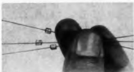
Type 375-P wirewound resistor is an encapsulated, precision unit that measures 1/8 in. long by 1/8 in. in diameter. Wattage rating is 0.05 w; resistance is 100 K; voltage is 50 v max. Temperature range is -65 to +125 C, standard tolerances are from 1% to 0.05%; standard temperature coefficient is  $\pm 0.002\%$  per deg C.
