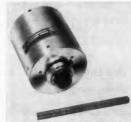
Model VM-1030 Delay Line features a continuous range of delays from 3 to 500  $\mu$ sec with an accuracy of  $\pm 0.5$   $\mu$ sec. It has an optimum pulse input of 1  $\mu$ sec and can be supplied with an impedance range of 50 ohms to 4 K. Insertion loss at the end of the range is 56 db and the maximum number of pulses per second is 300 kc. The unit is 4.406 in. in length with an OD of 3.398 in. Total weight is 2 lb.
