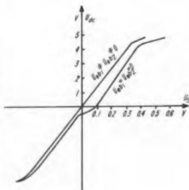
Fig. 3. Dependence of the dc load voltage of a push-pull phase sensitive circuit on the signal, for different (but constant) emitter - base voltages  $U_{eb}$ .
