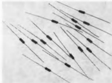
Types 1N625 through 1N629 diodes are fast recovery units providing 400,000 ohms in 1 μsec. Types 1N482 through 1N485 diodes are high-conductance units with a 100-ma max avg forward current at 1.1 v. The devices are designed for airborne and industrial computers. Shock and vibration resistance exceeds MIL-STD 202A.
