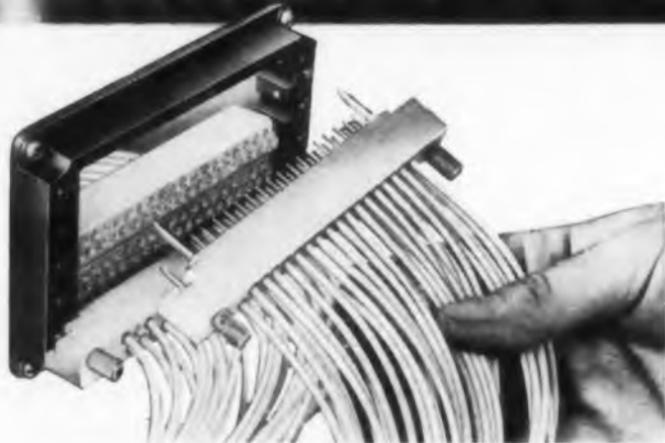
HYFEN-type connectors like those used in the "vest pocket" air defense system have pins and sockets tool-crimped on cable ends, snap-locked in inserts with wide range of configurations. HYFEN and STAPIN inserts are mounted in panels as required.
