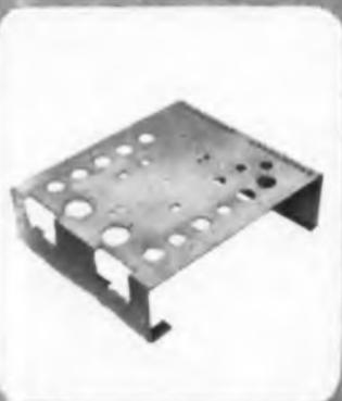
Card-mounted circuitry is snapped in or bracket mounted to pre-punched, pre-shaped chassis.
