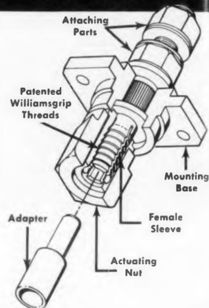
**Williamsgrip electrical connectors** provide quick connect and disconnect with a flick of the wrist... plus full positive connection insuring maximum conductivity without the use of springs, slip joints or friction methods.
