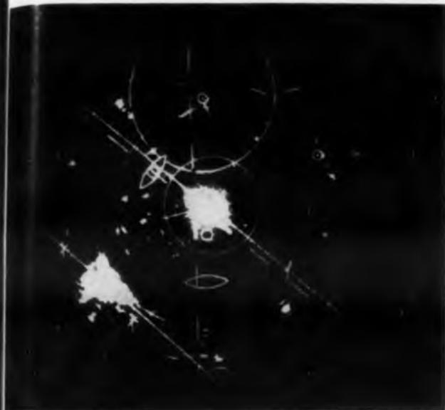
Effects of moving target capabilities of Texas Instruments ASR-4 radar are shown in display.
