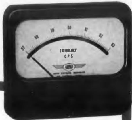
These highly accurate, dependable Frequency Meters by Airpax, are completely self-contained. Connection is simple. Two meter terminals protruding from back of case connect directly across 100 - 130 volt source. Airpax MAGMETER® frequency sensing circuit is insensitive to voltage variations, responding only to frequency changes.
