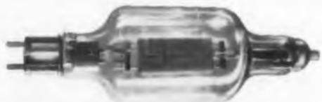
**HIGH-VACUUM, HIGH-VOLTAGE** rectifier made by General Electric with shield of Electronic Grade "A" Nickel.
