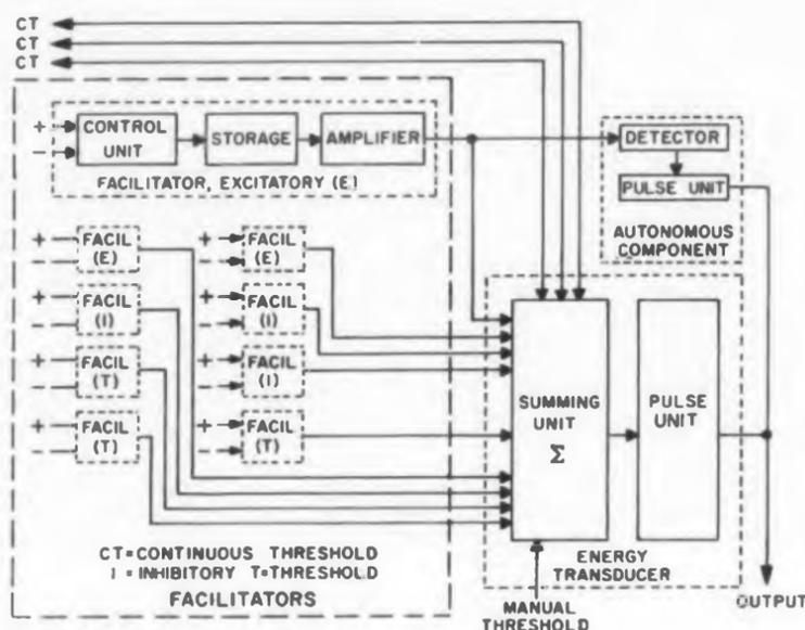
This "elementary unit" of the University of Illinois "adaptive reorganizing automaton" is believed to be the only neuron simulation that is truly active—one that gives a response when there is no stimulus. It is the basic building block of the adaptive machine, which has learned to recognize such situations as a person walking from left to right across the field of its photocell retina.
