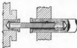
Coupling is used for the transmission of power or control of movement between parts located close together in a piece of equipment. It is not a separate type of flexible shaft but an added application.
