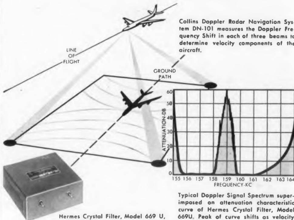
Collins Doppler Radar Navigation System DN-101 measures the Doppler Frequency Shift in each of three beams to determine velocity components of the aircraft.
