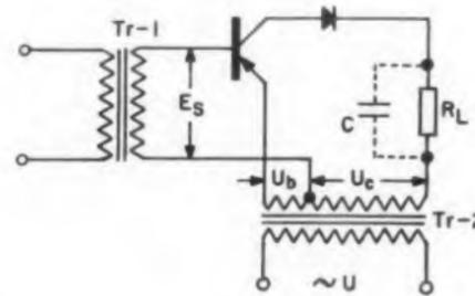
Fig. 1. Single-ended phase-sensitive circuit.
