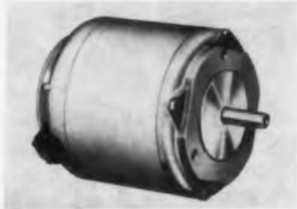
Type SS250 synchronous motor is designed primarily for industrial uses. It has a torque of 250 oz-in. and a constant speed of 72 rpm. A dc voltage applied to its field windings converts one revolution of the motor shaft into 200 precise steps. Ratings are: input, 120 v, single phase, 40 to 70 cps, 0.6 amp max at 60 cps; 72 rpm output at 60 cps.
