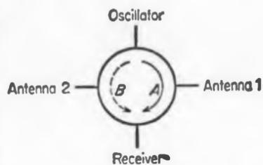
Fig. 3. Switching of antennas using circulator.
