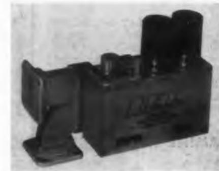
The MMX-6 matched X-band microwave receiver head end assembly covers the 8.5- to 9.6-kmc range with a maximum noise figure of 7.5 db. It has a typical noise figure of less than 7 db, an if bandwidth of 8 mc and an if gain of 25 db. The MMX-6 is electrically similar to the MMX-2.
