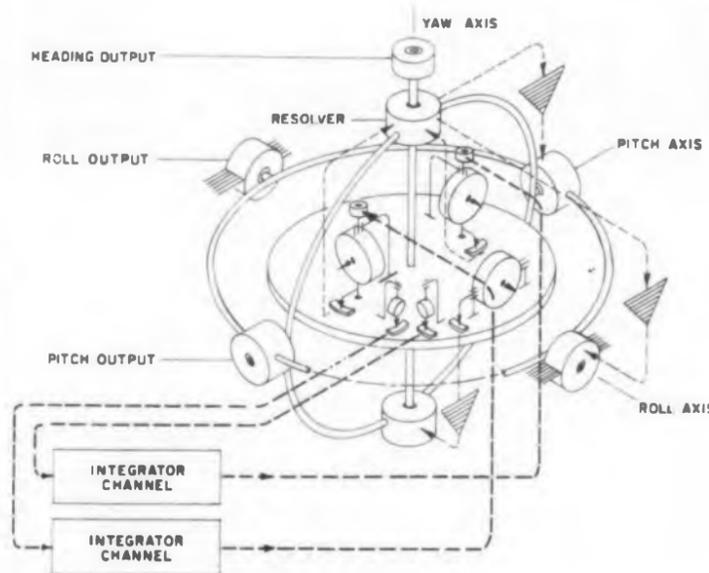
**Fig. 2.** Three-gimbal stable platform consists basically of three single axis systems to control roll, pitch and yaw. An additional azimuth coordinate resolver is also required.
