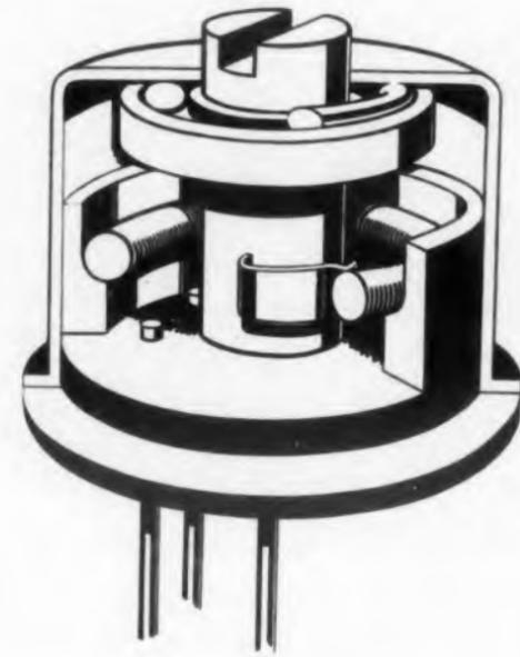
Cut-away shows simple construction of miniature trimming pot. Total outside diameter, including flanges, is 0.345 in. Pot is said to be one quarter the volume of conventional trimming units. Rotor screw is at top.
