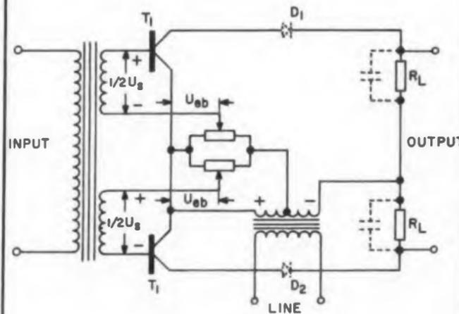
Fig. 2. Push-pull phase-sensitive circuit.
