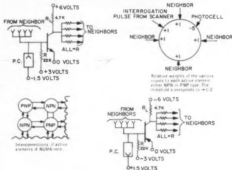
**Wiring of the elements** of the active array permits weighting of inputs as shown. Circuit at upper left is for npn units, circuit at lower right, for pnp units. Each photocell is 1 cm sq. Circular drawing at upper right shows relative weights of inputs; threshold corresponds to plus one half.
