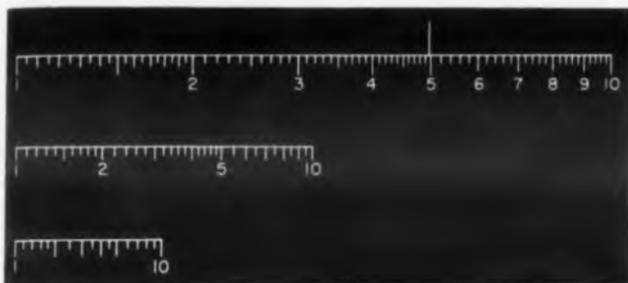
Fig. 3. Logarithmic scales of arbitrary units divided according to rules for maximum readability.
