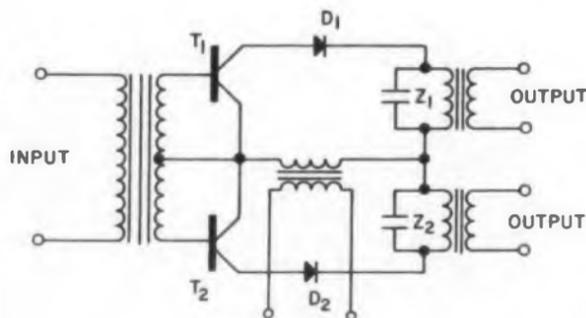
Fig. 4. Phase-sensitive circuit feeds load through twin transformers.
