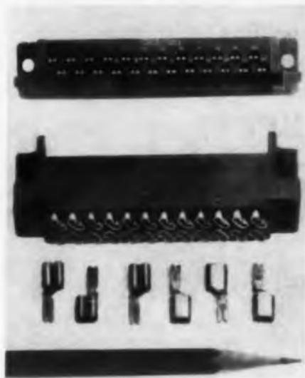
The series 7009, Varitwin-Pin printed circuit connectors have 24 contacts. Wire terminations are twin taper-pin type. Insulator is one-piece, glass-filled diallyl phthalate. Contact terminations have dual connections and accept Series 53 taper pins. A polyethylene tab can polarize the unit.
