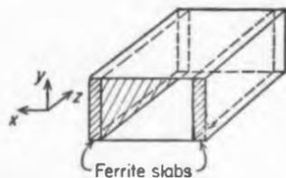
Fig. 4. Magnetic tuning of the resonance frequency of a ferrite-loaded cavity.
