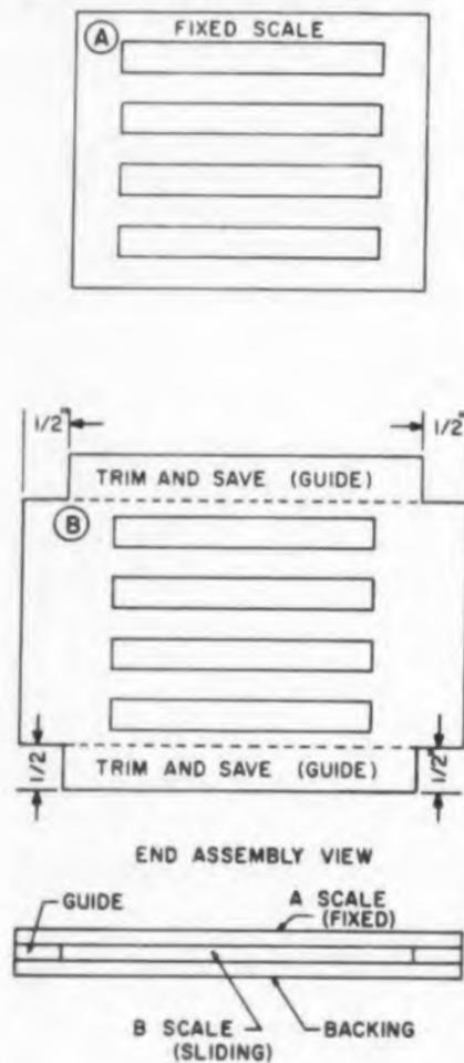
Fig. 1. Assembly details for the transistor parameter converter.
