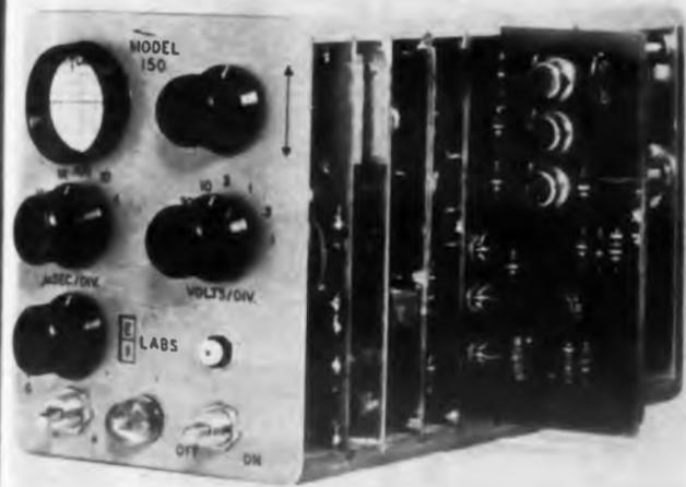
The Oscilloscope consists of 11 parts, the case, guide rails, "mother" board, 5 circuit cards, plug-in front and rear panel assemblies.
