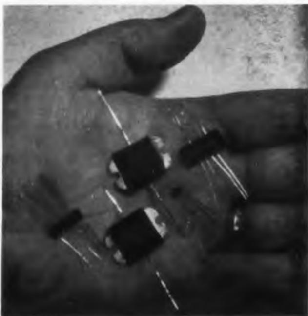
Westinghouse functional blocks are (left to right): multiple transistor switch, high-level two-stage amplifier, high-level three-stage amplifier, pulse generator, and bistable multivibrator.
