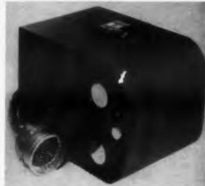
This Oscillograph, model 560A, is a miniature instrument weighing less than 10 lb. It is capable of accurate data recording under severe shock accelerations. Some models have withstood two-phase shocks in excess of 3,000 g for 2 msec and 300 g for 25 msec. The unit can record 14 different data traces on 3-5/8-in. wide record paper or film.
