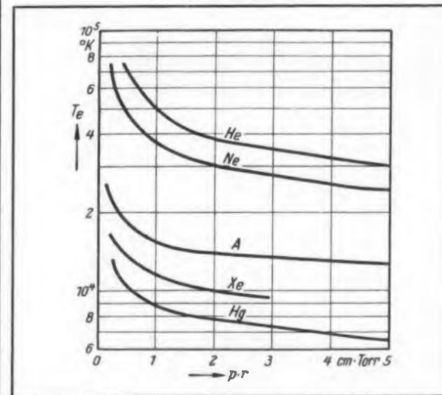
Fig. 1. Electron temperature,  $T_e$ , of various gasses as a function of discharge pressure-distance product (1 Torr = 1/760 atmosphere).
