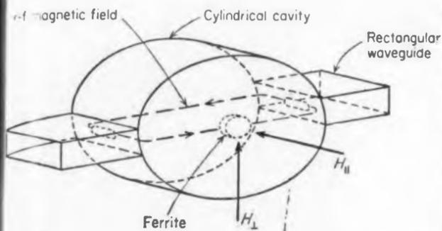
Fig. 6. Ferrite-loaded band pass filter,  $TE_{111}$  cavity mode.
