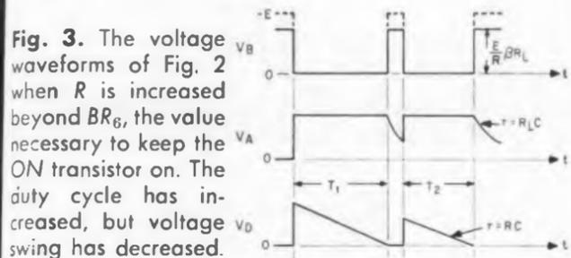
**Fig. 3.** The voltage waveforms of Fig. 2 when  $R$  is increased beyond  $BR_6$ , the value necessary to keep the ON transistor on. The duty cycle has increased, but voltage swing has decreased.
