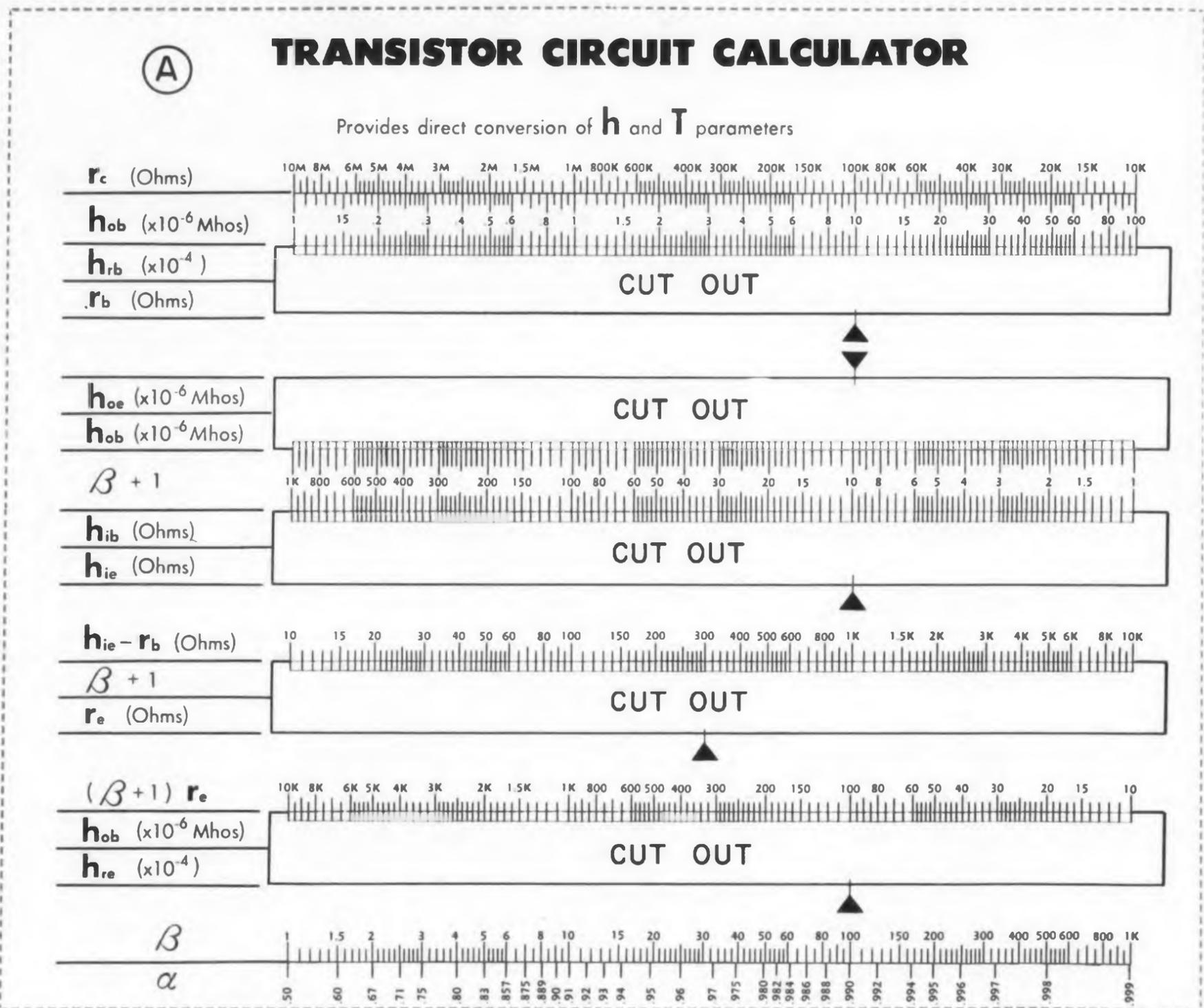
Next, center the A scale on one of the cardboards, and paste it in this position. Rubber cement is recommended. With a sharp razor blade or Exacto knife, trim along the outside guide lines, and then cut out the areas indicated, including those portions of the scales lying within. The A scale is now prepared.
