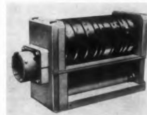
The model 602 electro-mechanical programmer is designed for programming on-off functions. It will handle 30, 2-amp circuits. Time range is 60 to 5,000 sec. Accuracy is 1%, 3% or 5%. Units include reset, solenoid latching, and a positive zero-time indicator.
