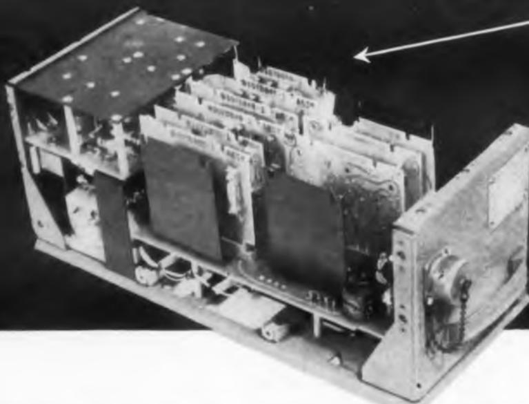
Uncovered control panel with transistorized panels in position.
