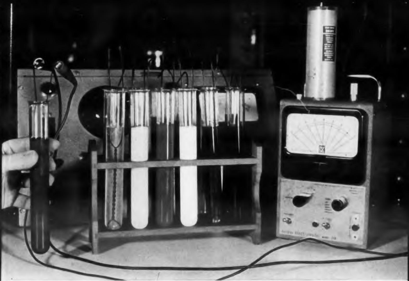
Compatibility testing of Epoxy Magnet Wire with encapsulating materials.
