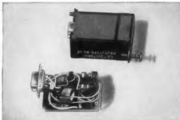
Eight amplifier module potted with RTV by the Armament and Control Section of G.E.'s Light Military Electronics Department. Used on the Lockheed CF-104 and F-104C jet aircraft, RTV provides mechanical support and vibration damping, protects unit against moisture and ozone. (Bottom photo shows module before potting.)
