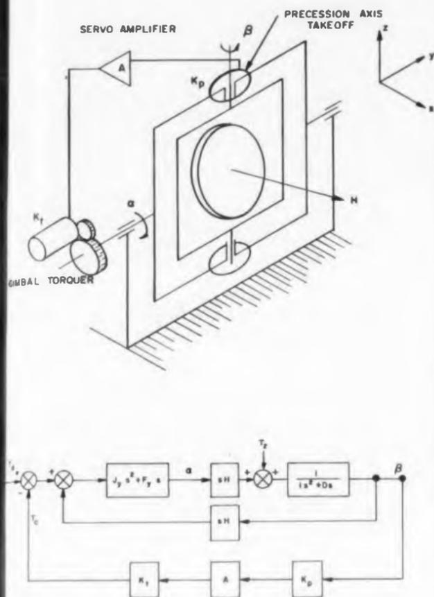
Fig. 1. Typical single axis platform with rate integrating gyros. The block diagram is used to analyze the platform motion.
