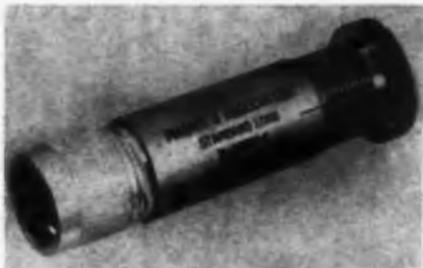
Model TL-2000 coaxial termination covers the 250 to 2,000 mc range, the TL-4000 covers the 2,000 to 4,000 kmc range; both units can be tuned to a vswr of 1.02 max within their respective frequency ranges. The variable mismatch that can be introduced is 1.5 from 1,000 to 2,000  $\mu$ c for the TL-2000 and the same for the TL-4000. This is done without changing the reference plane. Impedance is 50 ohms; power handling, 1 w cw.
