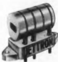
**CAT. 8715**—Ultra-High Temperature Socket for G.E. 7296 Triode can be soldered to printboard or mounted above or below a chassis. High Alumina insulating material; contacts gold plated Inconel-X. For continuous operation at 1000° F (538° C).
