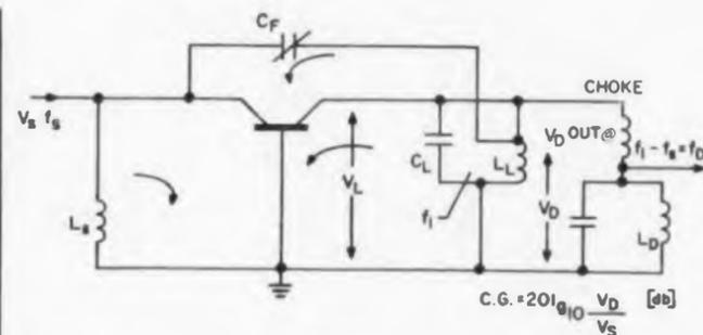
**Circuit designed** by Dr. Vodicka varies entire input impedance of parametric transistor for high-efficiency amplification.
