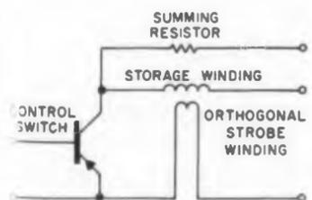
Schematic of integrator includes one resistor for summing.
