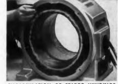
ENCAPSULATION OF STATOR WINDINGS, introduced by General Electric motor departments, extends service life of motors. RTV's resistance to moisture and other contaminants enables these dripproof motors to meet certain applications formerly requiring enclosed units.
