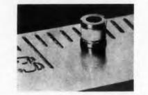
Having outside dimensions of  $1/8 \ge 1/8$  in., these microwave diodes offer cut-off frequencies up to 120 kmc. Applications are in travelingwave, broadband parametric amplifiers. The diodes can be supplied to  $\pm 10\%$  capacitance tolerance. Other uses are as low-loss rf switches in resonant cavities at microwave frequencies and for doppler radar sideband modulators. Type 4253X has a cut-off frequency of 120 kmc and type 4254, 100 kmc. Capacitance at zero bias is 1.4 pf.
