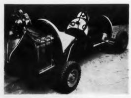
A prototype zinc-oxygen fuel cell is the power source for this racer. Tank in rear contains oxygen which is admitted under low pressure into the cell where power is produced by oxydizing zinc fuel in potassium hydroxide electrolyte. The cell will be developed first for electric industrial trucks. After testing, it might be adaptable to automobiles and trucks.
