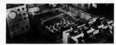
In production, this breadboard static inverter will be compressed into a package providing 50 w per lb, 3.5 w per cu in. of 3-phase, 400 cps, stepped-sine-wave, 110 v ac.
