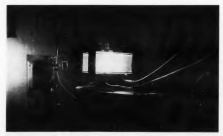
The discharge of this exploding wire generates cylindrical shock waves. The waves are being studied in plasma and astrophysic research conducted at the Boulder, Coio., laboratories of NBS.
