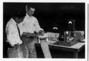
Stephen Chai and Glenn Cooper, Westingbouse development engineers, calibrate the Visicorder and other equipment used in water wheel generator tests.
