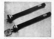
Model 1058 coaxial termination handles 75 w of average power without artificial cooling. It is for use over the S-band from 2.5 to 3.5 kmc and has a maximum vswr of 1.15. Length is 10 in. It can be furnished with either UG-45/U or UG-46/U connectors.
