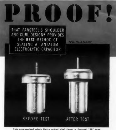
tantalum capacitor before and after being subjected to internal pressures of 600 psi. As shown, the test resulted in a stretching and deformation of the silver case, but no failure or leakage whatsoever in the seal.
