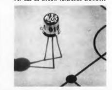
Types 1N2041 and 1N2969 germanium tunnel diodes, designed for use as circuit reference elements, have peak current ratings of 4.7 and 2.2 ma, respectively. These ratings are held to a variation of no more than 10%. Peak-to-valley ratio for both devices is 8:1. The 2N2941 has a total capacity of 30 pf and the 2N2969, 20 pf. The units have typical peak point voltages of 55 mv, typical valley point voltages of 350 mv, and typical forward peak point current voltages of 500 mv.
