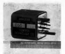
Model 250 isolation amplifier has an input impedance of 200,000 ohms and an output impedance of 700 ohms. Gain is unity. The unit uses silicon transistors and operates on standard 28 v dc power. Uses are in computers, servo devices, and automation applications. Able to meet MIL-E-5272 requirements, the unit operates from -55 to +125 C.
