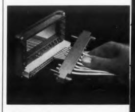
Both inner and outer contacts are crimped to the conductors, simplifying a previously complicated and difficult process. In addition this process eliminates many of the parts formerly used, and also eliminates any heat in the connection process. The result is a reliable coax connection, easily and quickly installed.
