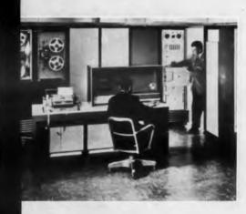
FLIGHT TEST CHECKOUT - Lockheed engineers monitor automatic checkout equipment in final check of test missiles prior to shipment to Cape Canaveral or Vandenberg AFB for development flights.
