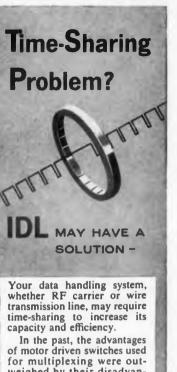
for multiplexing were outweighed by their disadvantages. They were smaller, lighter and simpler but, because of high contact resistance, bounce and short life, they contaminated data.
