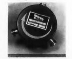
Designed to operate at 1400 mc, model X-101A broadband, three-port circulator has better than 15 db isolation from 1200 to 1500 mc and a peak isolation in excess of 20 db. Ratios of isolation to insertion loss are high over better than 10% bandwidths in the range of 1 to 2 kmc. From 1200 to 1500 mc the insertion loss is 1 db; at band center it is typically 0.5 to 0.6 db. The unit can be provided with an electromagnet for applications requiring a switchable unit.
