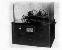
Model 8540 arc resistance tester provides 15 kv at 60 ma ac for testing the ability of solid electrical insulating materials to resist the action of an arc in accord with ASTM Spec D-495 and Federal Spec LP406B. The bench-type instrument is suited for laboratory and production quality control applications. Voltage control is continuously variable from 0 to 15,000 v.
