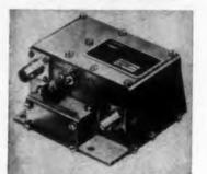
Model PA-11 10- to 25-w amplifier is for use with 1- to 5-w rf transmitters in the telemetering band of 215 to 260 mc. The frequency range is continuously tunable. The bandwidth is  $\pm 3$  mc. Input is 1.8 w and output is 10 w min into a 50-ohm resistive load with 1.8 w of driving power. The unit operates without forced-air cooling at rated temperatures and power. Heat transfer is sufficient for plate dissipations up to 15 w at 185 F. The unit stands shock and vibration.
