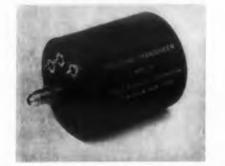
This series of pressure transducers, ranging from 0 to 25 up to 0 to 300 psi, is designed to stand 1,500 psi without shift or damage. The sensor design needs no auxiliary cut-off valving equipment. The units are for control, telemetry, and propulsion pressure measurement systems. Model 101, shown, measures 2.75 x 3 in. and is suited for differential pressure measurement applications involving the introduction of high pressures to the sensor and the instrument case.
