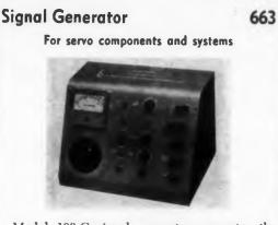
Model 100-C signal generator generates the waveshapes necessary for frequency and transient response tests of servo components and systems. These include the forcing voltages for the servo and the accessory waveshapes for display on the CR oscillograph. Outputs are low-frequency signals for dc servos or suppressed carrier modulations for ac servos. Data frequency coverage is in ranges of 0.01 to 1 cps and 0.5 to 30 cps. The unit accommodates carrier frequencies from 60 to 2500 cps.
