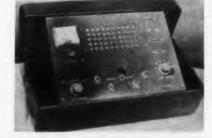
This automatic circuit tester is able to test 60 circuits per min. Designed for testing cable assemblies and components, the unit has applications in missile, instrument, and industrial fields. Three types are offered: a 50-circuit unit, a 100-circuit unit, and a 200-circuit unit. Continuity currents are 5 and 500 ma and 1 and 2 amp. The hi-pot voltage is variable up to 3000 v dc. The instrument measures  $11.5 \times 24 \times 15$  in.
