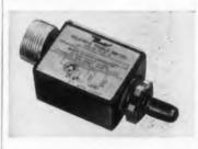
Developed for the severe environmental conditions outlined in MIL-E-5272A, this small, lightweight unit consists of a miniature micro-switch actuated by a toggle held in place by a solenoid-operated detent. In case of circuitry failure, the manually-operated toggle switch is returned to normal position automatically. Write for details.
