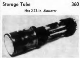
Type K1938 direct view storage tube is 2-3/4 in. in diameter. Over-all maximum length is 9-11/16 in. from the face to extremity of the 14-pin low-leakage type base. Writing speed is as high as 100,000 ips and resolution is 50 lines per in. It has a storage time of 2 min, erase time of 50 msec, and brightness level of 3,000 ft-L at 8 kv.
