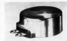
Designed for electronic heating or cooling applications, the Klixon 4286 low-differential, precision thermostat opens or closes on temperature rise. It is for use as a control device in guided missiles, aircraft control, computers, and crystal ovens. Continuous temperature exposure limits are -65 to +270 F; the temperature setting range is 0 to 250 F. Approximate weight is 3.5 g.
