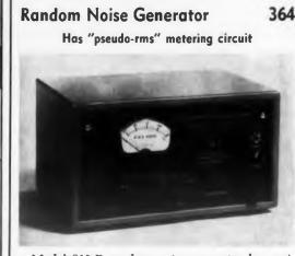
Model 811-B random noise generator has uniform output and a "pseudo-rms" metering circuit which reads identically on sine waves and white noise. It provides an output of at least 2.5 v rms on all ranges, and response is from 2 cps to 1.5 mc. A meter input jack enables its meter to be used for measuring other signals. It is available as a chassis unit, in a cabinet, or on a 19 x 5-1/4 in. rack panel.
