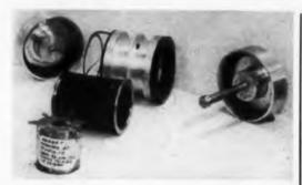
**Moon seismometer** built by Lamont Geological Observatory disassembled after air drop tests. Magnet (foreground) cracked on impact, but the rest of the device withstood damage. Dark cylinder in center is the seismic mass and carries windings for a push-pull moving coil pickup.
