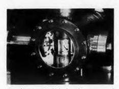
The chamber in which photodetachment and crossed-beam experiments are conducted. Ions enter from the left and interact either with electrons traveling vertically or with photons coming in through front window.
