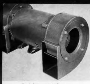
Fig. 2. Duplex centrifugal blower uses common motor to drive two fan wheels.
