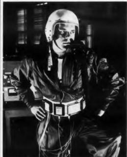
Laboratory spacemen at the Boeing Space Medicine Section in Seattle are wearing instrument-laden belts during physiological experiments. The instruments shown include an electrocardiograph, phonocardiograph, respirometer, and electro-encephalograph. Designed primarily for laboratory work, the instruments are said to give results equal to those of standard-size equipment. They are packaged to operate from -40 to +110 F, with static acceleration up to 1 g and vibration up to 5 g and 500 cps.
