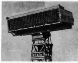
The corporate structure antenna is divided into a myriad of separate radiating elements, each of whose radiation can be carefully controlled.
