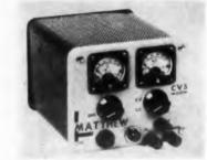
Designed for powering solid-state equipment, model CVS-300 power supply provides up to 400 ma at 30 v max on constant current operation and up to 500 ma at 4 to 36 v on constant voltage operation. A front panel switch sets the unit for constant current or constant voltage operation. Regulation is better than 1% against line and no load to full load variations. Ripple is less than 5 mv. For bench use or rack mounting, the unit measures 4.75 x 4.5 x 6.25 in.
