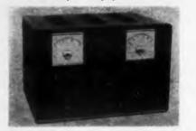
For measuring rf parameters of both npn and pnp transistors, model 1802 test set provides direct readings of the alpha cut-off frequency and gain bandwidth product for junction transistors up to 50 mc. It also provides direct readings of the RC product and the collector output capacity. The instrument is line-operated and needs no auxiliary equipment.
