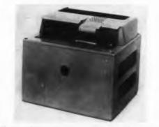
For reading out information stored on perforated paper, plastic, or metallic tapes, model 100 tape reader is for line-by-line reading at speeds to 60 lines per sec. A motor containing a printedcircuit armature can be started and stopped several hundred times a second. The tape reader has only one moving part. Its dimensions are 10-3/4 x 8-3/4 x 9 in.
