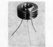
Types 2208 and 2209 heat sinks, designed especially for Mesa transistors, can be used for printed circuit board applications or can be mounted directly to the metal chassis. Heat generated in the transistor junction is conducted to the sink where it is removed to the surrounding air by means of fins.
