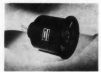
Operating on 115 v at 60 cps, type GR vane axial blower delivers 220 cfm of air at 1.75 in. of water static pressure and 3.5 cfm at 0 in. back pressure. Maximum current of free air delivery is 1.8 amp. Speed is 8000 rpm. The unit weighs about 4.5 lb and measures 4-3/4 in. in diameter and is 6-3/8 in. long. Housed in a black anodized aluminum enclosure, the blower can meet Mil specs.
