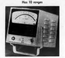
Model P-301 electronic millivoltmeter has 10 standard ranges from 0 to 10 mv up to 0 to 300 v. A dc meter, the instrument has an accuracy of  $\pm 2\%$  full scale on all ranges. Zero drive is  $\pm 1\%$  full scale for 8 hr. The input resistance is 10 meg.
