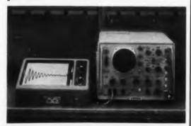
**Display scanner** (plugged into lower left part of scope) drives conventional pen recorder to present duplicate of scope waveform. (Waveform on paper has been touched up slightly to compensate for photographic losses.)
