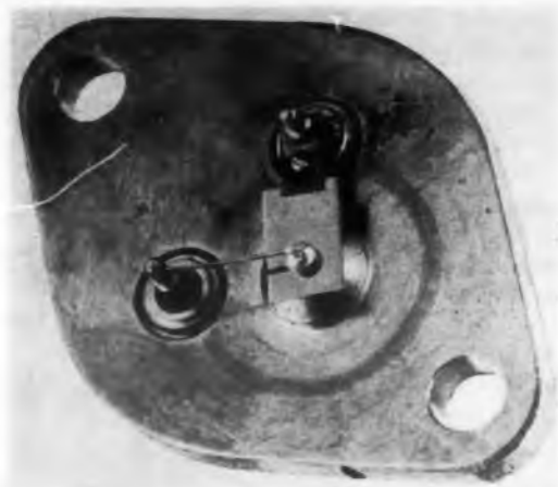
Fig. 1. A developmental 15-w MADT transistor, capable of switching 1 amp at a 5-mc clock rate.
