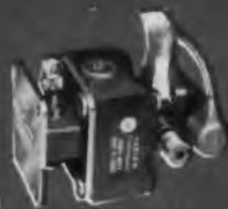
V-8302 Mixer with Varian VA-2F.8 diode and Boman BL-8-009 crystal protector tube
