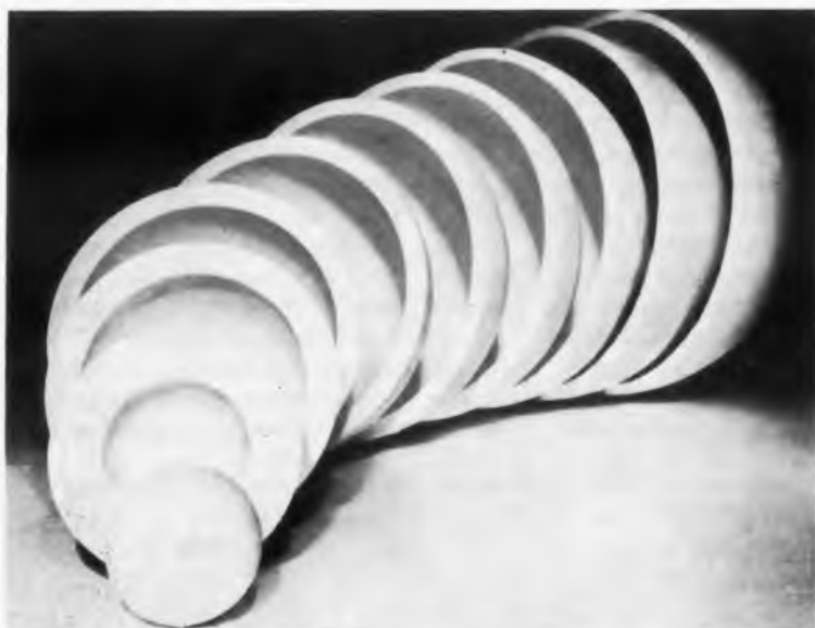
Fig. 3. Hemispherical half-shell construction of stepped-index Luneberg lens.
