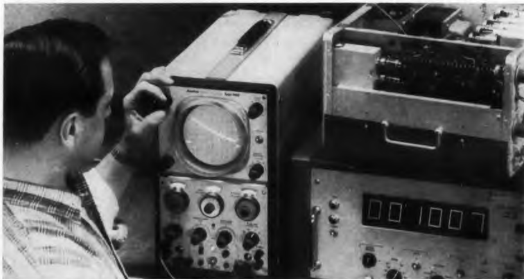
Calibrated sweep length pinpoints a desired time interval of digital decade counter and feeds start and stop triggers to Berkely Time Interval Meter. Scope shows number of counts per decade while Interval Meter displays duration in digital form.
