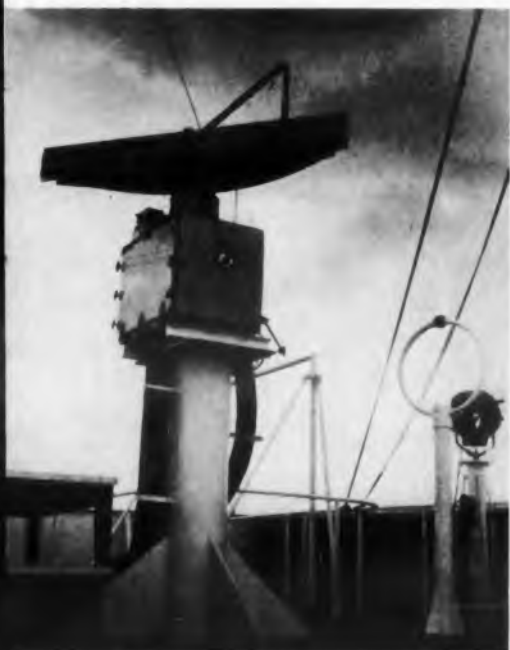
Fig. 4. The TMR case and antennas are mounted here on a ship's deck. The loop around the antenna is the feeder waveguide for the upper (transmitting) antenna.
