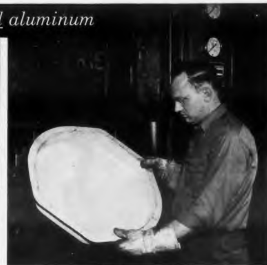
DRAWING. This gyro cover is drawn in a single operation. It replaces a part which consisted of welded components.
