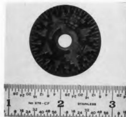
The left photo shows a complete unit; the right, the magnetic encoder disk.
