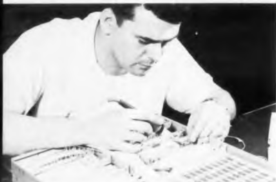
Terminal boards for Jupiter missile control system built by Chrysler Corp. Missile Div. fabricated from glass laminate made with Dow Corning Silicones.
