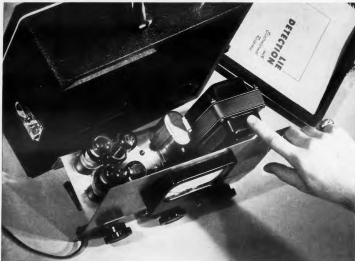
B & W Associates built in a Sola regulated plate-filament power transformer as an integral component in their portable lie-detection apparatus.
