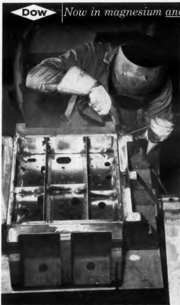
WELDING. Heliarc welding joins parts of this control central case. Dow facilities and personnel for welding are government certified.
