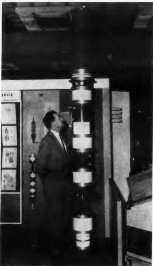
The klystron being fondled by Eitel-McCullough's H. C. Warner was used to power a radar signal to Venus and back—a distance of 56 million miles. Eimac displayed it at the show.
