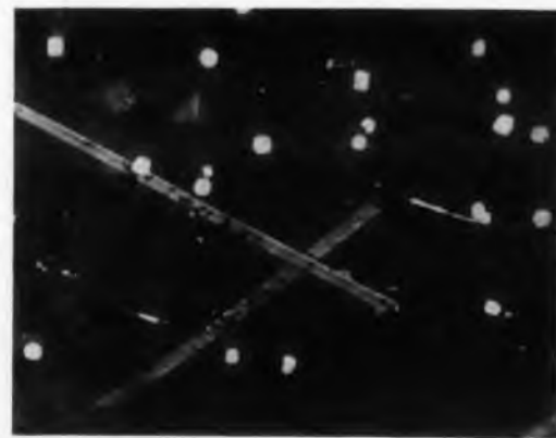
Common table salt and pepper dramatize the smallness of Pacific Semiconductors' "picotransistors."
