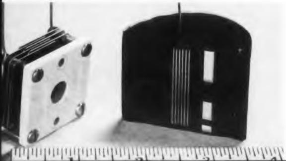
Analysis of the problems of size, weight, reliability and environment convinced engineers at G-M Laboratories Inc., Chicago, that a silicone insulating system would provide the best design for their servo motor. The stator is vacuum impregnated with solventless resins which fill the coil interstices. The void-free results achieved are clearly shown below by the bisected encapsulated capacitor.
