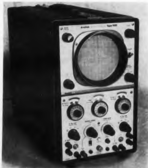
Null-readout , dual-channel scope gives voltage and time on 1-per-cent-accurate readout controls.
