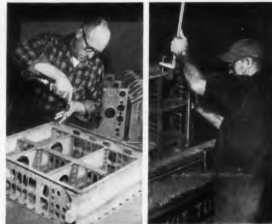
ASSEMBLY of this 4-deck housing with rivets, bolts and welds precedes FINISHING with Dow Number 17 anodic treatment.
