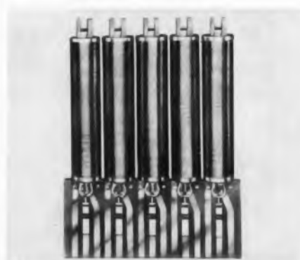
Fig. 2. Ten switches mounted in line, five on each side of a printed-circuit board, with five magnetic coils. This assembly may be mounted directly into a rack, or it may be enclosed in a flat, rectangular container.
