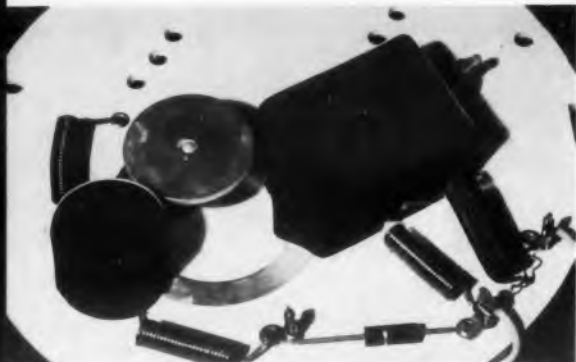
Silastic RTV protects General Instrument Corporation's Radio Sondes against high potential arcing and corona at 60,000 feet, as well as against launching shock and vibration at 565 knots.
