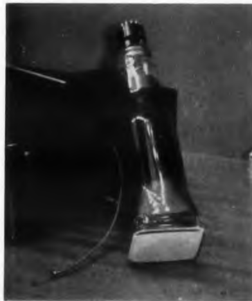
Transistorized oscilloscope crt developed by Electronic Tube Corp. rests against a scope camera. The rectangular-face tube is about 13 1/2-in. long. Electrostatic horizontal tapered deflection plates are almost as wide as the tube's inner diameter.
