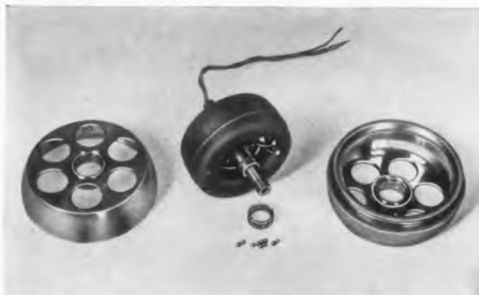
Gyro spin motor produced by Fafnir for the B-58 Hustler bomber. Fafnir super-precision ball bearings have inner races ground on the shaft, and outer races in the motor housing.
