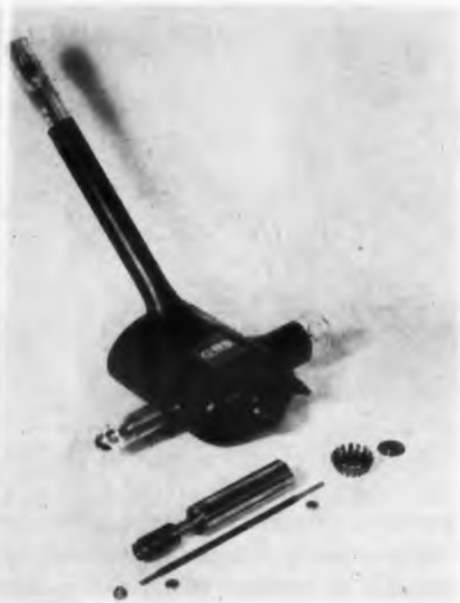
Line-scan tube on which Photoscan system is based has a phosphor-coated anode that rotates at 1,600 rpm to provide a high-density flying spot for scanning of film. Anode, shown disassembled in foreground, has a motor rotor on its shaft.
