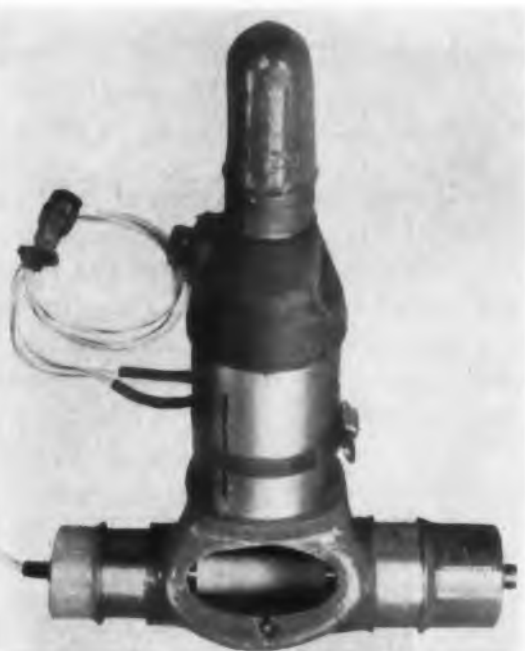
Encapsulated line-scan tube is a production version for military environments.
