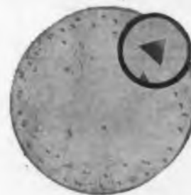
Dislocation density. Knapic silicon monocrystals grown by a modified Czochralski technique: Crystal diameter to \frac{1}{2} "—None; \frac{3}{8} " to \frac{1}{4} "—less than 10 per sq. cm.; \frac{1}{4} " to 1\frac{1}{4} "—less than 100 per sq. cm.; 1\frac{1}{2} " to 2"—less than 1000 per sq. cm.
