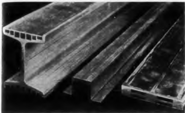
Fig. 2. Rigidamp structural members. Viscoelastic medium between cell and insert absorbs dynamic energy when beams flex under impressed vibration.
