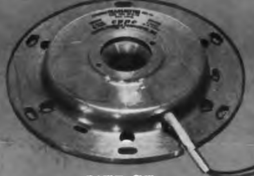
SIZE 37 Accuracy: \pm 4' max. error.
