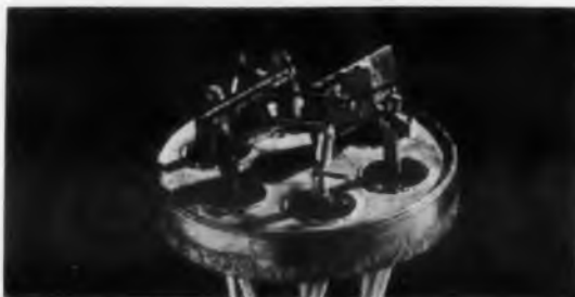
The multi-headed transistor is a combination of any type or types of transistors now in use.
