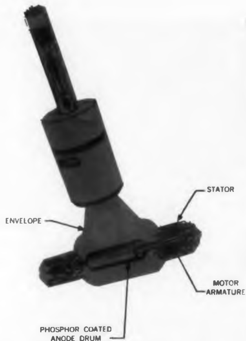
Line-scan tube on which Photoscan system is based has a phosphor-coated anode that rotates at 1,600 rpm to provide a high-density flying spot for scanning of film. Anode, shown disassembled in foreground, has a motor rotor on its shaft.
