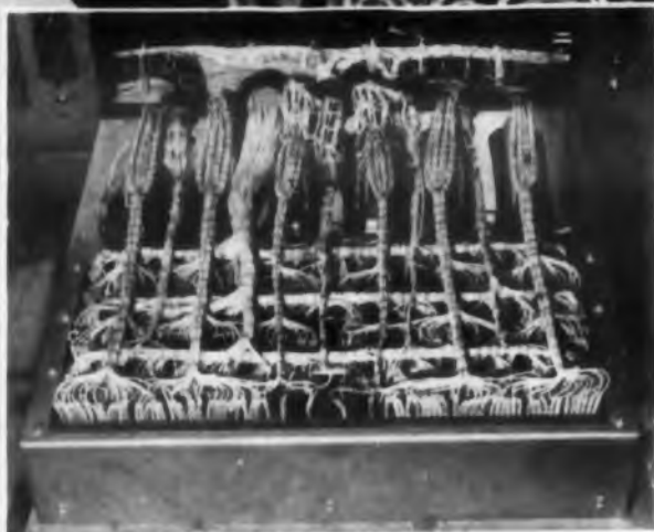
View of a portion of a SAGE Display Console. Nearly a mile of wire and cable is used in each of these consoles. Tensolite supplies wire and cable to meet the specified requirements.
