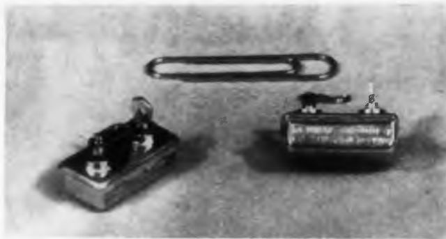
Fig. 3. These tiny Fenwal Thermostats can control to within 1/2 deg C.
