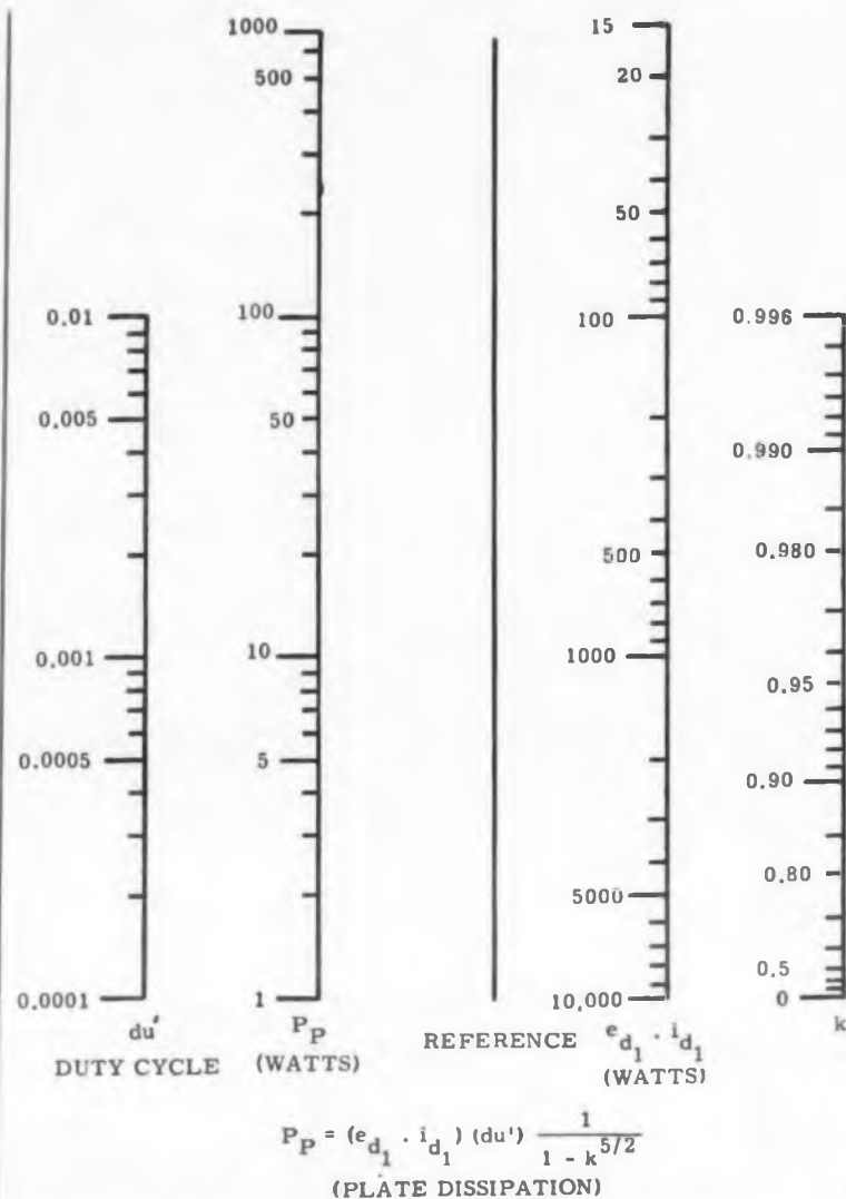
Fig. 5. Use this nomograph to determine plate dissipation.
