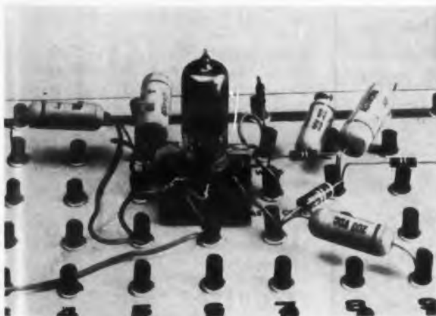
Fig. 2. The terminal cells are shown supporting different wires on a breadboard layout. Wires are easily inserted with no soldering or screw-turning required.
