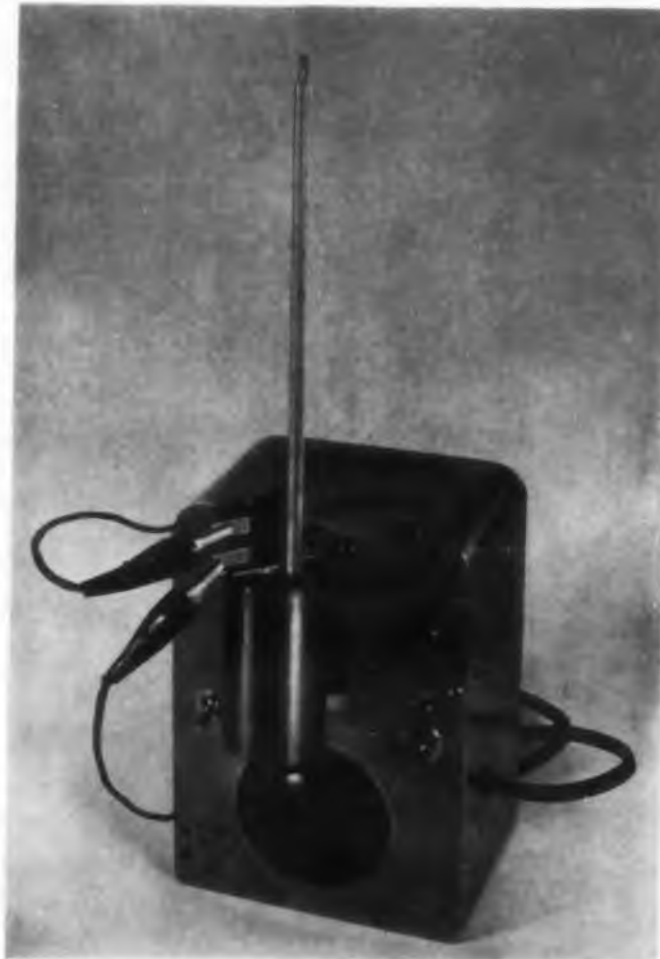
Fig. 1a. The control knob of this thermostat tester is rather close to the heat unit, an undesirable operation factor.
