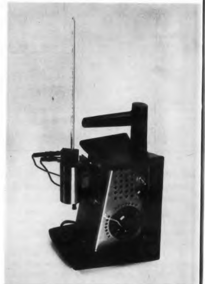
Fig. 1b. By placing the control to the side, operator safety is achieved. An opening in the self-contained handle provides storage for the thermometer during transit.
