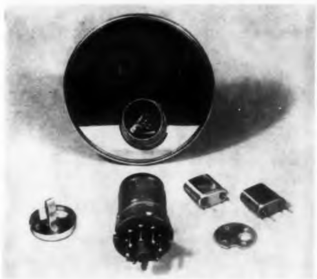
Fig. 5. If the control cannot be placed close to the crystal and heater, it should be mounted on a large mass in the oven. The mirror shows the control mounted on the base of the oven where it will respond quickly to cooling tendencies.
