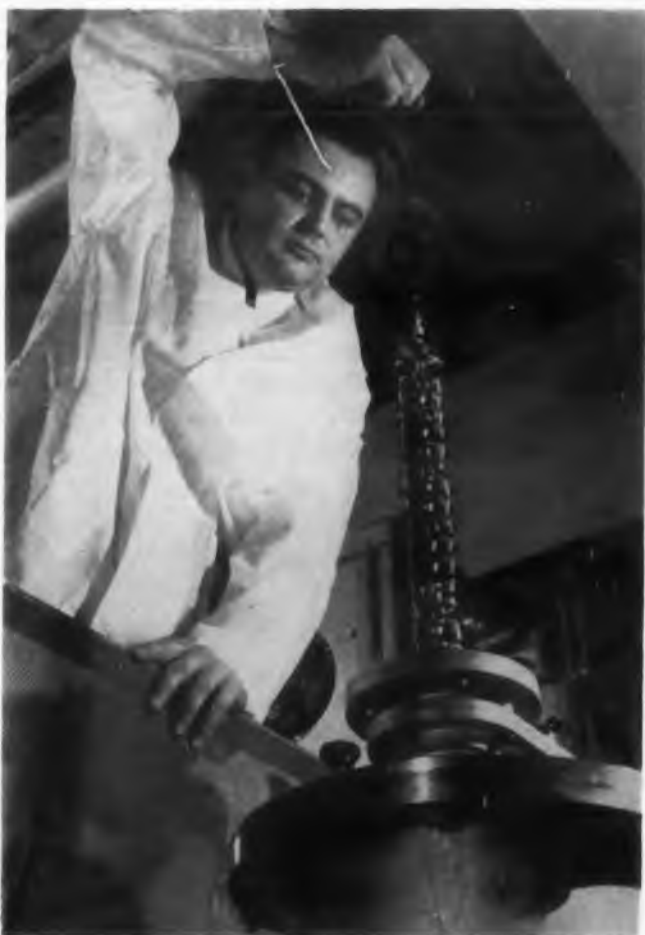
Fig. 2. A "shish-kebab" containing approximately 100 nuvistors is lowered into an exhaust and sealing machine.
