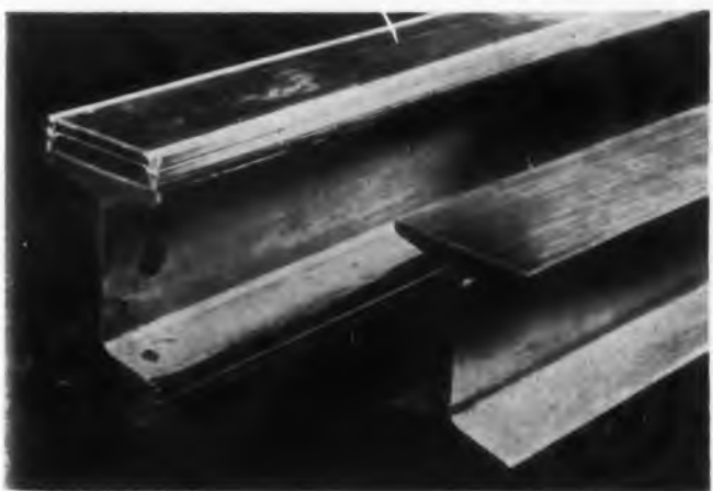
Fig. 3. Strip dampers on beams on left offer means of "fixing" the resonant response of conventionally designed structures.
