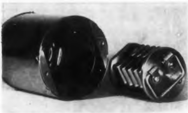
Fig. 2. Brass chassis provides thermal inertia to control crystal temperature closely.
