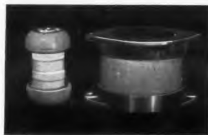
A size reduction is dramatically illustrated when comparing an HPD rated at 25 amps with a conventional CM85 mica capacitor.
