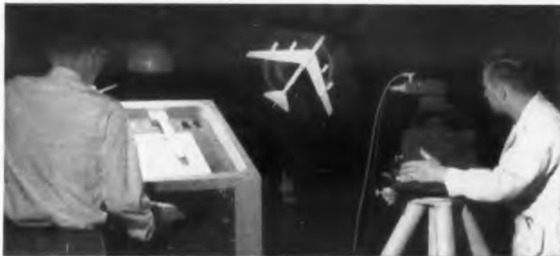
DARK TUNNEL. View in 100-foot dark tunnel, part of extensive Boeing infrared research and development facilities. Boeing investigations include use of infrared, visible and ultra-violet techniques for use in communication, navigation, detection and guidance at altitudes above tropopause. IR systems, inertial navigation, electrical power systems for satellites, shockwave radiation and refraction and iridome heating are other areas of assignments open at Boeing.
