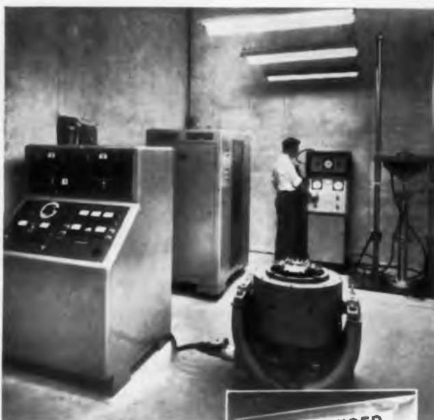
Vibration, acceleration and shock tests for qualification approval purposes are made in this room.
