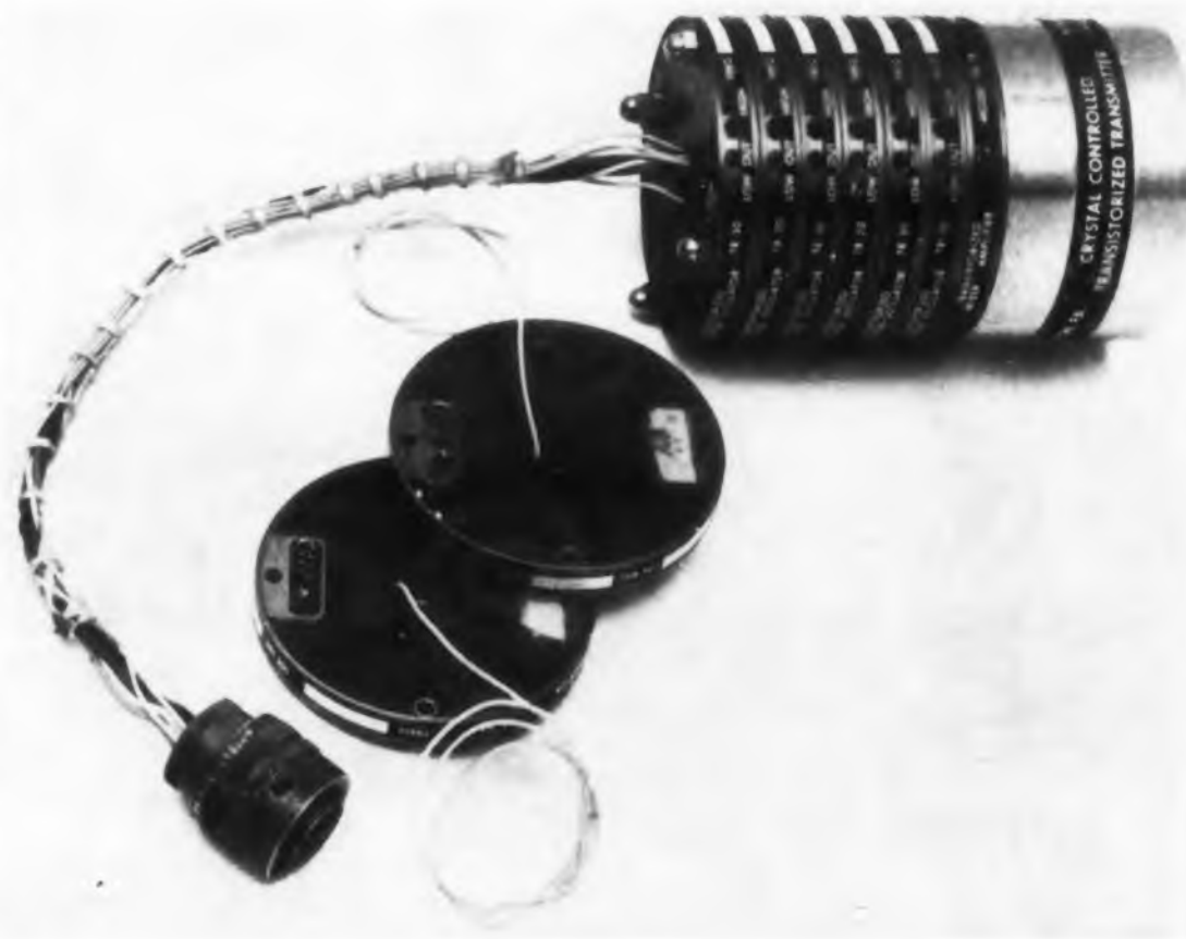
Complete cylindrical telemetry system, upper right, is made up of the wafer modules shown. Subcarrier oscillators can be readily added or removed as desired.
