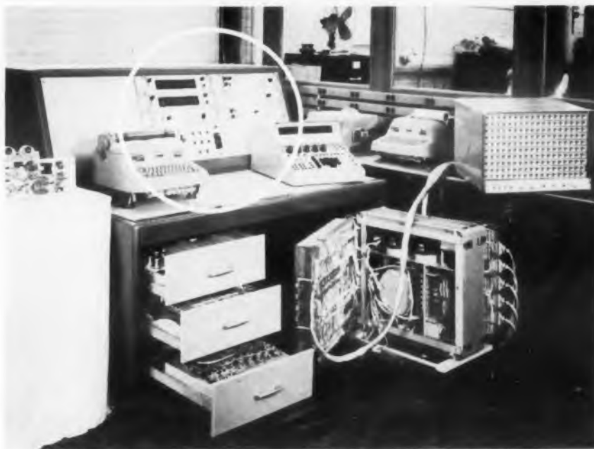
Multi-purpose digital measuring and recording system measures AC volts, DC volts, ohms and ratios. Prints and punches information for immediate reading by the operator and subsequent data reduction.
