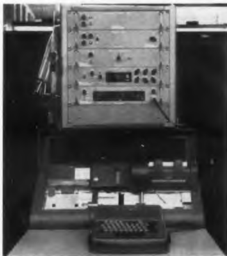
Resistor scanning unit — Scans large numbers of resistors, measures values from 0.1% to 0.01% and records the information on punched cards. Operation is automatic and operates entirely unattended.
