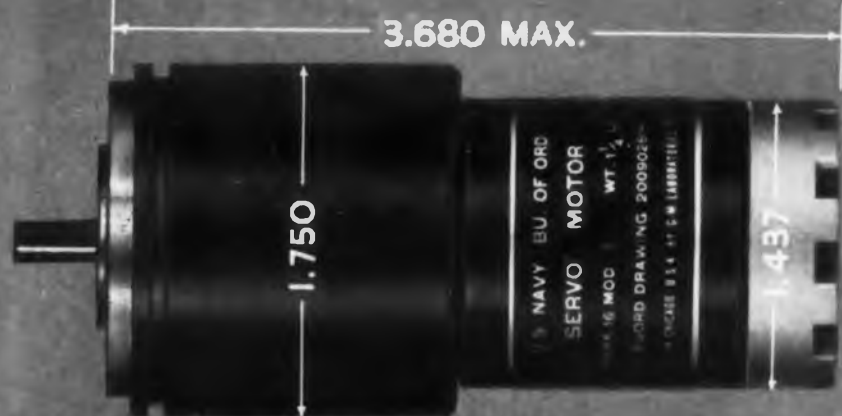
BuOrd Mark 16 Mod 3 SERVO MOTOR Tachometer Generator for transistor operation 115 volts fixed phase 36/18 volts control phase, 4500 RPM (min).
