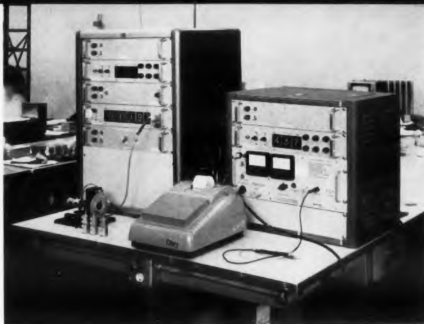
Resistance measuring system — Used as a secondary standard to make accurate, resistance measurements required for checking linearity of multi-turn potentiometers.
