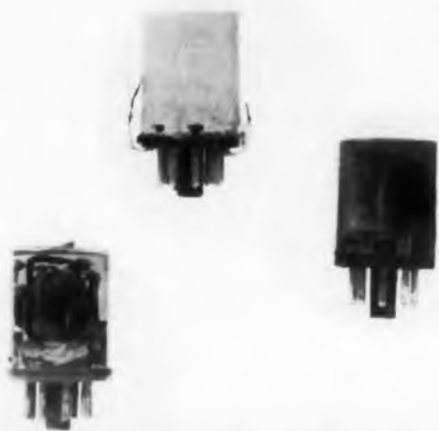
Fig. 1. How the 10 mc oscillator assembly was imbedded. Sample second from right shows thermocouple leads.
