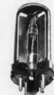
HG Relay cutaway to show magnetic switch surrounded by operating coil and encased in a metal housing.
