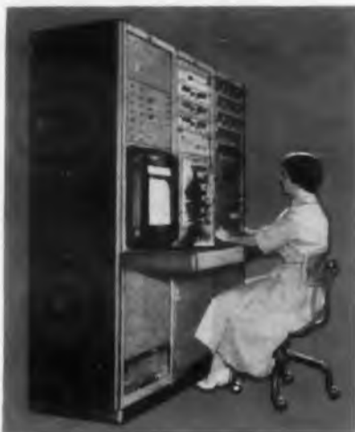
EMCOR Cabinets house "SMART" — The Sequential Mechanism for Automatic Recording and Testing designed and built by Texas Instruments Incorporated, Dallas, Texas. The unit evaluates transistors automatically and economically with consistent accuracy.
