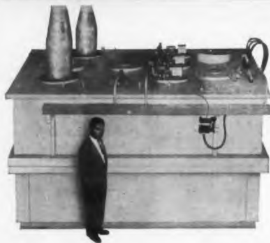
120 KV 2 A DC power supply installed at Eitel-McCullough, Inc. for klystron testing
