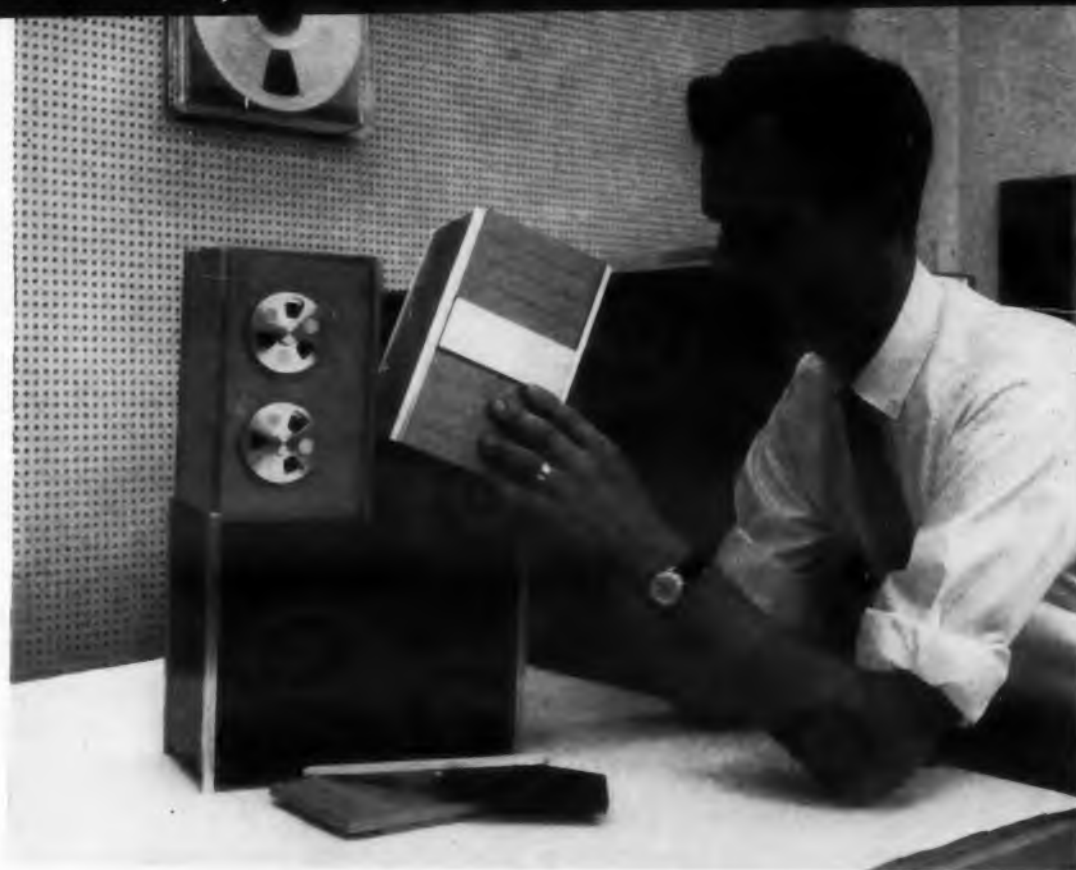
This quarter-scale model was made up to determine ease of interchangeability of various sections of the machine.
