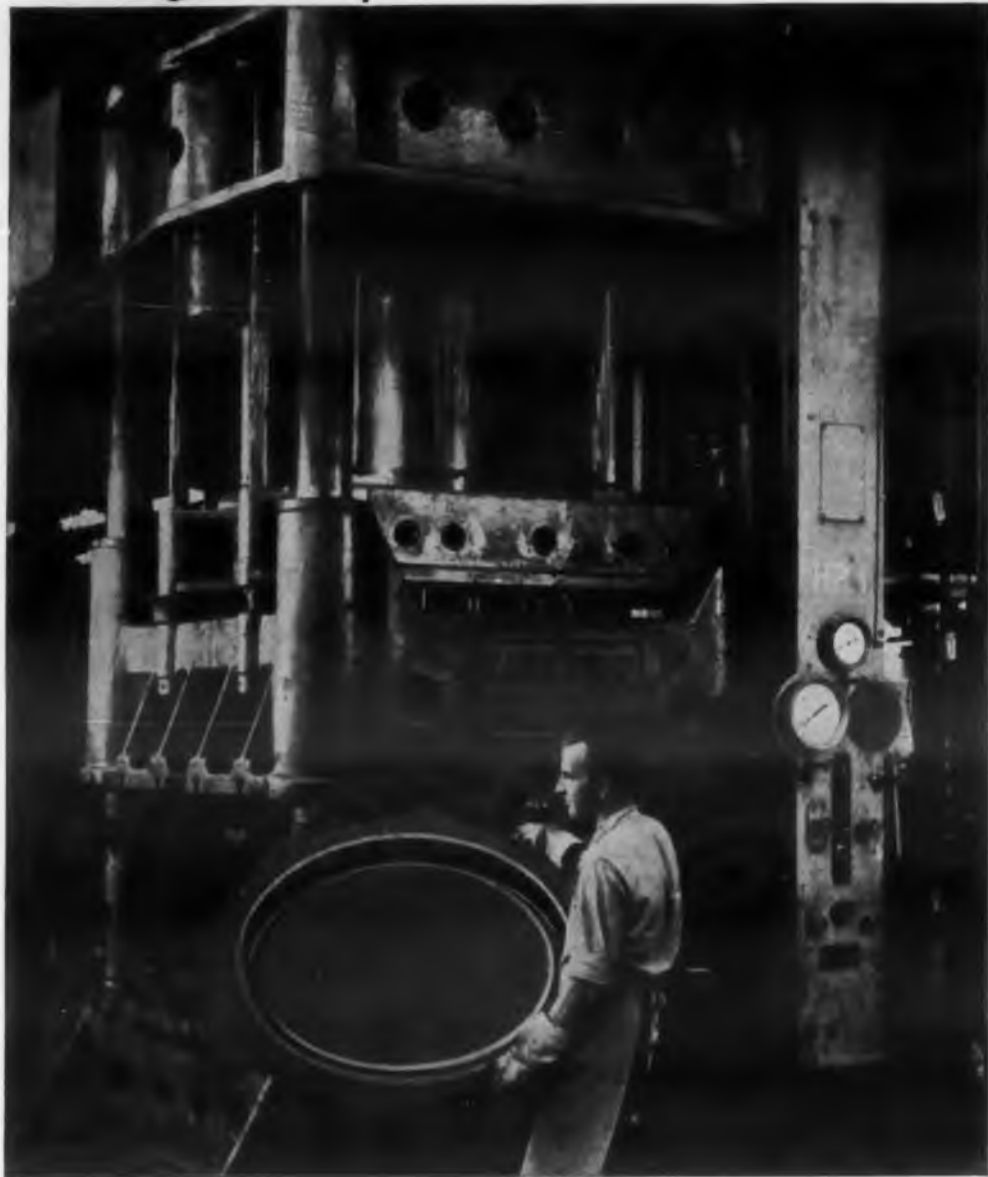
400-TON PRESS draws end pieces of magnesium transmitter housing for missile ground support electronic system. Heated dies make possible one step draws.
