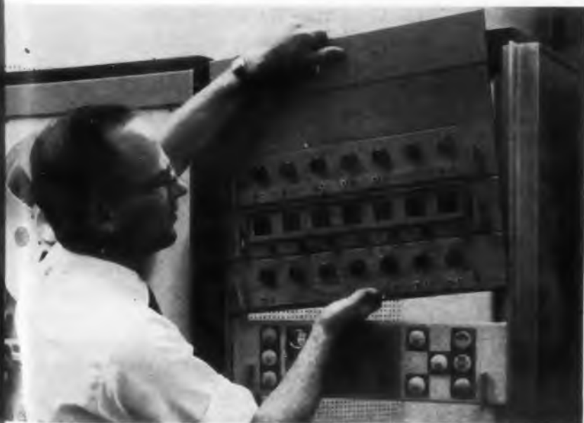
Industrial designer fits dummy of oscilloscope portion of a tape recorder into a full-scale model.
