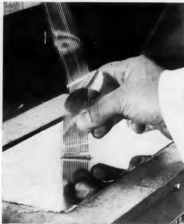
Fig. 5. End-stripped cables can be either hand soldered or dipped in solder, as shown.
