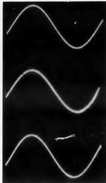
Fig. 11. No change in exposure is seen as signal frequency is increased from 30 kc to 300 kc to 3 mc. Sweep rate was adjusted to maintain 1/4 cycle/in. on the crt. X-gain was held constant. Camera set at f/5.6 , 1/50 .
