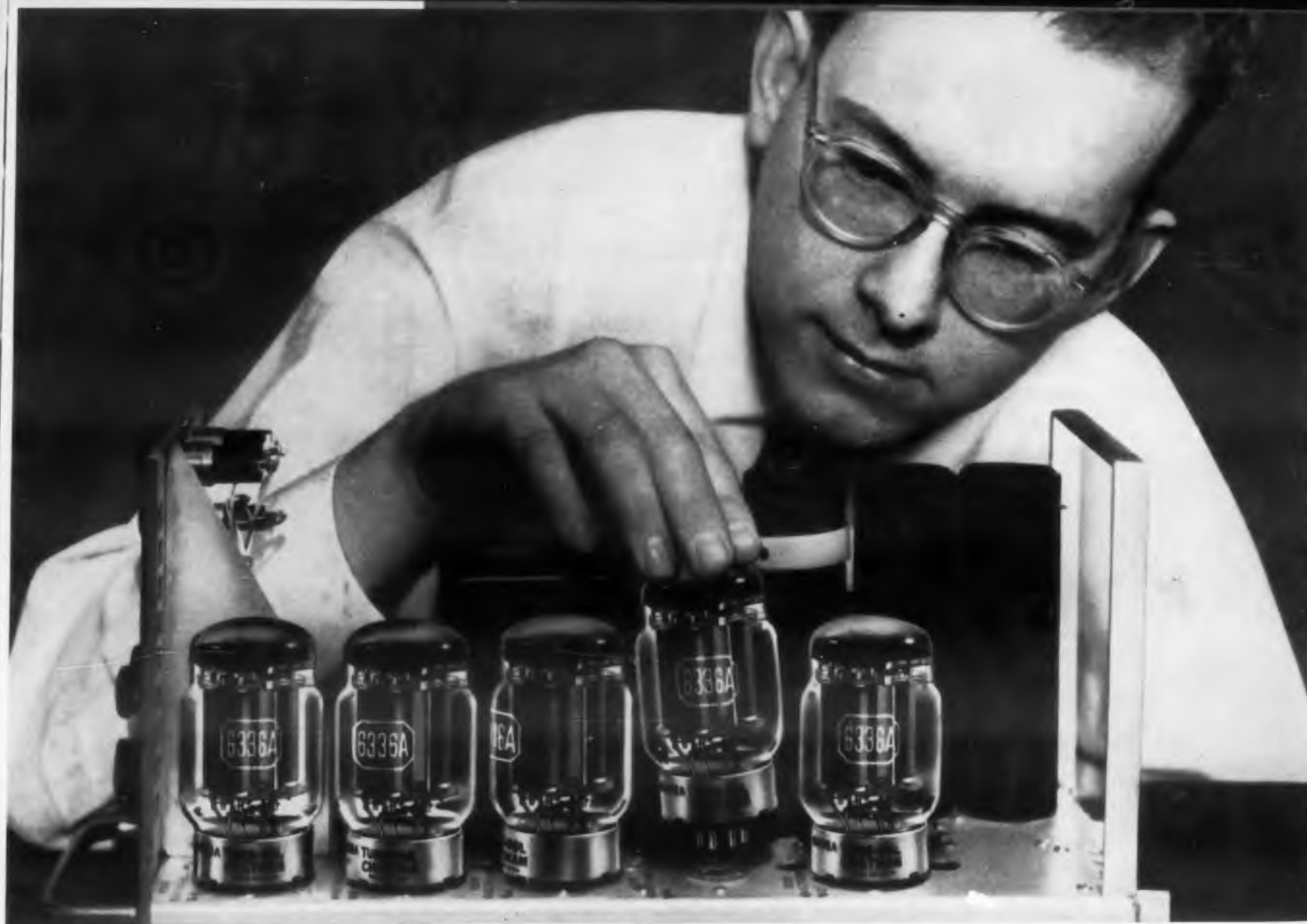
Engineer A. M. Darbie installs a Tung-Sol/Chatham 6336A twin power triode in a Harrison Labs 2B regulator, part of a 200B high current power supply. Superior power handling ability of the 6336A lets Harrison Labs offer the regulator with a 5-tube complement in addition to a 7-tube model.
