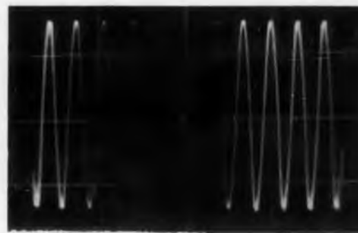
Fig. 7. Part of left trace was lost due to shutter being open long enough (1/10 sec.) for only two to three sweeps. Keeping the shutter open longer (1/2 sec.) for right trace yielded uniform trace intensity.
