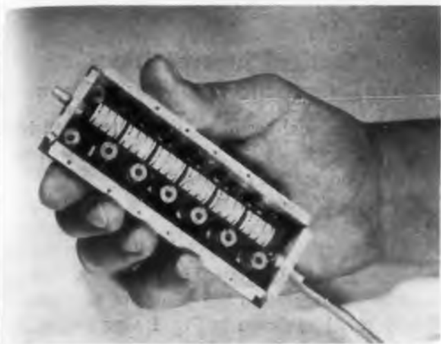
Fig. 2. Six-stage if amplifier using ceramic tubes squeezes neatly into 2½ cu in.
