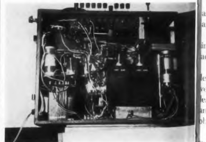
Fig. 2. Inside view of the dual-beam scope. The entire instrument is in a case 5 x 13 x 16 in.
