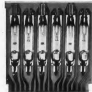
HG6F Relay printed circuit panel showing six in-line mercury-wetted contact switches mounted in minimum space.
