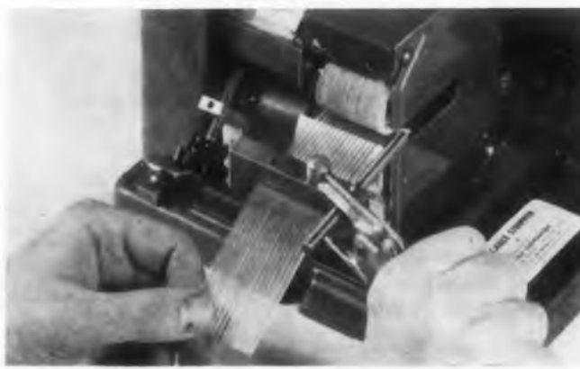
Fig. 2. For production, stripping machines can be used to remove insulation from as many as 300 conductor ends in a minute.
