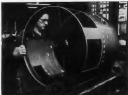
"WRAPPER", or shell of housing is roll formed of magnesium sheet.
