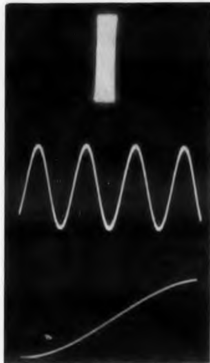
Fig. 10. Only the X-gain was changed for these three pictures. A 30 kc trace was expanded from 16 cycles/in. on the crt. Camera set at f/5.6 , 1/50 .
