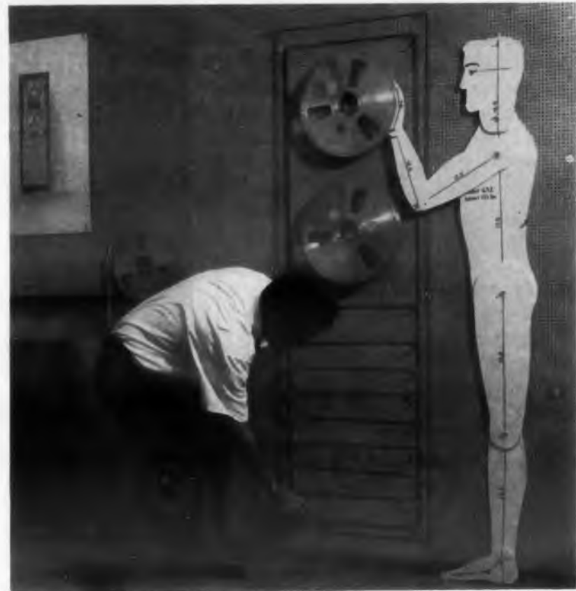
A mock-up is made using yarn to outline the recorder rack. "Average man," right, assists in determining most comfortable operating positions.
