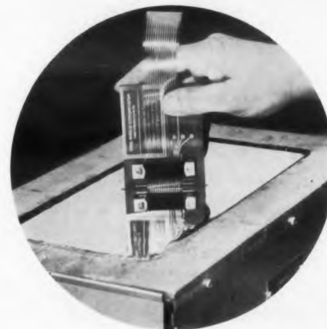
Fig. 7. (above) Dip soldering can be used to attach flat cable to a printed wiring board.
