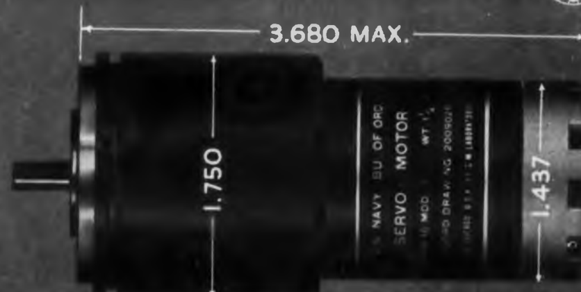
BuOrd Mark 16 Mod 3 SERVO MOTOR Tachometer Generator for transistor operation 115 volts fixed phase 30/18 volts control phase, 4500 RPM (min)
