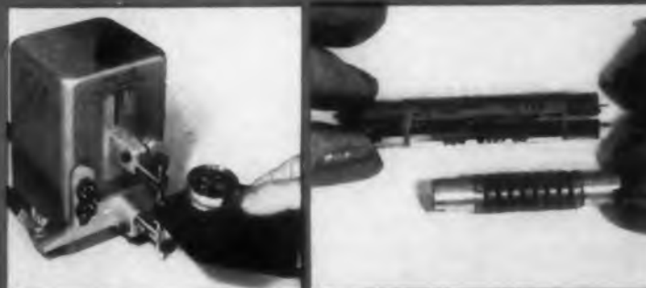
Weldmatic pressure gage reads firing force...calibrated from 0 to 50 lbs., insures exact weld pressures from job to job. (Right) Welded filter cartridge and completed miniaturized Collins filter.
