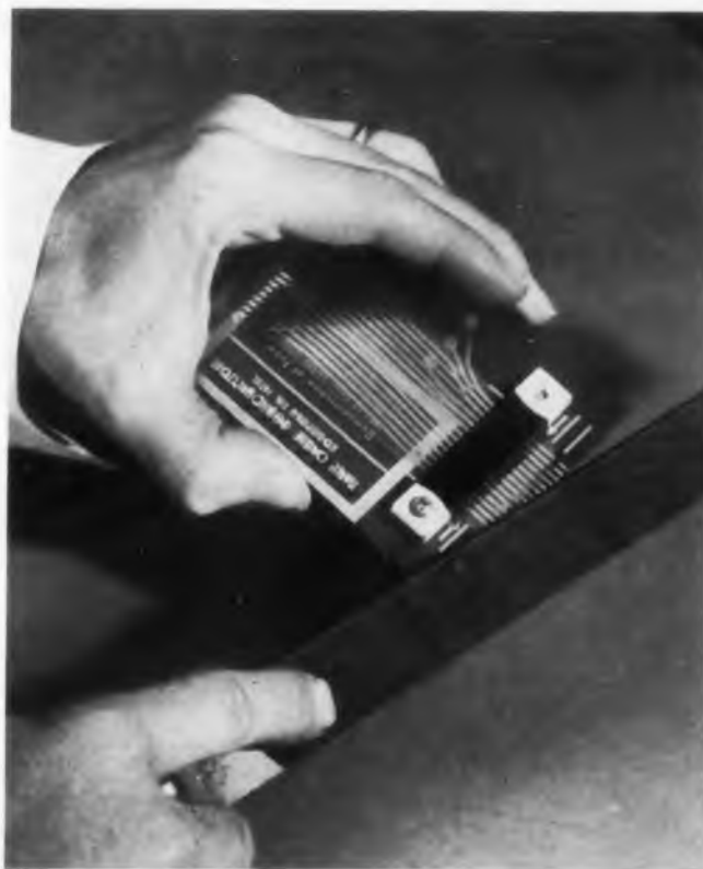
Fig. 8. Excess cable is trimmed off with one pass of a file
