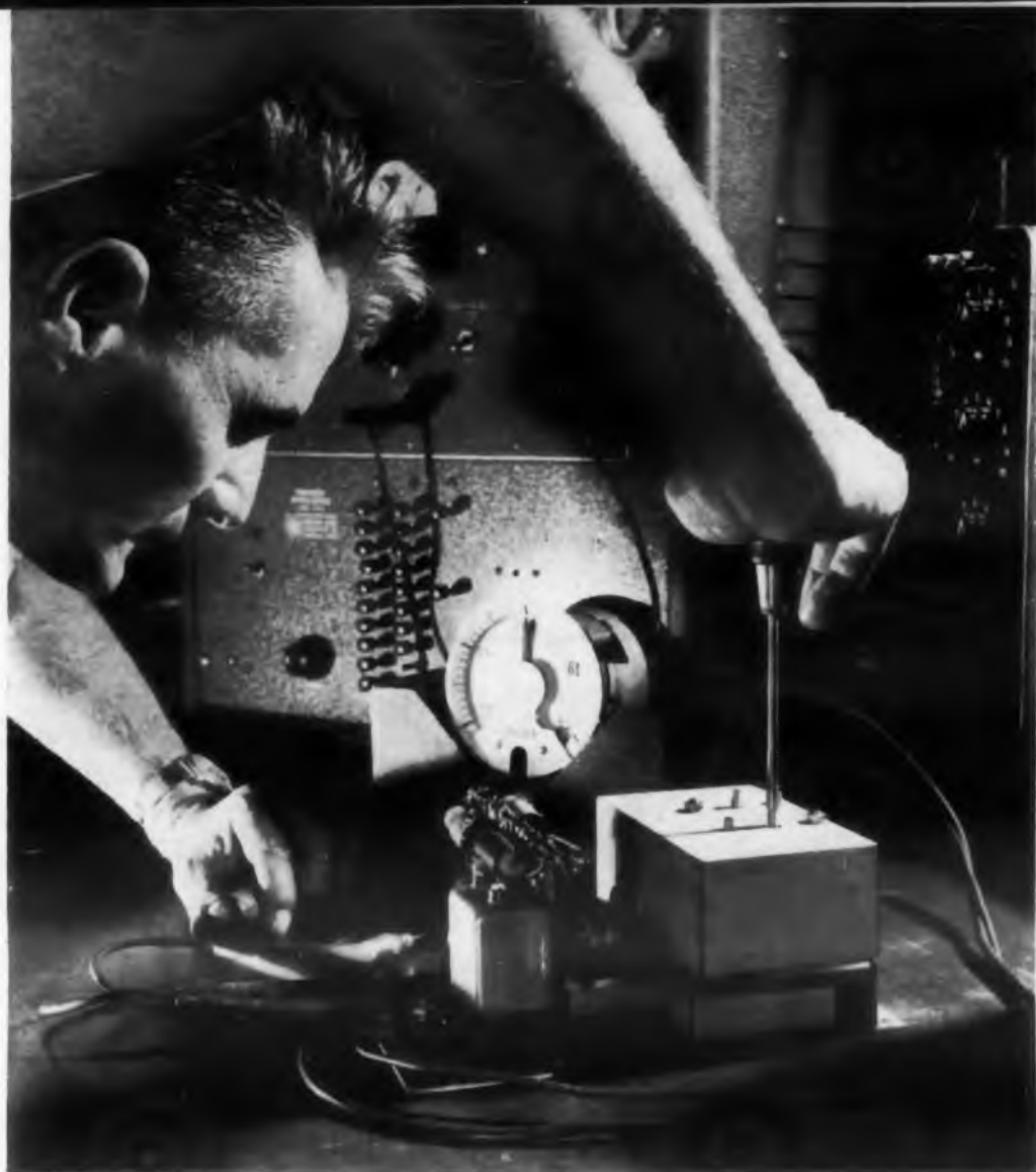
Fig. 3. Frequency meter being adjusted for use with a dc indicating voltmeter which will be calibrated to read frequency in cps.
