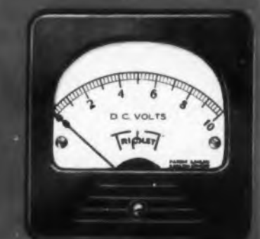
Rectangular Flush Mounting (1 1/2") Model DC 227-T, AC 237-S, RF 247-T, Dyn. 361-A
