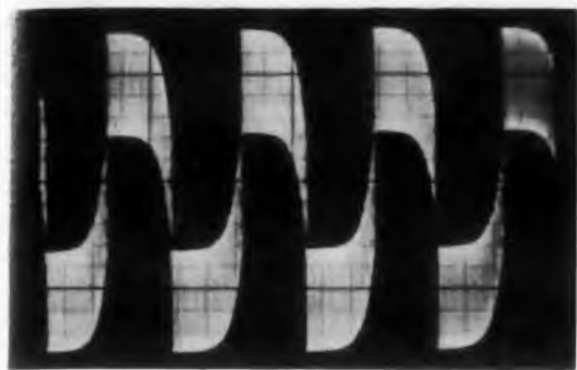
Fig. 6. Left signal has slow modulation, gave blurred record when exposed for 1/2 sec. Increase of shutter speed to 1/50 gave well-defined right trace. Aperture setting changed from f/16 to f/4.
