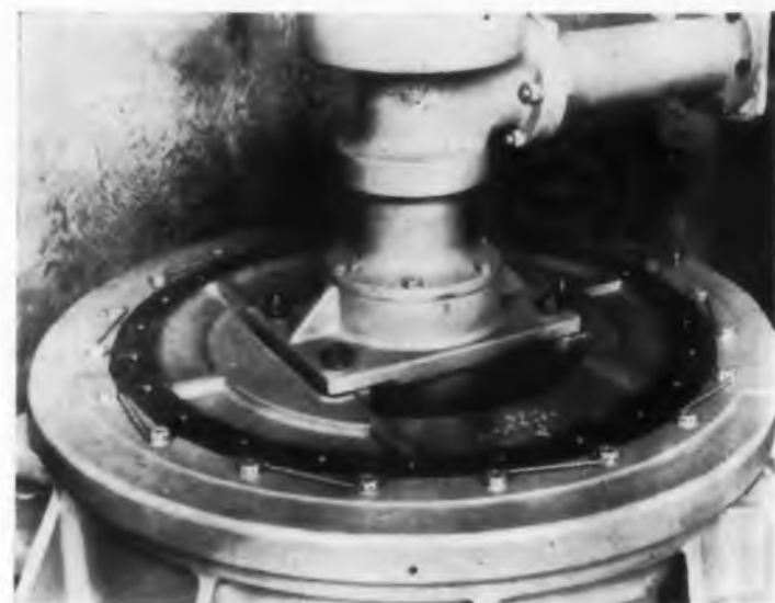
Fig. 3. Rotary joint is changed easily by removing the four bolts which attach it to the antenna turntable flange.
