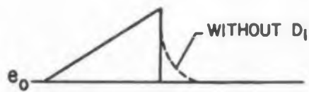
Fig. 2. Faster fall time results when the timing capacitor discharges toward a negative voltage and the diode clamps at ground.
