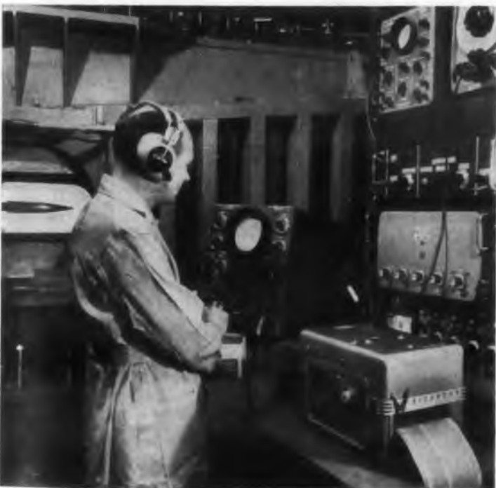
Z. A. Woodard, Jr., ARO, Incorporated, instrument technician, operates the Visicorder in the measurement of aerodynamic damping coefficients.
