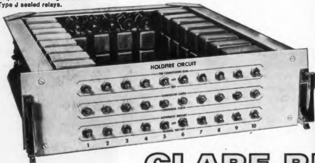
View of control rack of Model III Sequencer showing 56 CLARE Type J sealed relays.
