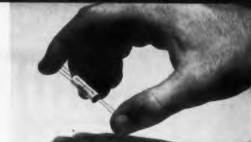
Unimite is world's smallest 1-amp relay
