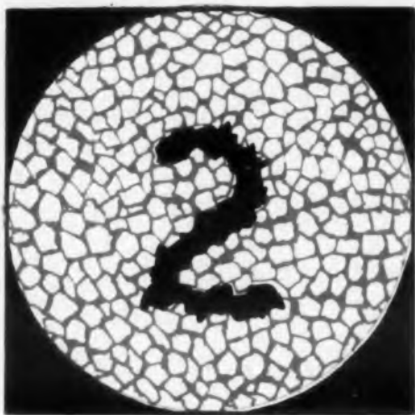
How an image would look through a lens on the end of a glass-fiber bundle.
