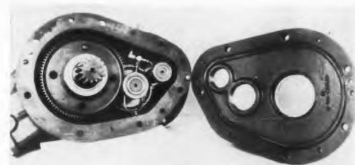
Fig. 2. Basic simplicity of modules, illustrated by this compact, weatherproof gearbox, eliminates the large and difficult castings and intricate component design required to adapt conventional pedestals for a new antenna system.
