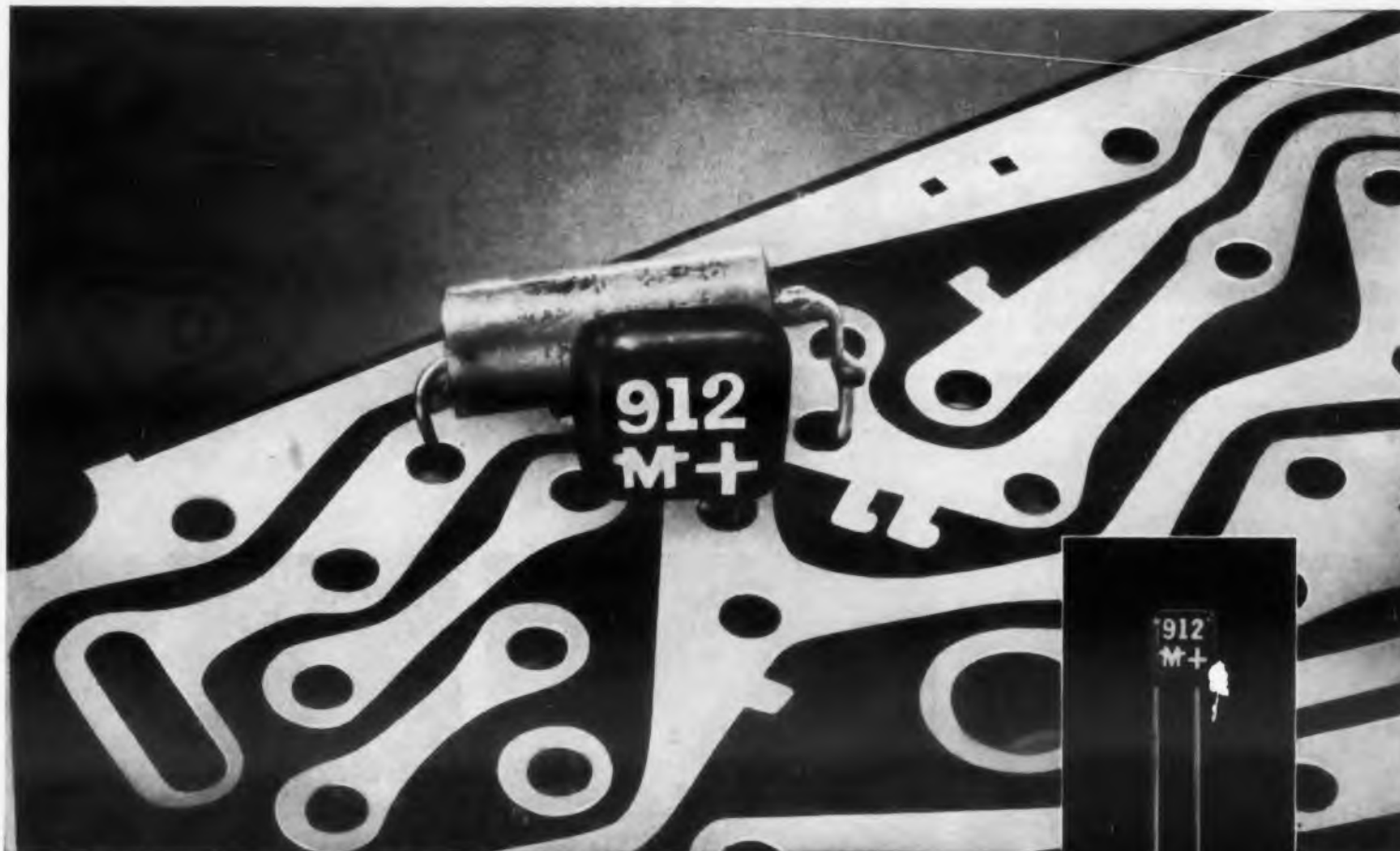
Comparison of area required to mount new Mallory TAM capacitor versus metal cased unit of same rating.
