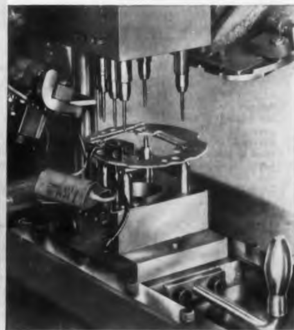
Simultaneous multiple eyeletting from either or both sides of machine. Typical six eyelet application illustrated. 50 years' experience is your assurance of complete dependability.
