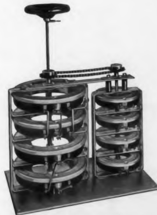
Two groups of four Ohmite taper-wound rheostats mounted in tandem, controlled by a single knob through a chain drive.
