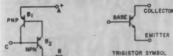
Fig. 2. Analogy between two transistors, a pnp and an npn, and a single Trigistor. Trigistor's three leads correspond to terminals A, B, and C of the two-transistor circuit.
