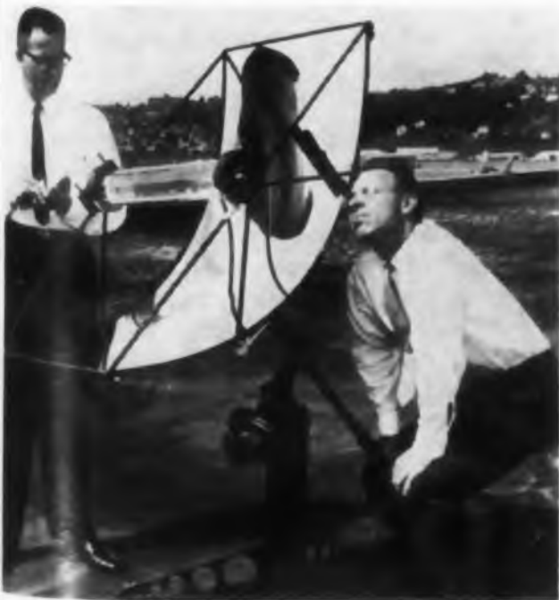
Working model of solar-powered thermoelectric generator can produce 2.5 w according to its designers, Niles F. Shuh, of Westinghouse, (left), and Ralph Talbot, of Boeing.
