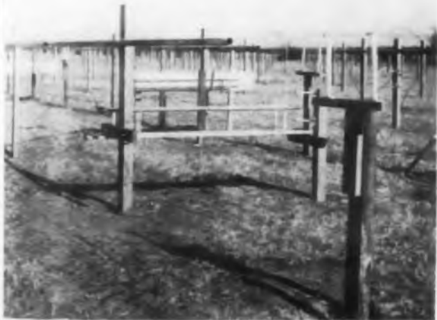
These dipoles are part of a 4-acre array of 1024 dipoles mounted 4.5 feet above a ground reflecting screen to study vertical incidence scatter from the atmosphere.
