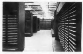
Heart of the SAGE System is the 275 ton IBM computer, one of the world's largest and most reliable. Shown here are some of the computer frames containing pluggable electronic units that perform the data processing involved in solving air defense problems.
