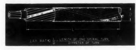
Fig. 1. Lay ratio defined and illustrated.
