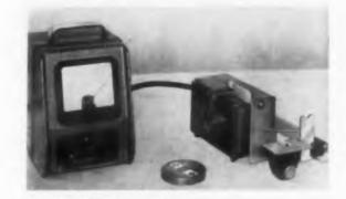
Model 100 Talysurf is a portable, semiautomatic instrument for production inspection and precision testing of surface finish. The assembly includes work table, pick-up, stylus, support, and motorized drive. It can carry small work in universal work-holding fixtures or be fitted with quick loading production tooling. The same unit, inverted, can be used to check large flat or cylindrical work.
