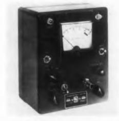
The model 219 A transistor tester permits the measurement of transistor beta parameters with transistors in the circuit. Beta and collector leakage current parameters may be measured with the transistors removed from the circuit. The unit is packaged in a compact carrying case and operates from either a self-contained battery supply or 110 v, 50 to 60 cps.
