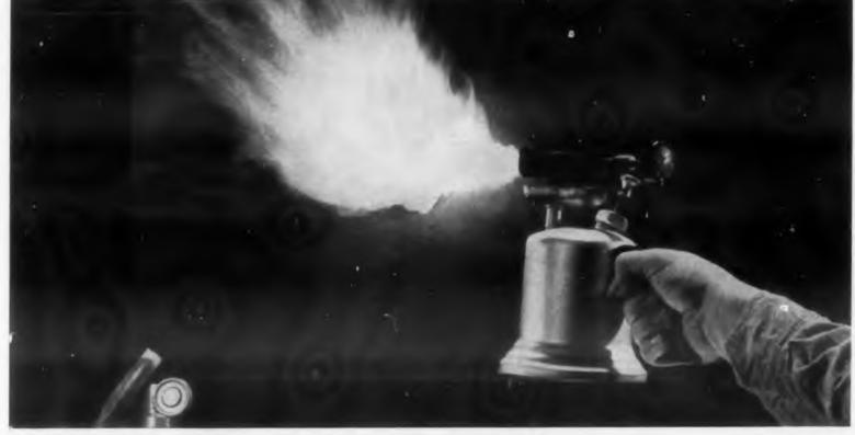
Sheet of Synthane to which blowtorch is being applied
