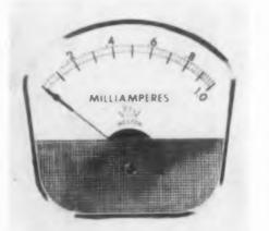
These panel instruments feature the Cormag mechanism for positive shielding from external magnetic fields. Model 1741 is a 4.5 in. dc unit and model 1724 is a 2.5 in. ac unit. Also available are three ac moving iron type instruments capable of obtaining controlled ballistics characteristics.
