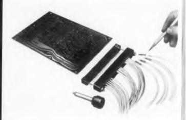
A new addition to the HYFEN® line a printed circuit connector, has been announced by the Omaton Division of the Burndy Corp.
