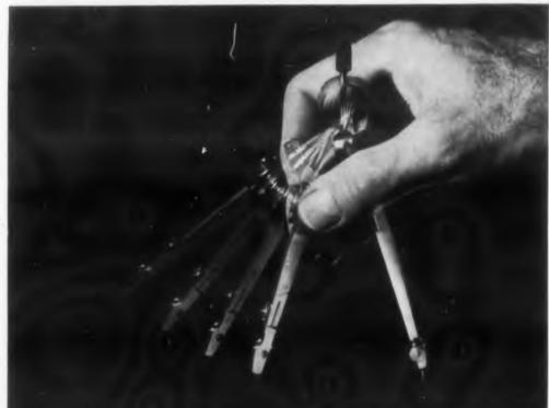
expand automatically. Stop approximately where you want, and make precise adjustments with a micrometer screw. To go from large to small, simply squeeze the legs of the compass together, then adjust precisely.
