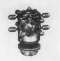
The model RB4 transfer relay is designed for high voltage applications involving antenna switching, pulse forming networks, and similar rf and de circuits. The 4pdt unit has a vacuum dielectric, sapphire actuating rods, and removable actuating coils for 26.5 or 115 v de operation. Peak test voltage is 25 kv de or rf and rated operating voltage is 20 kv at 2.5 mc and 10 kv at 16 mc. Contact resistance is under 0.01 ohm and current rating is 13 amp rms at 60 cps and 8 amp at 16 mc.
