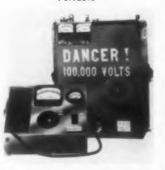
Series VON portable high voltiege de insulation test instruments and power supplies have ranges from 30 kv at 40 ma to 250 kv at 7 ma. All models are sectionalized to provide maximum portability and minimum weight, and supplemental stages may be added to the base power units to increase voltage ratings.
