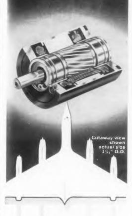
Air-Marine's new S frame motor offers outstanding reliability even at extremes of temperatures and altitude. Two models are available: the Hi-Slip which increases speed with altitude lower densities, and a CONSTANT SPEED, 11,000 rpm or 20,000 rpm.
