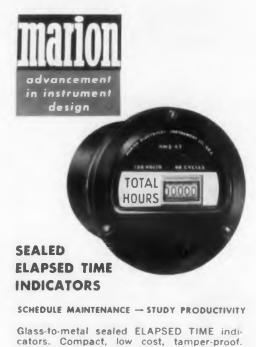
cators. Compact, low cost, tamper-proof. Standard ASA MIL dimensions,  $21_2^{\prime\prime}$  and  $31_2^{\prime\prime}$  sizes. Easy to read standard size counter registers 1/10 hour steps to 9999.9 or hour steps to 99999. Hermetically sealed. Shielded. Starts, operates continuously from  $-55^{\circ}$ C to  $+85^{\circ}$ C. For 110-125 or 220-250 volts 60 cycle A.C. Bulletin on request. Marion Electrical Instrument Co., Manchester, N. H., U. S. A.
