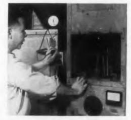
Flame retardant test on Synthane for switchgear application. Heat is supplied by coi' circling the sample. Temperatures up to 1600°-1800°F are measured with optical pyrometer.
