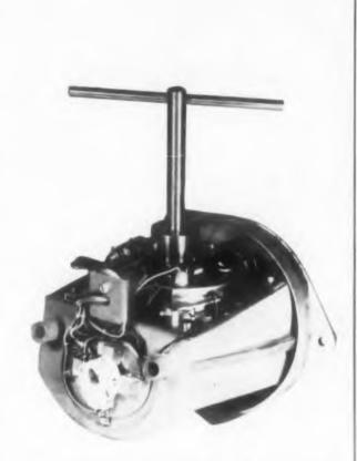
**Fig. 1.** Caging and winding of the gyro is done with a removable key at the factory. The unit is capable of being stored for an indefinite period in this condition.
