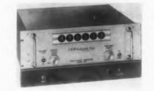
The 1300 series of electronic tachometers and frequency counters includes types for remote indication, for explosion-proof installation, and for dual readout requirements. Time bases available have fixed selectable times of 0.1, 0.5, and 1 sec. The units have an accuracy of  $\pm 1$  count, a display time that is adjustable from 0.1 to 10 sec, and a sensitivity of 50 mv rms. They have an input impedance of 1 meg and automatic or manual reset.
