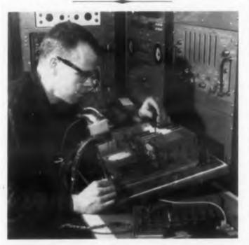
**Missile telemetry package**, designed for Boeing's IM-99 Bomarc by Texas Instruments, Inc., must operate to beyond 145 deg. F. Since the transistors in the package will not work well beyond 145 F, and since the missile's surface temperature, at Cape Canaveral, may reach 160 F, cooling was required.
