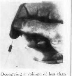
0.0066 cu in., the Wee-Ductor rf choke coil covers a full range of inductances from 0.1 to 1000 µh and has a high current rating at 125 C. It consists of a high permeability ferrite sleeve and core sealed in epoxy resin for moisture resistance per MIL-C-15305A. The unit is 0.15 in. in diameter and 0.375 in. long.
