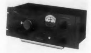
Current as low as 10<sup>17</sup> amp, and voltages as low as 0.02 my can be measured with the Cary Model 32 electrometer. It also measures C14 activity to 5 x 10-15 curies per mg BaCO<sub>3</sub>, and H<sup>3</sup> activity as low as 10<sup>-10</sup> curies per mg H<sup>3</sup>. The unit accommodates ionization chambers from 50 to 1500 ml, as well as solid and liquid sample accessories. Ranges: 10, 100, 1000 mv, 10 v. Accuracy of the unit is  $\pm 0.25\%$ . It consumes 50 w at 115 v, 60 cps.
