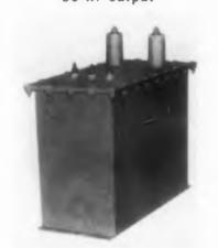
Designated Model PS-30T, this 30 kv, full-wave voltage-doubler power supply operates on 117 v, 60 400 cps. The unit delivers 1 ma continuous and 1.75 ma peak current. Ripple is 1.5% at 1 ma and regulation is approximately 7% from moload to full load. It has replaceable 1B3 rectifier tubes and plastic dielectric capacitors. Dimensions of the case are 5-1/4 x 11-3/8 x 9-1/2 mol and the unit has oil-tight solderse il terminals.
