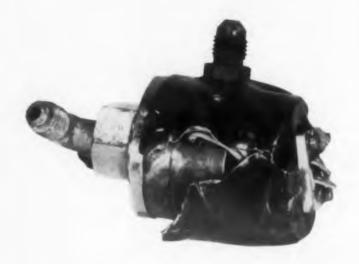
PACE Model P1 transducers were used by a missile component manufacturer to measure pressure during a centrifuge test. The transducer shown above broke loose, and was repeatedly battered against a concrete wall until the centrifuge stopped.
