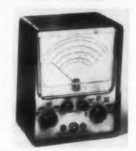
The VT-10 VTVM has an edgelighted 6-in. meter for accurate reading. Sensitivity of the unit's movement is 400 µa, with 2% accuracy. For measurement stability 1% precision resistors are throughout the range switch. The unit has 7 ac (rms) and de ranges, 0 to 1500 v. Also 7 ac peak-to-peak ranges, 0 to 2000 v. Other ranges include resistance, 0 to 1000 megohms, and db.
