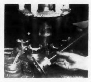
Aircraft gyro electrodes use epoxy resins to support and encapsulate a silver ring inside an index ring. Minneapolis-Honeywell Regulator Co. selected Bakelite epoxy for this job for its high strength and for matching the temperature coefficient of expansion of the metals over a range from -65 to 165 F.
