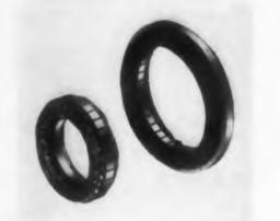
Available in size 20 and 27, these pancake synchros and resolvers feature accuracies down to 5 min and are made for instruments such as inertial guidance systems. Their electrical properties are designed to meet specific applications or to match standard components for accuracy, voltage gradient, and impedances. They may be obtained with integral flanges and hubs.
