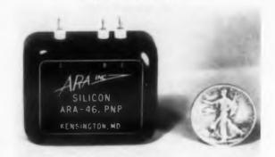
The ARA-46P silicon composite pnp transistor is thermally compensated to operate at temperatures up to 200 C. It has the general characteristics of a small signal transistor at the input and that of a power transistor at the output. Operating specifications are: collector voltage, 40 v; collector current, 3 amp; power dissipation at 25 C, 35 to 50 w; power dissipation at 150 C. 2 to 5 w; current gain, 10,000; input impedance. 2000 ohms; output impedance, 500 ohms.
