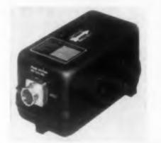
Flexible design of the series 1080 gyros allows the unit to be made into a directional gyro or a free gyro as well as a vertical gyro. Weighing a maximum of 4.75 lb, the unit's maximum dimensions are **3.7/8 x 3.7/8 x 6 in**. Standard extitation of the gyro motor is 115 v, 400 cps, 3 phase. Optional excitation: **26** v, 400 cps, 3 phase; 115 v or **208 v**, 400 cps, 3 phase; 4 wire. Standard pickoff is 115 v, 400 cps, 1 phase, with optional rated at 26 v, 400 cps, 1 phase.
