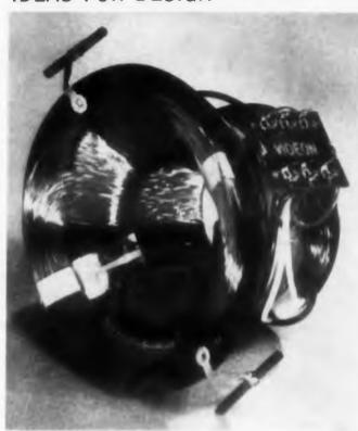
Standard horizontal deflection coils and toroidal vertical deflection coils are wound on a ferrite wedgeshaped ring in this TV yoke made by the Videon Company in France.
