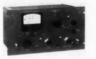
Designed primarily for telemetering instrunentation, this instrument measures: the dropint characteristics in a magnetic tape recording over a range of operating frequencies from 7.5 o 80 ke; a dropout amplitude range from 15 to 55%; and a dropout width range from 38 to 360 usec. For each dropout detected with respect to a predetermined amplitude and width, a 70 v positive going, rectangular pulse is emitted. It measures dropouts in accordance with Mil-T-21029 (Ships).
