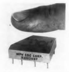
Model SR-104 is a one-core-per-binary-bit uni with a 5 kc information rate and a 10 to 1 signal to noise ratio. Its operating temperature range is -55 to +125 C. A 14 µsec, 22 v output pulse is obtained by applying a 10 µsec, 7 ma input pulse and subsequently an 8 µsec, 300 ma shift pulse. Encapsulated in an epoxy compound, the unit occupies a total volume of 0.2 cu in.
