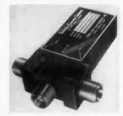
Type SP2T is a 0.7 lb rf coaxial lobing switch with a range of 100 to 10,000 mc, a maximum vswr of 1.2 to 1, and an isolation rating of 50 db down. Make before break or break before make switching is available. The unit is hermetically sealed, glass to metal, and has a minimum life of 1000 hr. Several models are available with a choice of type N, HN, or SC rf connectors.
