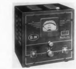
The Matchmaster is an instrument which tests transmitters without signals on the air. It consists of a dummy load with a direct reading rf wattmeter and a standing wave ratio bridge. It is useful for measuring the swr in antenna feed lines, the adjustment of radio transmitter power output before going on the air, and many other applications. All components are contained in a cabinet  $6 \ge 8 \ge 8$  in.
