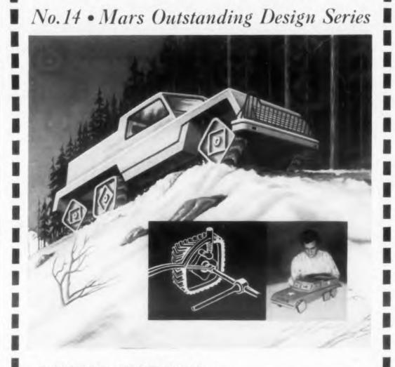
**SQUARE WHEELS?** Yes ... square wheels. Operating by means of a floating axle and cam gear, they take the bumps out of rough terrain and provide more traction. U.S. Patent No. 2786540 has been granted to designer Albert Sfredda of Bethlehem. Pa., for his invention.
