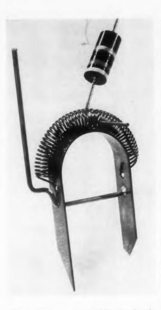
**Fig. 1.** Simple component holder saves breadboarding time.
