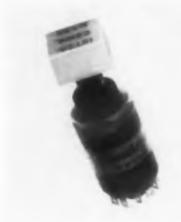
This dpdt double break switch-light combination has an independent 28 v lamp circuit for panel mounting. It is supplied in momentary snap action or push-on push-off snap action with contacts rated at 28 v de, 5 amp, inductive. Operating pressure is approximately 4 lb with 5/32 in. overall travel. The unit has a 5/8 in. mounting thread, a 7/8 in. case diameter, and a 1-3/8 in. length from mounting surface to and including terminals.
