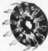
For Printed Circuits: Special lug design for insertion into printed circuit boards.
