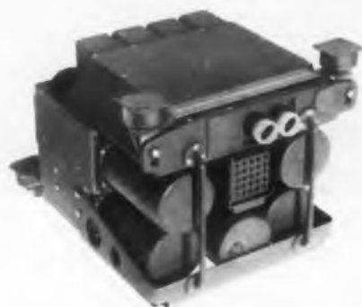
Centralized Air Data Computing System
