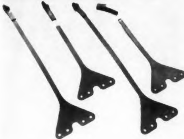
Improved design breaks later in different place (bottom right).
