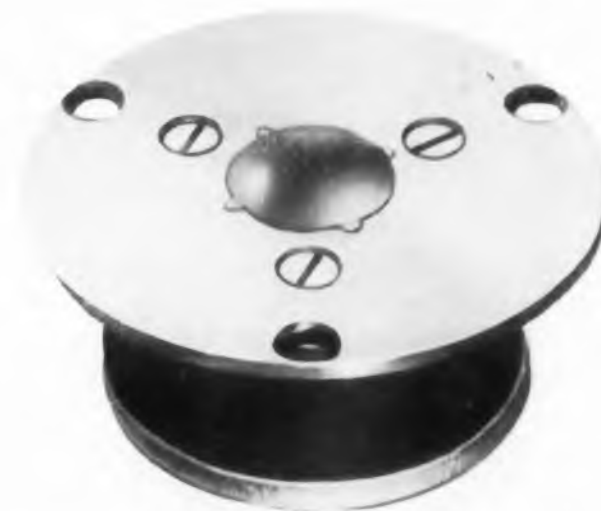
Fig. 1. Synthetic rubber in the gap of Acoustic Research's tweeter holds the self-supporting voice coil in the magnetic gap. The entire moving system (diaphragm, voice-coil, and rubber suspension) weighs slightly more than a gram.
