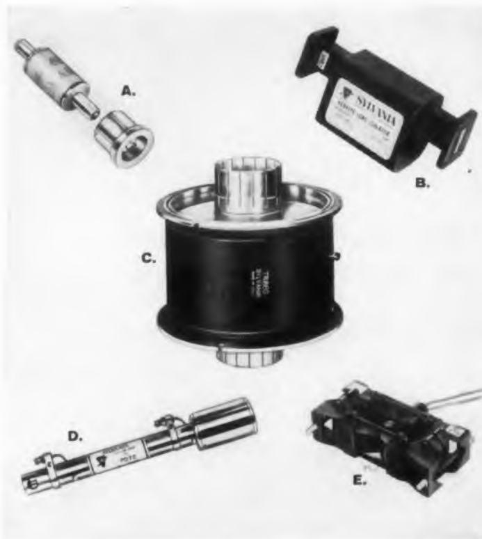
A. Microwave Crystal Diode, B. Ferrite Isolator, C. Coaxial TR Tube, D. Traveling-Wave Tube, E. Ka Band Magnetron.
