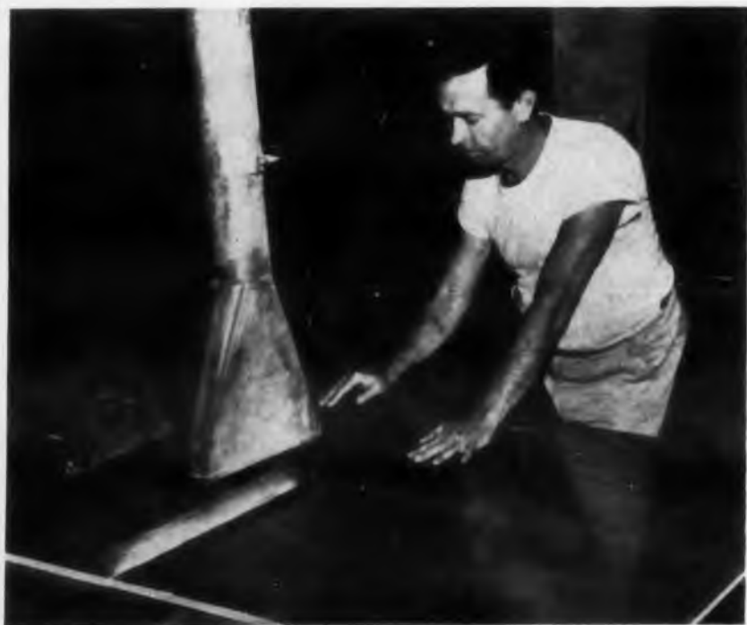
Sawing a full sheet of glass base laminate.
