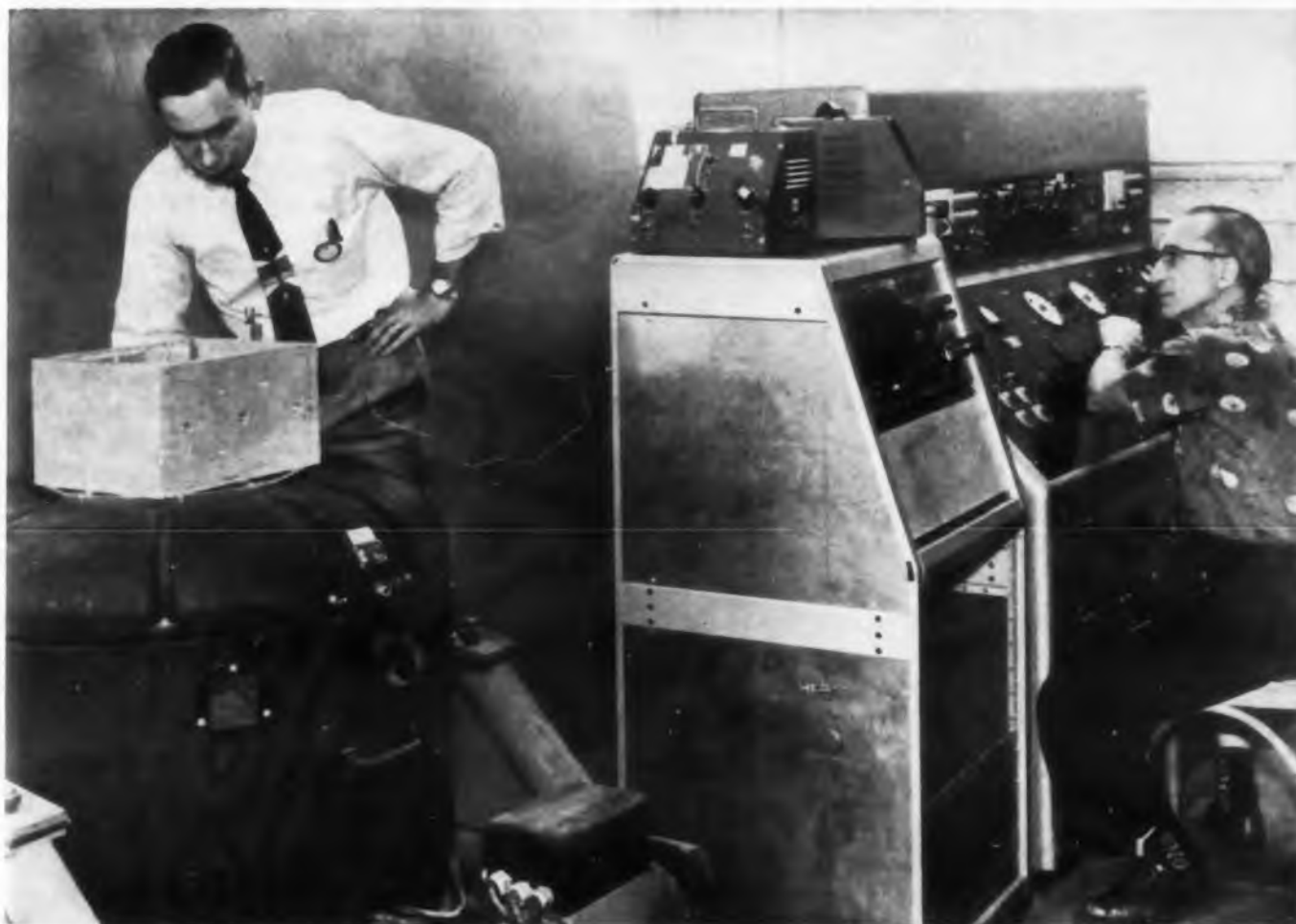
Missile parts must take a beating. In this vibration test, the specimen is mounted in the heavy jig. Acceleration and frequency are monitored at the test console.
