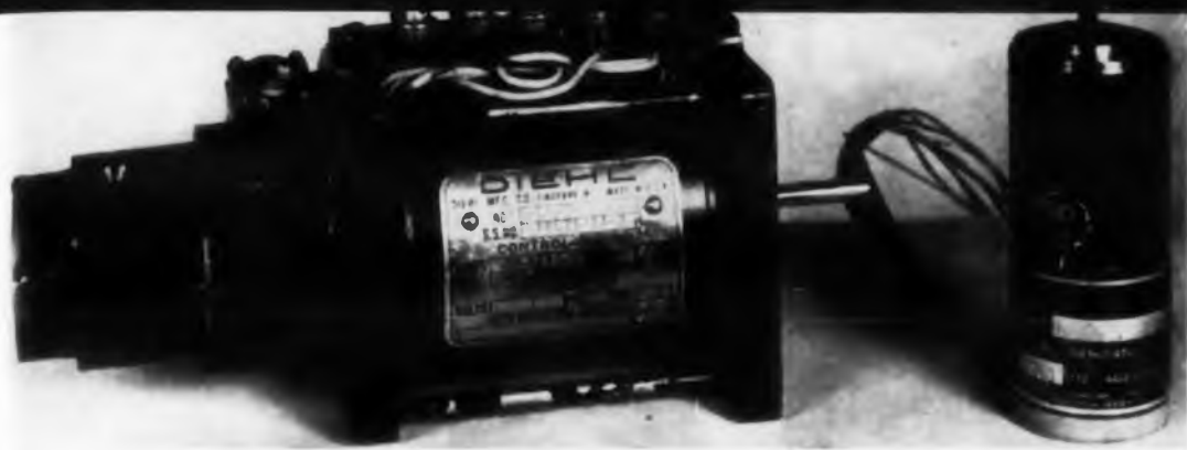
Fig. 2. Large 60 cps motor (left) replaced with smaller motor when 400 cps power supply was adopted.
