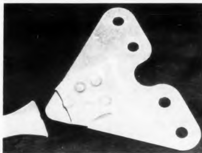
"All shook up" by exposure to 400 cps vibration at 26 g.
