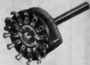
Type H: Standard 12-position; 1-7/8" diameter; 15-30-60° throw; phenolic, Mycalex or steatite.
