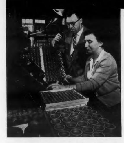
Mr. Cliff Horstman checks performance readings for Hipermag cores using the Roberts Dynamic Tester. This production-line test eliminates costly and complicated testing at your plant. After the Roberts test, Hipermag cores are "pegged" here according to their performance characteristics. This practice assures perfect performancematching every time.
