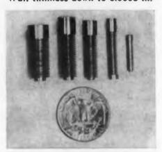
These flexible metal bellows range from 1 to 0.125 in. O.D. and come in any wall thinness down to 0.0008 in. The metal is a nickel alloy of high tensile strength and low hysteresis with resistance to corrosion and temperature.
