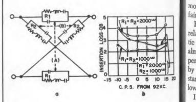
**Fig. 4.** Parameters of a narrow band crystal filter with two balanced quartz units.
