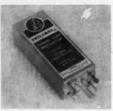
For operation with transistors or tubes, MI series tuning fork resonators take 15 g 11 msec shock. In frequencies from 400 to 2200 cps, and in 0.01, 0.02, or 0.05 per cent accuracy ratings in -55 to +85 C range. Accuracies unaffected under 5 g vibration to 40 cps.
