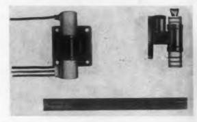
Two series of ceramic-metal reflex klystrons. The 1K20 models cover the 8500 to 11,700 mc range at output power levels to 50 mw. They withstand 15 g vibration with less than 100 kc frequency deviation. For use at any altitude, they are rated at 250 C seal temperature.
