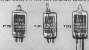
triggering requirements. Tubes hold off high voltage, pass high peak current with low tube voltage drop. Three types available: 7190—pin base, 7191—top anode connector, 7192—flexible leads.
