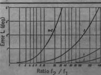
Fig. 2. Curve to relate error in degrees, L, to frequency ratio and number of sections, n.
