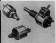
MINIATURE-Type G. Solid molded element. Only 1/2" in diam. Plain or lock bushing; also with line switch. Rated 0.5 watt at 70°C. Values to 5 megohms.
