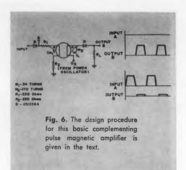
A small voltage does appear across the load resistor  $R_L$  of the amplifier (Fig. 6) due to the magnetizing current  $I_{m2}$ .
