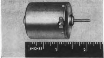
quality, this compact governed d-c motor is available in speeds from 1500 to 5000 rpm. Designed to operate over a voltage range of about 4 to 30 volts d-c, it is ideally suited for many applications such as: drive mechanisms in photographic equipment . . . marine navigation equipment . . . portable dictating machines . . . signal-seeking radios . . . tape players . . . and many types of portable instruments. Is this the answer to your design problem, too?
