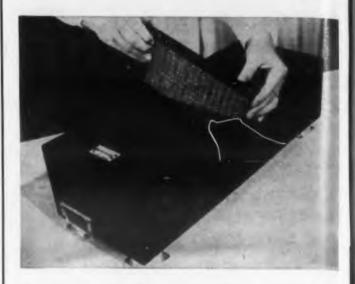
Gevic computer, for a typical fighter bomber application, will weigh only 45 pounds and occupy 0.8 cu ft. Arithmetic module is being inserted in package.
