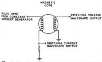
Fig. 3. This circuit was used to provide the switching data plotted in Fig. 4.
