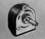
INDUSTRIAL—Type H with solid, hot molded resistor element. Quiet, improves with use. Life over 100,000 cycles. Rated 5 watts, 40°C; and 3 watts, 70°C.
