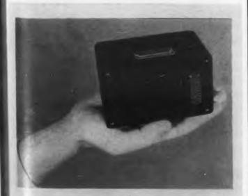
Electronic commutator has no moving parts and can handle 1000 samples per sec.
