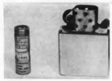
The model K nuclear battery delivers higher currents than Strontium-90 models, but is much safer to use. It uses krypton-85, a low cost radioisotope that diffuses quickly upon contact with air. A miniature unit has a current rating of 10 to 1000 μμα, an open circuit potential of n gage several thousand volts, and a linear charging rate to several hundred volts.
