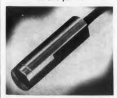
The OL-12-E features balanced low impedance windings, low record current, and high playback voltage for use with transistorized circuits. Bit densities of up to 200 bits per in., at 1 mil spacing, read and record information at high frequencies.
