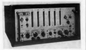
The model 13-20 counter measures frequencies from 10 cps to 1.1 mc, periods from 0 to 10 kc, time intervals from 3 µsec to 100,000 sec, and 1 to 999,999 total events. The instrument also measures time and frequency ratios frequency drift, and similar quantities, and will count and totalize discreet electrical impulses. Power input is 115 v ±10 per cent, 60 cps, 280 w
