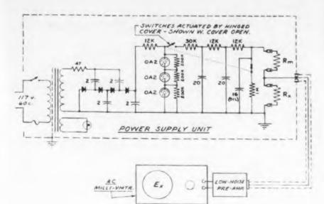
Fig. 1. (left) Circuit diagram of the system for measuring noise value.
