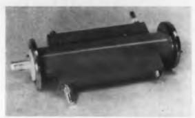
The model JP 400 mc precision coaxial directional coupler provides a forward output which is  $50 \pm 0.3$  db down from the forward power at center frequency. Reflected output is  $40 \pm 0.3$  db down from the reflected power.
