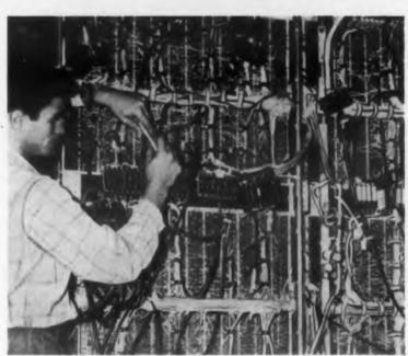
Univac engineer wires central computer with new FLEXOLON high temperature hook-up wire. Greater flexibility of the new wire also reduces wiring time.
