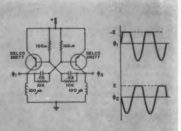
**Fig. 5.** The circuit and output waveshapes of a 100 kc transistor oscillator. It can drive approximately 50 pulse magnetic amplifiers.
