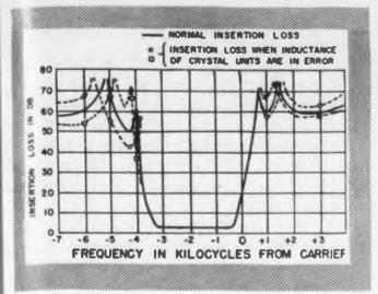
Fig. 3. Insertion loss of a crystal bandpass filter. The dotted curves show the effects of a one per cent change of the inductance of one of the crystal units in either lattice branch.
