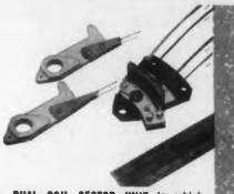
**DUAL COIL SECTOR UNIT** in which elements are independently phasable with slider positions.
