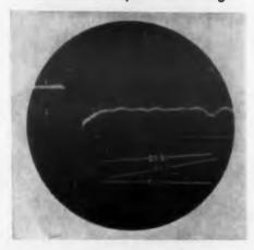
Germanium diode S570G has a 0.9 musec switching time. It has a stored charge, after a 10 ma forward current, smaller than that of a 3 μμf capacitor at 6 v. The S555G diode is specified at 6 musec and offers better dc charac-
