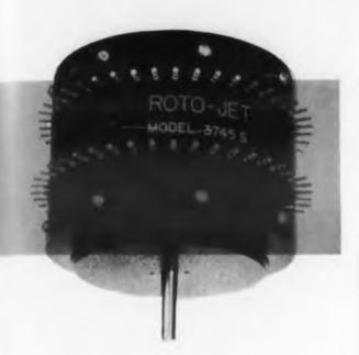
more than satisfactory force. Closure time is fast, being in the order of 40 µsec. Contact is broken in about 20 µsec. These times represent the leading and trailing edge duration of the typical square wave pattern. Duty cycle (ratio of closed contact time to total time between successive contacts) can be adjusted from 30 to 90 per cent.
