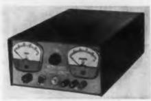
The transistorized Model SC-18-0.5 delivers 0 to 18 v, 0 to 0.5 amp. Regulation for line or load is less than 0.1 per cent or 0.003 v, whichever is greater. Ripple is less than 1 mv rms. Recovery time is less than 50  $\mu$ sec. Stability for 8 hr is less than 0.1 per cent of 0.003 v, whichever is greater.
