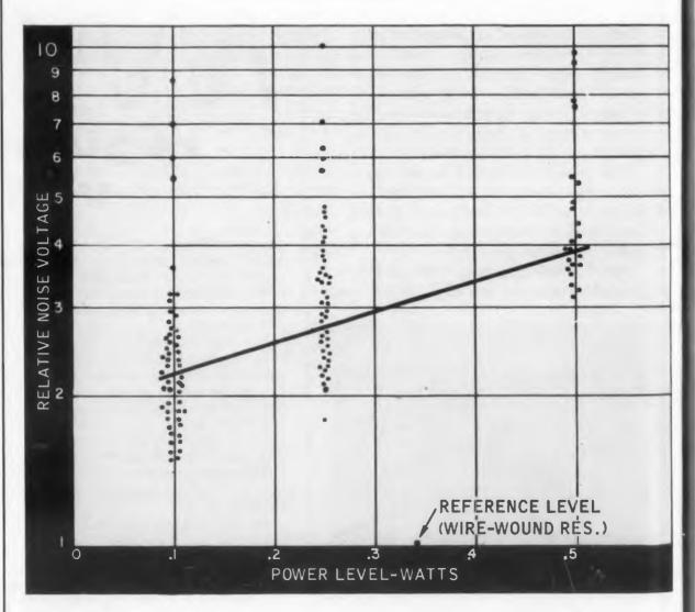
Fig. 2. Noise vs load characteristics for a typical lot of 80-1/2-watt 50 K deposited carbon resistors. Some samples too noisy to be shown on the graph.
