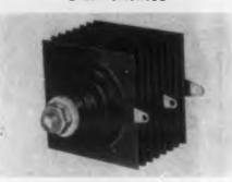
The selenium in these rectifiers has parallel grains. This structure allows higher current ratings for a given cell size. The rectifier is available in cell ratings of 18 to 36 v.
