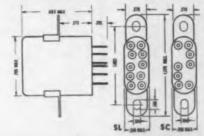
SL—dual coil latching relay. Operates on a 1 watt, 3 ms pulse at nominal voltage. Permanent magnet latch locks the armature in either position. SC—non-latching relay with series-connected dual
