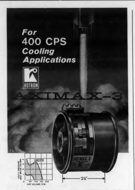
For airborne and missile cooling applications, the AXIMAX-3 when turning at 20,000 rpm will deliver 165 cfm at free delivery. This performance is possible although the fan is only 2.8" in diameter, 2.3" in length and weighs a mere 14 ounces.
