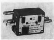
The frequency response of the Model 201 decade amplifier is flat within  $\pm 2$  per cent dc to 100 kc, and 1 db to 500 kc. Its input impedance dc-coupled is 400 K shunted by 30 µµf; output impedance is nominally less than 100 ohms. It is a gain of 10, and its equivalent noise level is less than 20 µv.
