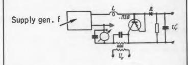
Fig. 4. Dielectric amplifier stage. A 24 mv signal (Ur) can be amplified to about 0.3 v at F = 1 kc, showing a good possibility of amplifying low-level signals. The author states that this is by far not the optimum design.
