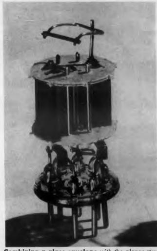
Combining a glass envelope with the planar structure of the ceramic stacked tube, the ceramic-in-glass tubes are capable of surviving extreme conditions of shock, vibration, and fatigue. The new structure (below) is shown with standard (T51/2) 6J6 mount (above) with which it is directly interchangeable.
