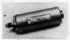
Series P300 pressure to frequency transducers have infinite resolution and provide 1 per cent repeatability. Units can be supplied on any RDB standard subcarrier telemetering frequency between 1.7 and 70 kc.
