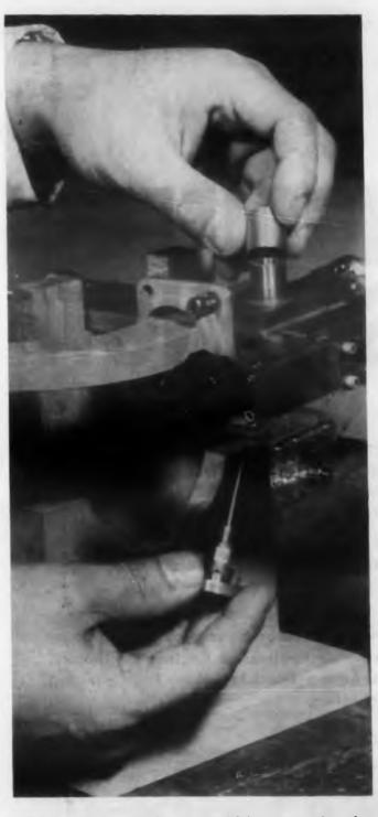
Equipment for studying amplifying properties of a nonlinear capacitor semiconductor diode. The right hand is holding the special diode and enclosure, and is about to insert it in
