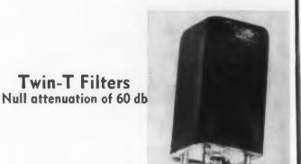
In these encapsulated, hermetically sealed twin-T filters, precision resistors and temperature compensating capacitors maintain attenuation over a wide temperature range. Null attenuation is 60 db or better. A range of null frequencies and impedance levels are available.
