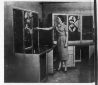
Two-unit Digital Data Recorder-Transcriber can make 10,000 measurements of temperature, pressure, strain and other variables in one second.
