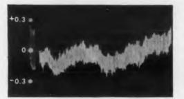
ACEPOT LINEARITY TEST Plot of voltage ratio error versus rotation illustrates linearity to better than  $\pm$  0.3%.
