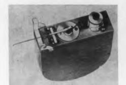
For use with transistor powered amplifiers in oscillograph recording applications, this galvanometer gives flat frequency response from dc to 35 cps, and extended flat response up to 200 cps with compensated signal amplification. Total dc coil resistance is 260 ohms, center tapped. A standard 3-in. pen can be driven 1 cm by 16.5 ma, or 4.025 v across the outside coil terminals. The unit comes in cased (model 8006) and uncased (model 8016) designs.
