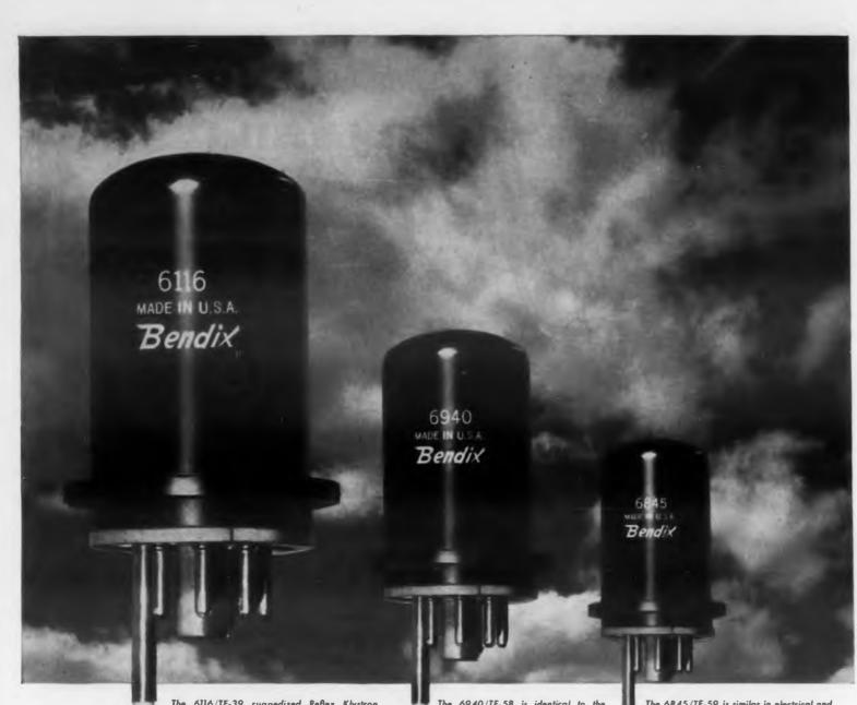
The 6116/TE-39 ruggedized Reflex Klystron thermally tunes a band of 8500 to 9660 MC by means of a diade within the vacuum envelope. Tuning speed over the required frequency range is 0.7 seconds min. to 3.0 seconds max.
