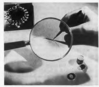
Shift register transistor is expected, with further development, to perform functions that now require a circuit arrangement of twenty transistors, forty resistors, and twenty capacitors. Object at upper left is a testing unit for the device. At lower right are elements of capsule in which an experimental unit is enclosed for testing. C
