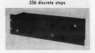
Used for the testing and calibration of multichannel pulse height analyzers with  $2^n$  channels, model PPG-256 precision pulse generator uses a mercury relay for the generation of positive or negative pulses, simulating the output of most radiation detectors. The output pulse amplitude may be varied over a 100 volt range in 256 discrete steps with a ratio accuracy of 0.1.
