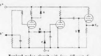
**Typical pulse circuit** with four different diode applications.
