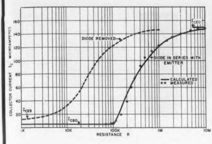
Fig. 5. Collector current of type 2N43 germanium transistor as a function of base resistance.
