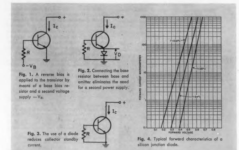
**SERIOUS** undesirable effects when biasing a transistor can be reduced by the use of a diode in the emitter circuit. An effective back bias can be obtained without appreciable increase in the collector standby current above cutoff,  $I_{CBO}$ .
