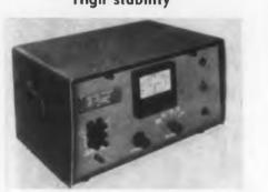
Model 343 impedance comparator features high stability. The equipment gives accuracy of 0.05 per cent over wide range of impedances from 10 ohm to 15 meg without adjustment.
