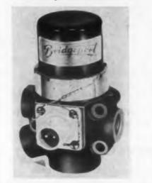
Containing a captive seal, this three-way solenoid-operated valve weighs 0.77 lb. It can handle pressures of over 3000 psi and withstands more than 350 F.
