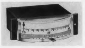
Expanded scale dc voltmeters can be supplied in the model 1135 and 1145 side indicator panel meters. The 1135 has a scale length of 2.1 in. and a panel area of 2 sq in. Scale length of the 1145 is 2.7 in., and panel area is 5.5 sq in. Voltage ranges lie between 4 and 265 v dc, and accuracy is  $\pm 2$  per cent of full scale.
