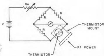
**Fig. 4.** D-C bridge circuit for measuring r-f power.
