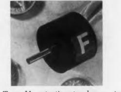
The Type 11 potentiometer has a starting torque of 0.5 gm cm. As part of the manufacturer's range of precision potentiometers, it is designed to provide analog conversion from mechanical rotation to an electrical signal. Linear and sine/cosine laws are available and other nonlinear functions can be manufactured. Potentiometer has good resolution and linearity. They are capable of reliable operation under severe shock.
