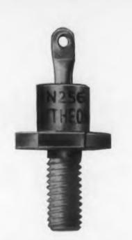
**Fig. 6.** Stud mounted diodes can carry more than 5 amperes.
