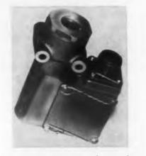
An intermediate mechanical snap action in the 90000 series pressure switch insures trigger switching of the electrical switch element and prevents welding of contacts. For use with hydraulic fluids or compressed air, the unit comes in pressure settings from 5 to 4000 psi.
