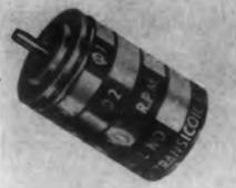
Weighing 0.9 oz, this size 6 servo motor will develop a stall torque of 0.125 oz-in., and has a free speed of 6200 rpm. The unit is available for 400 cps operation with 26, 33, or 52 v control phase windings. The control phase is center-tapped for operation directly with transistor amplifiers. Operating temperature range is from -55 to +120 C.
