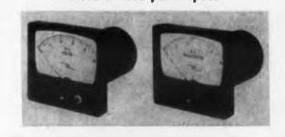
These single-range vtvm's require only as much panel space as ordinary 4-1/2 in. meters. The model 320 dc line comes in seven standard ranges from 0 to 1 to 0 to 1000 v. The ten standard ranges for the model 330 ac line are from 0 to 10 mv to 0 to 300 v rms. The ac meters operate at frequencies from 20 cps to 100 kc.
