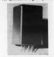
Containing all circuit types required for synthesis of digital systems, these transistor logic circuits and networks are designed for 100 kc operation and for use from -55to +75 C. They are packaged in encapsulated plug-in modules for in line or 9-pin miniature tube socket mounting.
