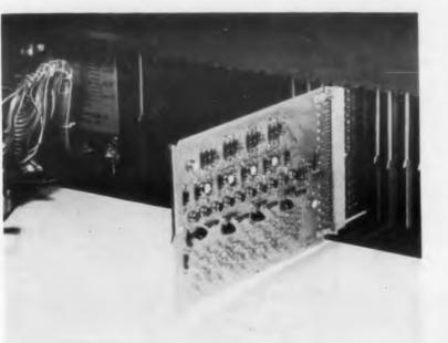
The housing is a green sand aluminum casting instead of sheet metal. It carries half the price tag of sheet metal. It can be drilled and tapped, and is available from the foundry on a few days' notice. Grooves in the floor and ceiling guide p-c cards into position for insertion.
