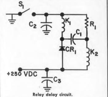
the discharge of  $C_1$ . The diode prevents  $C_1$  from discharging through any path except  $K_1 - R_1$ . The delay in drop-out of  $K_1$  is determined by the
