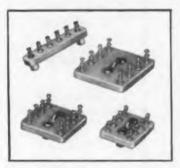
Cambion<sup>®</sup> grade L-5 silicone-impregnated ceramic terminal boards are completely unaffected by moisture, heat, and humidity. The brass terminals are silver-plated, the brass internally-threaded mounting studs are cadmiumplated — making for 100 percent protection. These
