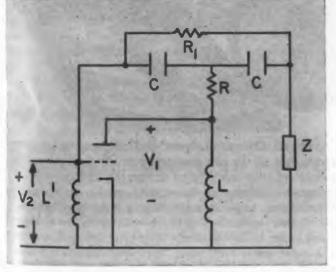
Fig. 3. Bridged Tee network used in an oscillator. Z is the load impedance. The element L' has been added to facilitate experimental adjustment to the required conditions.
