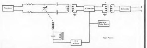
**Fig. 1.** Amplifier has a differential input and a floating output. Common mode rejection is 100,000 to 1.
