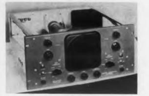
The type IT1193A cathode-ray oscillograph has identical horizontal and vertical deflection systems with maximum deflection sensitivity of 0.025 v peak-to-peak per in. from dc to 150 kc. Relative phase shift of the two amplifiers is not over 2 deg below 50 kc. All power supplies are regulated.
