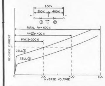
Fig. 1. Voltage sharing between unmatched series cells. (Germanium or large area silicon).
