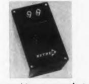
This precision mv per volt standard for convenient calibration and maintenance of strain gage systems provides a series of bridge outputs from 0.00 mv/v to 4.80 mv/v in eight increments. Nominal outputs are guaranteed to 0.25 per cent.
