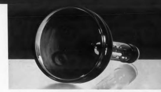
New five-inch experimental evaporated phosphor CRT
