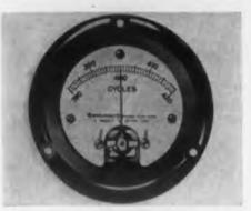
A self-contained, needle-indicator type unit for panel mounting, this 400 cps expanded scale frequency meter has a standard 380 to 420 cps scale readable to accuracies of 0.25 per cent over its full range. Between 380 and 420 cps the bridge used in the meter provides an output linearly proportional to input frequency.
