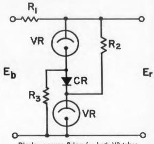
Diodes assure firing for both VR tubes.
