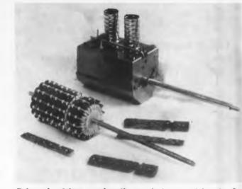
**Printed wiring and coils** are being used for the first time by the British for frequencies as high as 220 mc in this 14-channel TV current tuner developed by Sidney S. Bird, Ltd.
