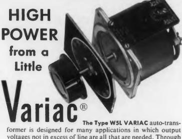
former is designed for many applications in which output voltages not in excess of line are all that are needed. Through modifications of the popular Type W5 units, the power rating of the Type W5L is increased to 1265 va. As with all VARIACS the output voltage is continuously adjustable from zero. Other VARIAC features included are Duratrak brush construction for extra-long life . . . excellent regulation . . . low losses . . . linear output. The Type W5L VARIAC is moderately priced at \$17.50.
