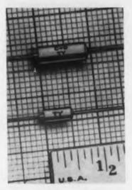
This series of small, tantalum solid electrolyte capacitors have useful temperature characteristics with a -80 to +85 C range. They have good stability of capacitance with time and temperature and are resistant to corrosion and vibration effects.
