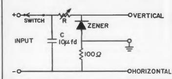
**Fig. 4.** A simple zener curve tracer to be used with a calibrated dc scope.
