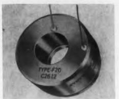
Type F20 electromagnetic focus coil is designed for photographic, flying spot, military and other special purpose tubes requiring short focal lengths at up to 25 kv accelerating potential without overheating. Minimum spot distortion is achieved by machining coil case to close dimensional tolerances. Sharp focus for high beam currents is assured by a large id to focus gap ratio.
