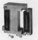
**REDUNDANT** — Close-spaced record-reproduce head speeds data processing by reading and checking tape immediately after recording. Reduces necessary equipment and power for checking register.
