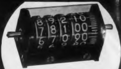
High speed, non-reset, direct reading counter to indicate increment of measurement in radar navigation instruments.
