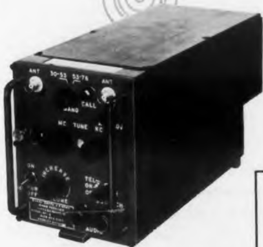
VHF, 920 Channels, fully transistorized Radio Receiver by Avco Mfg. Corp., Crosley Division
