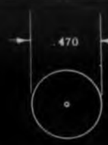
18-Series: Same as 06-Series electrically, but designed for lower cost commercial applications. Lengths 11/16" to 1-1/16"
