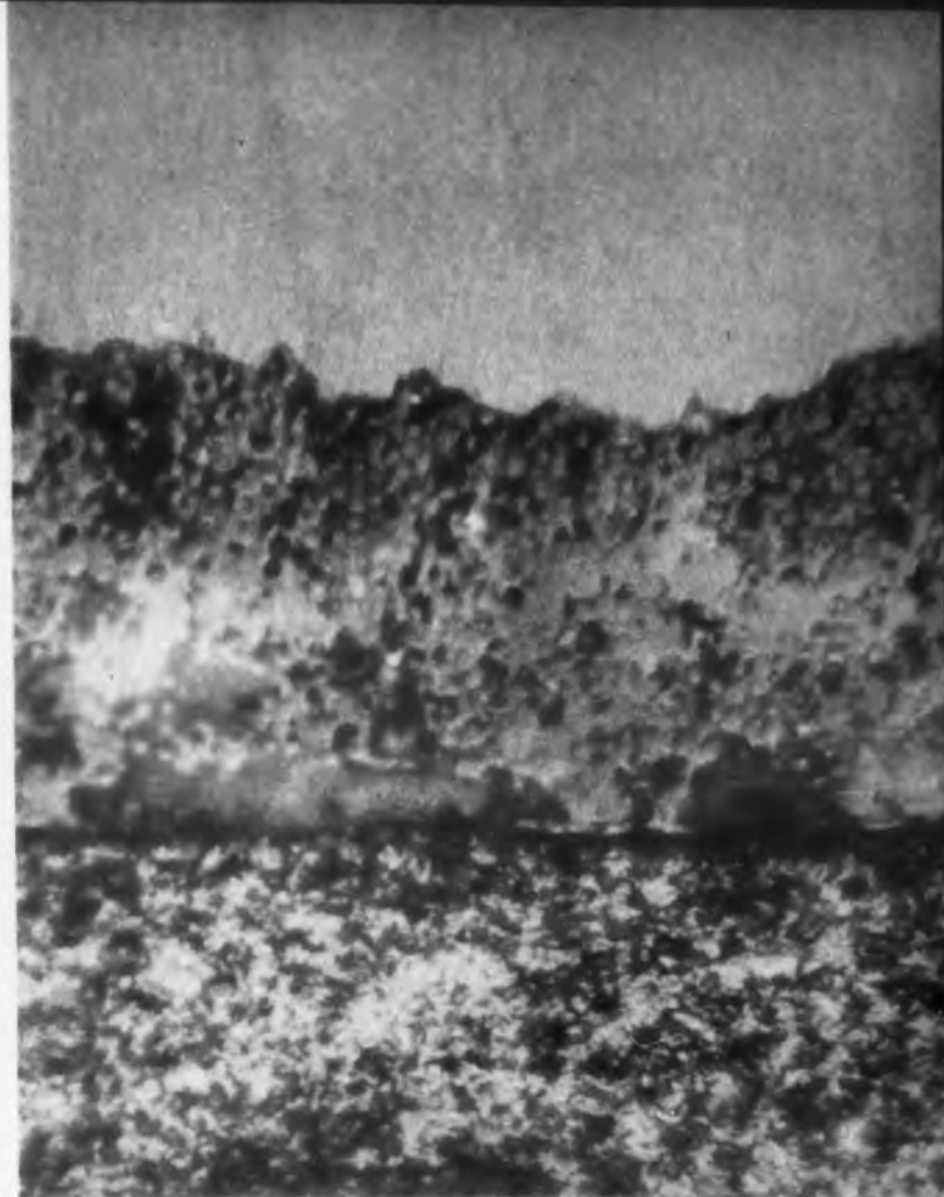
VITROTEX-D , magnified approximately 400X. The upper layer consists of glass fibers in fused Dacron*. Notice the even distribution which provides uniform insulation value—no large "islands" where fibers are missing.
