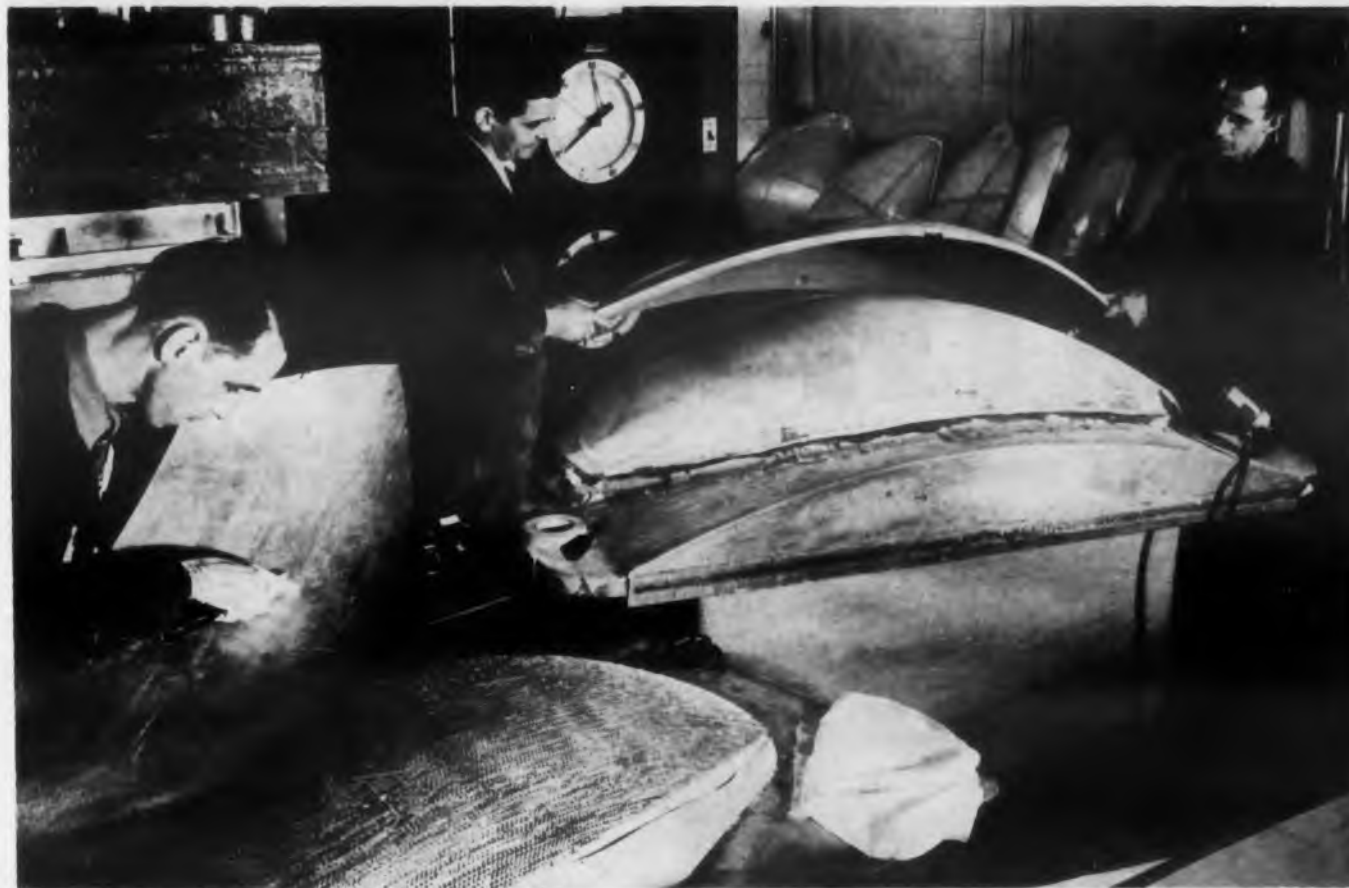
Fig. 3. Removing parabolic-reflector sections from the mold and checking for blemishes.
