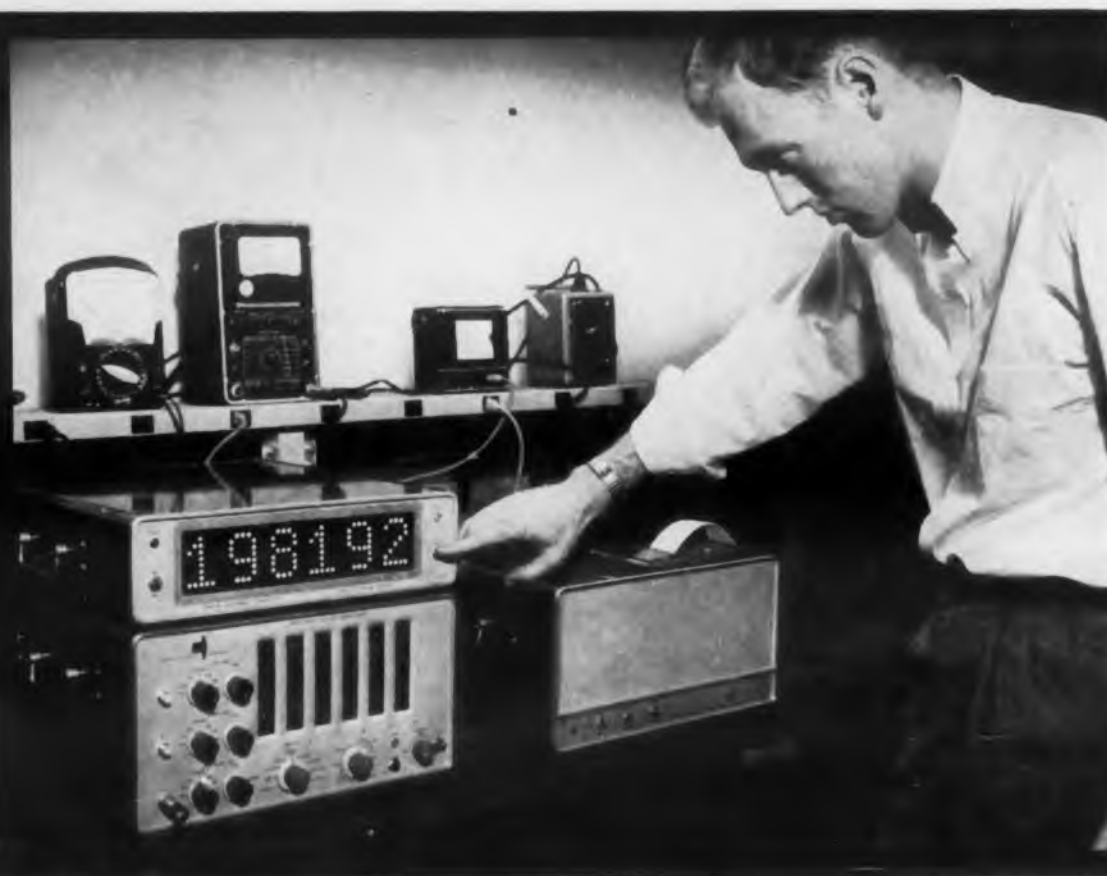
CMC's complete counting, timing, and frequency measuring system for laboratory and industrial use.
