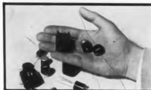
These miniature electronic components potted in Epon resin will withstand solder bath temperatures and retain excellent dimensional stability.
