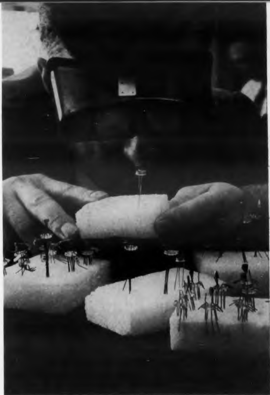
Developmental high-temperature gallium arsenide microwave diodes are examined by Dr. D. A. Jenny of RCA who developed new semiconductor device.
