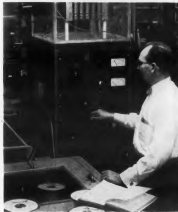
88 per cent extra margin of safety—This high potential test proved that Type EE extruded wire fell 88 per cent below FLEXOLON wire's minimum dielectric strength.
