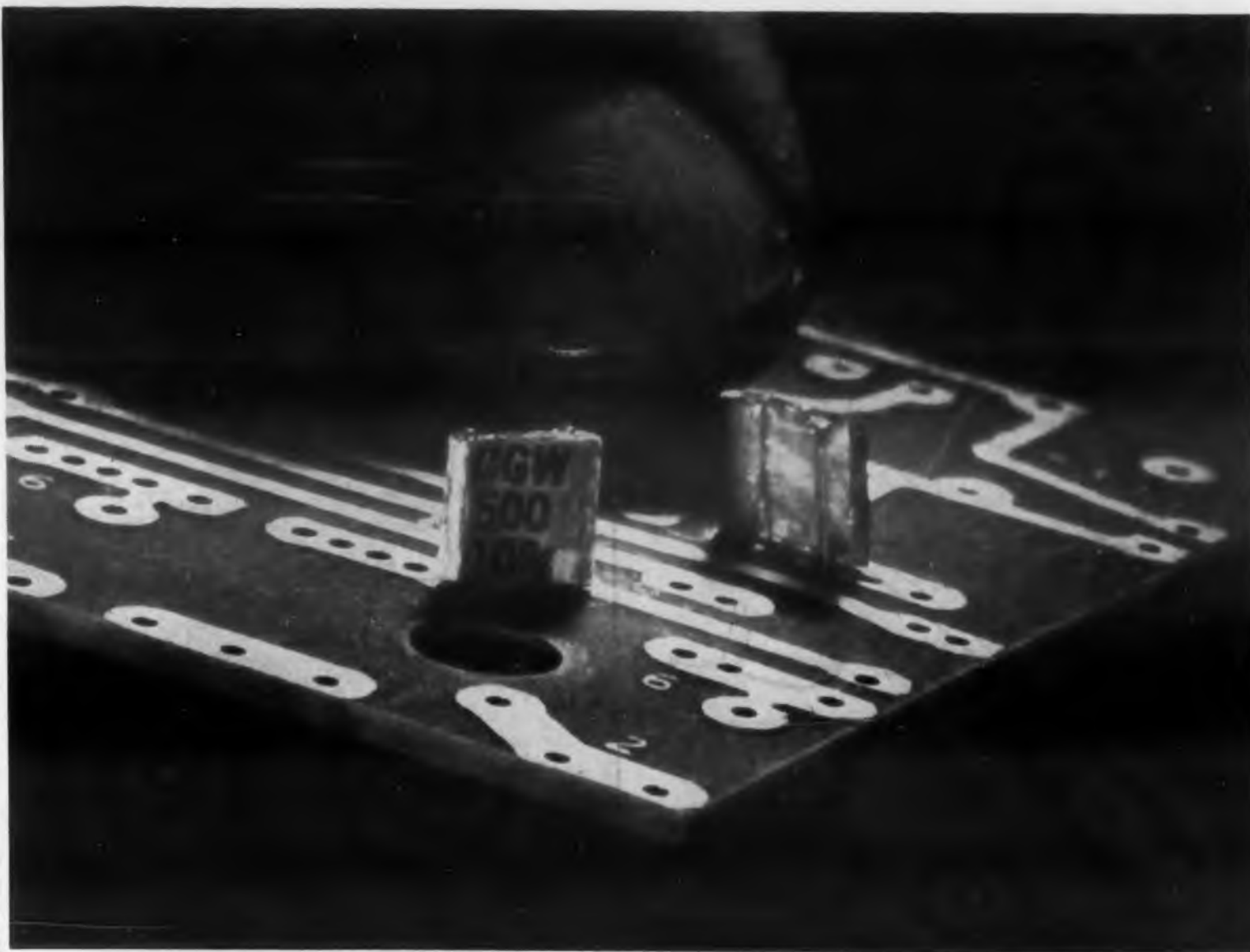
Truly sub-miniature, these capacitors were devised especially for printed circuits and automatic assembly. Since they retain all the properties of larger, pig-tail capacitors, they are well suited to general circuitry as well.
