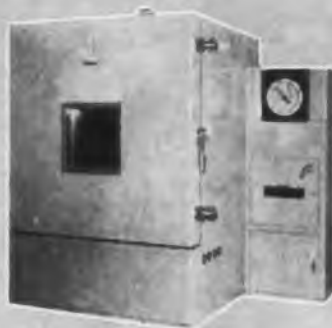
4 x 4 x 4 High-Low Temperature Chamber, +500° F. to -100° F., completely self-contained.
