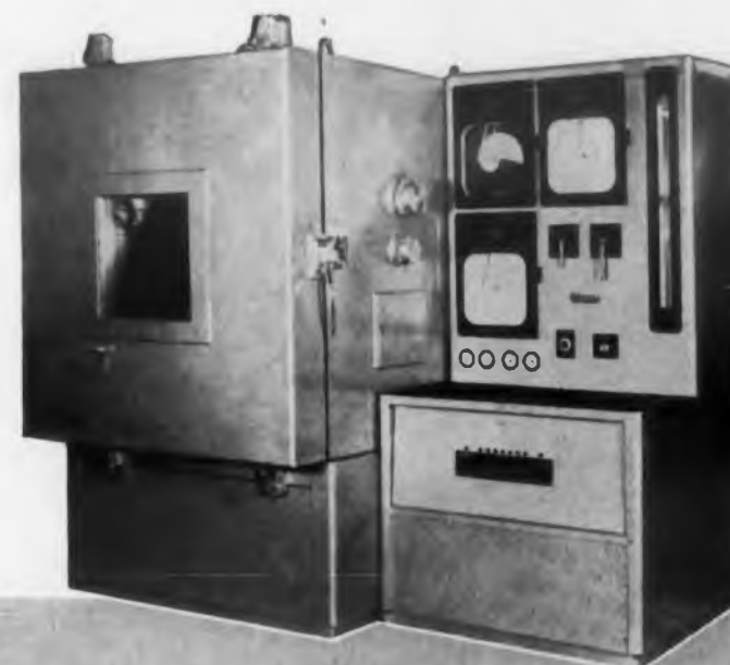
3 x 3 x 4 Altitude Temperature — Humidity Chamber, +500° F. to -100° F., 20-98% humidity, 100,000-ft. altitude.
