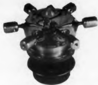
Vacuum transfer relay by Jennings can switch 15 kv at 200 C ambients.
