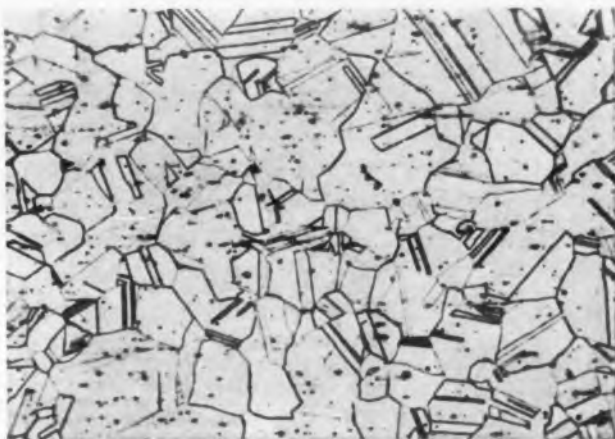
Polished and etched sample of Air Melted NICHROME* V in annealed condition.
