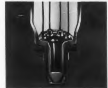
3. "New" Automatic Tip—Cross section of rigid pin base used on 110° picture tubes
