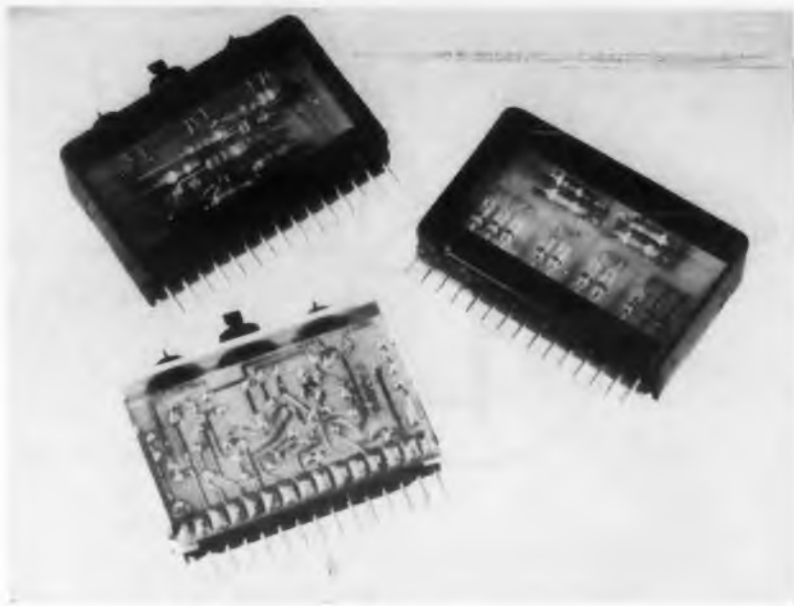
Fig. 2. Transistorized logical building blocks, 2\frac{1}{2} \times 2 \times \frac{1}{2} -in., simplify design and greatly reduce size of high-speed computers.
