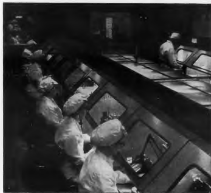
One "super-clean" area where various inspection and assembly operations are performed under conditions bordering on surgical cleanliness.
