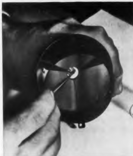
WEATHER EYES TO MEASURE CLOUD RADIATION. In the U.S. satellite, two "Weather Eyes" will peer from outer space at earth's cloud layer. Planned by the U.S. Army Signal Corps Engineering Laboratories and developed by the Perkin-Elmer Corp., Norwalk, Conn. to measure cloud radiation, these 4-ounce instruments are hardly larger than a pack of cigarettes. Each uses an f/0.7 mirror to pick up infrared cloud radiation and focus it on a tiny detector unit.
