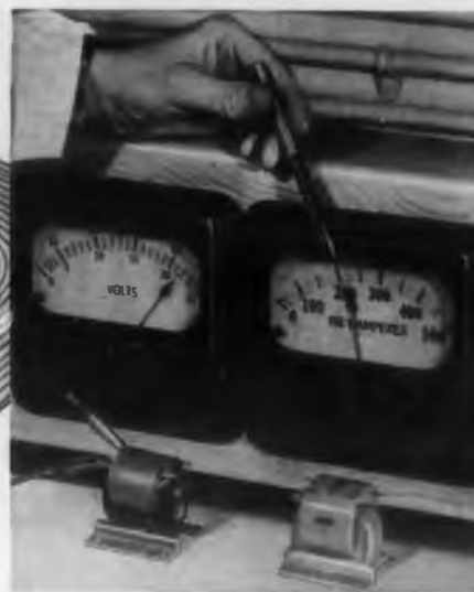
Both "normalized" and un-"normalized" cores record the same exciting current before encapsulation in high-temperature resin.
