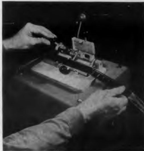
NATIONAL HELPS NEW SPLICER BOND FILM INSTANTLY —without disturbing original molecular orientation. Non-acetate film cannot be spliced satisfactorily by conventional methods. So the new device, developed by Shepard Laboratories, Inc., Summit, N. J. uses intense high-frequency heat to fuse the film instantly—without "burning" or affecting grain, high strength or durability. Side result: a superior splicer for all types of film.
