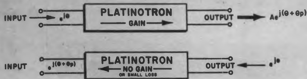
Fig. 1: The bi-directional properties of the platinotron allow rf energy fed into the output to appear at the input with little loss.
