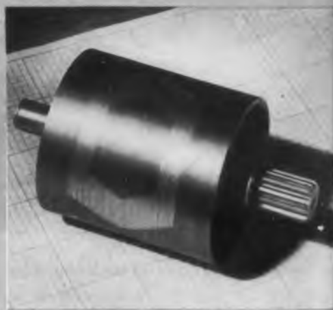
Fig. 1. Smooth metallic cylinder which replaces salient poles. Tests have been performed at speeds up to 60,000 rpm with excellent results.
