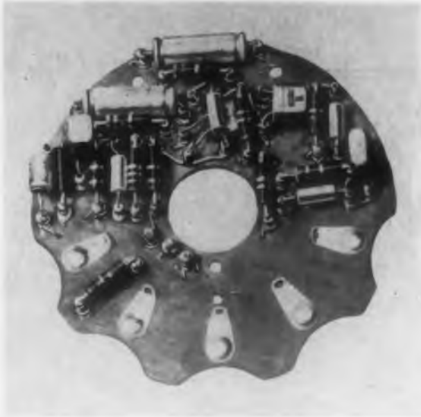
Fig. 2. Printed circuit construction of amplifier terminal board adds to compactness of unit.
