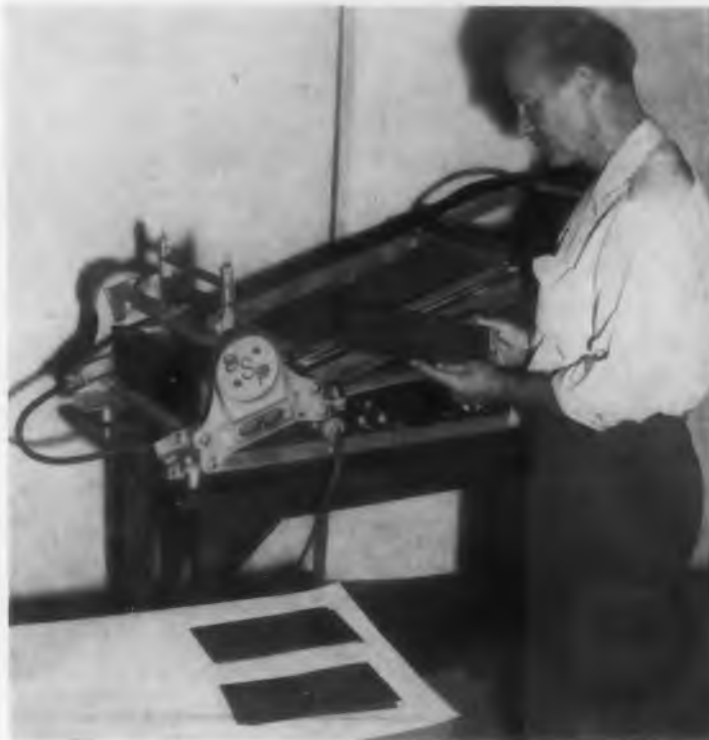
Fig. 1. Operator removing a printed-circuit board, produced in a laboratory by the dry-screen process described here. Only a few minutes were required.
