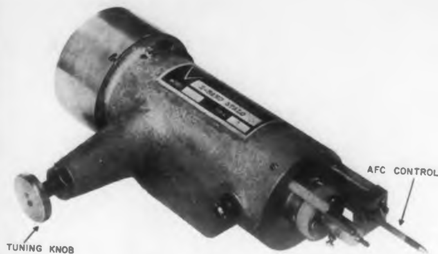
"S" band tunable stalo with AFC control.
