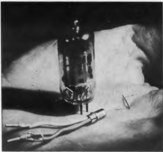
Applying superconductivity to computer problems, the Cryotron memory device is so small that 100 of them will fit in a thimble.
