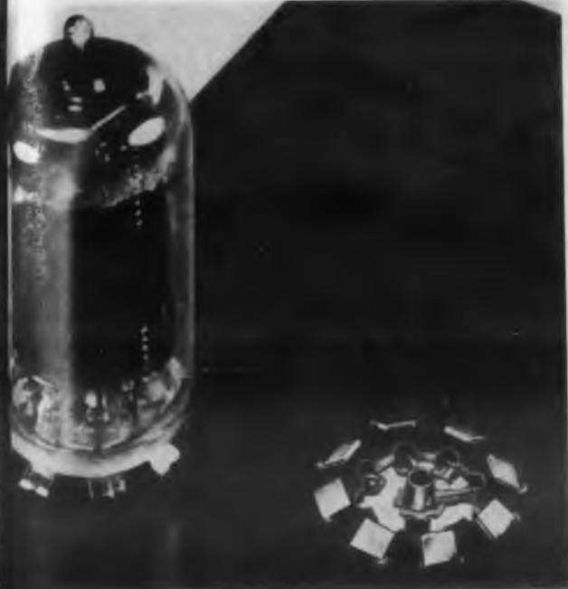
Cover Story: Shakeproof printed circuit tube socket. After shipping and assembly, center slug is stamped out.
