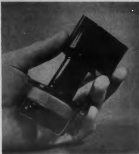
Fig. 2. The sounder of the tone-ringer circuit—receiver is shown in palm of hand and double tube resonator appears above.
