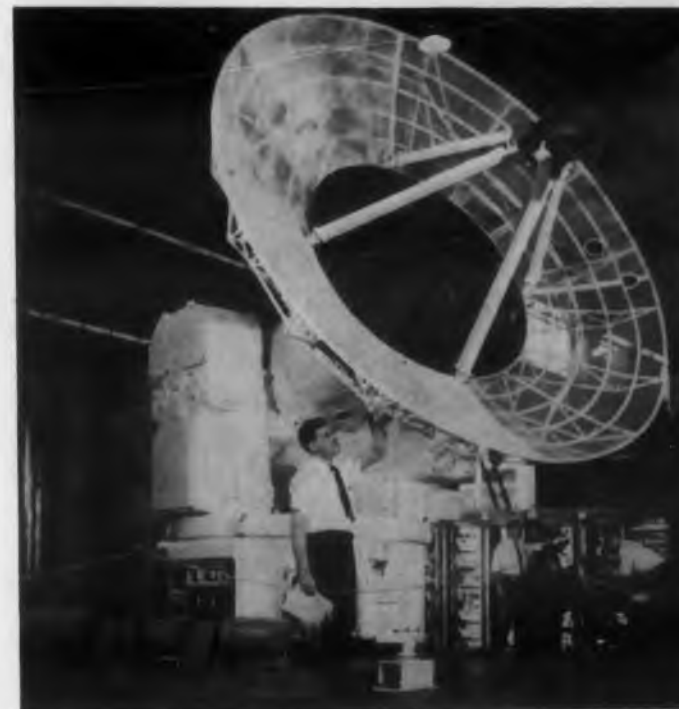
Antenna pedestal of new instrumentation radar system is designed for mounting on a detached tower, to minimize vibrations.
