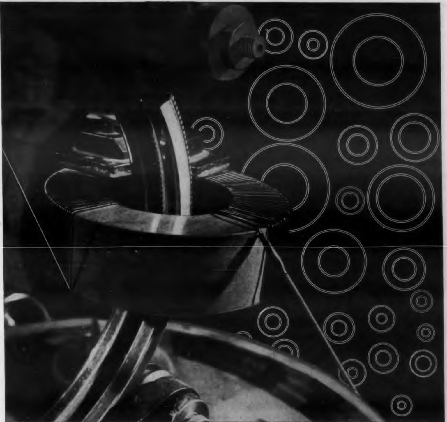
Cover Story: Shakeproof printed circuit tube socket. After shipping and assembly, center slug is stamped out.
