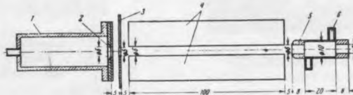
Fig. 1: Diagram of molecular generator arrangement. 1—beam source, 2—grid, 3—diaphragm cooled with liquid nitrogen, 4—electrodes of quadrupole capacitor, 5—resonator, 6—waveguide.
