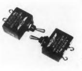
These miniature magnetic circuit breakers withstand 10 g at 55 to 1000 cps. The trip level is 135 per cent of rated load current. Units are available for interrupting 50 dc volts at cur-
