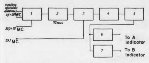
Fig. 6—Receiver. 1—balanced converter; 2—1st IF; 3—converter; 4—2d IF; 5 detector; 6—video channel of A-indicator; 7—video channel of B-indicator.
