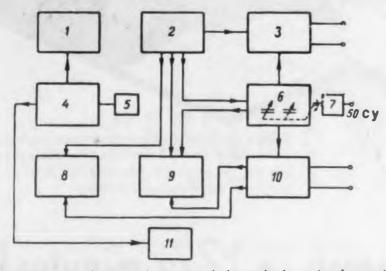
Fig. 1-Block diagram of automatic panoramic ionospheric station for vertical sounding. 1—power supply; 2—modulator; 3—transmitter; 4—automatic-control block; 5 electric clock; 6-master oscillator; 7-motor; 8-indicator with linear sweep (A); 9panoramic indicator (B); 10-receiver; 11-photographic recorder.
