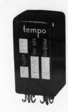
Both ac and dc models are available in a wide range of voltages and frequencies. The relay itself has dpdt contact arrangement, and contacts will handle a 2 amp resistive load. Power consumption is only 0.5 w.
