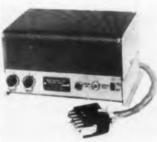
This wide range automatic light compensator (ALC) electronically compensates for variations in video signal level caused by variations in illumination, thereby eliminating the need for
