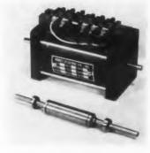
This new power servo has a high torque to inertia ratio and is capable of delivering 20 w output. The stall torque is min. 32 oz in. The torque to inertia ratio is 50,000, the weight only 4 lbs. The motor can be stalled continuously. The
