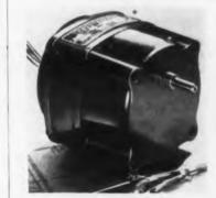
This 400 cy motor designed for airborne strip chart recorders and other applications, physically interchangeable with Holtzer - Cabot **RBC-**2505 60 cy motors, is designed for 115 v, 400 cy, 100 rpm, 7.5 oz in., continuous duty rating.
