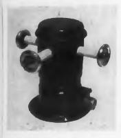
The Type RE4 single pole double throw vacuum relav has three high voltage terminals that are equally spaced on a 2-1/8 in. diameter glass bulb. Its operating voltage rating is 25 kv peak and for high altitude operation at this voltage it is provided
