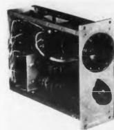
The Model 166 plug-in strip totalizer unit provides an accurate register in programs where speeds are too great for mechanical counters.
