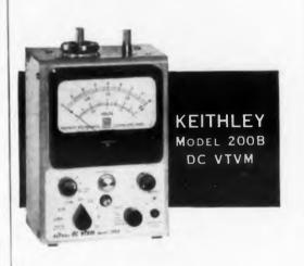
**BATTERY-OPERATED**, the Model 200B has voltage ranges of 0.008, 0.02, 0.08, 0.2, 0.8, 2, 8 and 20 volts full scale of either polarity. Accuracy is within 2%. Accessories permit measuring currents as low as 5 x  $10^{-14}$  ampere, resistances above  $10^{16}$  ohms, and voltages up to 20 kv.
