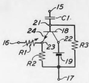
which has three terminals 15, 16 and 17. The network uses a condenser C1 in the branch between the terminal 21 for the base electrode of the transistor and network terminal 15. A battery 19 is provided in the
