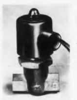
This solenoid valve for air pressures up to 100 psi, the Electroflo, may be secured with a full 3/8 in. or 3/4 in. orifice. Continuous duty solenoids are available from 6 v dc to 440 v ac. The overall length of the 3/8 in. valve is 2-17/32 in.; the 3/4 in. valve, 3-3/4 in. The inlet center to top dimension of the 3/8 in. valve is 4-3/8 in.; the 3/4 in.
