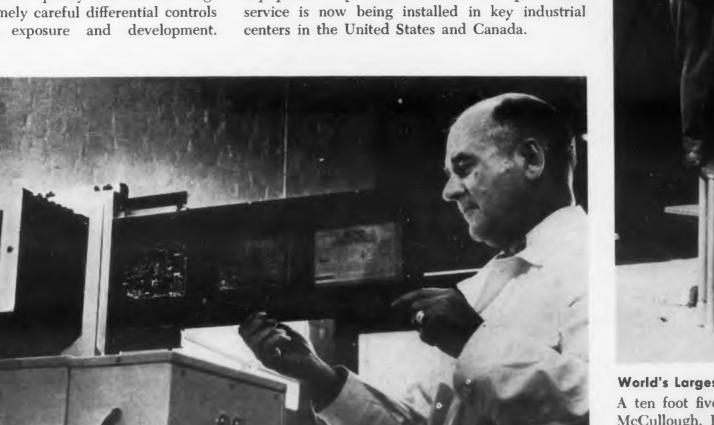
This projector is used for blowing up 105 mm negatives onto blueprint-size sheets of photopaper for exact reproductions of original engineering drawings.
