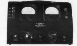
The Freed Type 1620 Megohmmeter is a versatile insulation resistance measurement instrument with a continuously variable DC test potential from 50 to 1000 volts.
