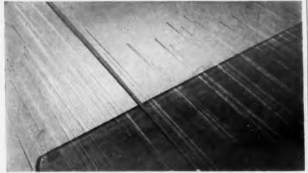
2. **EXCELLENT ABRASION RESISTANCE** of Analac is shown in this test. It has the same high windability normally associated with Formvar, Plain Enamel.
