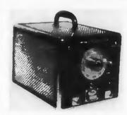
The Model 1065 variable filter is designed for use with IRD vibration analyzers and provides the facility for analyzing vibration at all frequencies in the range of 300 to 300,000 cy per min. Used with IRD
