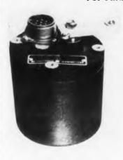
The D-9 permanent magnet type rotary servo actuator, for airborne applications, is designed for continuous operation at an output rating of 70 in-lbs at 8.5 rpm. Theoretical acceleration at stall is 40,000 radian/sec<sup>2</sup> and dynamic motor braking is incorporated. The unit has a weight of 1.9
