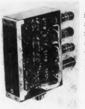
This counter, available in two models, the 369A and 369B, utilizes premium type tubes, conservative printed circuit design and few components. Power requirements are 6.3 v ac at 1.2 amps and 150-160 v dc at 7.5 ma. It will accept input pulses at rates varying from 0 to 100,000
