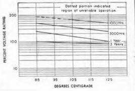
**OPERATES FOR 1 YEAR AT 125 C** Molded PVZ capacitors are designed for a minimum of one year's life at rated voltage and 125 C operation. Curves shown above are typical of performance.
