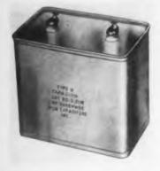
The type U line of capacitors developed especially for ultrasonic applications, are characterized by small size and low cost. Non-inductively wound and swedged with heavy terminal leads, the new type U capacitors utilize a high-breakdown plas-
