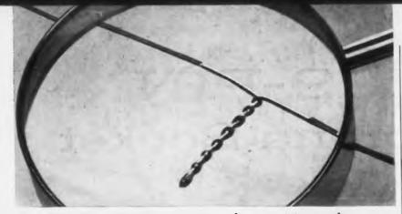
**STRONG JOINTS**—as strong as the same joints made in bare copper wire—are produced. Here in laboratory test, joint holds under high stress.
