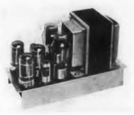
This regulated sub-chassis-mounted dc power supply has an output of 500 v dc at 300 ma max, which may be adjusted to any voltage between 300 and 500 v dc. The
