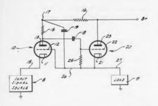
the input signal. The control grid of the first tube 10 is connected with the cathode of the second tube 20, and hence with the load 9, which is in the cathode circuit of the second tube or in cathode follower relation. There is, therefore, no phase reversal between the output signal and the input signal.
