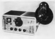
The Wide Range Type 504 heterodyne frequency meter is equipped with an interpolation dial which avoids ambiguity. Visual presentation is facili-
