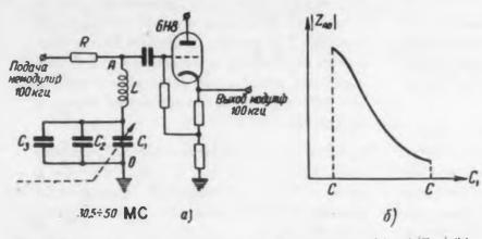
Fig. 3—Sweep-frequency modulator (a) and variation of load  $|Z_{AO}|$  (b).
