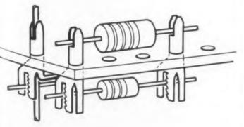
Push-in terminals clip component wires in place without soldering.
