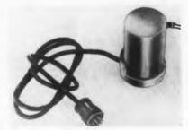
Based upon a differential transformer transducer principle, this series of instruments measures slowly varying environmental phenomena, from steady state to
