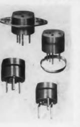
This multi - purpose socket may be used for 3 pin transistors with inline pins or with pins on a 0.200 in. diameter pin circle, accommodating triangular pin configuration, eliminating the need for stocking different types of sockets. The insulator body is made of low loss mica-filled phenolic, type MFE, in accordance with MIL-
