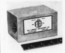
Although designed for self contained 400 cps input signals, this dc-ac magnetic amplifier is adaptable to input signals from dc to 1000 cps with the addition of a reference transformer. It
