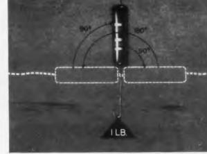
**HIGH LEAD BEND RESISTANCE** The new capacitors withstand one-pound-vertical-pull test moving the body of the unit 90°, then 180° in the opposite direction, then back 90°, to the original vertical position.
