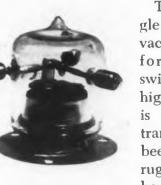
The Type JGF-RE2 single pole double throw vacuum relay is designed for antenna transfer switching applications in high altitude aircraft. It is a Type RE2 vacuum transfer relay that has been welded into a rugged gas-filled steel housing so that it can be
