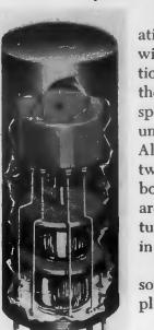
Designed for reliable operation at speeds up to 500 kg with maximum digit repetition rate above a megacycle. the Datakor DK107 is a highspeed magnetic shift register unit using two-cores-per-bit. All components including the two cores and four goldbonded germanium diodes are mounted on a miniature tube base and encapsulated in epoxy.
