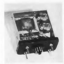
A miniaturized plugin control pack, containing all the basic control circuitry needed for use with contact meter-relays, measures approximately 4 x 2 x 4 in. A large number of circuit variations are available in the control pack. The stand-
