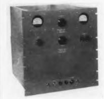
This closely-reguhigh-voltage lated, power supply is designed for use with high-voltage tubes. Output range is 400 to 4000 v dc, convariable tinuously switching; without current rating is 0 to 100 ma. Regula-
