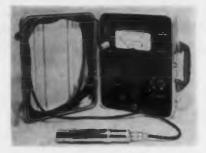
An all - purpose laboratory radiation detection monitor is designed for use in detecting alpha, beta (including Carbon 14 and Sulphur 35), and gamma radiation dosage, leak-
