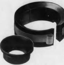
This ferrite "full-round" deflection yoke core for use in TV picture tube assemblies is pressed as a ring of perfectly uniform section and circularity. It is then "cracked" into two halves for
