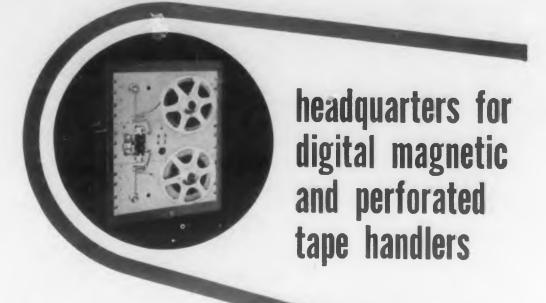
Model 902 Magnetic Tape Handler treats the tape gently while providing a start/stop time of 5-milliseconds. Fully reversible without stopping.
