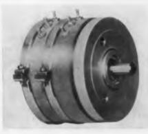
The Type 747-E Potentiometer provides a resistance range of 50 to 70,000 ohms with a standard linearity of ±0.15%. A special clamp band provides an unrestricted tapping area, allowing up
