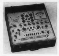
The Model 750 permits quick and accurate evaluation of any tube normally encountered in all phases of electronic work, including the latest military ruggedized types, TV, or hearing aid receivers. It also tests germanium diodes
