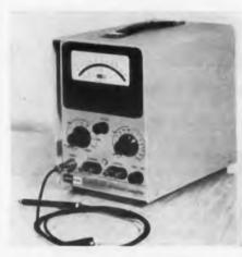
The Model 203 D-C Microvoltmeter-Ammeter is capable of making accurate measurements of voltages as small as  $10\mu v$  and currents as small as  $1\mu\mu amp$ . Fifteen voltage ranges cover from  $100\mu v$  to 1000v (full scale). Ten
