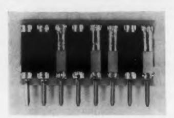
After the components are automatically inserted, they are dipsoldered to the clips.
