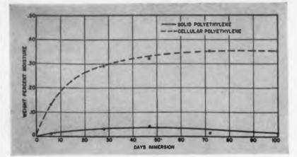
Moisture absorbed vs. days of immersion in tap water at 23 deg. C. Since BAKELITE Cellular Polyethylene is made up of hollow cells completely separated by walls of BAKELITE Polyethylene, its moisture absorption is low.
