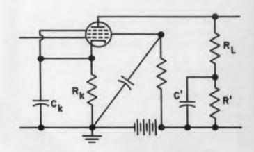
Fig. 4. Modified video amplifier, top, with its equivalent circuit, lower.
