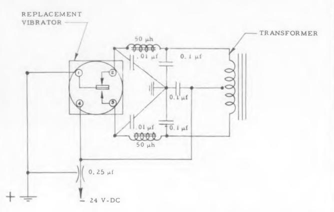
The suppression system applied to the vibrator in a 20-cycle ring includes a pi-type filter network on each line to the transformer; a feed-through capacitor on the d-c input to prevent interference from being conducted by the d-c line. Filter network can be mounted on the d-c input. In addition capacitors are installed just before the exit of the output leads from the shield, (not shown) to by-pass any residual interference that might have been coupled back into the leads.
