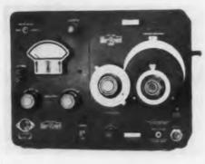
A new gridseparation oscillator, the Type 1218-A Unit Oscillator, for the 900-2000 M c range, is available by itself or incorporated in a new standard-signal generator.
