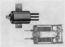
This relay is completely enclosed in a metal case, plugged with molded Bakelite on the contact end. Three contact leads are equipped with female
