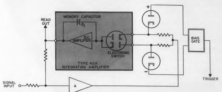
Fig. 5. In this signal amplitude memory, the amplifier is used as the output in a feedback loop.
