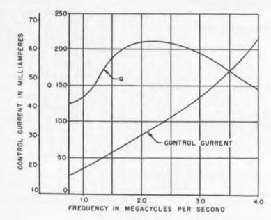
Fig. 7. The Q of the controllable inductor for the 2 to 4Mc band is highest at 2Mc, where the Q of the antenna is highest.
