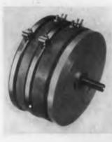
A special clamp band provides an unrestricted tapping area, allowing up to 33 taps, and presents a simplified means of phasing units in a ganged assembly without disassembling the units. The potentiometer is gangable in assemblies of up to 6 cup units on a single shaft. It has a diameter of 3-1/8" max and a cup width of 0.984". Potentiometer Div., Fairchild Controls Corp., Dept. ED, Robbins Lane, Syosset, L. I., N. Y.
