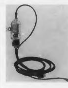
The Type RG-75 is a hotwire ionization gage that can be operated at atmospheric pressure without burning out and with no permanent effect on subsequent readings; accidental admission of air to a vacuum system does not destroy the gage. It is valuable not only in the high vacuum
