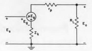
Fig. 2. Equivalent circuit for low frequency response, left. When E<sub>g</sub> is replaced by other variables, circuit at right applies.
