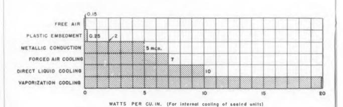
LECTRONIC heat removal can be divided into three phases: The removal of heat from the source: the intermediate phase of transferring the heat along a thermal path to the ultimate sink; and the dissipation of the heat at the ultimate sink.
