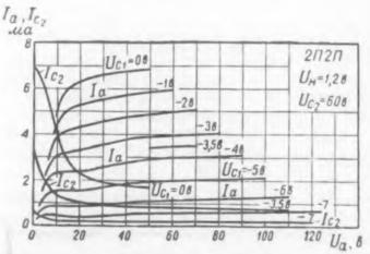
Fig. 4. Pentode 2P2P. Variation of plate current and screen-grid current with plate voltage.
