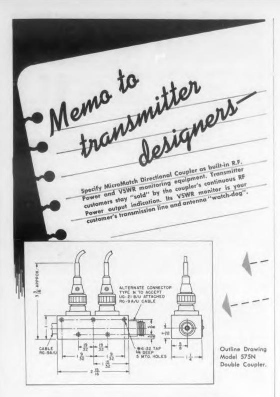
Performance proven, you will find these small, extremely low-cost MicroMatch couplers now incorporated in the most modern Government and commercial transmitters. MicroMatch Directional Couplers produce an output essentially independent of frequency over the range of 20 to 2000 megacycles. Couplers are adjusted to produce full scale meter deflection at power levels of 1.2 watts to 120 KW. Accuracy of power measurement is plus or minus 5% of full scale.
