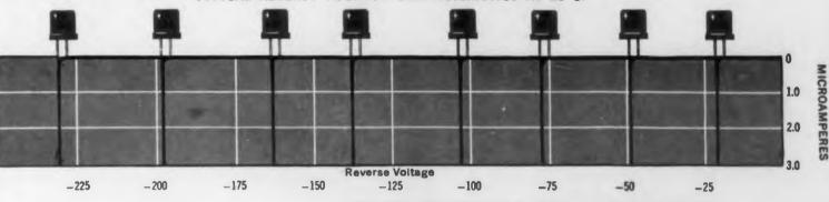
Raytheon Bonded Silicon Diodes provide low reverse current and good stability at high temperature. Every diode receives four temperature cycles of one hour at -55°C and one hour at +150°C, followed by thirty-six hours at 95% relative humidity and 70°C. Exact characteristics are maintained after temperature cycling and stability remains excellent over long periods.
