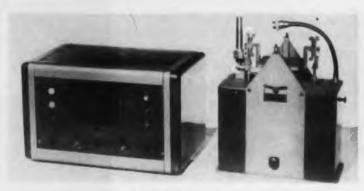
This "Simulation Table" is a single degree of freedom roll table for angularly displacing gyros and accelerometers, either statically or dynamically. It features a threshold of less than  $5\mu$ radians and a natural frequency greater than 15cy. Extremely smooth operation is obtained by using a specially designed, driven pendulum mechanism.
