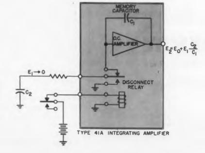
Fig. 3. An incremental charge is being inserted into an amplifier.
