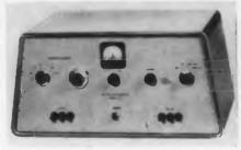
The Model D-4, a d-c wide-band stabilized amplifier, has a gain of 50,000 with drift, referred to input, of less than 25- $\mu$ v/hour. Frequency response is d-c
