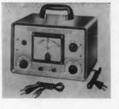
The In-Circuit Capacitor Leakage Tester, Model 383, shows the presence or absence of leakage in virtually all paper, mica, or ceramic capacitors while connected in the circuit, eliminating disconnecting and resolder-
