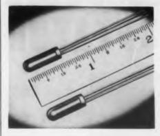
Matched - pair Type 2-OC72 highcurrent low-voltage power transistors are designed for such applications as portable phonographs and radios, and similar mass-produced devices. Efficiency is
