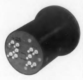
So we added the extra terminals you see in the photo. The "AMPL" leads go to the center arms of an external DPDT switch. The "METER" leads go to one side of the switch, and the relay leads to the other. In "Relay" position, a 5MVAC input signal will cause 100UADC to actuate the relay, and rapid, Go-No Go production tests can be performed by means of indicating lamps. When actual measurements are required, flipping the switch to "METER" position enables direct read-out of the signal.
