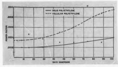
BAKELITE Brand Cellular Polyethylene for wire and cable insulation is a superior low-loss plastic that consists structurally of unconnected hollow cells. It is produced by the formulation of solid polyethylene with a foaming agent which, at the time of extrusion causes expansion to a cellular form. Properly extruded, the material will expand 100 per cent, giving a density about half that of solid polyethylene.
