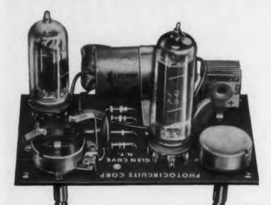
Audio amplifier unit by Photocircuits Corp., Glen Cove, N. Y., using Revere Rolled Printed Circuit Copper.
