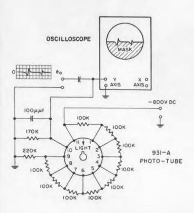
ASED on the well-known principles of the photoformer, the function generator described in this article can be assembled from equipment commonly found in the design and development laboratory. This generator will produce voltage waveforms as a single or multiple valued arbitrary function of a linear time sweep or a controlled variable voltage.
