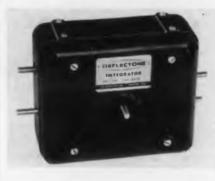
The Model 256, a 5" ball and disk type integrator, features two integrator sections driven by a common input. Output shaft speeds are independently adjusted by separate
