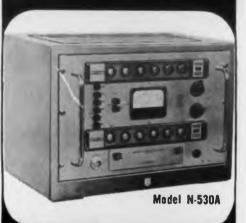
The simplicity and accuracy of Dekatron counting and timing circuits make the Ekco Model N-530A Automatic Scaler the most outstanding and most versatile instrument of its kind. This scaler will time a predetermined count, count for a pre-determined time or can be manually operated.
