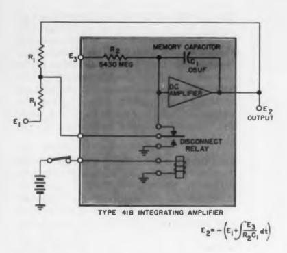
Fig. 2. In this circuit the amplifier is used as a voltage integrator.
