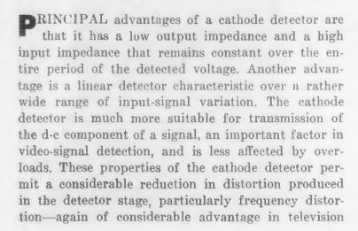
receivers. Among the disadvantages of cathode detectors are a reduced sensitivity to weak signals (below 1-3v); this is hardly significant with modern signal levels
