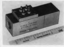
A line pressure rating of 250psig, together with high natural frequency and relative insensitivity to acceleration, are features of the Model P 134 Differential Pres-
