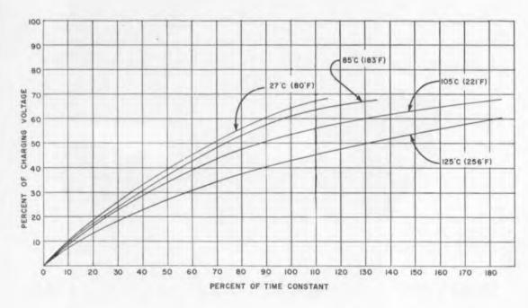
Fig. 5. Charging curves for 1.0mfd Vitamin Q capacitor at various temperatures.
