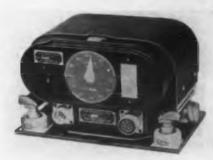
The RD-106/ ANH-2 is a recorder primarily intended for making voice recordings in aircraft from microphones, radio sets, and intercommunication sys-
