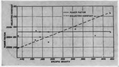
4. Power factor and dielectric constant at 1 megacycle vs. specific gravity. BAKELITE Polyethylene has a dielectric constant about midway between that of solid polyethylene (2.3) and that of the inert gas yielded by the blowing agent (1.0). Its value depends on the degree of expansion of the foam. The low power factor remains uniform.
