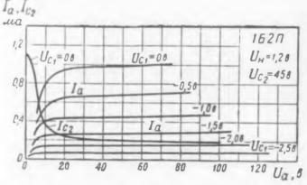
Fig. 3. Diode-pentode IB2P. Variation of la and la with U.
