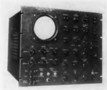
This dual-beam oscilloscope is particularly useful in the investigation of long-time phenomena using sweeps up to 10sec (200sec on special order). Signals on the two beams may be related using
