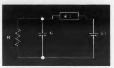
Fig. 1. Equivalent circuit of capacitor. R1 (or Z1) and C1 refer to resistance and storage effect of dielectric.
