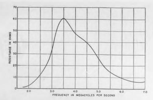
Fig. 1. The resistance of the antenna vs. frequency is plotted here.
