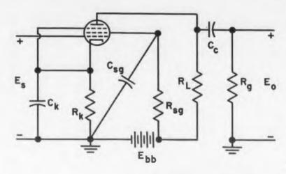
Fig. 1. Conventional-type video amplifier stage.
