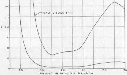
Fig. 4. The upper curve of antenna Q is the same as the lower curve, but magnified 10 times.
