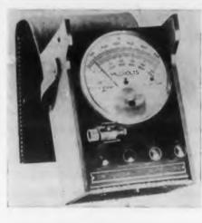
This self-contained, combination tester, Model 32-JP-4-MV, is designed for checking the millivolt output of thermocouples in both open and closed circuits, from 0-50mv and 0-1000mv. It will test either single or multiple thermocouples. It will also
