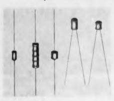
These subminiature units use extremely fine sizes of resistance wire to obtain two or three times the resistance value previously supplied on miniature bobbins. They are fully encapsulated
