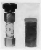
"Celab" resistance material is a variable resistance means capable of wide application. A quarter of a thimble-full of this powder will be an excellent insulator at 1 lb pressure, but will be a good conductor at 12-20 lb pressure. In a resistor, the
