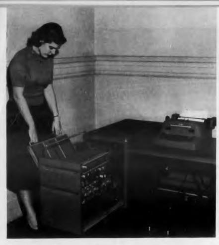
A plugboard memory is being inserted into the Wordwriter. Although no attempt was made to develop a compact commercial equipment, the memory apparatus easily fits into one-half of a standard desk.
