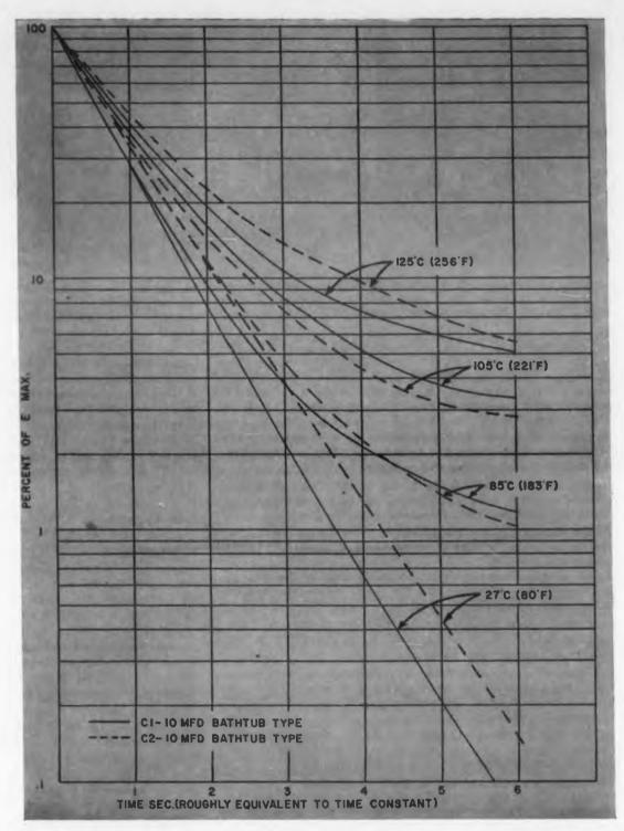
Fig. 2. Variation of capacitor discharge with temperature for different bathtub capacitors.
