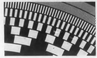
Gurley, manufacturer of the standard binary code disc for the electronics industries, is now able to supply four versions for use in either photo-electric, magnetic or contact types of pickups.
