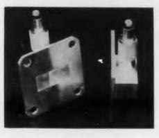
This crystal holder · is specifically designed to house a new microwave crystal recently released by Sylvania Electric Products Co., the IN369. The crystal and holder combination have val-
