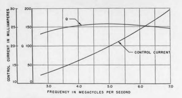
Fig. 6. The inductor for the upper band is designed for max Q at 6.6Mc, where the Q of the antenna peaks again.
