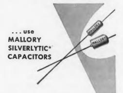
Capacitances up to 30 mfd. at 6 volts are compressed into subminiature case only  $\frac{1}{32}$  in diameter by  $\frac{3}{8}$  long, with temperature range from  $-55^{\circ}$  C. to  $+85^{\circ}$  C. Ultra-miniature Type TAW, rated 4 and 6 mfd. at 4 volts is only 0.145 in diameter by  $\frac{3}{8}$  long.
