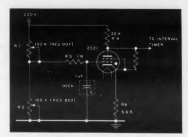
Fig. 4. Schematic for measuring charging curve of capacitor. Result shown in bottom graph.
