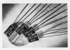
The 2N138 is a p-n-p fused-junction germanium transistor for pushpull class B audio output applications. It is sold only in pairs matched for optimum out-
