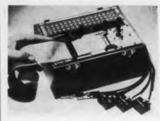
"Record-a-meters" are compact, rugged, lightweight, direct-writing oscillographs used in place of, or in conjunction with, meter-type test equipment to secure a continu-
