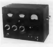
The precision wide-range Capacitance Bridge, Model 74B, is capable of making either direct or grounded capacitance and conductance measurements from 0.001 to 11,000-
