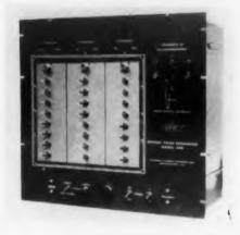
Model 300 is for use in the milliµsec to µsec range with fast pulse systems, oscilloscopes, wideband amplifiers, delay lines and other equipment employed in nuclear, radar, TV, u-h-f and other related fields. It generates square
