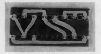
The printed circuit on the phenolic board is made by the "embossed" process.
