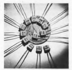
Eight new bonded silicon crystal diodes have been added to this line, providing a group of 12 hermetically sealed units having peak inverse voltages ratings from 3.0 to 225v. Four of the new units are designed for use as voltage
