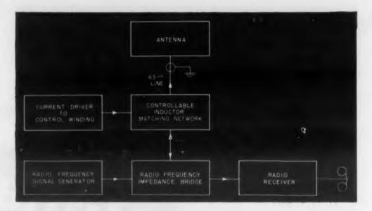
Fig. 5. The current driver in this measuring circuit is varied to make the matching circuit present a 63-ohm resistance to the r-f bridge.
