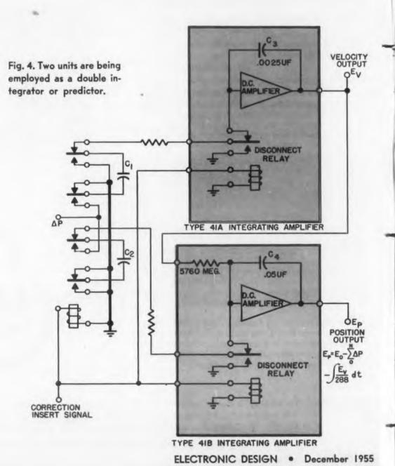
log computers and tracking systems can be filled by the relatively compact and inexpensive electronic integrating amplifier discussed here. One or more of these amplifiers can replace bulky and expensive servomechanisms having mechanical ball-and-disc integrators and very much slower response times. The circuit diagram and technical specifications of this device were given in a previous article\*.
