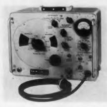
The Model 162 AM Signal Generator includes all components except the power supply, are in the r-f cavity to minimize leakage. Bands are changed by a rotating turret arrangement. Internal modula-
