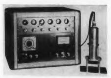
The GT-6 Glow Transfer register is used in conjunction with this firm's Model 200 Scaler. The register is exceptional in that a preset count of any number from 10 to
