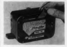
The Model 143 "Zero - Max" infinitely variable speed reducer has a constant torque rating of 30 in-lb throughout its speed range of true zero to 1/4 the input speed (0-450-
