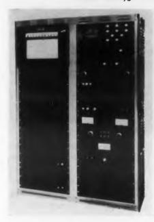
Two pulse height analyzers. Models 3300 and 3301, are of 100 and 256 channels counting capacity and use magnetic core memory circuits. They are based on the Argonne National Laboratory Model 101 design. Rates of accumulation of data may exceed 1.000.000epm, and input pulse rates of as much as 10 times
