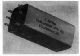
An inexpensive, distributed-constant delay line, the Type T30036 is designed for use as a compensating delay in the luminance channel of color TV receivers. It has a high impedance of 4300 ohms and uniform response to 4Mc. Phase characteristics also are linear within 5%. Total delay is  $0.8\mu \rm sec$ , and rise time is only  $0.1\mu \rm sec$ .
