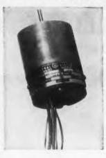
The miniature d-c servo motor 5BBY13DJ7 is capable of withstanding a high potential of 1500v and of responding to field currents of 0.0075amp. Suited for aircraft applications on blowers, actuators, tuners, and similar devices, the motor will operate equally well at sea level or at 50,000' and within temperature limits of -65° to 165°F. It is also used as a
