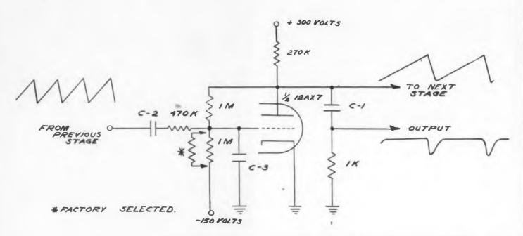
Each tone generator is made up of four of these direct-coupled divider stages.
