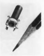
This phenolic coil form, Type SPC, is for printed circuitry. It is available in two diameters with four terminals each, and can be dip soldered after mounting.
