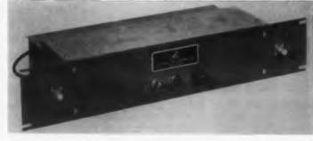
This distributed amplifier, Model 500, is designed for use as an oscilloscope drive, or for general laboratory uses. It has particular application in the field of amplification of narrow pulses, such as are found in the nuclear instrumentation field. Size is  $13\frac{1}{2}$ " x  $23\frac{1}{8}$ " x  $5\frac{1}{4}$ " over-all (approx). The power supply is a separate unit.
