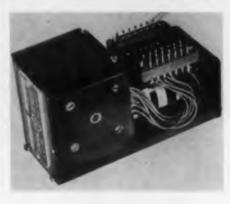
The Model No. 1205 is a high-speed sampling switch for telemetering, data recording, and related applications. It has two synchronized poles, with 30 contacts per pole. Fifteen alternate contacts and collector rings per pole
