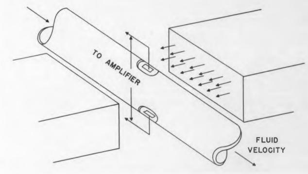
Fig. 3. This diagram illustrates the principle of the magnetic induction flowmeter.
