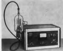
Nos. RG-2 and RG-3 Ionization gage controls measure pressures from 1micron to 2 x 10<sup>-10</sup>mm Hg. High stability and linearity are provided by a new type of circuit using an ion current amplifier
