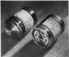
To qualify for the job, the molded parts withstood five room temperature shock tests at 50 "G's" plus constant vibration in the order of 25 "G's" for 4 hours at 600 F. Finally, the potentiometer was subjected to 1050 F for 15 minutes. The terminal blocks molded of Dow Corning 301 Molding Compound were somewhat shrunken and charred, but the brass inserts were still firmly retained.
