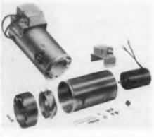
This compact vane axial fan is less than 7" x 4" x 5-1/4". The unit delivers 60cfm at 5" pressure water gage, and 112cfm at 1". It is designed and built especially to meet the service re-
