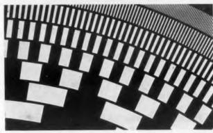
Gurley, manufacturer of the standard binary code disc for the electronics industries, is now able to supply four versions for use in either photo-electric, magnetic or contact types of pickups.
