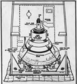
Shield of Du Pont "Alathon" serves as insulator for both the deflection yoke and kinescope retaining assembly on RCA Victor's new 21-inch color-TV set. (Kine shield molded of Du Pont "Alathon" polyethylene resin for RCA Victor by Sinko Manufacturing & Tool Co., Chicago, Ill.)
