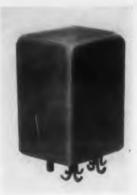
Contacts are silver, rated 2amp 28v d-e, and 115v a-c; 100,000 operations is the life expectancy at rated resistive loads. Operating power is 40mw for dpdt, and 20mw for spdt. The unit contains a high-efficiency double-coil magnetic circuit with a resistance up to 12,000 ohms, with a maximum dissipation of 1w. Size is (approx) 1" x 1" x 2" long. Magnadyne Co., Dept. MS, 84 S. Water St., Port Chester, N. Y.
