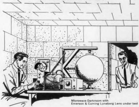
Eccosorb CH is a series of broadband absorbers reflecting less than 2% of the energy incident upon its surface. It is composed of enmeshed, rubberized fibers and made in sheets 2 feet by 2 feet in various thicknesses. Eccosorb CH is light weight and flexible. It is easily mounted and its natural, white surface color gives good light reflection.
