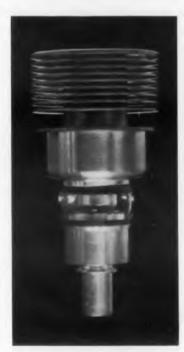
ML-322 U.H.F. diode for modulation clipper at frequencies to 1500mc. Extremely rugged. Oxide coated disc cathode (also used in ML-381 and ML-2C39A). Convection cooled anode; 15 watts diss. Peak inverse volts: 1800. Peak plate ma: 600. Average plate ma: 100.
