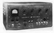
The 1000-A is a precision variable time delay generator which provides a positive pulse variable in delay in increments of 0.1 usec. The delay
