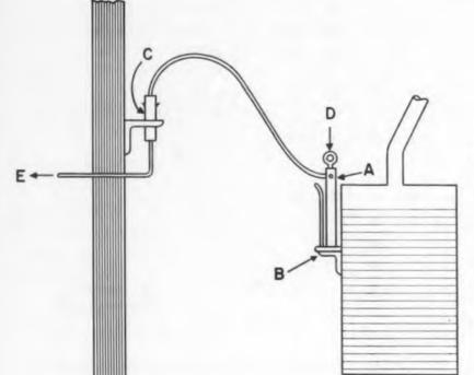
Fig. 2. A liquid-level detector for processing plants.
