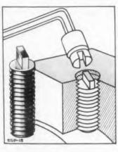
"Flush-Lok" slabbed head set screws are for applications in which the slab portion cannot extend beyond the tapped hole. In addition, there is a positive locking action that is effectively retained in all positions. Also, being flush with the surface, the screw becomes practically tamper-proof as well as resistant
