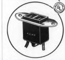
No. 221 (above) with soldering terminals and steel bracket with #6 clearance mounting holes. Also No. 222 with 6-32 tapped mounting holes. No. 223 (left) with 8" #14 or #16 plastic wire leads and steel bracket with #6 clearance mounting holes. Also No. 224 with 6-32 tapped mounting holes.
