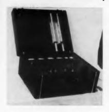
With this unit, a thyratron actually functions in an operating circuit with meters indicating operating points, permitting quick comparison with tube manufacturer's specifications and curves, and automatic indication of critical grid volts. An average
