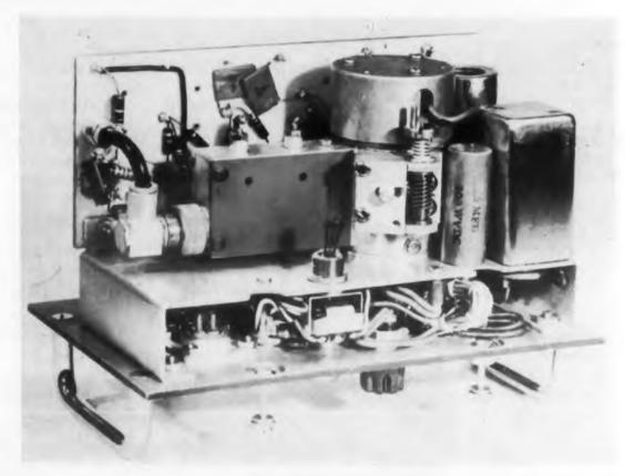
The miniaturized two-stage pre-selector is indicated by the color block. The plastic board is a terminal board and not a printed circuit board.
