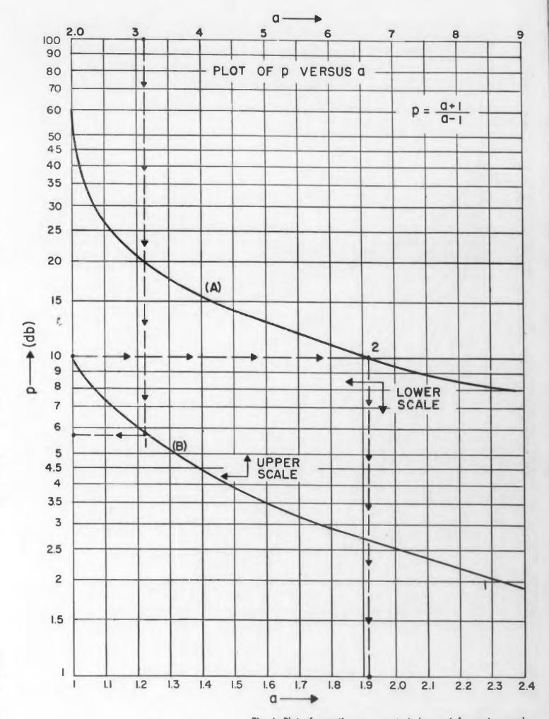
Fig. 1. Plot of equation p = a + 1 / a - 1 for various scales.
