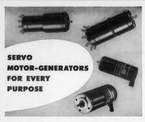
Kearfott Servo Motor-Generators are characterized by low rotor inertia, low time constants and high stall torque. Motor-Generator combinations provide ½ to 3.1 volts per 1000 R.P.M. with an extremely linear output over a speed range of 0-3600 R.P.M. and useful output up to 10,000 R.P.M.
