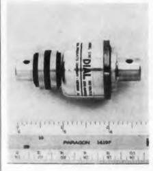
The Model C-130, a small but powerful electromagnetic clutch, is for instrumentation, servomechanism, control, and automation applications where there is need for a simple disconnect. It measures only 1-5/16" diam x 2-5/8" long, weighs 5-1/2 oz, has a
