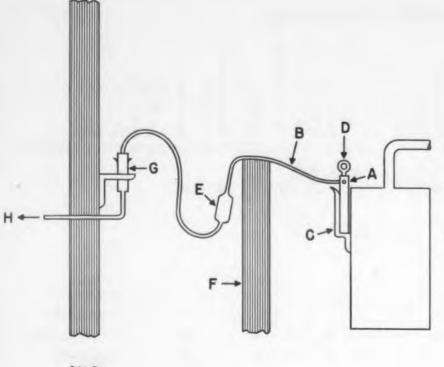
Fig. 1. A simple radiation detector and preamplifier for use in a processing plant.
