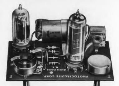
Audio amplifier unit by Photocircuits Corp., Glen Cove, N. Y., using Revere Rolled Printed Circuit Copper.
