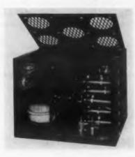
A line of magnetic amplifier voltage regulators is built by this firm to customer specifications. The typical unit illustrated takes a 120v single-phase 400cy input and delivers a d-c output of 15-150v at 0.05 - 0.50amp (to fields of exciter); va rating is 50; volt-
