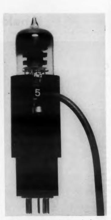
The base diameter of this Rotoprobe for 7-pin miniatures is 0.75". It is 1.87" high measured from the socket.
