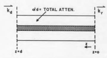
where  $K_r =$  reflection coefficient at the load or z = 0.
