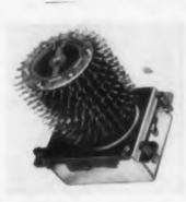
The Type E-RVF is a 30-point, 6-level rotary switch available with either two rows of contacts per level or one row of contacts and one common ring contact. Each wiper consists of two flat bifurcated springs, providing double contact surfaces at each
