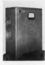
With three-phase 230-250v 60ey input, this portable laboratory power supply transformer unit has two output ranges: 211-640v 31-amp, in 10v steps, and 100-295v 66amp, in 4v steps. Adjustment is by eight fine steps and eight coarse steps with overlap. Taps are changed on three phases simultaneously. It is de-
