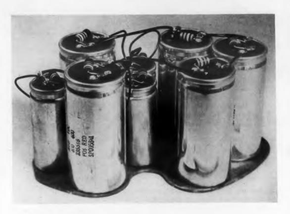
High voltage capacitor network before and after potting. Curing takes place in mold at room temperatures. No machining or shaping is necessary.
