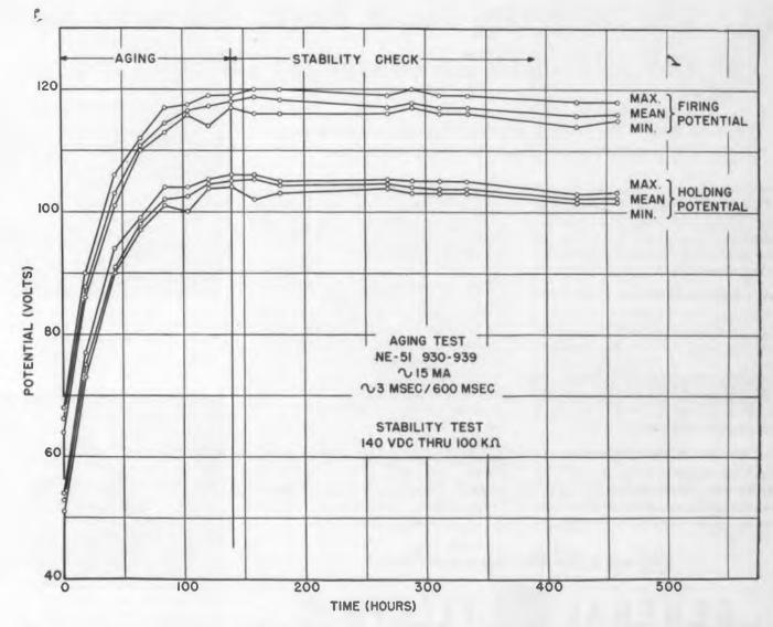
Results of aging tests of type NE-51 cold-cathode gas diodes. Processing was continued until the rate of change of characteristic voltage dropped appreciable.
