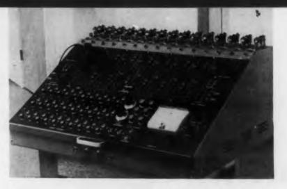
The 15 amplifiers are mounted in a thermally and electrically shielded portion at the top of the cabinet.
