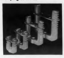
The clamp is a two-piece assembly consisting of a U shape and keeper plate. The U shape is serrated and designed for permanent attachment to a chassis. The keeper is pushed over the ends of the U and comes to rest in the proper position for retaining the wires firmly in place. To change, add, or remove wires, the ends of the U are simply pressed toward each other and the keeper is removed. Dakota Plastics Co., Dept. ED, 810 N. Mayo Ave., Compton, Calif.
