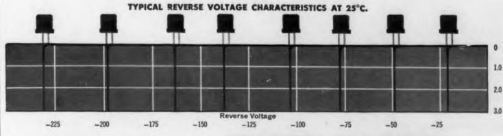
Raytheon Bonded Silicon Diodes provide low reverse current and good stability at high temperature. Every diode receives four temperature cycles of one hour at -55°C and one hour at +150° C, followed by thirty-six hours at 95% relative humidity and 70°C. Exact characteristics are maintained after temperature cycling and stability remains excellent over long periods.
