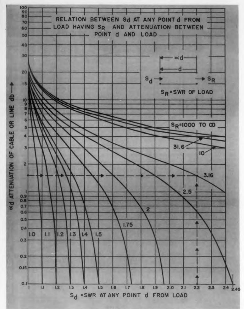
Fig. 2. Relation of standing wave ratio at any point d from a load for various values of SWR of load or attenuation of cable or line.
