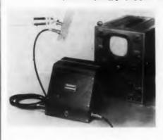
This detector determines the presence of corona in high-voltage rotating apparatus. It consists of a probe mounted on the end of an insulating pole, a control unit, and cables. It is connected to
