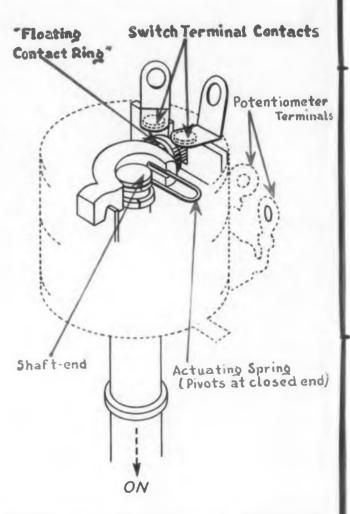
Floating contact ring is engaged with terminal contacts as shaft is pushed in. U-shaped spring is pivot. Because ring floats, contact life is long.
