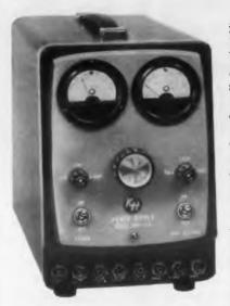
For the most exacting d-c regulation, the Krohn-Hite Model UHR-225 POWER SUPPLY provides unsurpassed performance. It is low priced and compact (7½" wide x 10" high). It has 0.002% regulation and 100 microvolts ripple over the entire operating range (150-500) volts and 0-200 MA). For line voltages between 105 and 125 volts, full rated current can be drawn continuously with a substantial margin of safety. The internal impedance is less
