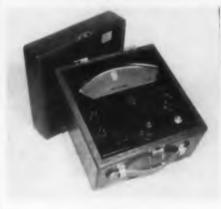
This ohmeter and megohmmeter permits measurement of high resistance values to a fraction of 1%. It has a zero adjustment which compensates for varying battery voltages; once zeroed for one scale, the adjust-
