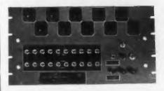
This timer, for use in the controlling of a sequence of events, contains 10 stages of thyratron-controlled time-delay circuits. The length of de-
