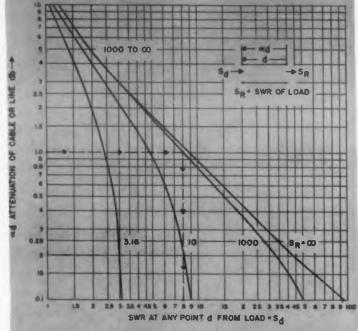
Fig. 3. Relation between  $S_d$  at any point d from load for various values of  $S_r$ . See also Fig. 2.
