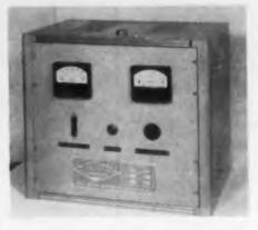
Illustrated is a typical "Sel-Rex Reactronic", a regulated d-c power supply unit for continuous output of 5-amp at 150 v. Static regulation is ±1% from no load to full load. These units are
