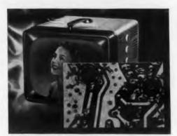
PORTABLE TELEVISION. Printed circuit hoard in this new receiver contains more than 50% of the wiring. Smaller chassis, yet full size screen. G-E Thru-Con Boards reduce as-
