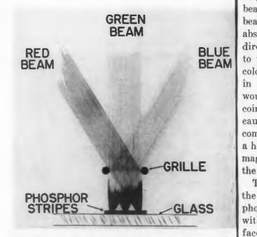
The electron beams are reduced in diameter by the grill in the "post-acceleration" tube.
