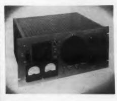
The Type 1002-C is a wide-range incremental - inductance bridge that will measure from 0 to 5h, and 5 to 180h at any frequency from 60 to 1000cy. It is used to measure small choke coils, toroids,
