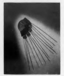
These p-n-p fused junction germanium transistors which are one-quarter to one-third the size of former units have a volume of only 0.0087 cu. in. They are designated types 2N130, 2N131, 2N132 and 2N133. The first three are intended for use in audio or low radio frequency applications; the fourth is a
