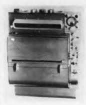
The Series 700C Recording Oscillograph is engineered to centralize all automatic operating controls on a front panel and designed to simplify internal adjustments. Record magazines can be loaded in daylight and handle film or paper up to 12" wide. Record speeds range from 1/32 to 144ips.
