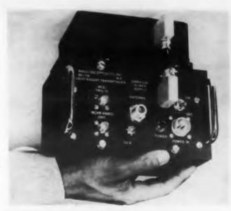
The separate power supply chassis is mounted on top of the transponder. The device can also be made with an integral power supply.
