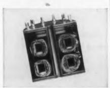
Section of magnetic amplifier coils embedded in Epon resin by Westinghouse Electric Corporation, Pittsburgh, Pennsylvania.
