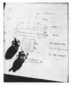
Silicon rectifiers capable of handling up to several kilowatts of power have been announced by this firm. These diodes have a typical forward voltage drop of only 0.7v at a current of 8amp and a cell temperature of 190°C.
