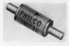
Specifically designed for u-h-f tuners, this mixer diode (1N1-73A) is made by a special process which results in uniform characteristics for tuner
