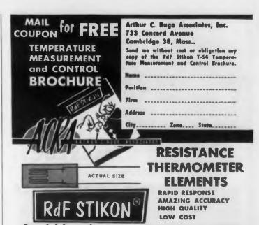
Intended for surface temperature measurement and control, an RdF Stikon consists of a temperature-sensitive grid of very fine nickel wire bonded into a paper-thin wafer of flexible insulating material. Attached by cement to almost any surface anywhere, an RdF Stikon is unaffected by shock or vibration. The response is extremely fast and amazingly accurate.
