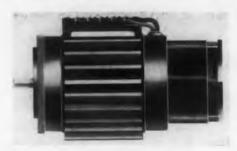
This 35w, 2-phase, a-c servo motor-tach-ometer generator unit operates on 115v 60cy. It can be used to regulate the speed of a motor or to stabilize closed-loop circuits. Because the motor and tachometer are mounted on a single shaft, backlash is zero. The motor component is rated for continuous duty at rated output. It can be stalled continuously with one phase of the motor excited at rated voltage and frequency. Minimum locked torque is 45 oz-in. Free acceleration is 10,600rad/sec<sup>2</sup>.
