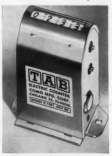
The "Tab Electric Counter" contains a one-piece cog-action actuator that insures positive stepping for each impulse up to 300cpm. This counter is a rugged, 6 oz unit of the nonreset type, with a cadmium-plated case. The four-digit model is 1-7/8" x 1-3/8" x 2-5/8" high. Numerals are black on white
