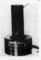
This high-speed precision sampling switch with integral motor and planetary gear reduction is available with 1, 2, or 3 concentric poles, 60 contacts per pole, utilizing a semi-molded contact plate construction for long life and dimensional stability. Connections to each pole are made by wire leads molded into the plate
