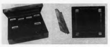
The "Universal Magnetic Testing Set" is a complete unit designed to make measurements that conform to the methods and specifications of the ASTM as described in their specifications on "Standard Methods of Testing Magnetic Materials." It includes dec and acc ammeters, rms and flux voltmeters, a low power factor wattmeter, a multirange fluxmeter, and a 25cm Epstein frame as specified by ASTM.
