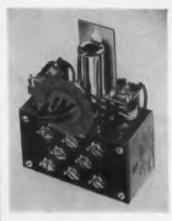
A repetitive series of circuit closures can be produced automatically by the Model S44 cold-cathode - tube electronic timer. The load circuit remains closed for a fixed time of about 60millisec, and the time between circuit closures can be adjusted to any value from as low as 0.03sec to 24sec. A maximum current rat-
