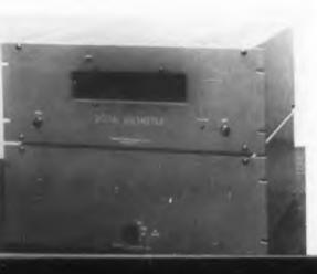
Four-digit unit has 0.1% accuracy. Switch selects a-c or d-c. Size is 14" x 19".
