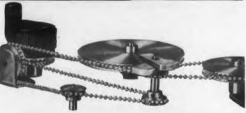
Now successfully employed in radio and TV tuners, recorders, air conditioners, timing devices, etc. Designed for economical, positive gear trains or drives free of slippage and backlash.
