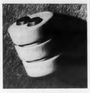
The tube is actually 3/8" long x 5/16" diam, about the size of a pencil eraser.
