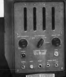
Measures frequency, speed, rpm, rps, random events Measures weight, pressure, temperature, acceleration\* Direct numerical readings 1 cps to 120 KC High accuracy, simple operation, compact, rugged
