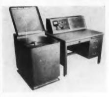
The Model CK-9X is a compact acceleration testing machine that tests and calibrates small assemblies while at the same time subjecting them to multiples of the acceleration of gravity. It is
