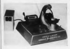
This portable toroidal coil winder is designed for both laboratory and production. It features quick set up and quick wire change. Any of three winding
