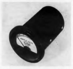
Basic sensitivity is 10MV rms, but it has a scaleplate with 2 ranges, 0-1 & 0-2.5, labeled Ripple Volts. An input resistor chain provides appropriate meter ranges for all the predicted ripple levels and is mounted right on one deck of an external selector switch while the second deck of the switch holds the 11 leads from the power supplies to be tested.
