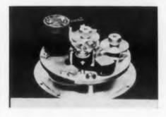
The "Glennite" Model KAT-1 is a tape-recording accelerometer system which can reliably measure accelerations up to  $\pm 60$ g in guided missiles, air, sea and land vehicles, underwa-
