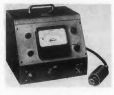
The Model P-2 Power Meter operates over the entire frequency range of d-c to 11,000Mc. Power is measured in three ranges: 0-1mw, 0-10mw, and 0-100mw. This unit is a true rms milliwatt indicating
