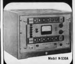
The simplicity and accuracy of Dekatron counting and timing circuits make the Ekco Model N-530A Automatic Scaler the most outstanding and most versatile instrument of its kind. This scaler will time a predetermined count, count for a pre-determined time, or can be manually operated.
