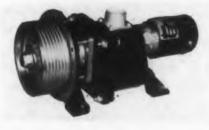
The Series 171 consists basically of a continuous-duty motor driving two counterrotating magnetic power clutches and gear reduction from the clutches to the output shaft. Its low-inertia factor is due to the magnetic powder clutches. Since the motor runs continuously, it is necessary to overcome only the inertia of the clutch and gearing during acceleration. The clutch has a torque-to-inertia ratio of 440,000-rad/see<sup>2</sup> and requires less than 1w to produce full output torque.
