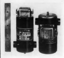
The Model T-198A "Pulsitometer" is a vibration-resistant keyer originally designed to be used in the overheat warning circuit of all aircraft gas turbine engines, whether jet or turboprop. It utilizes
