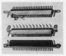
Complex, specialdesign, "Continental" connectors are now available from this firm on a mass production basis. A completely equipped tool room produces single cavity molds for prototype samples.
