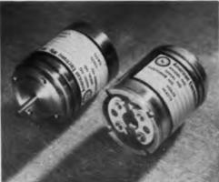
the order of 25 "G's" for 4 hours at 600 F. Finally, the potentiometer was subjected to 1050 F for 15 minutes. The terminal blocks molded of Dow Corning 301 Molding Compound were somewhat shrunken and charred, but the brass inserts were still firmly retained. No. 9
