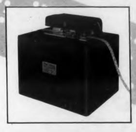
The Ferranti High Speed Tape Reader accelerates to full speed within 5 milliseconds and stops within 3 milliseconds. It has been in use at leading computer installations for over two years and has achieved a sound reputation for simplicity and reliability in regular operation.
