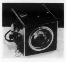
This instrument is specifically designed for the rapid measurement of speed and the study of rotating and vibrating or reciprocating mechanisms in slow motion. The objects to be viewed are illumi-
