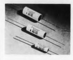
In these "Steacaps", steatite encased tubular paper capacitors, the capacitor section is assembled in a dense steatite tube that is a practically perfect moisture barrier. The ends
