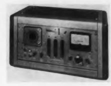
The Model 200 Scaler utilizes decimal or binary units which are directly interchangeable; it may be changed from one to the other in a matter of seconds. A direct-coupled
