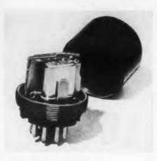
The Type VCO-2 temperature - controlled oven is for use with JAN type HC-6/U and HC-13/U crystals. The unit comprises a heavy anodizedaluminum housing arranged to accept two, two-prong mounted crystal units. The base of
