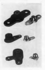
This all-metal self-locking miniature nut is designed to use only one-half the space of comparable standard anchor nuts and to be only one-fifth weight, thus effecting weight savings of 80%. It retains the full tensile strength of the original "Kaylock" selflocking standard anchor nut.
