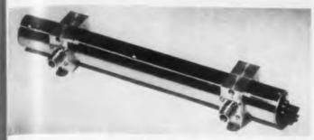
Based on several design innovations, the Model 81,-24-10M S-Band Traveling-Wave Tube is housed n a reduced-size package of 1-1/2" diam x 13" long, neluding the solenoid, and weighing approximately lb. Both dispersive and non-dispersive low-level ubes are currently being produced for S-band operaion, 2-4kMc.
