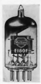
The Mullard E180F is a new miniature pentode with a high mutual conductance of 16.5ma. This, together with its low interelectrode capacitances, makes the tube ideal for all wide-band amplifier applications, such as radar i-f amplifiers, high definition television cameras and transmission equipment, and carrier telephone equipment, especially that used with coaxial telephone cables.
