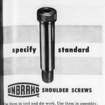
se them in tool and die work. Use them in assembly. These heat-treated alloy steel screws have knurled eads for sure finger grip and fast assembly; accurate ex sockets for positive nonslip internal wrenching. houlders are held to extremely fine tolerances, and inished threads run close up for maximum holding ower. Standard sizes—1/4" to 3/4" in a full range of ody lengths—are stocked by authorized industrial istributors. Write for Bulletin 877. STANDARD RESSED STEEL Co., Jenkintown 12, Pa.
