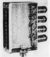
Two Digital Decade Counters, each available in three variations, are for use wherever high-speed electronic counting is required. Both types employ the printed circuit principle, thereby permitting maximum ventilation, low operating temperature and longer life.
