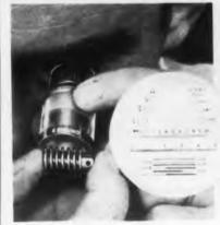
A "vest-pocker size version of th firm's pocket com parator, this tim device is about half the size of the larger unit. Its ma jor feature is real non-warpable etched-glass reticle instead of the film reticle found other low-price
