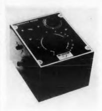
This "R.C." low-cost, completely self-contained, portable resistance - capacitance bridge is designed to increase the speed and accuracy of making measurements on capacitors from 10 mm/d to 50 mmfd, and resistors from 10 ohms to 50 megohms. It can also be used for mak-
