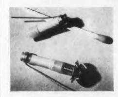
Only 3/4" in overall length, this midget glass rotary trimmer capacitor features a very low minimum capacitance and smooth trimmer adjustment. It is suitable for application in any commerical
