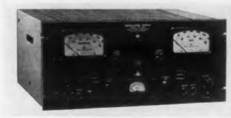
The Model D3-300D Power Supply provides two high-voltage output ranges, each independent of the other, on one compact chassis. It delivers 0-300v d-c at 300ma max load; 0-300v d-c at 150ma max; d-c variable bias 0-150v at 5ma max load (regulated by VR tube); and 0-10v a-c unregulated, at 10amp max load which is variable with powerstat control.
