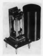
The P255A Polarized Relay utilizes a reed-type, Permaloy armature with anti-chatter contacts. The armature is equipped with extra-heavy (3/32" diam) palladium-copper contacts. The contact screws have 1/16" diam tungsten contacts rated at 2amp 110v d-c.
