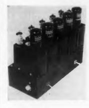
Making use of quickly interchangeable plug - in miniature decade counters, the direct-reading Model C-101 multiple decade counter employs one 30kc and four 10kc decade counters. The 30kc counter is provided with an input shaper circuit and is operable with inputs ranging from 6v to 50v.
