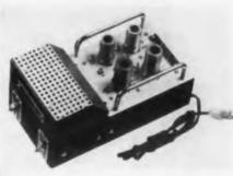
These converted are constructed the modular pri ciple of employi plug-in r-f secti to cover the v. spectrum from Me to 300Me. No figure at 150Me
