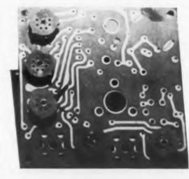
The printed-circuit board with sockets added.
