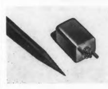
The dimensions of this standard series of subminiature bandpass filters are 23/32" x 23/32" x 1-1/16" high. The units have a 0.55 cu in displacement and exhibit excellent
