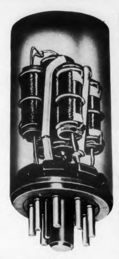
Five precision resistors attached to octal tube socket.
