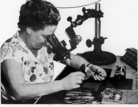
At the Hathaway Instrument Company, tiny galvamometer coils are wound with wire so fine that it is almost invisible to the unaided eye. Ingenious tooling and use of an AO Stereoscopic Microscope assure fast, precise workmanship.
