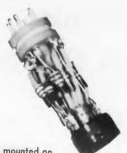
Components are mounted on a turret socket prior to the encapsulation process.
