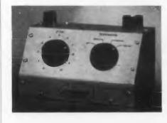
The Model GD-D2-1000-1 Decade Delay Line has an overall delay of 1µsec. Dial-selected taps are at 0.1µsec intervals. Impedance is 1000 ohms, and overall rise time is 0.1µsec.
