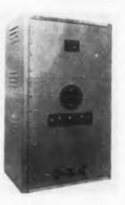
The Model 1420-B Variable Frequency Electronic Generator is a versatile power source for use in the development or testing of equipment operating over a range of power supply frequencies. The frequency range of its internal oscillator is 50-6000ey with an external oscillator of 25ey-20kc.
