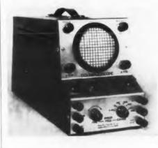
This D-C "Midgetscope", Model No. 534, combines linear sweep with d-e amplifier for color TV restorer circuits and for complex waveforms. Other features include provisions for a-c coupling; full
