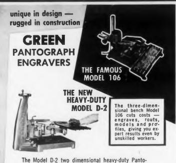
The Model D-2 two dimensional heavy-duty Pantograph is a precision machine with a multitude of new features. Open on three sides, it permits complete freedom for engraving, milling, profiling large panels (up to 30" in diameter) or bulky pieces. Single, micrometer adjustment controls vertical depth of cut, automatically adjusting copy table with pantograph. Range of reduction ratios from 2-to-1 to infinity! Vertical range over 10 inches!
