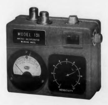
The model #131 "S" Band Wavemeter (Amerac's version of the popular military model TS-117) covers the frequency range from 2400 MC to 3400 MC in 16 revolutions of the micrometer thimble, by either the transmission or absorption method.
