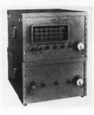
The 8Mc Counter Chronograph, Model 471, is a rugged instrument for testing radar and sonar equipment. It is designed to permit calibration and other detailed tests under field or shipboard conditions. Housed in two drip-proof heavy-gage reinforced aluminum cabinets, it con-
