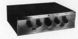
The cabinet (4" x 14-1/2" x 11-1/2") of the Radio Craftsmen "Solitaire" has a simulated leather finish. The bottom view of the chassis shows the diagonally mounted tubes and input and output terminals.
