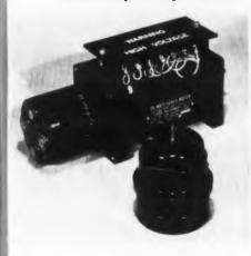
This precision a-c Rate Generator is designed for any use which requires a high degree of accuracy in the linear translation of rotational motion into voltage. It is a "drageup tachometer" incorporating a specially
