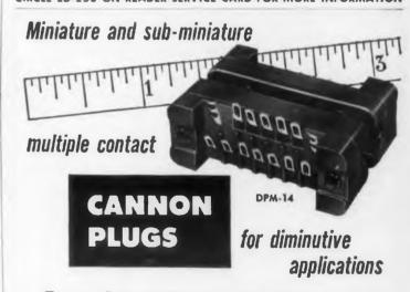
Turn to Cannon when you want midget connectors! Type DPM-14 illustrated has 2 (10 amp.) No. 16 and 12 (5 amp.) No. 20 brass contacts. Entire assembly only ¾" x 2". Similar unit, Type DPM-A20 has 2 No. 16 and 18 No. 20 contacts. Ideal for rack, panel, and instrument applications.
