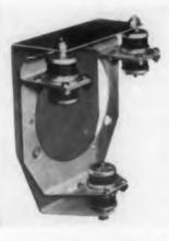
This mounting system. Model 1102, incorporates three all-metal double-act ing mounting units. Located in the vertical plane of the center-of-gravity of the instrument, the mount ing units combine to give a natural frequency of ap proximately 15cy. Effectively isolating vibration and shock forces, the sys-
