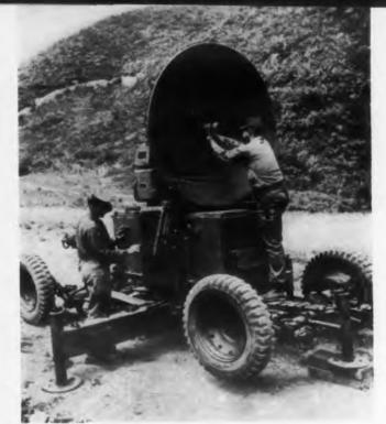
Mortar-Detecting Radar... The development of a mortar-detecting radar, already battle proven during the Korean war, has been announced by the U. S. Army. Within a short time after an enemy mortar commences firing, the detector system relays its position to an artillery fire direction center. Artillery fire is then pin-pointed on the mortar.
