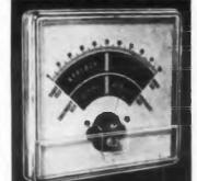
The Model No. 23 Meter can be provided in all ranges of microamperes. milliamperes, amperes. volts, and millivolts. It is available for use in electronies, automotive, radio. radio test equipment, industrial equipment, and all other types of equipment wherever an indicating
