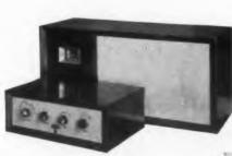
The wooden cabinet of the Altec-Lansing "A-339A Melodist" matches the cabinet of this firm's "700A Melodist" speaker. The heat shield over the rectifier and power tubes of the amplifier produces a "chimney effect".
