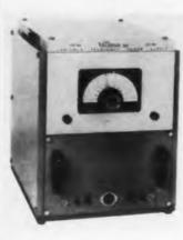
The Model VFS - 250 Variable Frequency Power Supply is a compact, semiportable source of 45cy to 2000cy alternating current, with available output up to 300va. Voltage, frequency, and power output of this multi-purpose frequency changer make it suitable for three main categories of use: (1) testing airborne electronic and
