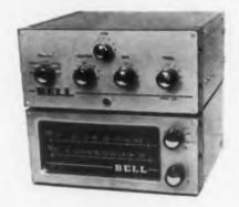
The Bell "2256" (top) is the same size (4" x 9-1/2" x 8-3/4") as the "2255" tuner. The bottom view of the unit shows its "split-chassis" construction, which also aids cooling.
