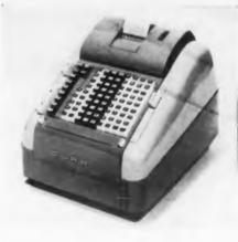
This Time-Data Printer, can record (1) one or two sets of manually or remotelyentered data, (2) an entry identification number or symbol, and (3) the time-of-day when the data are taken. Time is indicated to 0.01
