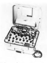
This dynamic tube tester, Model VTT-1, is capable of measuring the true dynamic mutual conductance as well as the plate current of all tubes normally encountered in electronic work, including sub-miniature, ruggedized, and hearing-aid tubes. Actual operating conditions of the
