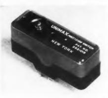
A movement differential of only 0.0005" maximum and low actuating force, combined with high repeat accurracy, are featured in Series WHB precision snapswitches. These
