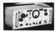
Model 541-A (TS - 710/TSM)Crystal Impedance Meter is designed to measure directly the effective resonance and antiresonance of quartz
