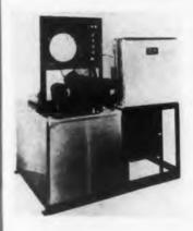
This low cost, low temperature test cabinet is especially designed for occasional testing and where the power supply is limited or no water is available for cooling freon. It utilizes dry ice as a refrigerant which is placed in a holding tank and immersed in brine. The brine is then circulated through cooling
