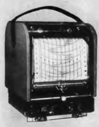
MAGNETIC FLUID CLUTCH meter movements make possible a sensitivity of 0.45 inch per 100 microamps combined with adherence to rigid military aircraft requirements for shock, vibration, explosion, and humidity resistance. High resultant torque permits the startling reduction in recorder size and weight and creates a new degree of independence from shock, vibration and pen drag.
