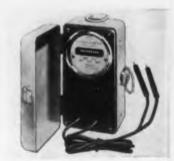
Insulated test probes are provided for shunting a portion of the voltage in the tested line across the are 10,000-ohm internal resistance of the meter. An electromagnetic coil-armature combination applies mechanical energy at the frequency to be measured to lat 4 the entire row of reeds. Only the reed having a nat a sp ural frequency corresponding to line frequency will latio undergo vibrational response.
