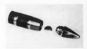
Only I" long, this plastic encapsulated transmitter has an even smaller mercury battery beside it. The transmitter and 200hr cell fit into the nose of the illustrated projectile.
