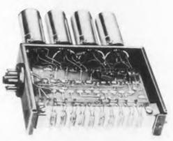
The neon lamps (bottom) on this Detectron Decade Totalizer indicate one digit of the count.
