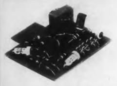
Fig. 2. Transistorized amplifier mounted on phenolic printed circuit board.
