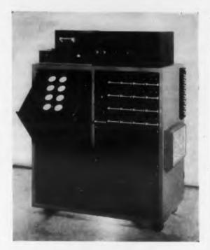
Time marks are regularly recorded on the left edge of the record paper by the oscillograph.
