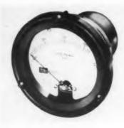
Voltage readings accurate to 0.5% over the frequency range of 50cy to 2000cy are obtained with the "Expanded Scale Panel Voltmeter". Use of a thermal bridge permits the indication of a narrow voltage
