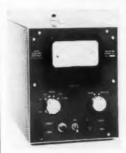
The Model D-1 "Regmeter" provides direct measurement of power supply internal resistances without a complex laboratory setup. It measures from 0.02 ohms to 1,000 ohms in voltage sources with outputs ranging from 0 to 500v. The instrument may also be used as an accurate, stable a-c voltmeter
