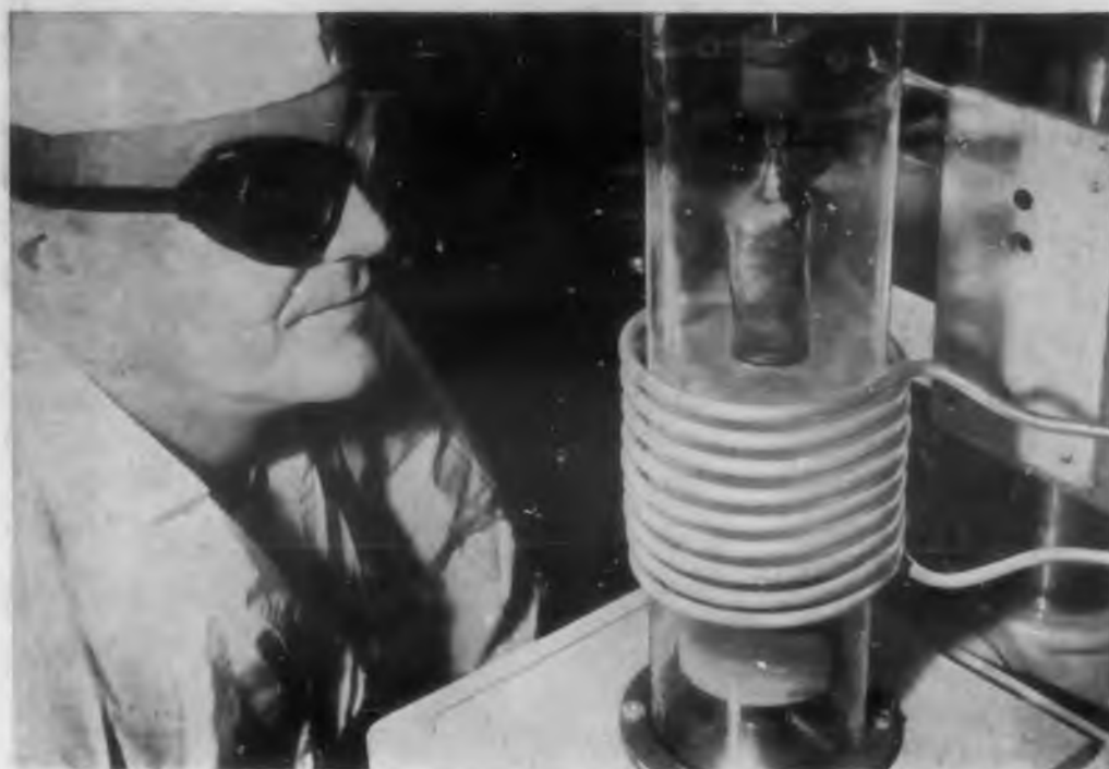
"Growing" germanium in an induction furnace for use in the new Honeywell H-2 Power Transistor
