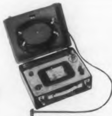
Model H. 0-6000 fpm at 2% accuracy. Continuous calibration check. $175.00
