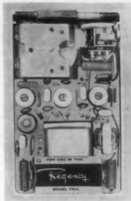
The chassis is a printed circuit board. The bar antenna is mounted at the top.
