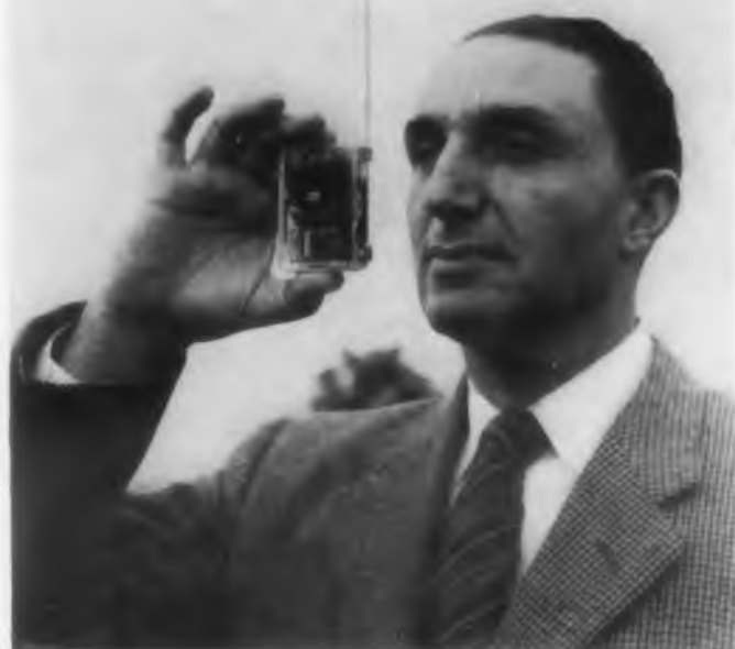
The solar-powered transmitter is being operated by its inventor, Edward Keonjian. The unit is 3" high x 2-1/2" wide x 5/8" thick, weighs 3-1/2 oz.
