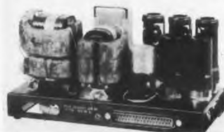
Fig. 5. The amplifier power supply subassembly.
