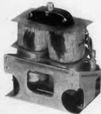
Fig. 2. One of the three control-transformer servo amplifiers.
