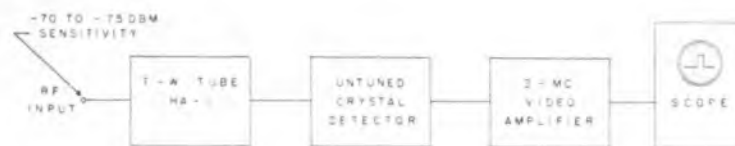
Fig. 4. Block diagram of a simple untuned receiver using the Amplifier.
