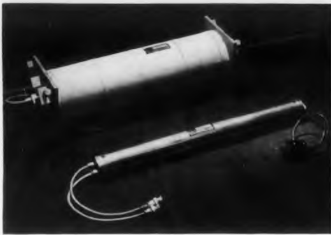
Fig. 1. The complete Type HA-1 Traveling-Wave Tube Amplifier (above) with the capsule containing the traveling-wave tube.
