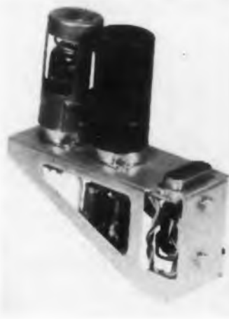
Fig. 4. The time motor in the computer is driven by a signal generated by this subassembly.
