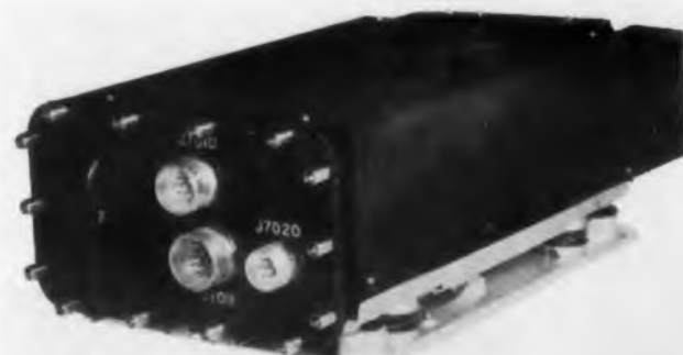
Fig. 8. The complete amplifier with its specially designed shock mount.
