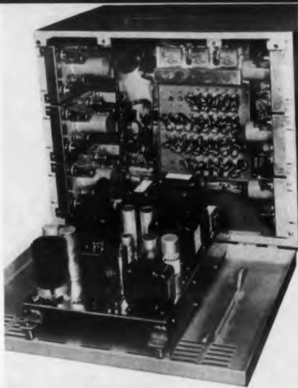
Fig. 6 (right). Power supply circuit for positive voltages. The required +100v is obtained through dropping resistors. The negative circuit is similar. The six voltages are then fed to regulator circuits.
