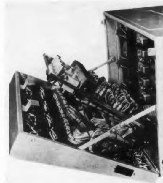
Fig. 3 (above and right). Two views of the front panel swung down showing how easily all components can be reached. All complex wiring is done on the rear of this panel and flexible cables are provided for the amplifiers and supply. The unit requires no internal cabinet wiring. Notice the open grid floor for cooling.
